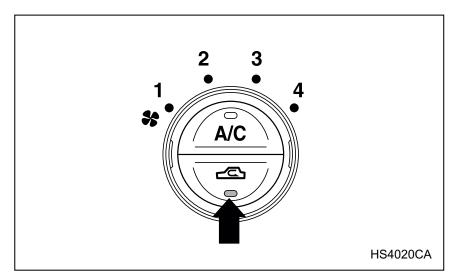
ON (Recirculation): Interior air recirculates inside the passenger compartment. Use this position when quickly cooling down the passenger compartment or to prevent outside air from entering the passenger compartment. The indicator light comes on when the "Recirculation" mode is selected.
