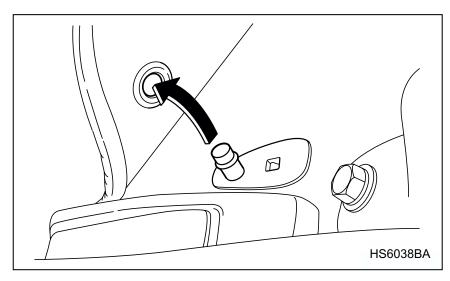
A retaining pin is located on the driver's side of the vehicle next to the fuel filler door release.
