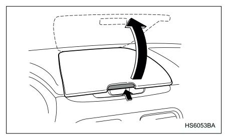
To open the dashboard compartment, push the button on the lid and the lid will automatically open. Be sure to close the compartment fully before driving.
