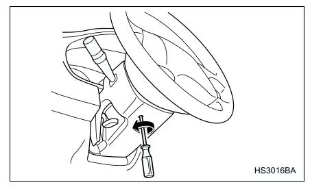
2. Remove the cover under the steering column using a phillips screwdriver.
