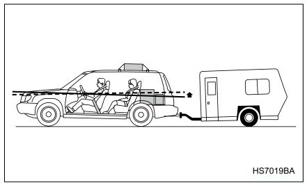
The self-leveling system is incorporated in the rear suspension shock absorber and operates only when the vehicle is in motion.
