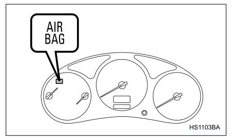
A diagnostic system continually monitors the readiness of the seatbelt pretensioner while the vehicle is being driven. The seatbelt pretensioners share the control module with the SRS airbag system. Therefore, if any malfunction occurs in a seatbelt pretensioner, the SRS airbag system warning light will illuminate. The SRS airbag system warning light will show normal system operation by lighting for about 6 seconds when the ignition key is turned to the "ON"
