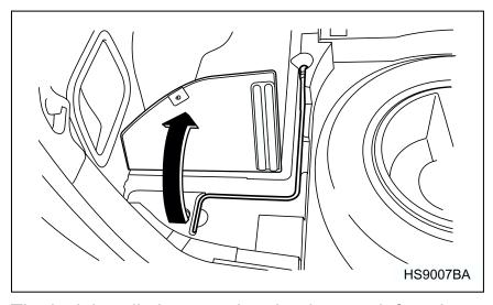
The jack handle is stowed under the rear-left and center lids in the cargo area.
