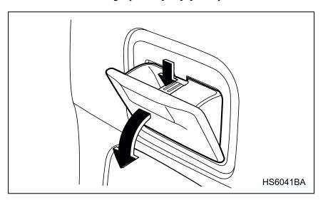
To open the ashtray, pull the upper edge of the lid. Fully close the lid after using it to help reduce residual smoke.
