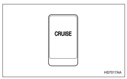
Cruise control enables you to maintain a constant vehicle speed without holding your foot on the accelerator pedal and it is operative when the vehicle speed is 25 mph (40 km/h) or more. Make sure the main switch is turned "OFF" when the cruise control is not in use to avoid unintentionally by setting the cruise control.
