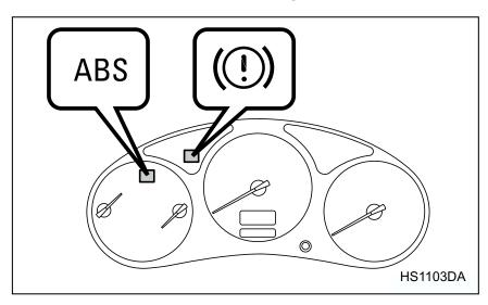
If a malfunction occurs in the EBD system, the system stops working and the brake system warning light and ABS warning light come on simultaneously.
