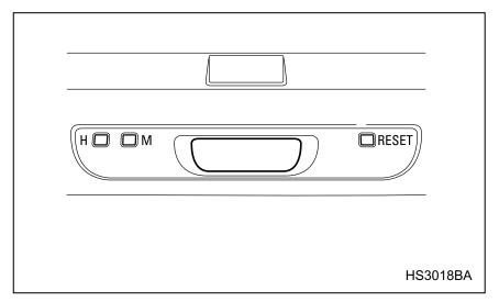
To set the hour, press the "H" button. To set the minutes, press the "M" button. To reset the minutes to "00" with a radio time signal, push the "Reset" button.
