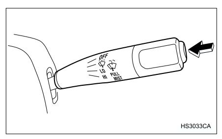
To wash the windshield, push the washer button at the end of the wiper control lever. The washer fluid sprays until you release the washer button. The wipers operate while you push the button.
