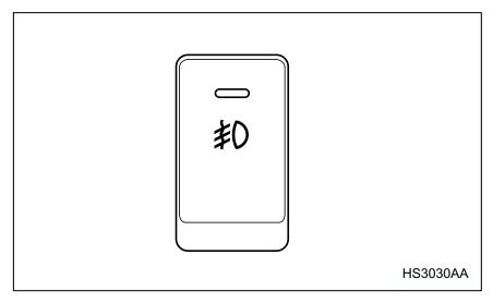
The fog lights operate only when the headlights are on low beam. Push the fog light switch to turn the fog lights on.
