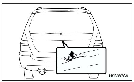
To open the rear gate, first unlock the rear gate lock then pull the outside handle up.
