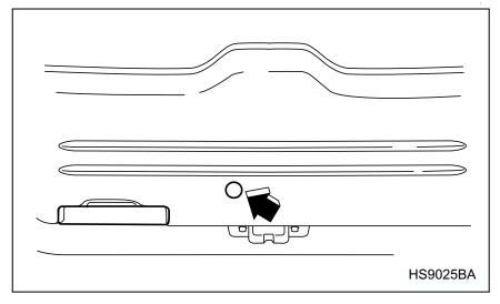
1. Remove the access cover at the bottom-center of the rear gate trim.
