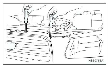
1. Remove the front grille. Use a screwdriver to detach the four clips at the top and the three hooks on the left, right and center.
