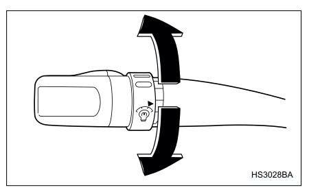
When the lighting switch is in the " $\exists DO\Xi$ " or " $\equiv D$ " position, you can adjust brightness of the instrument panel illumination for better visibility.
