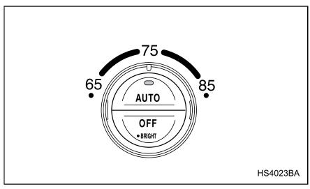
When the "AUTO" switch is pressed, the indicator light on the switch illuminates, indicating that the Automatic Climate Control system is operating in the automatic mode. In the automatic mode, the system maintains the desired cabin air temperature (this is set using the temperature control dial) by automatically controlling the fan speed, air flow mode, air inlet selection, and air conditioner compressor operation.
