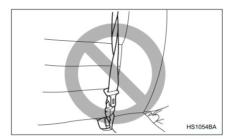
Fastening the seatbelt with the webbing twisted can increase the risk or severity of injury in an accident. When fastening the belt after it is pulled out from the retractor, especially when inserting the connector's tongue plate into the mating buckle (on right-hand side), always check that the webbing is not twisted.
