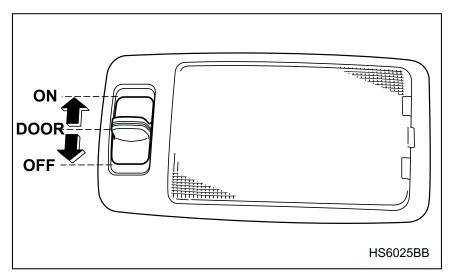
The dome light switch has three positions:
