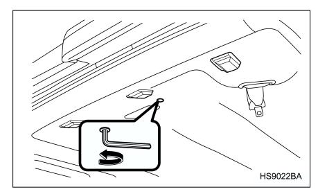
2. Insert a hex-headed wrench in the end of the motor shaft.
