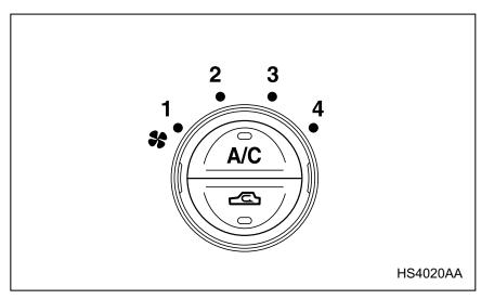
The fan operates only when the ignition switch is in the "ON" position. Select any of the four fan speeds by turning the fan speed control dial. The selected fan speed is indicated by illumination of the corresponding indicator light around the dial.
