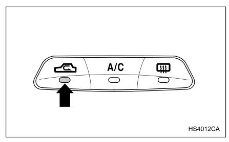
**ON position (Recirculation):** Interior air is recirculated inside the vehicle. Push the air inlet selection button to the ON position. The indicator light will come on.
