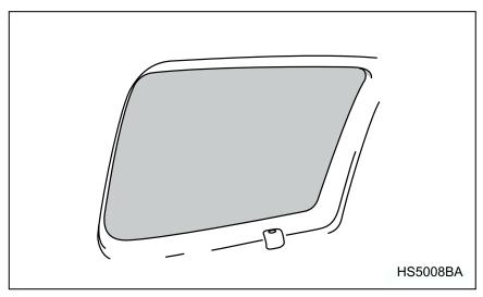
The antenna is printed on the inside of the left side rear quarter window glass.
