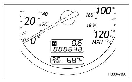
The ambient temperature gauge shows the ambient temperature in a range from –22° F to 122° F (–30° C to 50° C).
