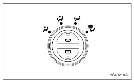
Select the desired air flow mode by turning the air flow control dial. The selected air flow mode is indicated by illumination of the corresponding indicator light around the dial.
