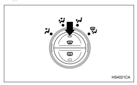
To defrost or dehumidify the windshield and side windows, push the defroster switch " \( \frac{\pmathbb{H}}{\pmathbb{N}} \) ". When the " \( \frac{\pmathbb{H}}{\pmathbb{N}} \) " switch is pushed, regardless whether the air conditioner is operating or not, outside air is drawn into the passenger compartment, the air conditioner compressor turns on, air flow is directed towards the windshield and side windows, and the indicator light on the switch comes on.
