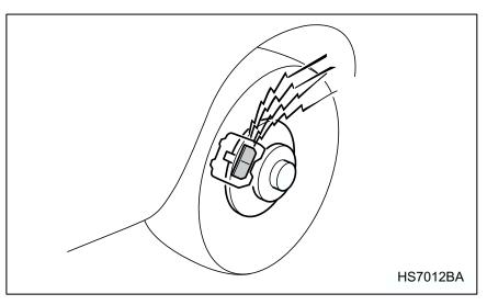
The front disc brakes and the right rear disc brake have an audible wear indicators on the brake pads. If the brake pads wear close to their service limit, the wear indicator makes a very audible scraping noise when the brake pedal is applied.
