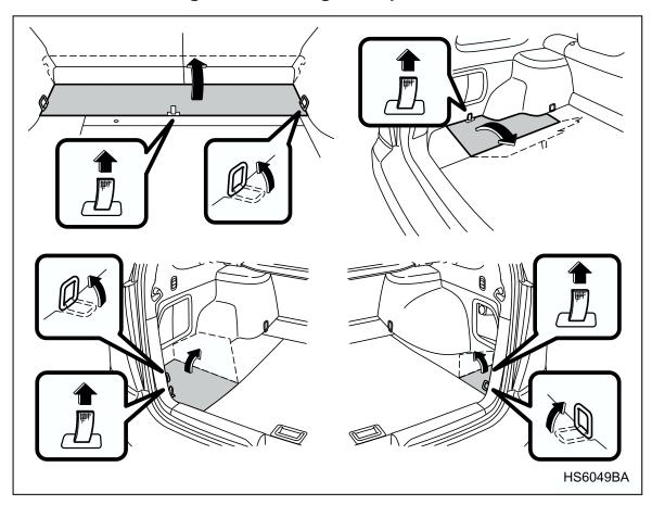
To open the lid, raise the cargo tie-down hooks and pull the tab up. The jack and jack handle are stored in the left side storage compartment.
