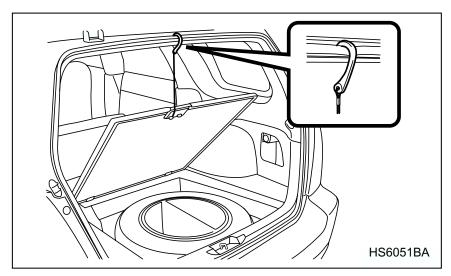
To keep the lid open, hang the hook provided on the backside of the lid on the rear edge of the roof. The storage bucket is put on the spare wheel.
