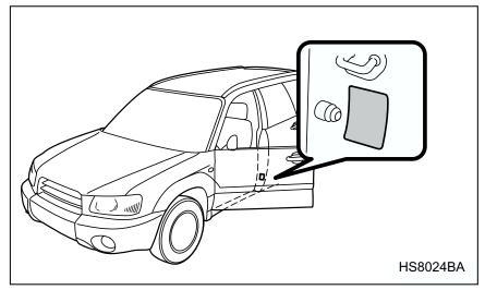
The load capacity of your vehicle is determined by weight, not by available cargo space. The maximum load you can carry in your vehicle is shown as the Vehicle Capacity Weight on the tire information label attached to the driver's side door jamb. It includes the total weight of driver and all passengers and their belongings, any optional equipment such as a trailer hitch, roof rack or bike carrier, etc., and the tongue load of a trailer.
