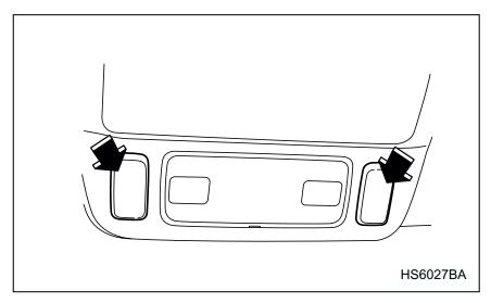
To turn on the map light, push the switch. To turn it off, push the switch again.
