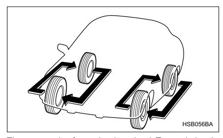
Tire wear varies from wheel to wheel. To maximize the life of each tire and ensure that the tires wear uniformly, it is best to rotate the tires every 7,500 miles (12,500 km). Rotating the tires involves switching the front and rear tires on the right-hand side of the vehicle and similarly switching the front and rear tires on the left-hand side of the vehicle. (Each tire must be kept on its original side of the vehicle.)
