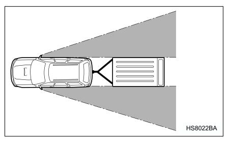
After hitching a trailer to your vehicle, check that the standard side mirrors provide a good rearward field of view without significant blind spots. If significant blind spots occur with the vehicle's standard side mirrors, use towing mirrors that conform with Federal, state/province and/or other applicable regulations.
