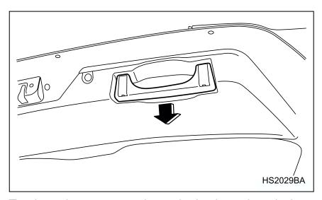
To close the rear gate, lower it slowly and push down firmly until the latch engages.
