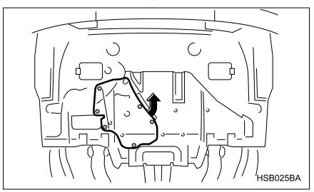
4. Open the access cover by removing the six clips and turning the access cover counterclockwise. The drain plug and oil filter will be exposed.
