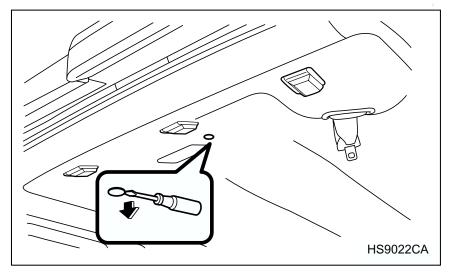
1. Remove the plug on the roof trim located to the rear of the moonroof by inserting the end of the regular scredriver between the roof and plug and prying it off.
