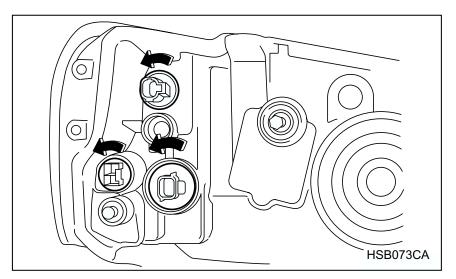
6. Remove the bulb socket from the headlight assembly by turning it counterclockwise.
