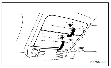
To open the console, push on the console lid lightly and the lid will automatically open.
