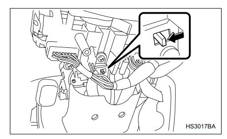
3. Turn the ignition key while pressing the key interlock release lever.
