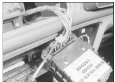
23.11b Disconnecting the wiring plug from the graphic display unit
