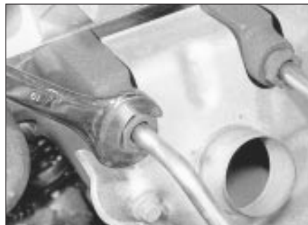
22.4 Unscrewing a pulse-air delivery tube union
