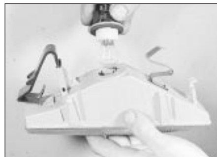
48.15 Removing a front direction indicator lamp bulb - models up to 1987
