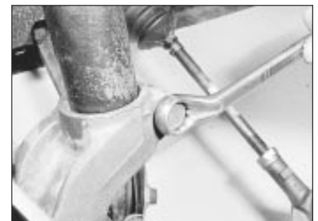
5.8 Unscrewing the hub carrier-to-strut pinch-bolt
