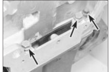
18.16 M8 cylinder head bolts (arrowed) located at front of cylinder head
