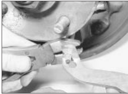
5.9 Disconnecting the handbrake cable from the trailing shoe lever
