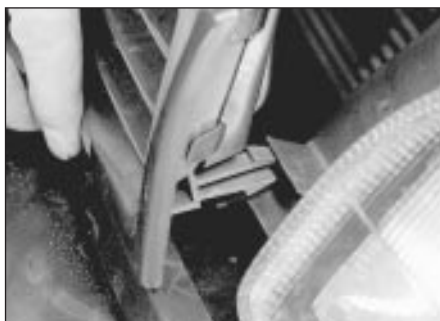
32.8 Removing the later type front grille panel
