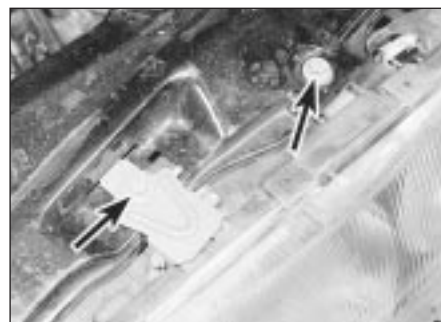
41.4a Remove the upper headlamp securing bolts (arrowed) ...
