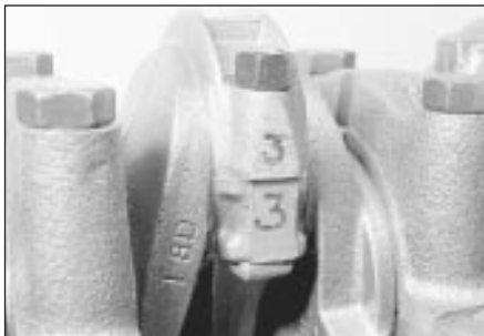
32.2 Big-end cap and connecting rod identification numbers
