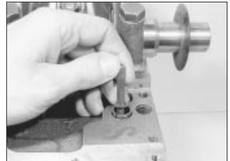
30.4 Withdrawing the oil pump driveshaft
