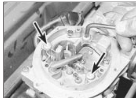
19.5 Removing the carburettor securing screws (arrowed) - Pierburg 2V carburettor
