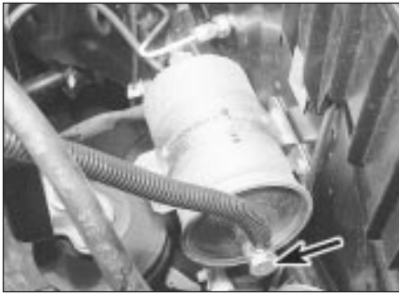
41.1 Fuel filter location - outlet union arrowed
