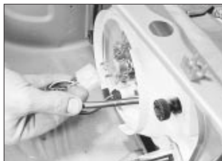
48.3a Pull off the wiring plug . . .
