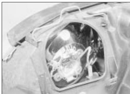
48.11 Auxiliary driving lamp bulb location - models from 1987
