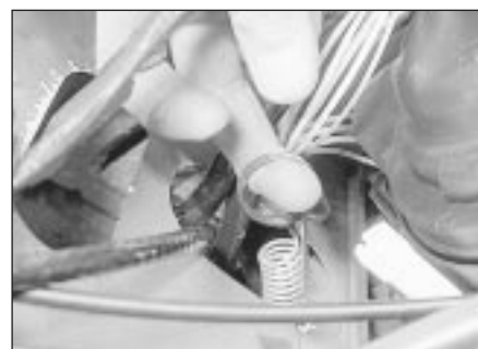
44.8a Unhook the front direction indicator lamp unit anchor spring ...
