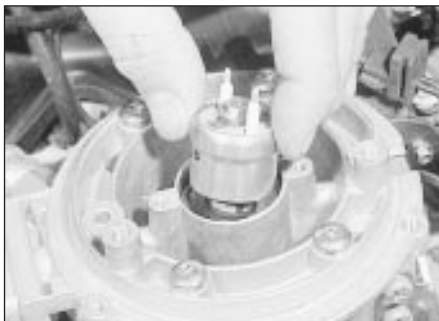
16.6 Withdrawing the fuel injector
