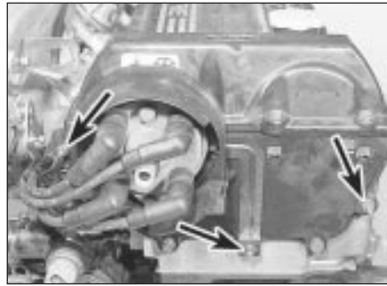
18.53 Upper timing chain cover securing stud locations (arrowed)
