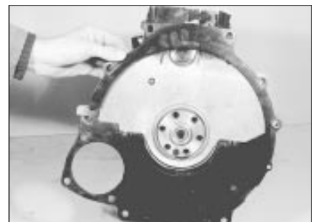
26.5 Withdrawing the engine adaptor plate
