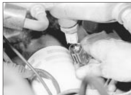
19.4 Disconnect engine temperature sensor wiring plug - ESC II system
