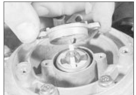
16.5b Removing the injector retaining collar
