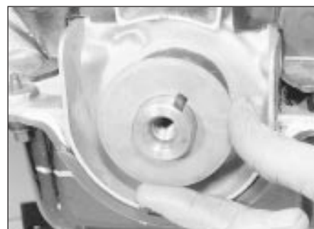
18.10c ... and the thrustwasher - 1.8 litre (R2A)
