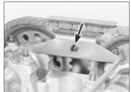
18.7a Upper timing chain guide securing lugs (arrowed)
