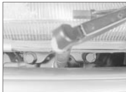
40.5b ... for access to the headlamp wiper motor mounting bolts
