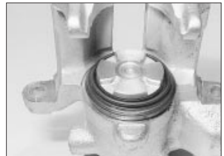
7.27 Dust-excluding seal fitted to piston and caliper bore
