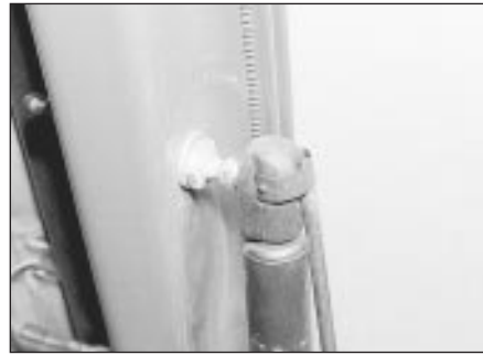
11.5 Prising out a tailgate strut retaining clip
