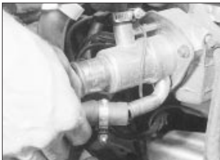
7.12a Disconnect the automatic choke hose...
