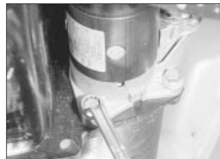
8.5 Unscrew the starter motor mounting bolts
