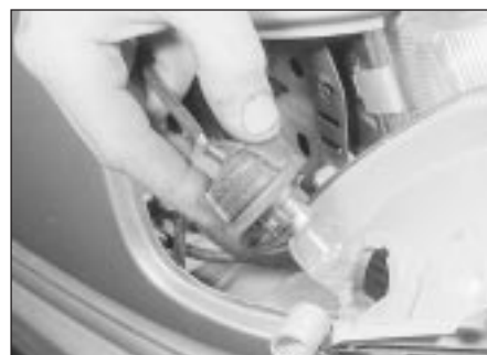
48.18 Removing a front direction indicator lamp bulb - models from 1987
