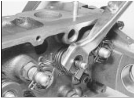
22.2a Compressing a valve spring
