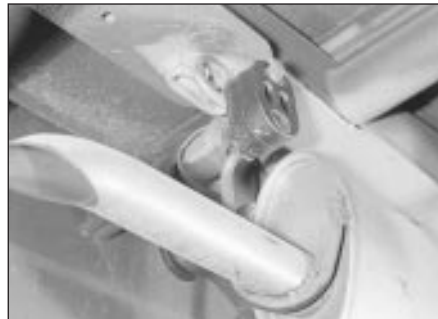
27.5b Rear exhaust mounting - P100 model
