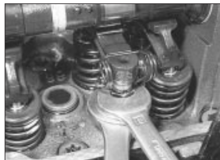
23.7b Adjusting a valve clearance
