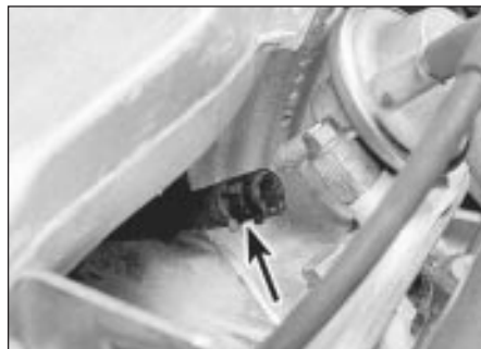
6.10 Disconnecting the fuel return hose (arrowed) from the pressure regulator
