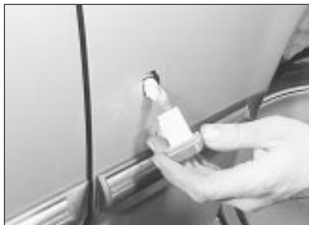
45.4 Withdrawing a front direction indicator side repeater lamp - models up to 1987
