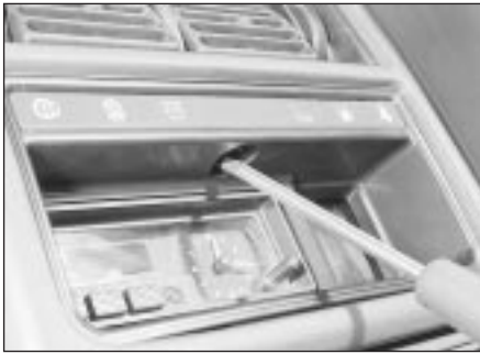
23.7 Remove the screw from the warning lamp facia panel
