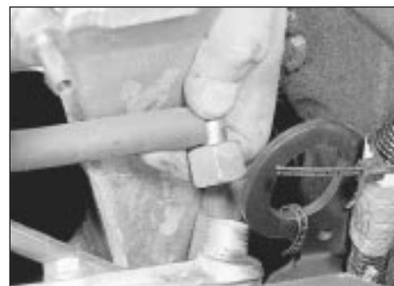
18.18 Disconnecting the fuel feed hose from the fuel rail
