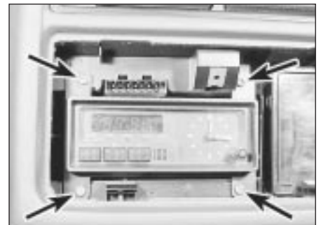
19.6 Multi-function digital/analogue clock securing screws (arrowed)
