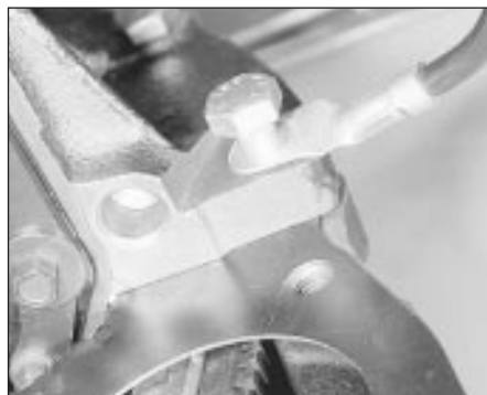
8.22a Earth strap location under engine-to-gearbox bolt - 1.8 litre (R2A)
