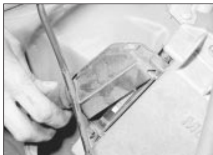
18.3b Disconnecting ESC II module wiring plug
