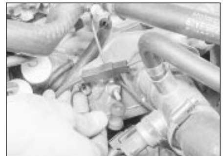
16.3b Disconnect the temperature gauge sender wiring - CVH
