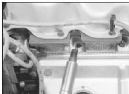
20.6 Removing a spark plug - CVH engine
