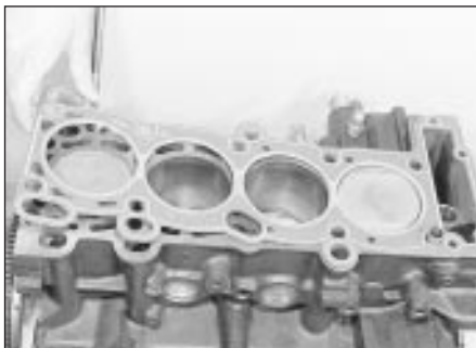
18.22 Fitting a new cylinder head gasket
