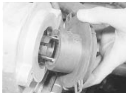
14.9 Removing the rotor housing
