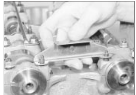
18.30c Fitting the timing chain guide plate
