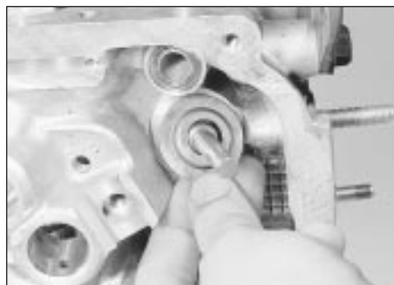
21.3a Remove the spring seat . . .
