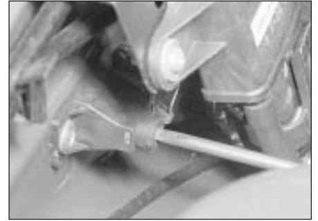
16.34b . . . to enable mixture adjustment - DOHC models
