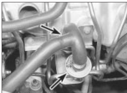
8.36 Pulse-air system check valves (arrowed) - 1.6/1.8 litre (R6A)
