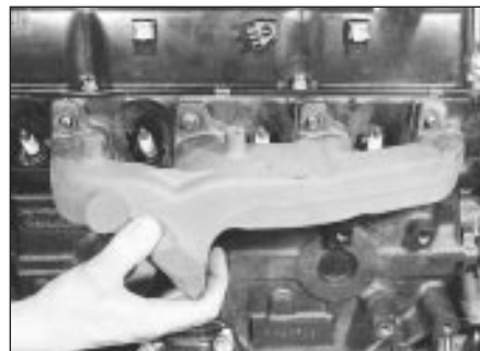
26.6c . . . and lift off the exhaust manifold - SOHC models
