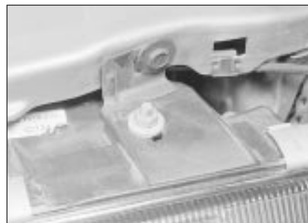
41.10b . . . the upper securing nut . . .
