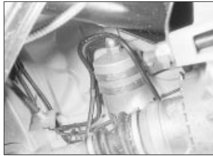
41.10 Fuel filter location (arrowed) under rear of vehicle
