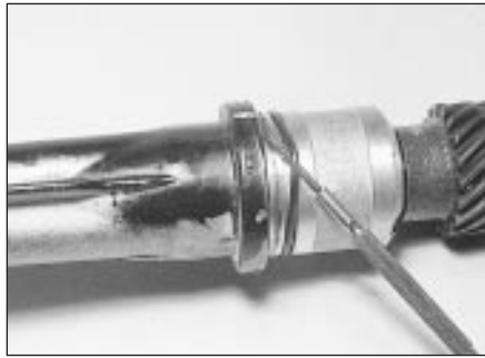
15.12 Removing distributor driveshaft O-ring - Motorcraft distributor
