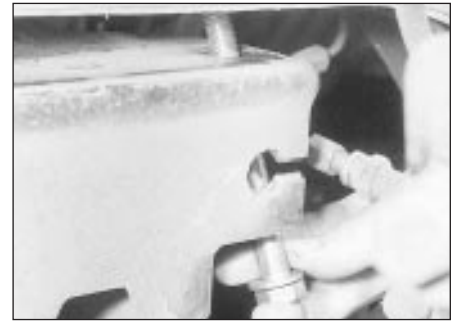
5.38 Removing a suspension crossmember securing bolt
