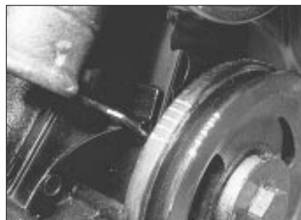
16.2a Highlighted timing marks - SOHC engine with cast crankshaft pulley
