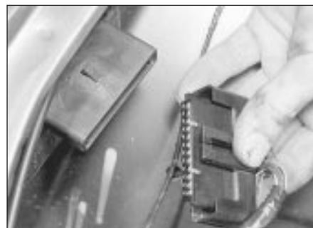
18.22 Disconnecting the ignition module wiring plug
