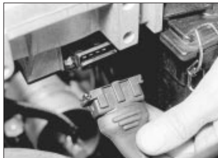
38.6 Disconnecting the airflow meter wiring plug
