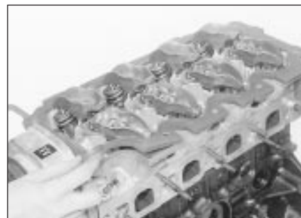
20.14 Ensure that the camshaft cover gasket locates over the edges of the cylinder head - 1.8 litre (R2A)
