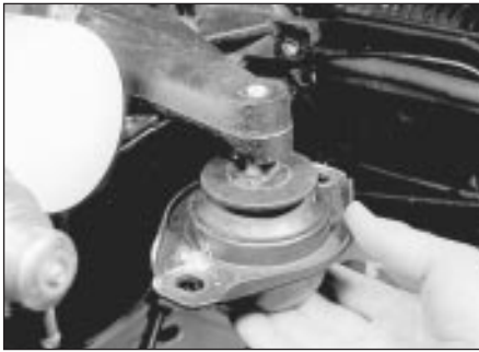
17.4 Withdrawing an engine mounting
