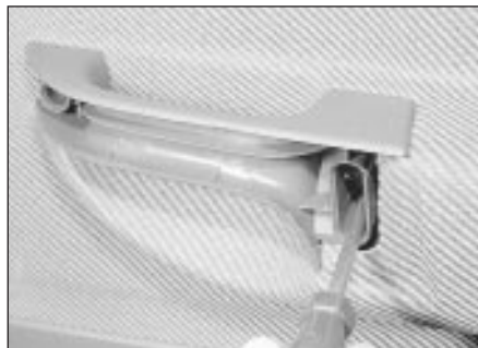
17.10b . . . and remove the armrest securing screws
