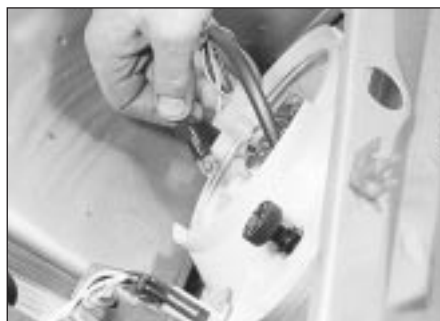
48.6 Removing a sidelamp bulbholder
