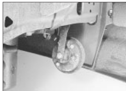
29.1 Horn location beneath front panel
