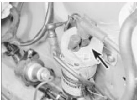
12.1 Ignition coil - CVH model. Plastic cover arrowed
