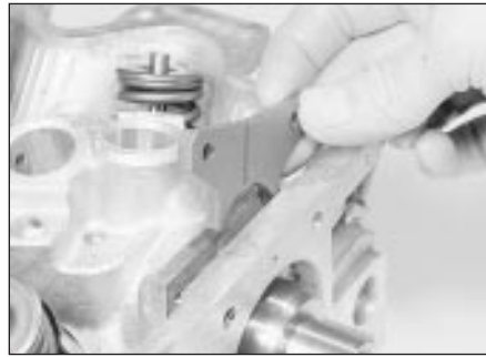
23.11a Refit the camshaft thrustplate . . .
