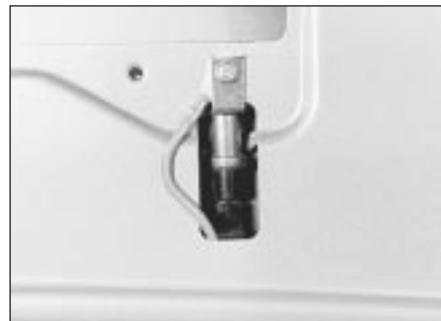
13.4 Luggage compartment lamp switch location - models up to 1987
