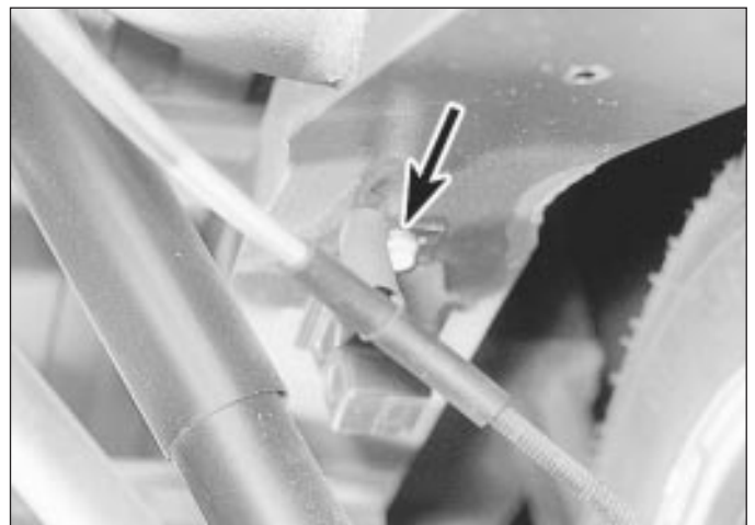
27.7 Handbrake cable support spring (arrowed)
