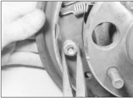
5.7 Using pliers to remove a shoe hold-down cup
