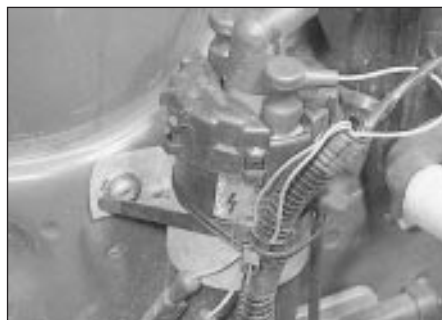
12.8a Ignition coil viewed with heat shield removed
