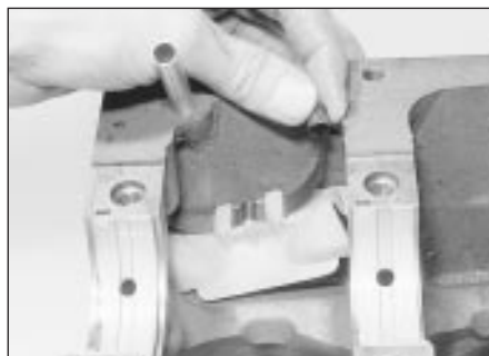
34.1 Removing the crankcase ventilation baffle
