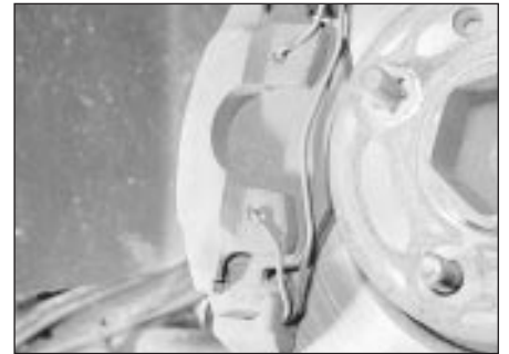
4.21a Later type front disc pad retaining clip
