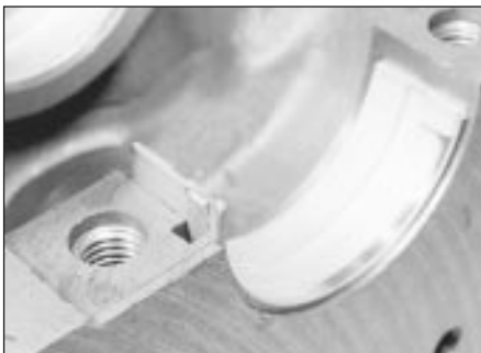
32.13a Rear main bearing shell in cylinder block - 1.8 litre (R2A)
