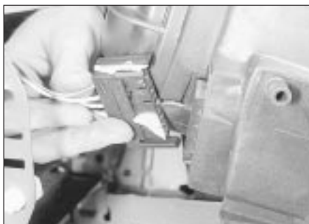
41.8 Disconnect the headlamp wiring plug - models from 1987
