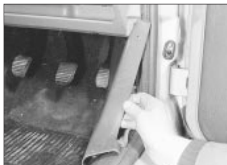
43.2 Withdraw the side trim panel from the footwell
