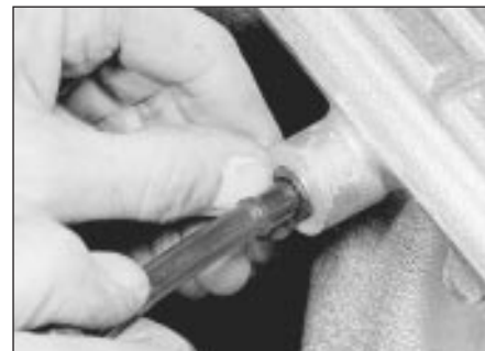
14.10 Disconnecting a later-type brake servo vacuum hose
