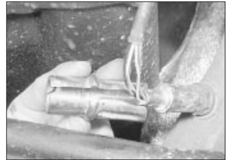
35.5 Sliding the heat shield from the exhaust gas oxygen sensor
