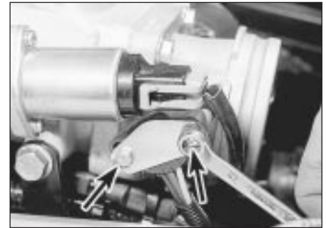
27.3 Unscrewing the throttle position sensor retaining bolts
