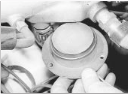
19.11 Removing inlet manifold heater - ESC II system
