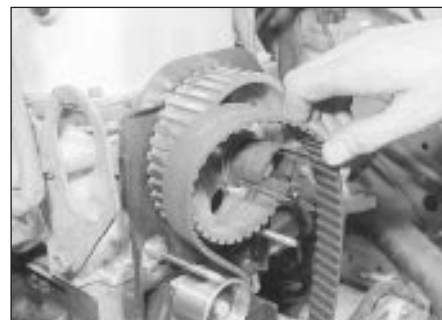
18.8 Withdrawing the timing belt - 1.8 litre (R2A)
