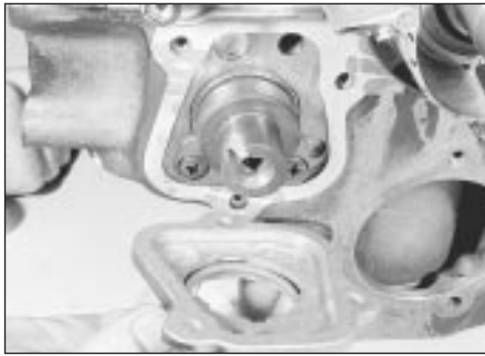
25.4 Unscrew the auxiliary shaft cover securing bolts and remove the cover
