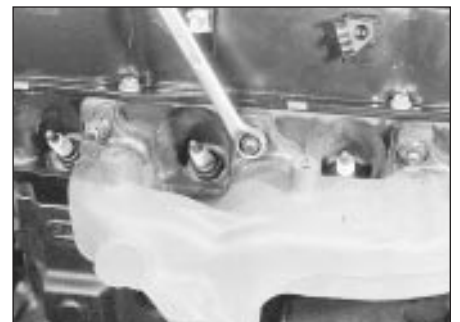
26.6a Unscrew the exhaust manifold securing nuts . . .
