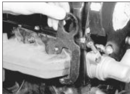
26.6b . . . noting the location of the front engine bracket . . .
