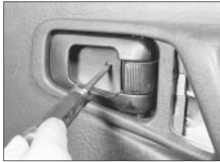
17.3a Remove the securing screw . . .
