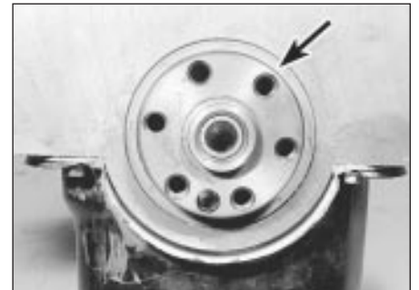
28.2 Crankshaft rear oil seal location (arrowed)
