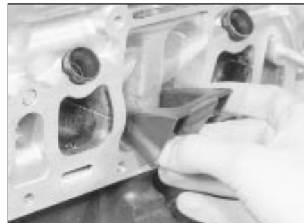
30.32 Removing a spark plug spacer from the cylinder head recess
