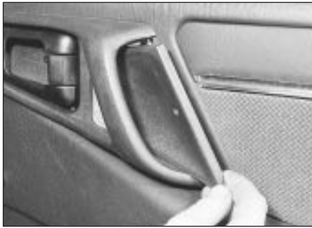
17.2 Withdraw the trim panel from behind the door grip
