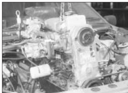
8.29 Lifting the engine from the vehicle - 1.8 litre (R2A)
