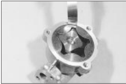
31.10a Checking the oil pump outer rotor-to-body clearance
