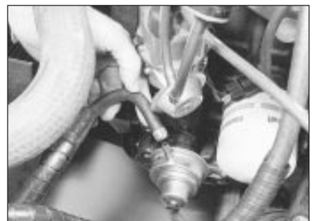
7.3 Disconnecting outlet hose from fuel pump - SOHC model
