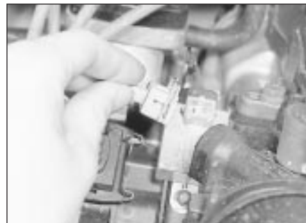
12.11b . . . and the suppressor wiring plug
