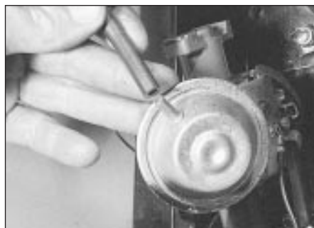
15.6 Disconnecting vacuum pipe from vacuum advance unit - Bosch distributor
