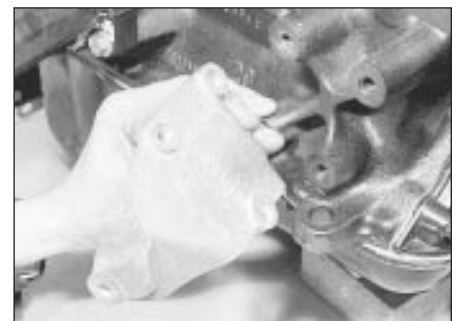
18.10b Removing the alternator mounting bracket
