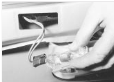
27.24 Removing a luggage compartment lamp bulb
