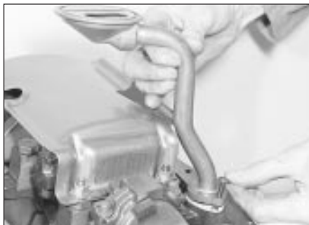
29.2 Removing the oil pick-up pipe
