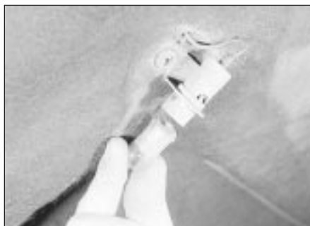
28.6 Removing an underbonnet lamp bulb
