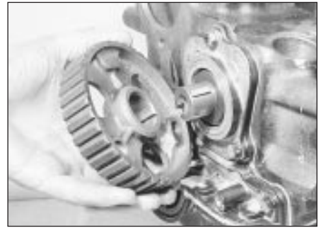
19.13 Removing the auxiliary shaft sprocket
