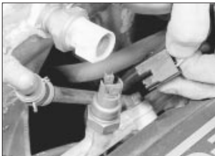
21.42 Disconnecting the fuel temperature sensor wiring plug
