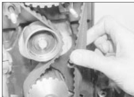
18.25 Twisting the timing belt to assess its tension - 1.8 litre (R2A)
