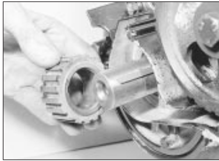
19.11 Removing the crankshaft sprocket
