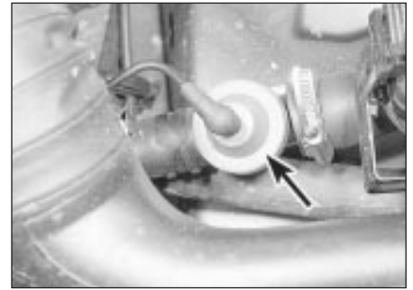
21.1 Pulse air system vacuum-operated air valve (arrowed)
