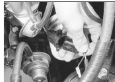
15.8 Disconnecting distributor wiring plug - Bosch distributor
