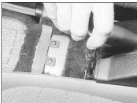
44.3a Removing a rear upper console panel front retaining screw - "high specification" model
