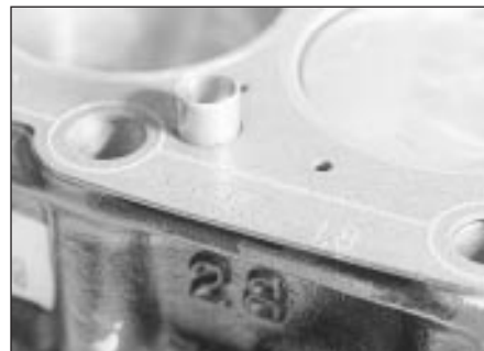
20.10b . . . then locate a new gasket with the red sealing bead and "1.8" mark uppermost - 1.8 litre (R2A)
