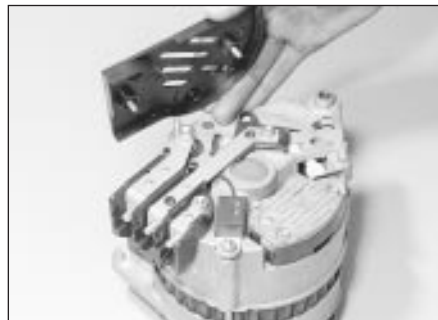
7.13 Removing the terminal cover from a Lucas A127 alternator.
