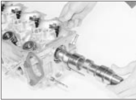
23.10 Refitting the camshaft - 1.8 litre (R2A)
