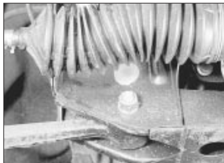
3.2 Front suspension lower arm-to-crossmember pivot bolt and nut
