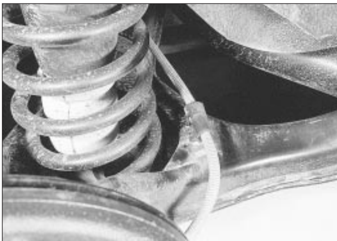
27.6 Handbrake cable-to-lower suspension arm attachment
