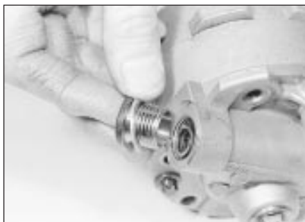
27.5a Unscrew the pressure relief valve plug and washer . . .
