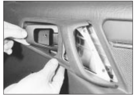
17.3b . . . and withdraw the handle surround and door grip
