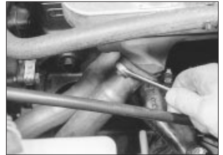
26.4 Unscrewing an exhaust downpipe securing nut
