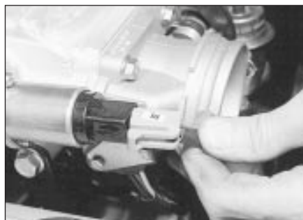
13.2 Disconnecting the idle speed control valve wiring plug
