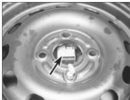
7.3b Fuel pump inertia cut-off switch location (arrowed) under spare wheel
