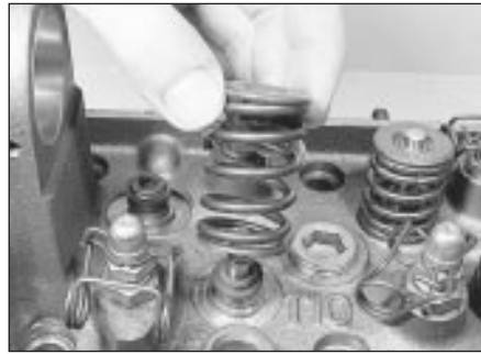
22.2b Removing a valve spring and cap
