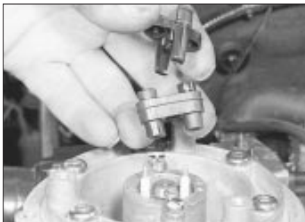
16.4 Disconnecting the fuel injector wiring plug
