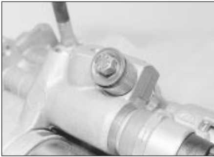
18.5 Hydraulic unit pump mounting bolt - ABS
