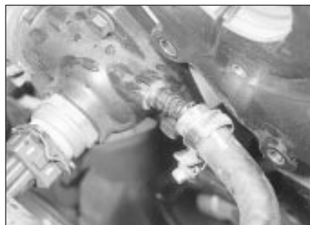
7.20a Disconnect the coolant hoses . . .
