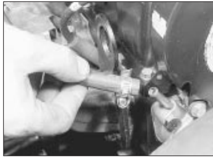
7.4b Disconnect the expansion tank hose from the thermostat housing
