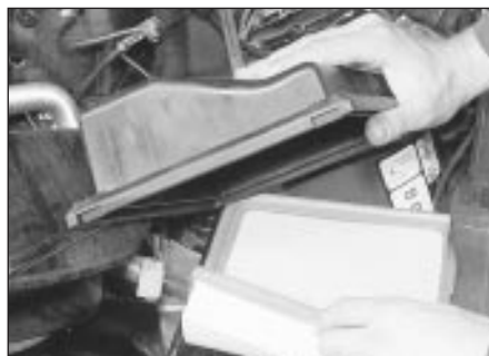
38.19 Lifting out the air cleaner element
