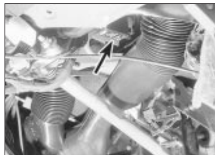
6.3 Direction indicator/hazard warning flasher relay location (arrowed)
