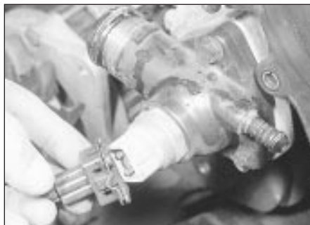
7.21 Disconnect the cooling fan switch wiring plug
