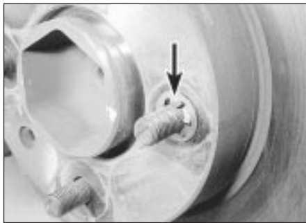
5.5a Brake drum retaining spire washer (arrowed)
