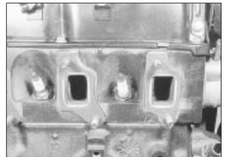
26.6d SOHC models have separate manifold gaskets for each exhaust port
