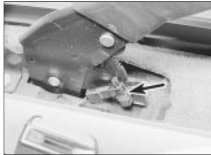
14.3 Handbrake "on" warning lamp switch location (arrowed)
