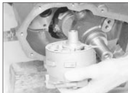
26.3b Withdrawing the oil pump
