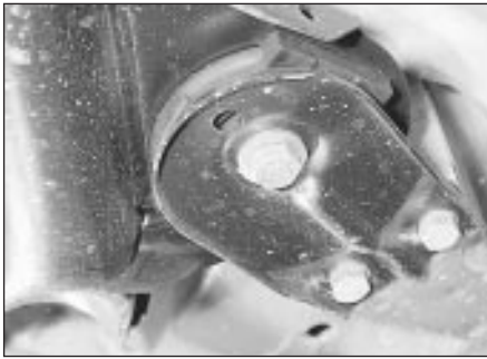
11.10 Rear suspension front guide plate
