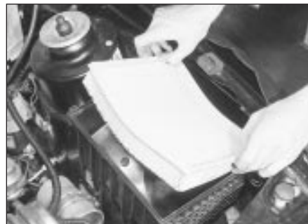
38.9 Unclip the lid and remove the air cleaner element
