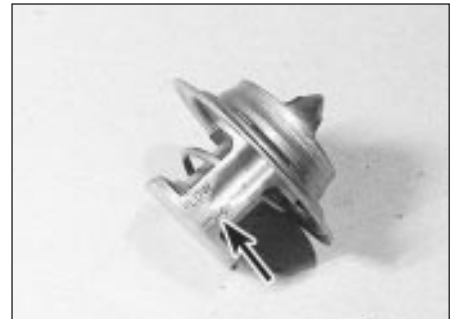
7.9 Thermostat flow direction markings (arrowed)
