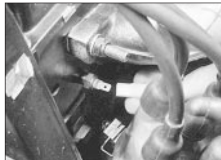
16.3a Disconnect the temperature gauge sender wiring - SOHC
