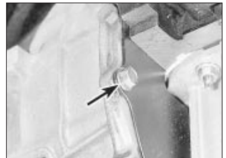
5.33 Engine adapter plate bolt (arrowed)
