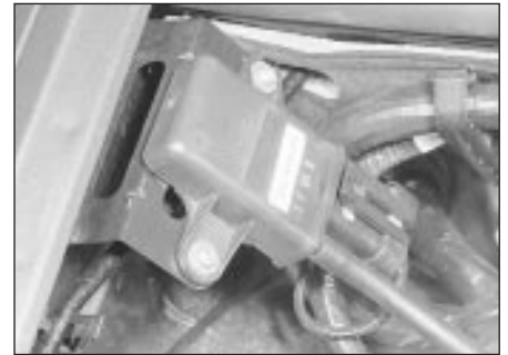
21.35 Manifold absolute pressure (MAP) sensor location
