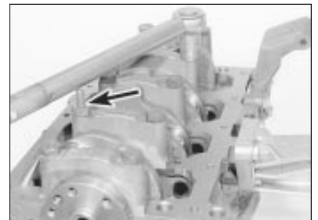
32.22b Tightening a main bearing cap bolt. Note stud bolt location (arrowed) on No 4 bearing cap - 1.8 litre (R2A)
