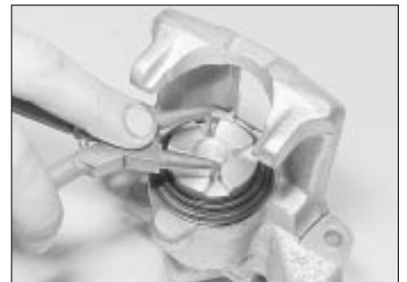
4.32 Retracting the piston using circlip pliers
