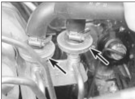
22.2 Pulse-air delivery check valves (arrowed)
