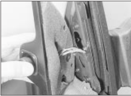
17.12b . . . and withdraw the mirror control panel
