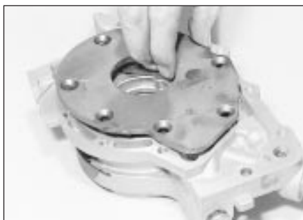
29.2 Remove the oil pump cover
