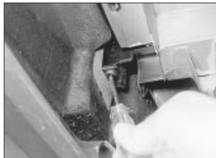
30.18 Adjusting the height of a rear bumper
