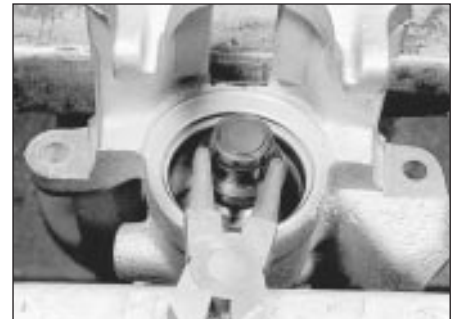
7.13 Using the piston adjuster nut to compress the adjuster spring
