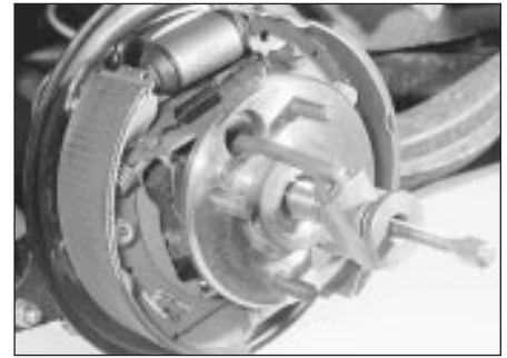
14.6 Pull the drive flange from the end of the driveshaft
