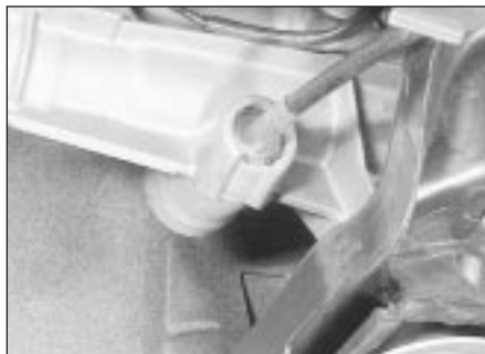
30.5 Speedometer cable end fitting in manual gearbox extension housing
