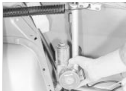
53.5 Removing an electric aerial - Saloon model
