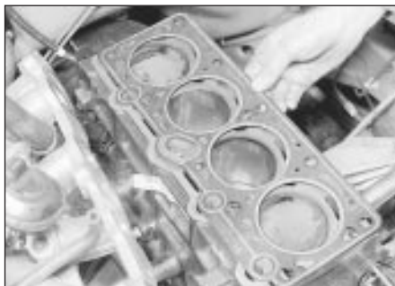
20.7 Recover the cylinder head gasket - 1.8 litre (R2A)
