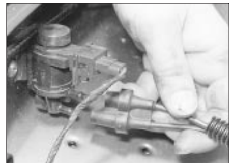
22.3 Disconnect the vacuum pipe connector from the solenoid
