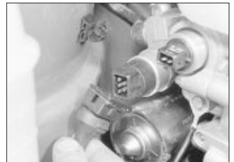
16.3c . . . and the pressure switch multi-plug - ABS
