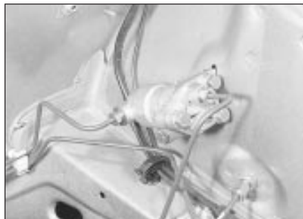
23.1a Early type deceleration sensitive valve
