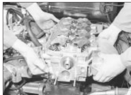
20.6 Withdraw the cylinder head bolts and lift the cylinder head from the block - 1.8 litre (R2A)
