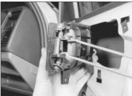
18.3b . . . and slide the handle assembly from the door aperture
