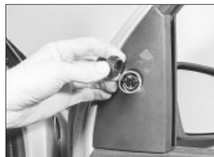
29.1 Unscrew the bezel from the adjuster knob . . .
