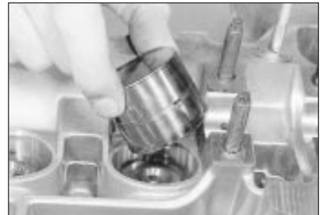
18.15 Withdrawing a cam follower
