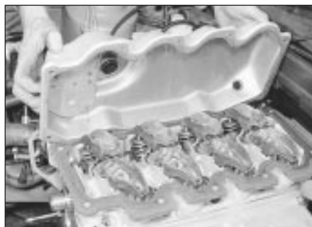
20.4 Remove the camshaft cover and gasket - 1.8 litre (R2A)
