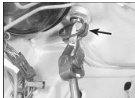
24.7 Intermediate shaft-to-inner column universal joint and clamp plate (arrowed)
