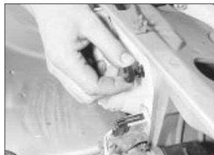
42.5 Adjusting the headlamp alignment
