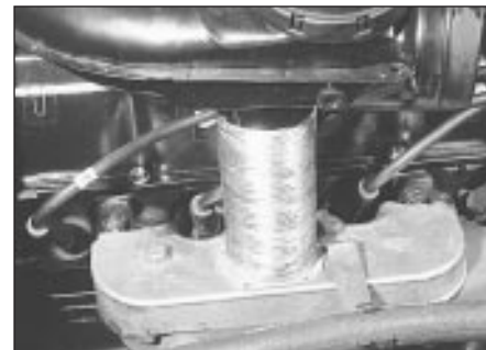
3.4 Hot air intake hose on hot air shroud
