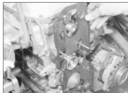
18.13 Removing the timing belt backplate - 1.8 litre (R2A)
