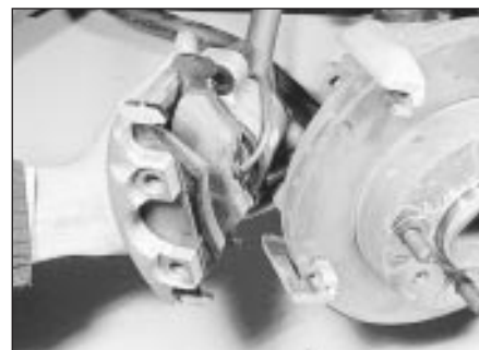
4.18 Withdrawing a caliper from its carrier bracket - Teves caliper
