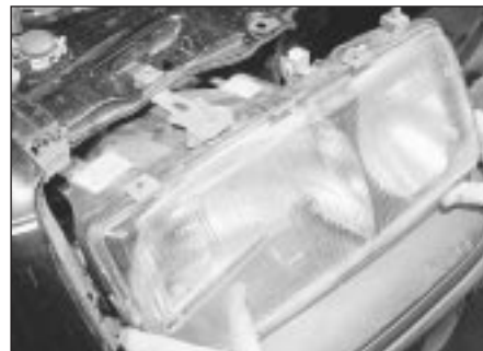
41.4d ... then withdraw the headlamp unit - models up to 1987
