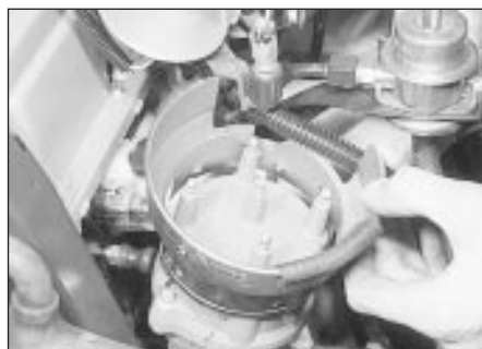
13.2 Unclipping the distributor screening can - Motorcraft distributor
