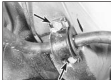
7.2a Bend back the locktabs (arrowed) . . .
