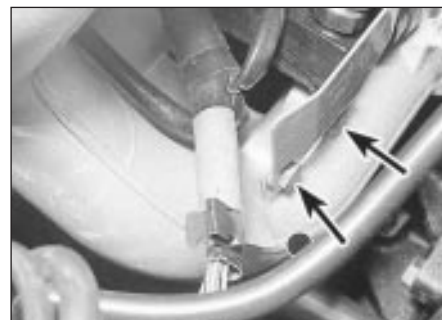
18.9b . . . and rear securing bolts
