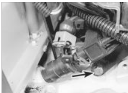
18.9a Fuel rail front securing bolt (arrowed) . . .
