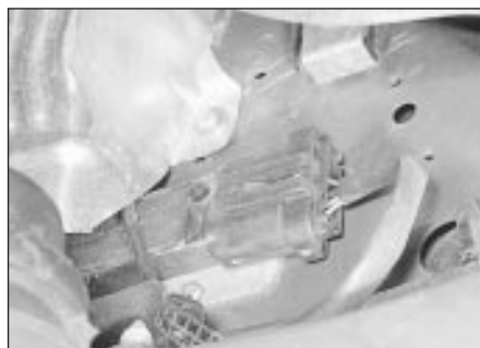
18.25 Ignition module location (arrowed)
