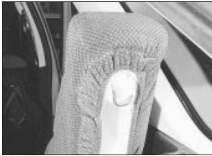
47.24 Rear seat side cushion removed exposing upper fixing hook
