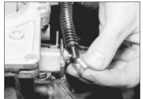
14.7 Disconnecting the throttle cable from the throttle lever - Ford VV carburettor
