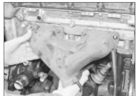
26.8c Fitting the exhaust manifold - DOHC models
