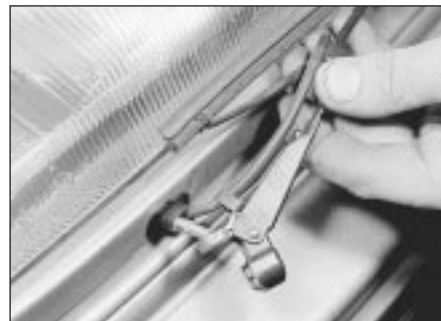
32.4 Removing a headlamp wiper arm
