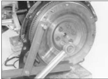
24.2 Using an improvised tool to hold the flywheel stationary while tightening the securing bolts - 1.8 litre (R2A)
