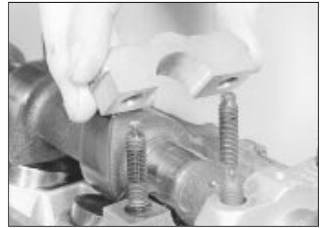
18.14a Lifting off a camshaft bearing cap
