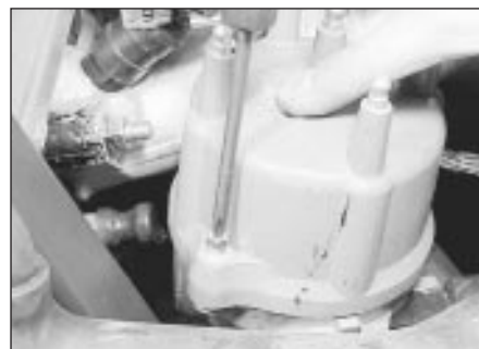
13.10 Removing a distributor cap securing screw - Motorcraft distributor
