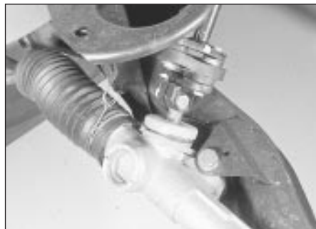
26.3 Intermediate shaft-to-steering gear flexible coupling
