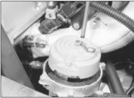
13.11 Removing a rotor arm (disc) securing screw - Motorcraft distributor
