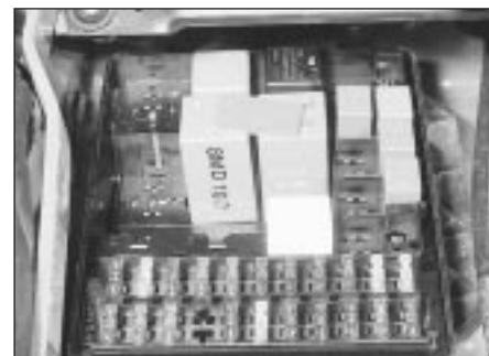
3.3b Fusebox cover removed to expose fuses and relays (1.8 CVH model shown)
