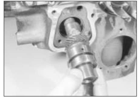
25.5b Withdraw the auxiliary shaft
