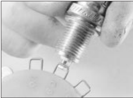
11.9b Measuring a spark plug gap using a wire gauge
