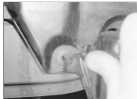
36.2 Releasing a wheel arch liner plastic clip
