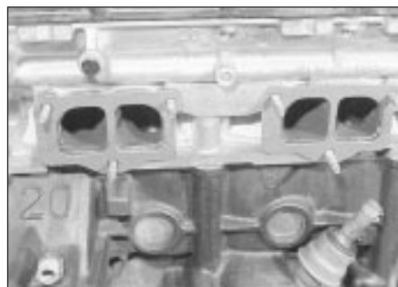
26.8a Exhaust manifold gaskets in position on cylinder head - DOHC models
