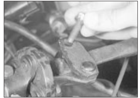
5.29 Removing the lower steering column clamp bolt
