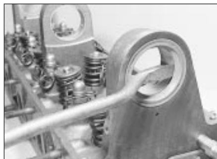
24.9 Prising out the camshaft oil seal
