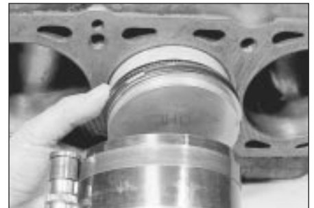
32.10 Fitting a piston ring compressor
