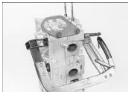
21.2a Compress the valve spring . . .
