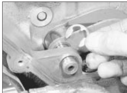
18.9a Removing the chain tensioner arm pivot pin circlip
