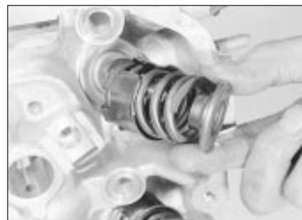
21.2c . . . then remove the cap and spring - 1.8 litre (R2A)
