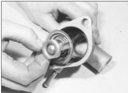
7.6b... and extract the thermostat...
