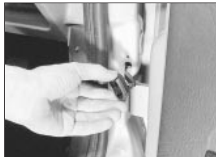
12.3 Withdrawing a courtesy lamp switch
