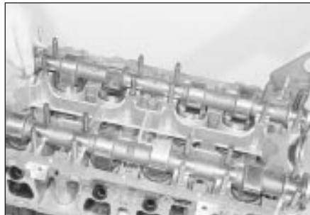
18.14b Lifting out the exhaust camshaft
