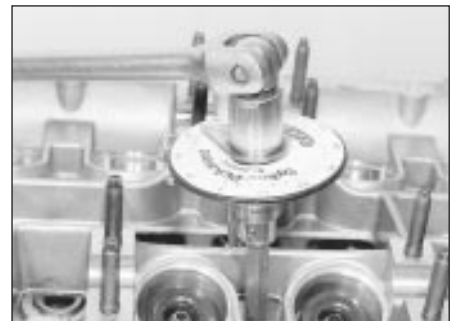
18.25b Tightening a cylinder head bolt using an angle gauge
