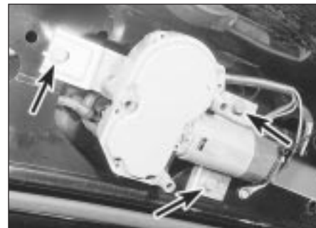
37.5 Rear window wiper motor location - mounting bracket securing bolts arrowed
