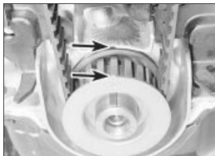
18.6a TDC lug on crankshaft sprocket aligned with notch in oil pump flange - 1.8 litre (R2A)
