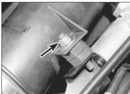
38.17 Air intake tube securing nut (arrowed)
