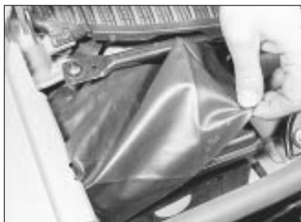
3.3a Remove the loose cover for access to the fusebox cover
