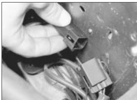
19.31 Disconnecting the exhaust gas oxygen sensor wiring connector - 1.6/1.8 litre (R6A)
