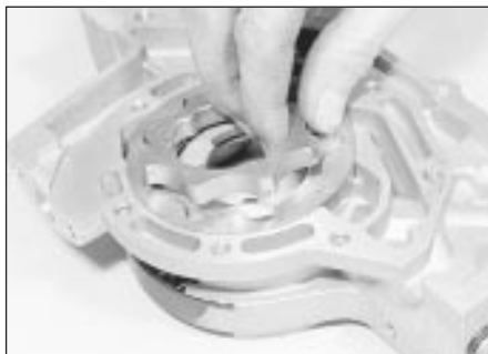
29.3 Lifting out the oil pump inner rotor
