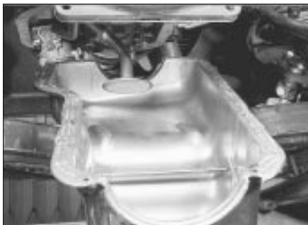
29.12 Unscrew the securing bolts and withdraw the sump
