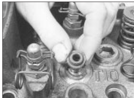
22.4 Removing a valve stem oil seal
