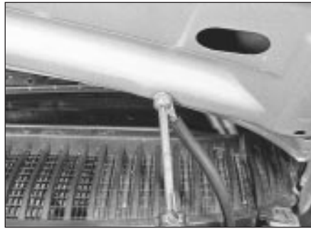
6.2 Remove the screw and disconnect the bonnet earth cable
