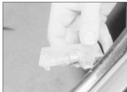
25.2b Removing a luggage compartment lamp
