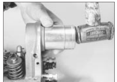
24.13 Fitting a new camshaft oil seal using a socket
