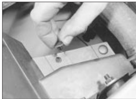
12.2a Remove the retaining clips followed by the screws . . .
