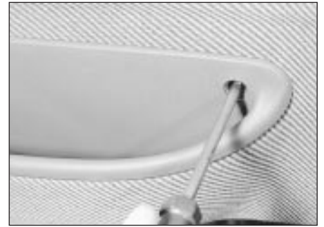
17.15b Trim panel securing screw at top edge of door pocket
