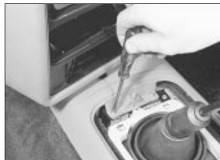
44.6a Removing a lower console panel front securing screw . . .
