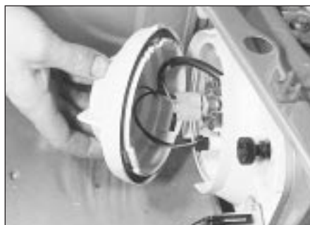
48.2 Remove the headlamp rear cover
