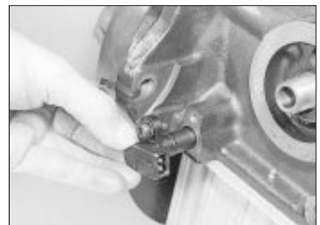
19.37 Removing the crankshaft speed/position sensor (engine removed)
