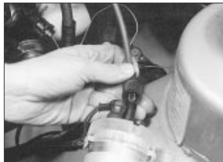
12.7 Disconnecting the HT lead from the coil
