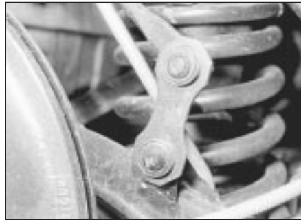
17.2 Anti-roll bar-to-lower arm connecting strap
