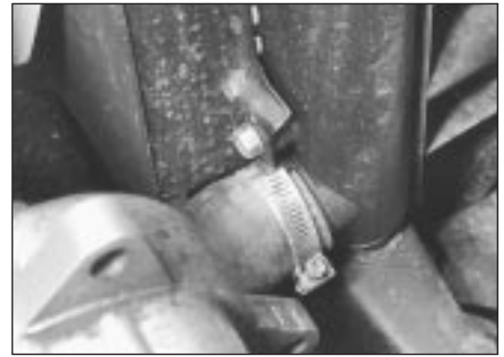
2.4b Radiator bottom hose connection - 1.8 litre
