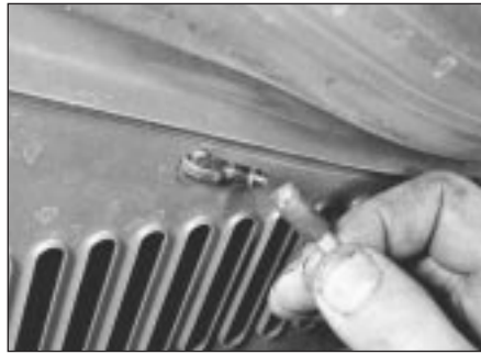
6.3 Disconnecting windscreen washer tubes from bonnet
