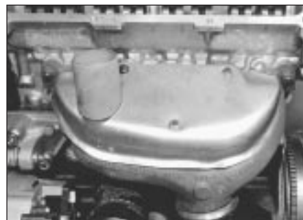
19.9 Warm air deflector plate - 1.3 litre
