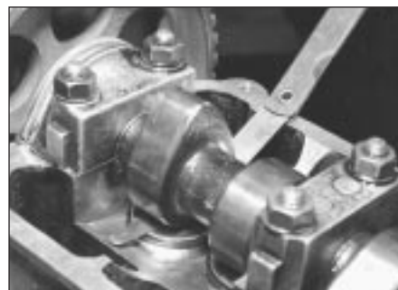
12.8 Checking a valve clearance - 1.6 and 1.8 litre
