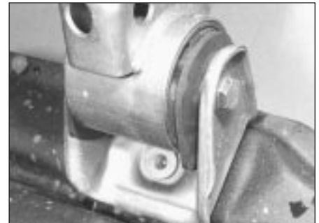
5.26a Undo front mounting through-bolt
