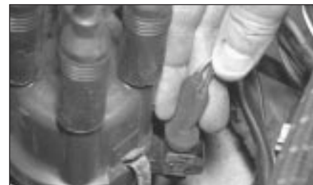
C Check that the LT lead connections are clean and secure.
