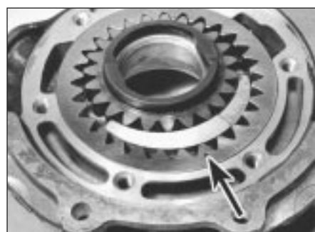
24.3b Outer rotor indentation (arrowed) must face cover
