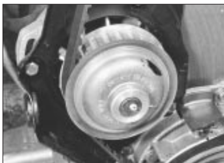
6.5 Disengage timing belt from coolant pump sprocket
