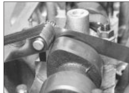
8.6 Measuring camshaft endfloat
