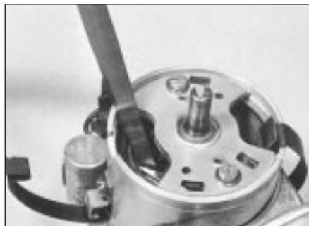
16.10a Checking contact breaker points gap
