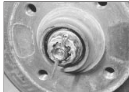
4.14 ... remove the split pin and lock ring ...
