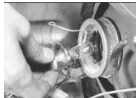
4.4 . . . and withdraw headlamp bulb
