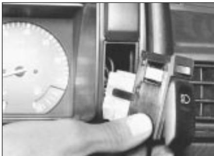
13.2 Facia switch removal
