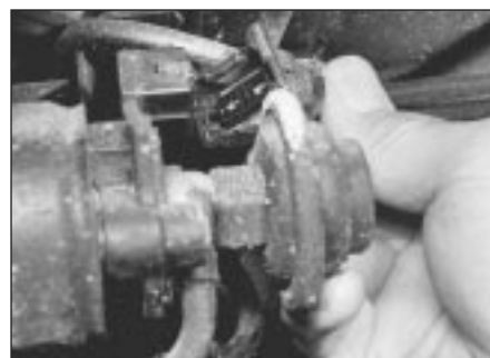
19.4 Disconnecting wiring connector from fuel pump
