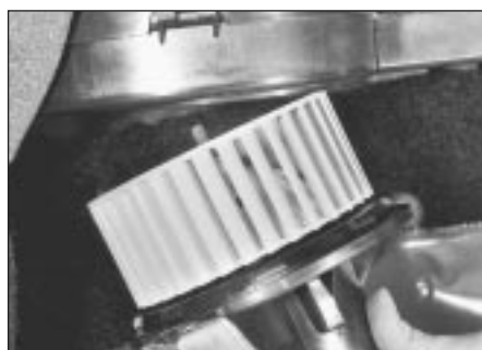
9.4 Blower unit withdrawal from housing
