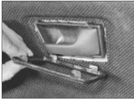
14.2 Removing door inner handle surround
