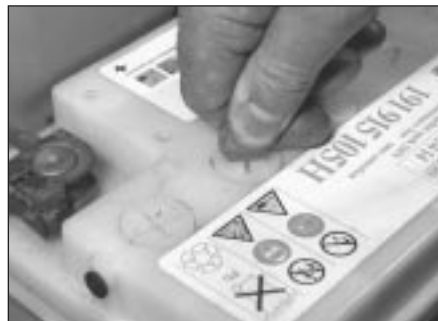
7.3a Remove battery filler caps . . .
