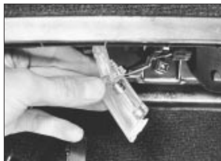
8.16 Luggage compartment lamp lens removal
