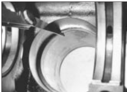
23.6 Checking piston ring gaps
