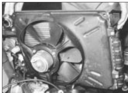
3.8 Lifting out radiator and cooling fan assembly
