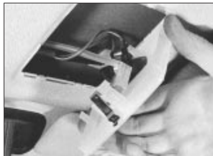
8.13a Interior light removal – 1.3 litre
