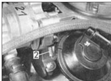
16.10 Fast idle speed adjustment screw (2)
