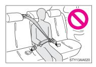
Do not use the rear center seat belt with either buckle released. Fastening only one of the buckles may result in death or serious injury in case of sudden braking or a collision.
