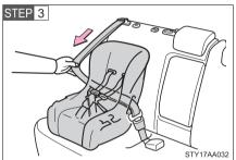
Fully extend the shoulder belt and then allow it to retract slightly into the ALR lock mode.
