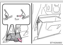
Pull up the box and disengage the claws. Remove the stoppers from the cutouts and remove the box.
