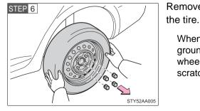
When resting the tire on the ground, place the tire so that the wheel design faces up to avoid scratching the wheel surface.
