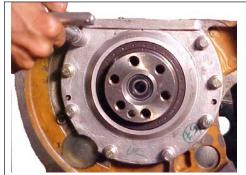
Remove the rear end oil seal with the retainer.
