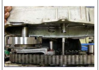
Assembly - Assembly Cover Install the return spring over rail shaft
