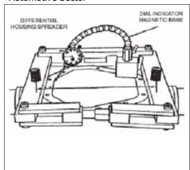
Using special tool expand the differential.
