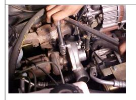
Remove the oil feed pipe and the oil return pipe.
