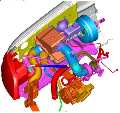
After filtration the air goes to the turbocharger.
