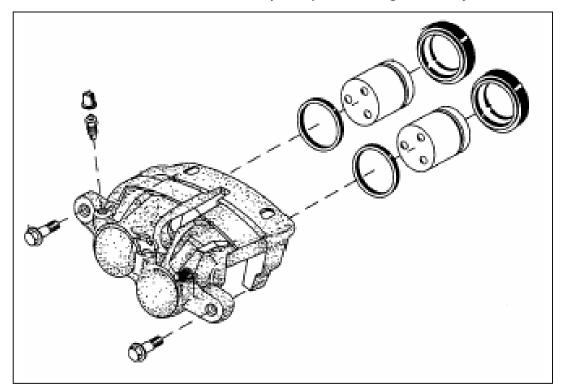
1. Loosen and remove the mounting bolts of the caliper.
