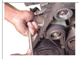
Loosen the tensioner bolt first. Loosen the belt tension with the bolt on bracket.
