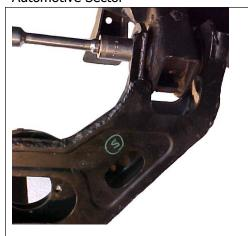
Loosen the lower arm mounting bolts ,and the upper arm side nuts. so that the lower arm movement is free
