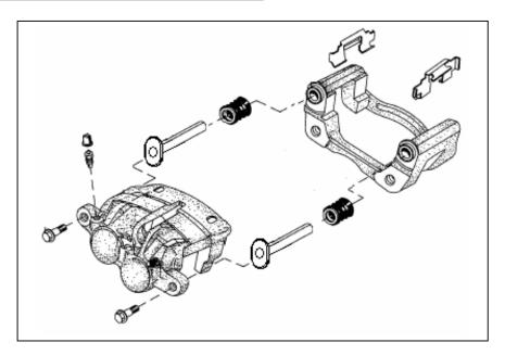
1. Separate the sliding pins from the carrier assembly .
