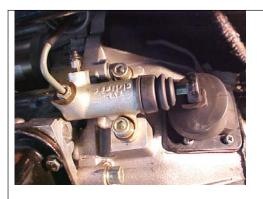
Clean the external areas of the clutch slave cylinder and remove the dust cap of the bleeder screw.
