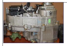
Disassembly - Assembly Cover ( Motor, Speed sensor, Clutch coil and Speedo Gear.
