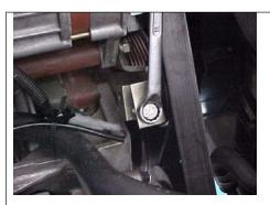
Loosen the belt tension-loosen the tensioner bolt.
