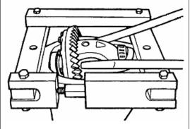
Pry differential case from carrier with pry bars. After differential case has been removed; remove the spreader.
