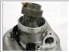
Install the Speedo gear over output shaft spline in the cover assembly
