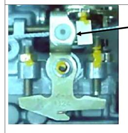
Set or ensure the gap between clamp and LFG screw, lock it at that position.
