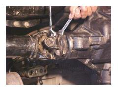
Remove the propeller shaft from the companion flange
