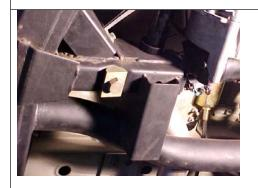
Put the height control arm assembly on chassis bracket.
