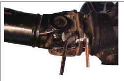
Remove the mounting bolts at the pinion end
