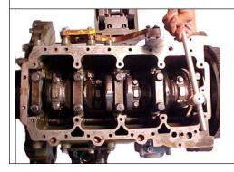
Remove the connecting rod caps and take out the pistons.
