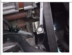
Adjust the tension by tightening the tensioner bolt.
