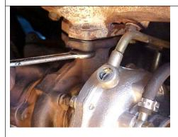
Remove the turbocharger mounting 3 nuts.
