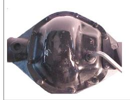
After draining the oil - remove the differential cover set screws.
