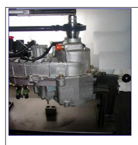
Remove the Rear Output flange.
