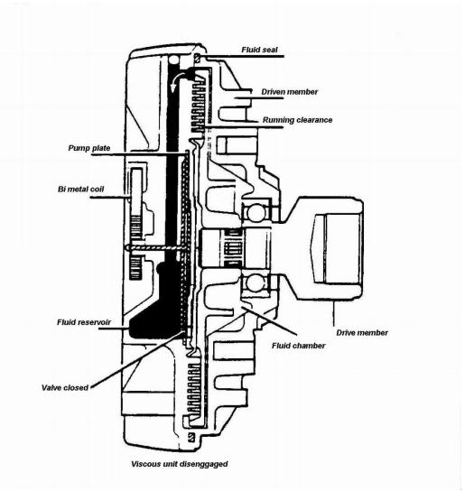
There are two main components of the viscous fan drive: input (drive member), which consist of a threaded shaft passing through a bearing into the clutch plate and secured to the water pump. The output (driven) member comprises of the main body to which the fan is attached, with the temperature sensing mechanism (bi- metal coil) and pump plates.
