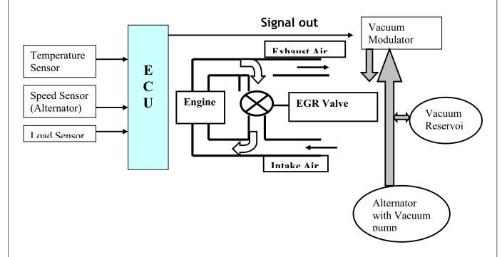
During acceleration and in higher loads the engine generates high combustion temperatures. The high combustion temperatures increase the NOx generation. The higher percentage of NOx generated in the combustion chamber come out through the tail pipe in the atmosphere.
