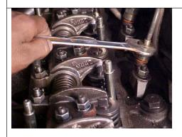
Remove the injector pipes.
