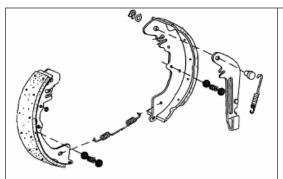
Place one shoe on backplate & assemble pin shoe hold down cup. Fit one end of the shoe return spring - lower (abutment spring) in the slot provided on brake shoe.
