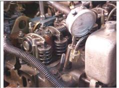
(To confirm the first cylinder TDC position remove the 1<sup>st</sup> cylinder injector, insert the MST and the dial gauge. Check by the dial if the piston is in TDC)
