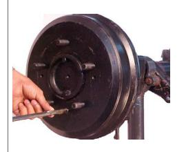
Remove the brake drum after loosening the two screws
