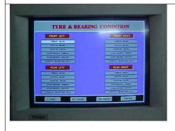
State the tyre and the bearing condition. The condition can be selected by moving the up or down arrow keys. For selecting particular condition press enter. For going to the next tyre condition press "tab" key. When the conditions are selected press "F5" key
