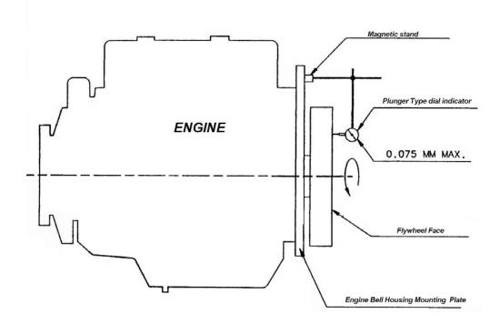
To measure the runout mount the base of the magnetic dial gauge on the block. Locate the dial gauge's needle on the outer surface of the flywheel.
