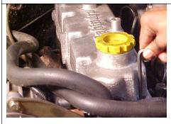
Remove the tappet cover mounting Allen screws along with the rubber washer
