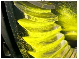
vehicle before taking decision to open/ overhaul. It is recommended that after draining the oil and opening the rear cover. Put paint marks in four different places. Then vehicle forward push the and backwards at least 15 feet. This will give a much better tooth contact under load. should be (lt remembered that
