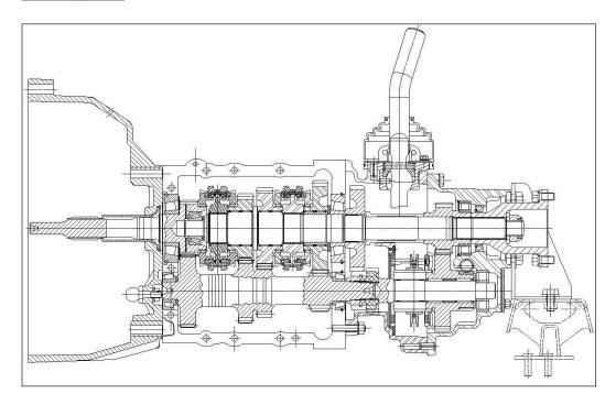
It is a 5-speed gearbox. All the forward speed is using baulk ring type synchronizer. The reverse gear is sliding mesh type with synchro brake.
