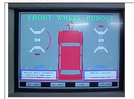
Move the tyre in the direction as shown on the screen by holding the sensor, after completing half rotation press the run out key on the sensor complete the remaining rotation.
