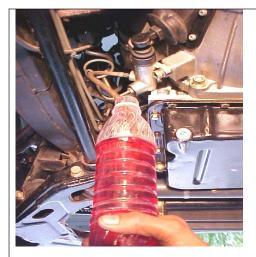
Connect bleeding tube, to bleeding screw on slave cylinder.
