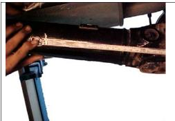
Mark & number the shaft 6 inches from pinion end at four positions 90° apart.
