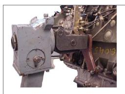
After removing the engine from the vehicle mount it on the engine stand.
