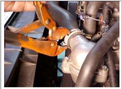
Remove hoses connecting the water pump to radiator.
