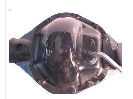
After draining the oil - remove the differential cover set screws.
