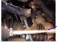
Slacken the track rod end lock nut.
