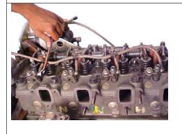
Remove the leak off pipe.
