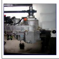
• Holding the flange with the help of flange holder, tighten the nut.
