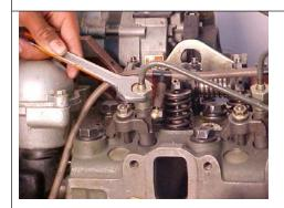
Remove the High-pressure pipes.
