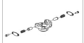
A) Springs towards  $1^{st}$  /  $2^{nd}$  gear position is softer than  $5^{th}$  / reverse position.
