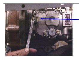
To lock the FIP Loosen the timing lock bolt. Move the lock plate away & then tighten the Timing lock bolt so that it locks the camshaft.
