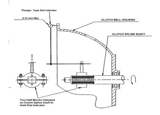
bell housing runout will also need to be checked.
