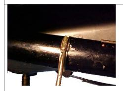
Install a screw clamp at position "1"
