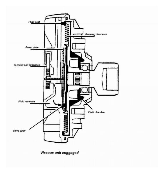
There are two sets of annular grooves. , One in the drive clutch and the other in the drive body, a specific clearance being provided between two sets of grooves. When this clearance is filled with viscous fluid a shearing
