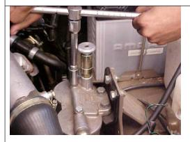
Loosen the filter mounting bolt.
