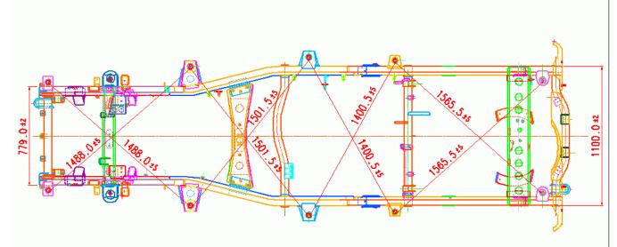
INSPECTION SKETCH FOR CHASSIS WITH BODY OUTRIGGERS
