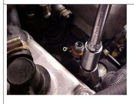
Remove the injector clamps.
