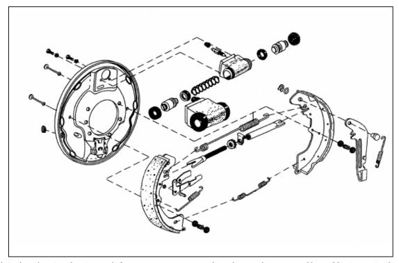
This brake is designed for use on rear wheels and is equally efficient in both forward and reverse direction of movement. A mechanical lever mechanism is incorporated for normal hand brake operation. The feature of this brake is that the brake shoe adjustment takes place automatically when the service brake is applied.
