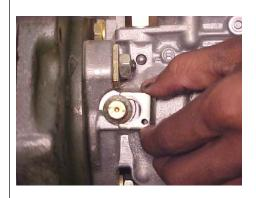
Loosen the timing lock bolt (FBB). Remove the triangular plate and then tighten so that the FIP's camshaft is locked.
