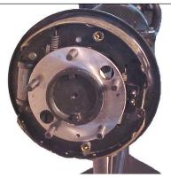
Remove the parking brake locking
