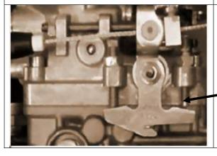
If rpm is out of specification adjust the fast idle screw to get required rpm.
