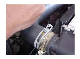
Remove the inlet and outlet hose for the intercooler.
