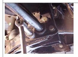
Tighten the Torque Arms 3 bolts (2 bolts onto the weld nuts and 1 free bolt +flanged nut)
