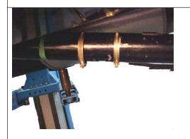
Increase the distance between the clamps until the vibration is at the lowest level.
