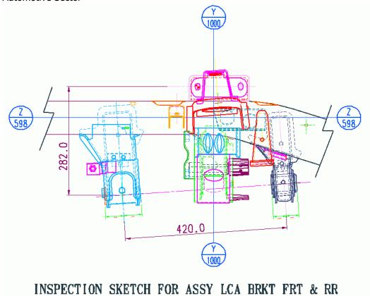
The dimension for the LCA bracket front & rear is the same.
