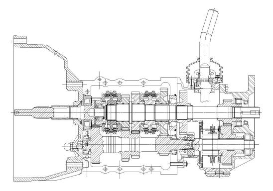
It is a 5-speed gearbox. All the forward speed is using baulk ring type synchronizer. The reverse gear is sliding mesh type with synchro brake.
