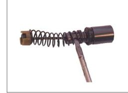
Using a screwdriver, lift the leaf retainer. spring Remove spring assembly from plunger.
