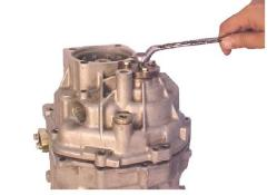
While tightening the centre bolt of the special tool; tighten it gently.
