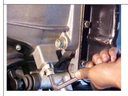
Remove the slave cylinder from the mounting bracket.
