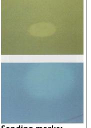
Sanding marks: scratches visible through the paint film.
