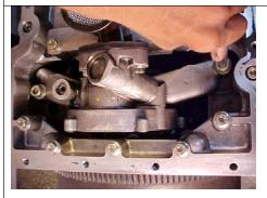
Remove the oil pump along with the suction.
