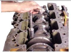
Remove the main bearing bolts.
