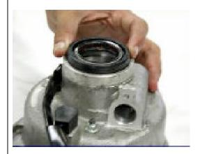
Press the new oil seal into the cover assembly.
