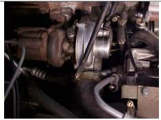
Remove the hose connection from the Turbocharger end TC to intercooler.
