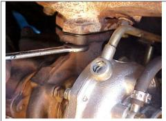
Remove the exhaust pipe from after the elbow. (Access is only after lifting it on a two post or in a pit and using a extension with UJ.)
