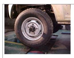
Slacken the wheel nuts. Raise the wheel and remove the front wheels.
