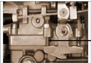
Set the idling to 845 - 850 rpm approx. by adjusting idling screw.
