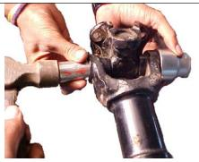
Applying the socket wrench on the outside of the propeller shaft flange, force out one end of UJ using a vise as shown. (One end 32 mm socket to receive other end 21-mm socket to push.)
