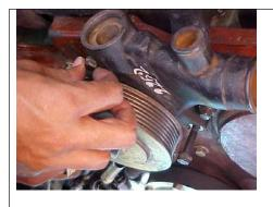
Remove the water pump assembly after removing the mounting bolts.
