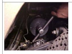
Remove the oil filter using the MST 545
