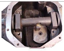
Place the setting gauge 2 - MST 582 (in the crown wheel bore)
