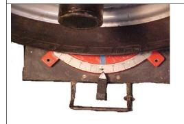
Remove the lock-pins of the turning table
