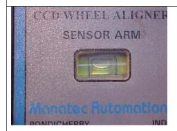
Ensure that the bubble in the spirit level of the rear sensor is set in the center of the marking made on it.
