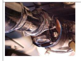
Remove the mounting bolts at the gearbox end.
