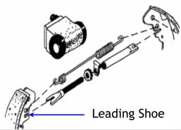
Hook the shoe return spring (short length coil) to the leading shoe with the adjuster assembly in its minimum length condition, assemble it in between the shoe webs.
