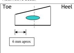
After the backlash has been achieved, check the tooth contact on both the drive and the reverse side.
