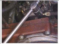
Remove the FIP connections and fuel supply.
