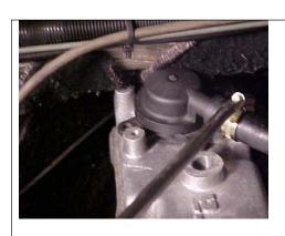
Remove the oil filler cap and the pipe from the ladder frame to the rocker cover.
