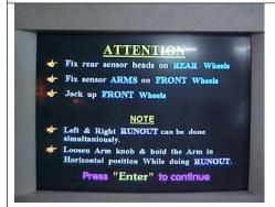
Fix the sensors on the rear as well as front wheels.
