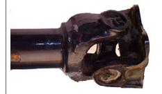
Remove the circlips holding the UJ in place.
