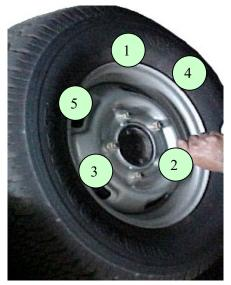
While tightening the wheel nut tighten as per the sequence shown.
