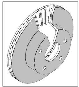
runout will cause brake pedal pulsation and rapid unven wear of the brake pads.
