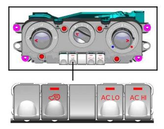
The left knob sets the flap position to direct the airflow to face only or face & feet or feet only or feet & defrosting or only defrosting.
