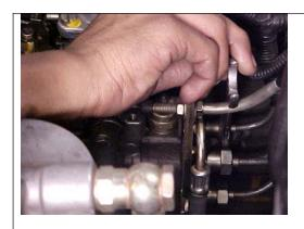
Loosen the high-pressure pipes from both the FIP end & injectors.
