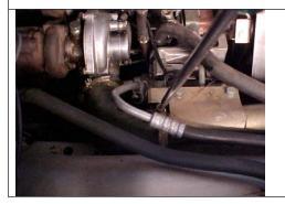
Please cover the opening to the turbocharger with cover to avoid accidentally dropping any foreign object e.g. spanner
