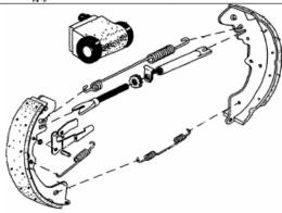
Fit the pawl lever to the spring dowel inserting one leg of the pawl between male push rod end & shoe web of the leading shoe & the other end of the pawl leg resting on the adjuster nut.
