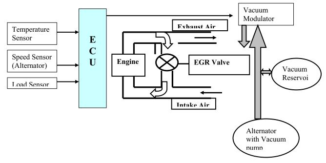
During acceleration and in higher loads the combustion chamber temperatures increase. The high combustion temperatures increase the NOx generation. The higher percentage of NOx generated in the combustion chamber come out through the tail pipe in the atmosphere.
