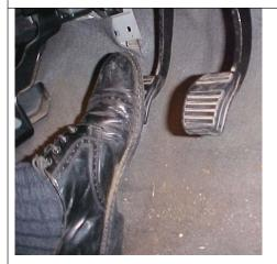
Operate clutch pedal 3 or 4 times slowly to the full stroke.
