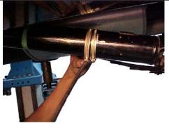
If the vibration decreases, install a second clamp and repeat the test.
