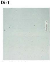
Small solid particles embedded in the paint producing a rough paint surface
