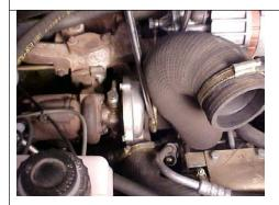
Remove the air intake hose to turbocharger.
