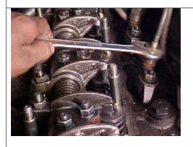
Remove the injector pipes.
