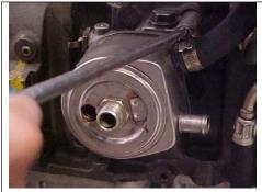
Remove the pipe oil cooler to the block.
