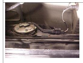
Disconnect the fuel gauges, tank unit electrical connection.
