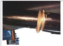
If the clamps cause an additional imbalance, separate the clamp (¼ inch above & below the mark.). Repeat the vibration test.
