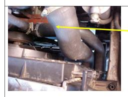
Remove the hose connected from the water pump to heater and also the heater return line.
