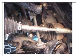
Jack the wheels, ensure that the anti roll bar link has been disconnected.
