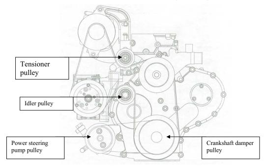
The belt must be routed correctly.
