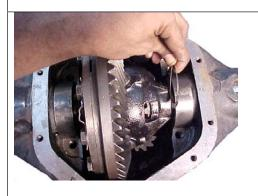
Push the crown assembly towards the pinion so that the backlash is zero.
