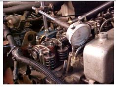
Bring the first cylinder into compression. Confirm using the MST
