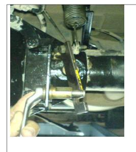
Loosen the nut & move the bolt in such away that the bolt is alligned & enters in the slot on the tool.
