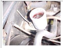
Fill the Reservoir clutch master cylinder up to the top level with recommended clutch fluid.
