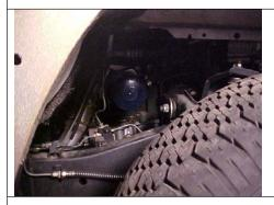
Take out the apron cover behind the wheel by carefully removing the plastic fasteners
