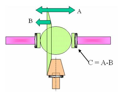
First the play of the diff cage or crown wheel with diff cage but without the pinion in place is checked. This play is A
