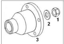
1. Unlock the output shaft nut
