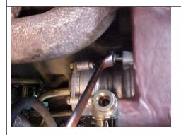
Remove the exhaust pipe at the Turbocharger outlet elbow.
