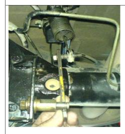
Put the projecting pin of the tool in the eye of the spring & allow the tool to hang freely..
