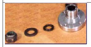
Position the flange on the upper output shaft in transfer case and install the flange, seal, washer and nut.
