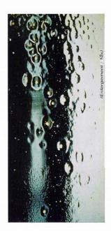
Cavities in the finish coat, possibly allowing the previous coat to show.
