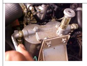
For bleeding the system, loosen the high-pressure pipe unions and use the hand primer.
