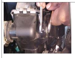
Remove the condenser mounting bolts.
