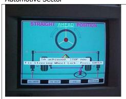
For achieving the straight ahead position move the steering wheel slowly to the directions as displayed on the screen first to the right and the to the left. Hold for some time at the end, for the computer to acquire data. Hold for some time at the centre position. Fix the steering lock at that Press "enter" position. kev continue.
