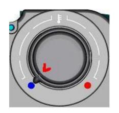
Keep the cooling & heating knob at the highest cooling point position.
