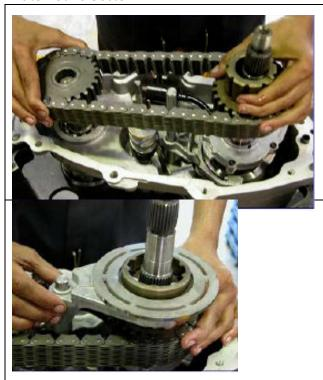
Install the spacer to the front output shaft and insert snap ring into the groove over spacer.
