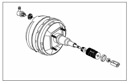
Note -- The Booster is a non- serviceable Unit & it should never be tampered with.
