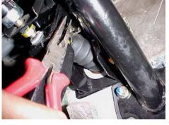
Remove the clevis pin lock & the clevis pin.
