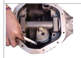
Measure the gap between the setting gauge 1 and 2 using a feeler gauge.
