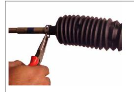
Remove the bellows along with the clips.
