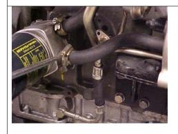
Remove the pipe from the oil cooler to the water pump.
