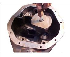
Place the setting gauge (MST 581) in the carrier (the pinions inner bearing outer race & shim should be removed) Please note that the lifting handle should be removed after placing it in position
