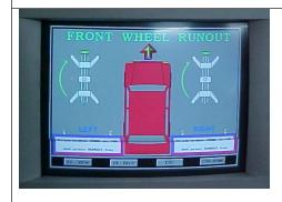
For the runout press the runout key on the sensor as shown in the figure.
