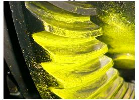
before taking decision to overhaul. It is recommended that after draining the oil and opening the rear cover. Put paint marks in four different places. Then push the vehicle forward and backwards at least 15 feet. This will give a much better tooth contact under load. (It should be remembered that
