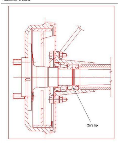
The assembly section is shown in the sketch attached. Please note the bearing direction the circlip
