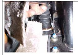
Rotate the master cylinder push rod till desired height of pedal is achieved.
