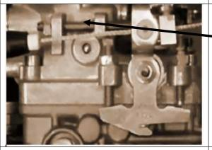
Re set the anti-stalling screw to get idling rpm of 855 - 860 approx.
