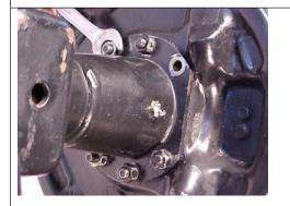
Loosen the 6 screws holding the retainer.
