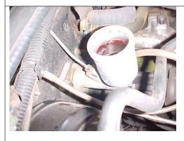
Check the fluid level in container and need be top up to the max. level.
