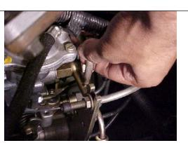
Avoid loosening only at one end as it can cause strain in the pipes, while removing the injectors
