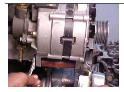
Remove the accessory like power steering pump. AC pump and the alternator.
