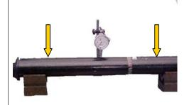
Measure the runout at the center and at the ends - away from the weld.
