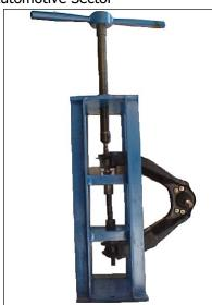
Caution: Use of any lubricant will result in degradation of the rubber bush and lower life. Pressing without soap solution will damage the bush
