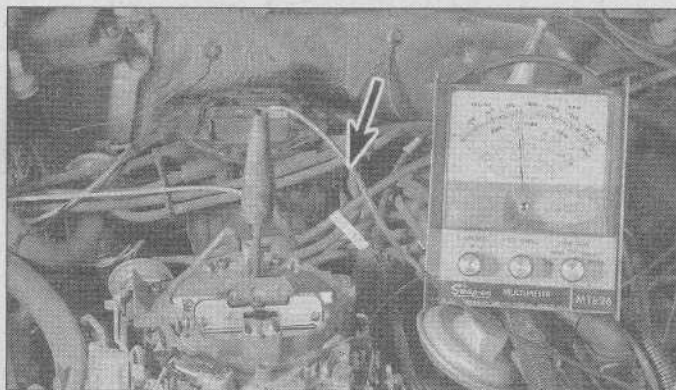
5.6 Use a jumper wire (arrow) to connect the tachometer lead to the TACH terminal on the distributor (HEI systems only)
