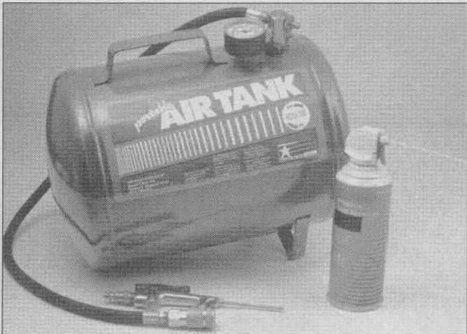
7A.13 If dips, which are water soluble, are used, it is necessary to use some type of compressed air to clean and dry off the parts after they have been rinsed off with water. You must be sure, regardless of how the parts are cleaned, that all air and fuel passages are clean and not plugged before reassembly. Compressed air is the most effective way to clear passages. If you don't have access to an air compressor, you can buy an inexpensive portable air tank, which can be filled at any service station, or buy a can of compressed gas designed for cleaning electronic parts. Warning: Always wear eye protection when using compressed air!
