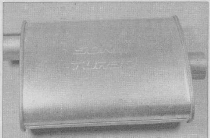
8.32 Turbo mufflers have large passages and high flow capacity
