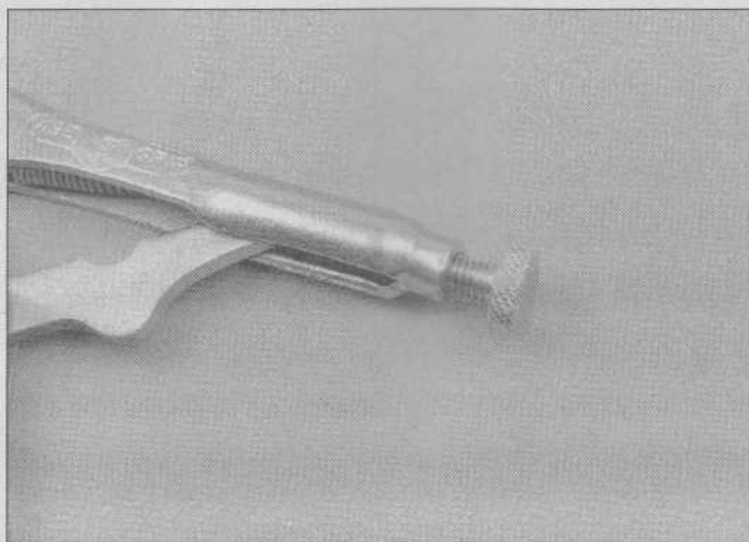
2.14 To adjust the jaws on a pair of Vise-Grips, grasp the part you want to hold with the jaws, tighten them down by turning the knurled knob on the end of one handle and snap the handles together - if you tightened the knob all the way down, you'll probably have to open it up (back it off) a little before you can close the handles
