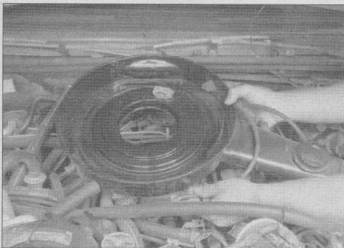
6.3a Remove the air cleaner housing . . .
