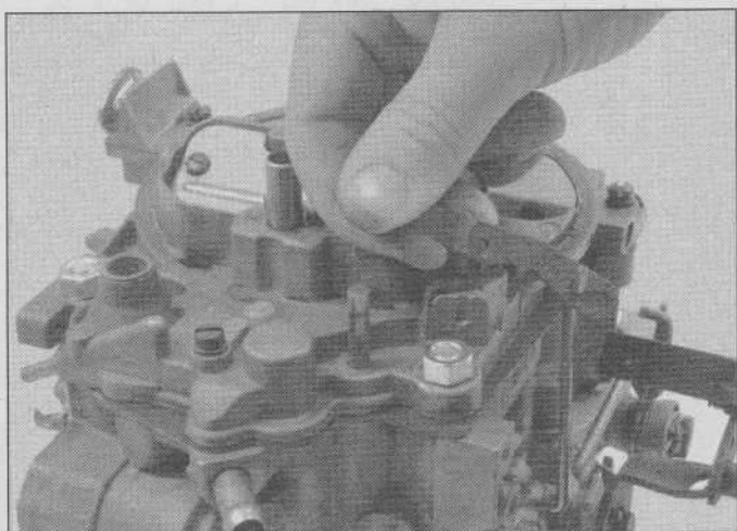
7D.16b . . . just far enough to lift the lever from the air horn and disconnect it from the rod.
