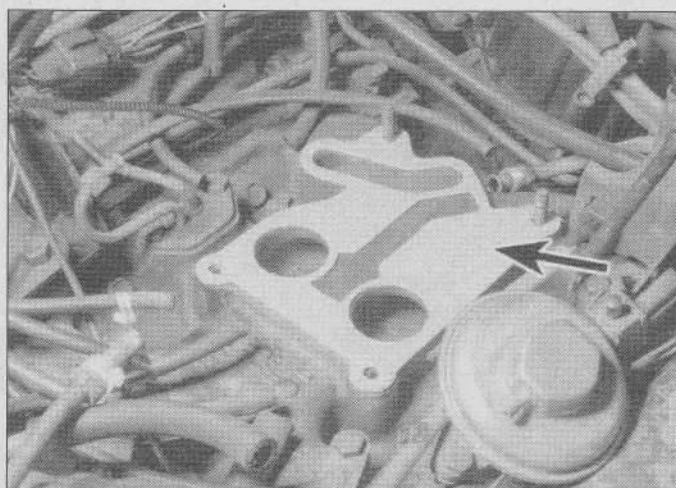
6.12 Always use a new carburetor base gasket (arrow). Old ones become crushed and hardened due to age and heat, and can't provide the kind of seal needed to prevent vacuum leaks (a very common source of driveability problems).
