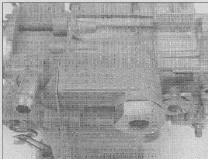
4.3 The identification numbers on a Monojet are stamped into the end of the float bowl right above the fuel inlet
