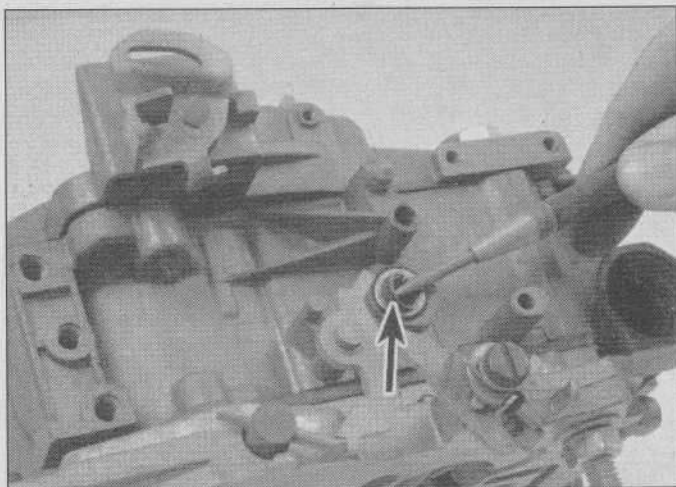
7D.15 Once the housing has been removed, carefully lift out and discard the choke shaft seal (arrow). Replace it with a new seal during reassembly.
