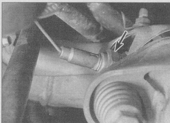
5.11 A typical oxygen sensor (arrow) mounted in the exhaust manifold
