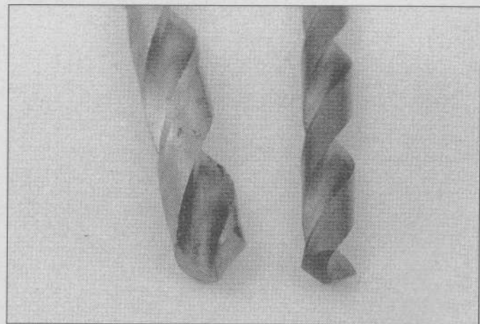
2.42 If a bit gets dull (left), discard it or re sharpen it so it looks like the bit on the right
