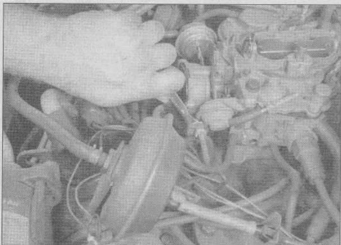
6.6 Detach the choke heater line, if equipped
