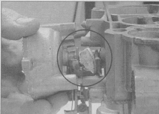
7D.14b ... then remove the choke housing assembly from the carburetor main body. Note: Carefully observe how the linkage (circled area) is assembled so you can put it back together correctly on reassembly.
