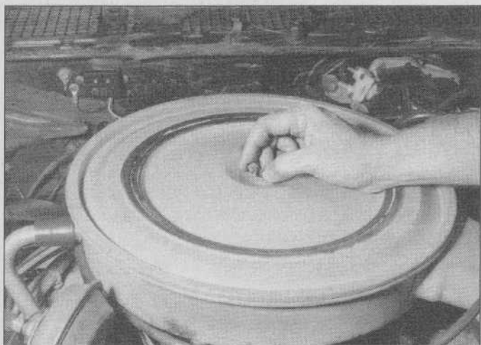
6.1 Remove the air cleaner housing cover
