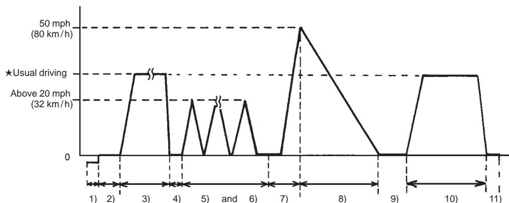
★Usual driving: Driving at 30 – 40 mph, 50 – 60 km/h including short stop according to traffic signal. (under driving condition other than high-load, high-engine speed, rapid accelerating and decelerating)
