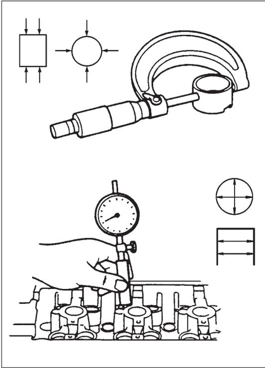
Measure cylinder head bore and tappet outside diameter to determine cylinder head-to-tappet clearance. If clearance exceeds limit, replace tappet or cylinder head.
