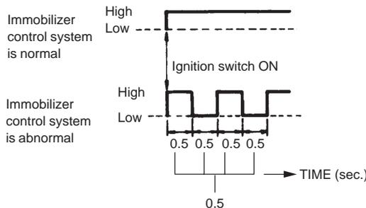
When ECM and Immobilizer Control Module detects a trouble which has occurred in the above areas, it stores DTC corresponding to the exact trouble area in ECM and Immobilizer Control Module memory.
