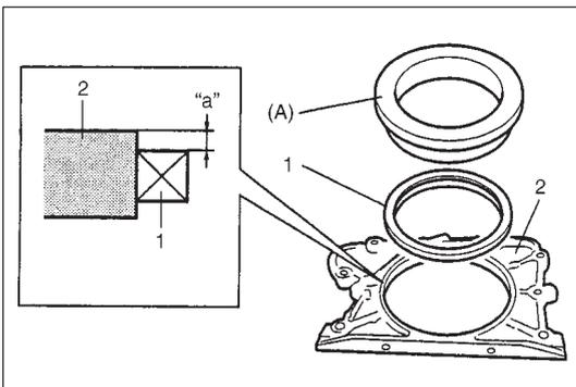
For oil seal installation, press-fit rear oil seal (1) to oil seal housing (2) by using special tool as shown in the figure.
