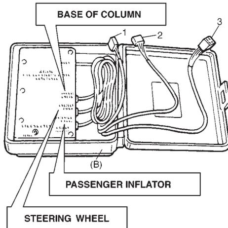
1. Connector for contact coil and driver air bag (inflator) module (Located near the base of the steering column)
