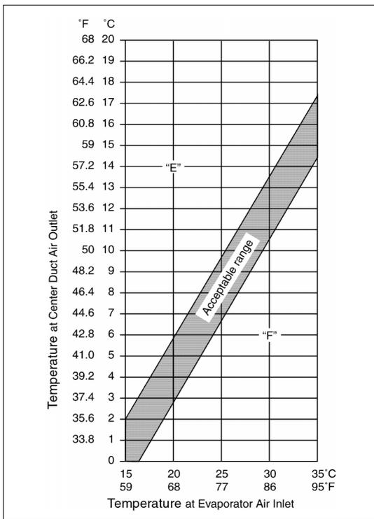
9) Check inlet port temperature-to-outlet port temperature relationship using graph.
