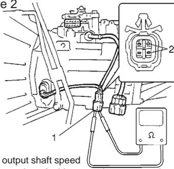
1. A/T output shaft speed sensor – input/turbine speed sensor coupler
