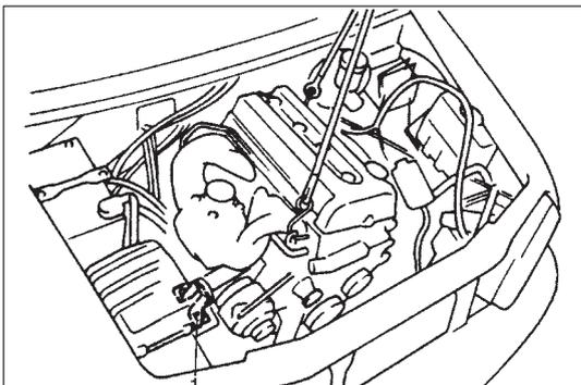
28) Install lifting device.
