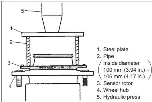
6) Install sensor rotor as shown (if equipped with ABS).
