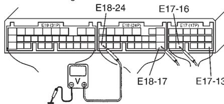
**TABLE B-7 A/C CONDENSER FAN CONTROL SYSTEM CHECK**
