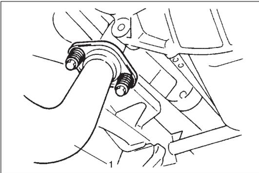
18) Disconnect exhaust pipe (1) from exhaust manifold.
