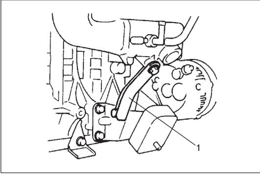
12) Remove intake manifold stiffener (1).
