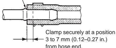
With bent pipe, fit hose as its bent part as shown or till pipe is about 20 to 30 mm (0.79-1.18 in.) into the hose.
