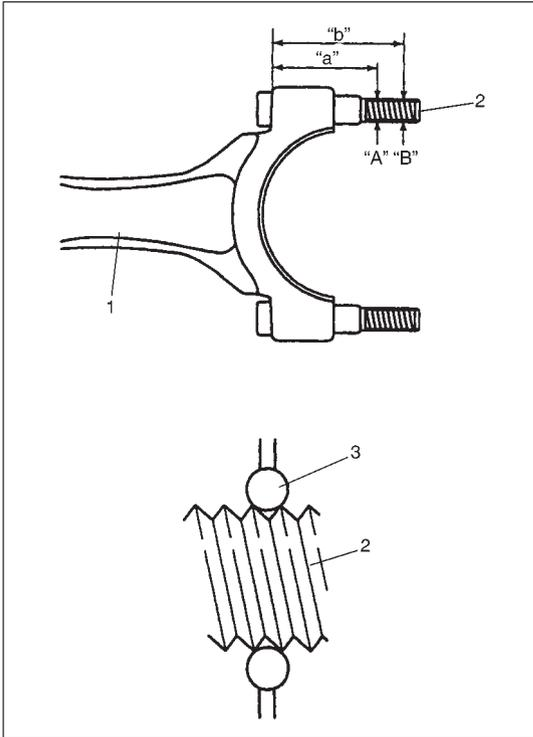
● **Connecting rod bolt diameter (Plastic deformation tightening bolt)**
