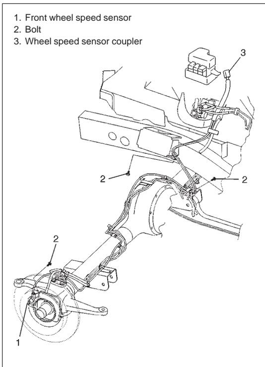
2) Disconnect front wheel speed sensor coupler.
