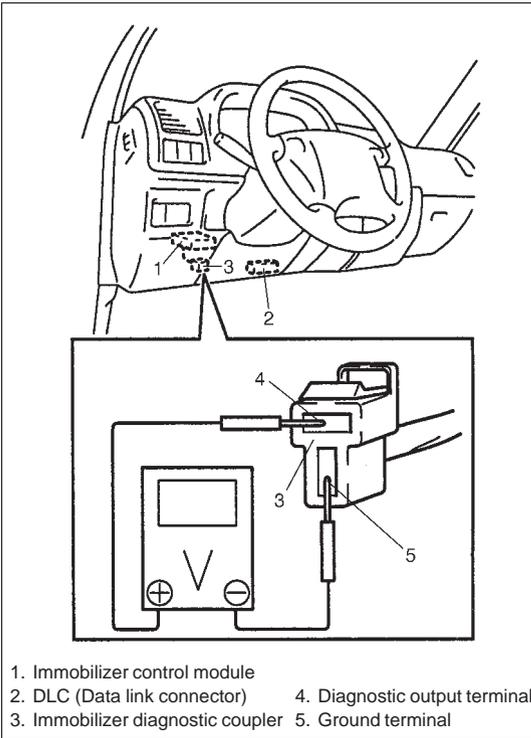
**EXAMPLE: ● COIL ANTENNA FAILURE (CODE NO. 13)**
