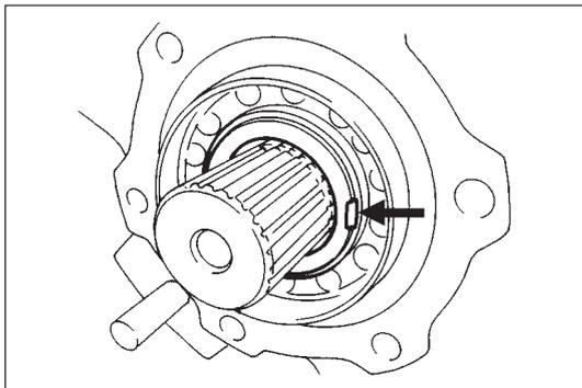
11) Caulk front wheel bearing lock nut at groove of spindle (for 4WD).
