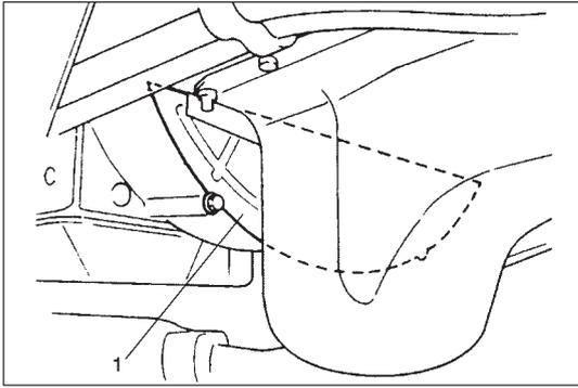
23) Remove clutch housing (torque converter housing for A/T) lower plate (1).
