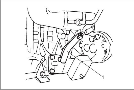
12) Remove intake manifold stiffener (1).
