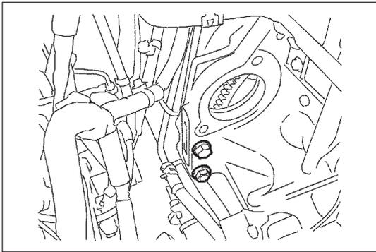
26) Remove bolts and nuts fastening cylinder block and transmission.
