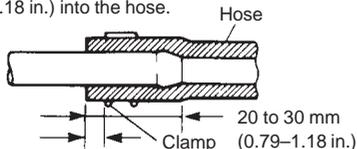
Clamp securely at a position 3 to 7 mm (0.12-0.27 in.) from hose end.
