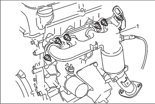
6) Remove exhaust manifold (1) and its gasket from cylinder head.
