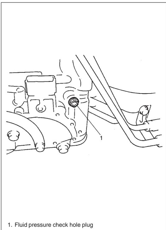
1. Fluid pressure check hole plug
