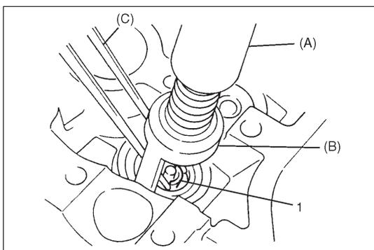
8) Using special tools (Valve lifter), compress valve spring and fit two valve cotters (1) into groove in valve stem.
