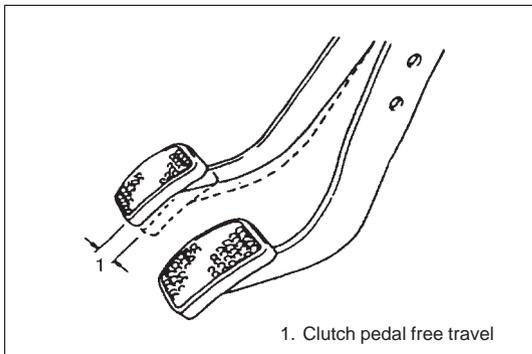
**CHASSIS AND BODY****ITEM 6-1****Clutch****Pedal inspection**
