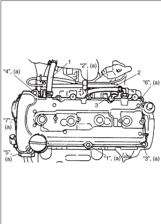
3) Install cylinder head cover to cylinder head.
