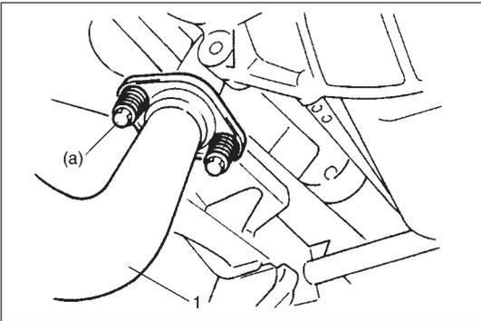
2) Install seal ring and install exhaust pipe (1) to exhaust manifold.
