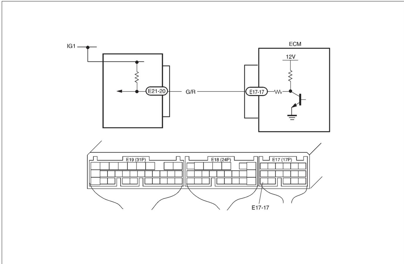
The serial data line is pulled up to about 12 V by ECM and TCM transmits information to ECM through it by controlling its grounding.
