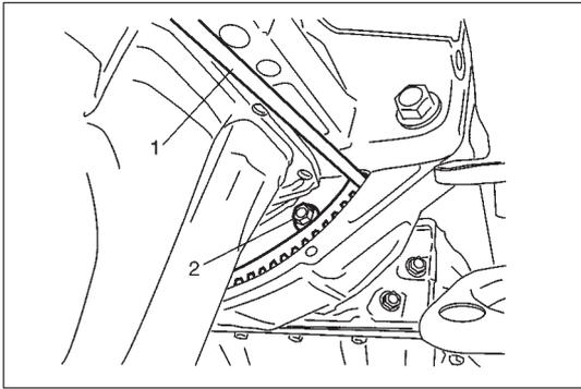
24) With drive plate locked by using a proper size rod (1) or the like, remove torque converter bolts (2) (vehicle with A/T).
