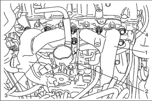
13) Remove intake manifold (1) with throttle body (2) and EGR pipe (3) from cylinder head (4), and then its gasket.
