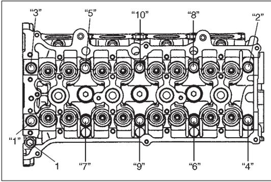
20) Loosen cylinder head bolts in such order as indicated in figure by using a 12 corner socket wrenches and remove them.
