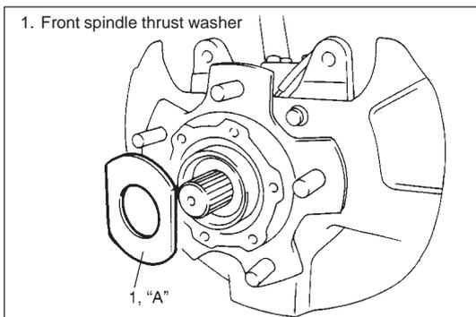
12) Apply lithium grease thinly to both surface, all around of front spindle thrust washer (for 4WD).
