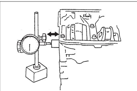
Use a dial gauge to read displacement in axial (thrust) direction of crankshaft.
