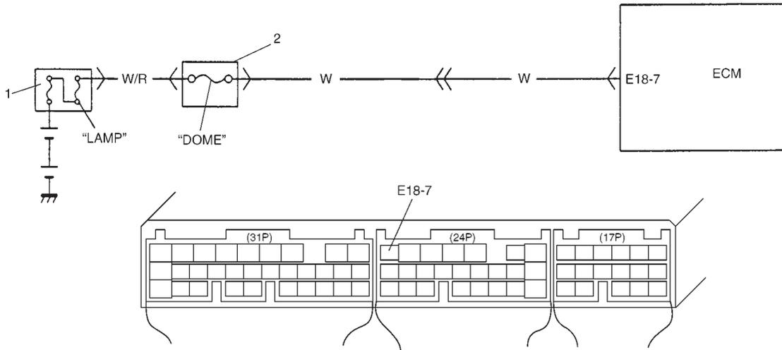
Battery voltage is supplied so that diagnostic trouble code memory, values for engine control learned by ECM, etc. are kept in ECM even when the ignition switch is turned OFF.
