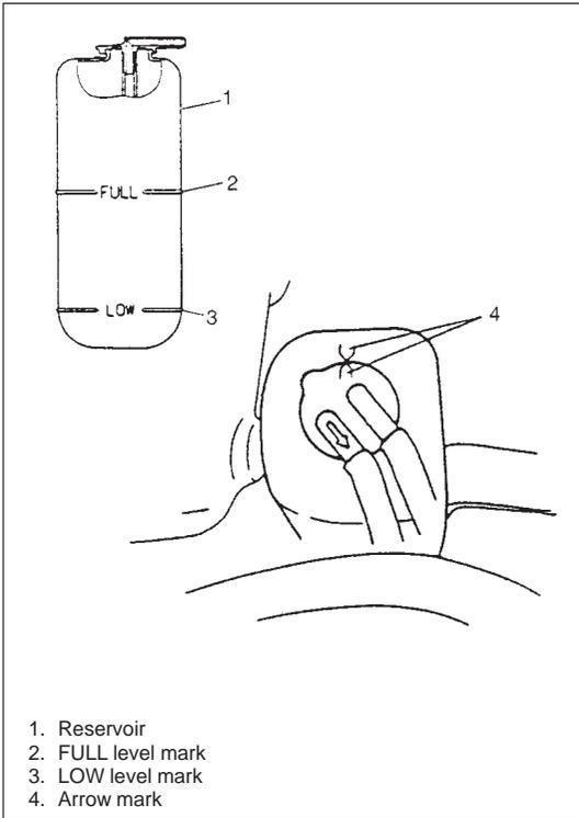
6) Add coolant to reservoir so that its level aligns with Full mark. Then, reinstall cap aligning arrow marks on reservoir and cap.
