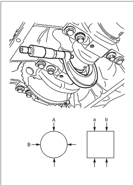
**Crank Pin and Connecting Rod Bearings**
