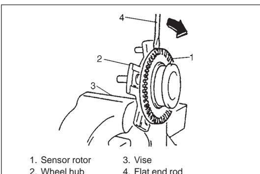
10) Remove sensor rotor from wheel hub as shown (if equipped with ABS).
