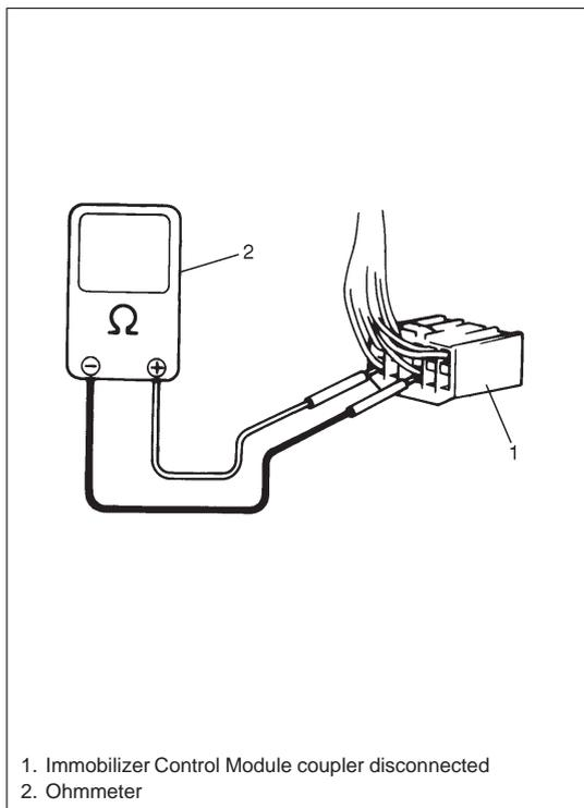
**Resistance Check (Vehicle not equipped with air bag system)**
