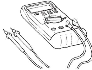
Digital multimeter for which the maximum test current is 10 mA or less at the minimum range of resistance measurement.
