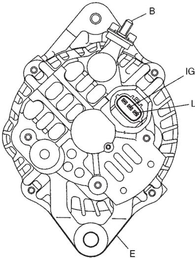
B : Generator output (Battery terminal)
