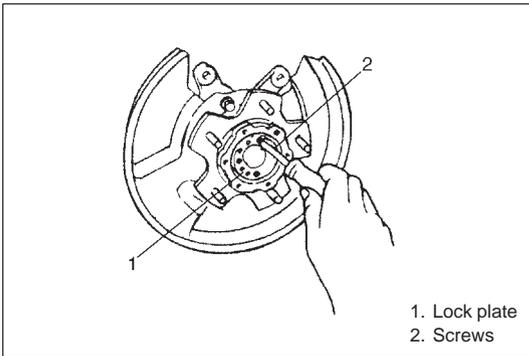
6') Remove front wheel bearing lock plate by loosening 4 screws (for 2WD).
