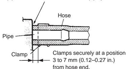
With following type pipe, fit hose as far as its peripheral projection as shown.
