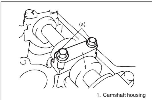
8) Install camshaft housing (1) and tighten them to specified torque.
