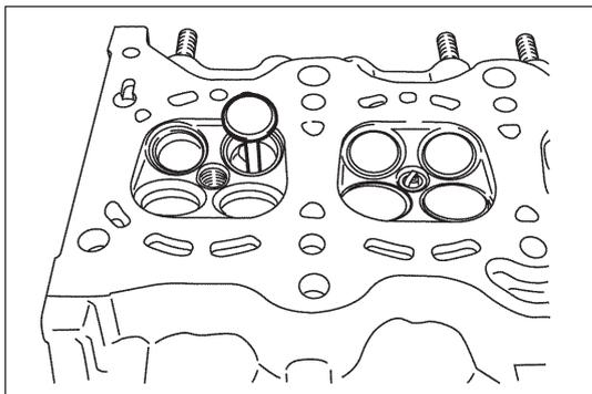
6) Install valve to valve guide.
