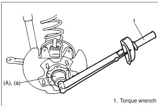
10) Tighten wheel bearing lock nut to specified torque while turning wheel hub by hand.
