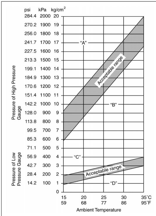
8) Check for each pressure of low side and high side if it is within shaded range of graph.
