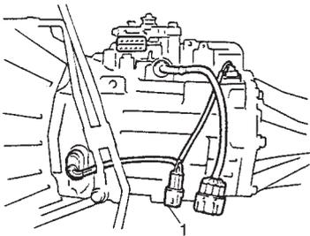
1. A/T output shaft speed sensor – input/turbine speed sensor coupler
