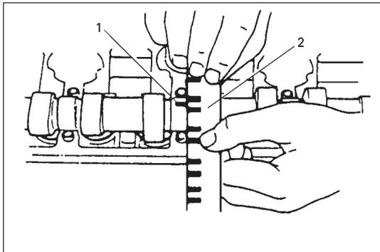
7) Remove housing, and using scale (2) on gaging plastic (1) envelop, measure gaging plastic width at its widest point.
