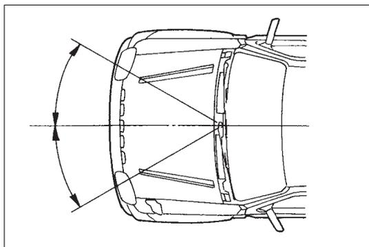
The air bag system is designed to activate only in severe frontal collisions. It is not designed to activate in rear impacts, side impacts, rollovers, or minor frontal collisions, since it would offer no protection in those types of accidents.
