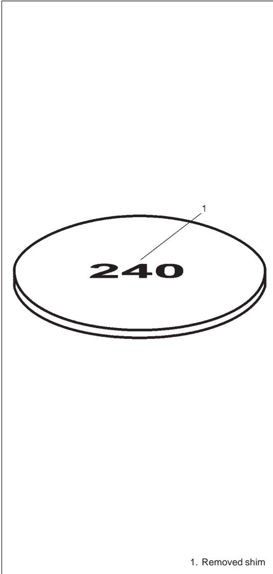
5) Check removed shim for No. (1) and determine replacement shim by calculating shim No. with the following formula and table.
