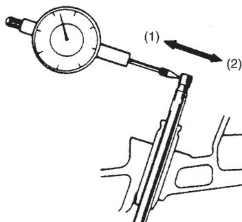
If bore gauge is not available, check end deflection of valve stem with a dial gauge instead.
