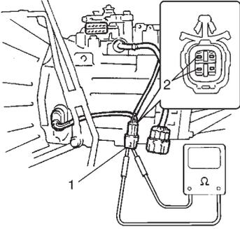
1. A/T output shaft speed snsor – Input/Turbine speed sensor coupler
