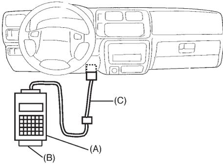
When using duty meter (Vehicle without immobilizer indicator lamp):
