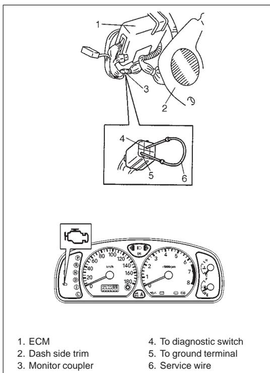
EXAMPLE: When serial data link wire is defective (Code No.83)
