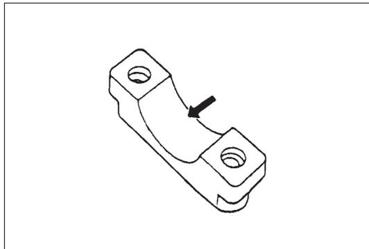
Check clearance by using gaging plastic. Checking procedure is as follows.
