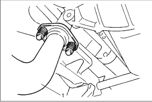
5) Disconnect exhaust pipe (1) from exhaust manifold.
