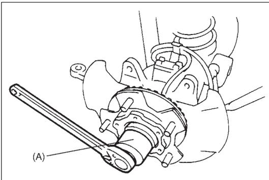
7) Uncaulk front wheel bearing lock nut (for 4WD).
