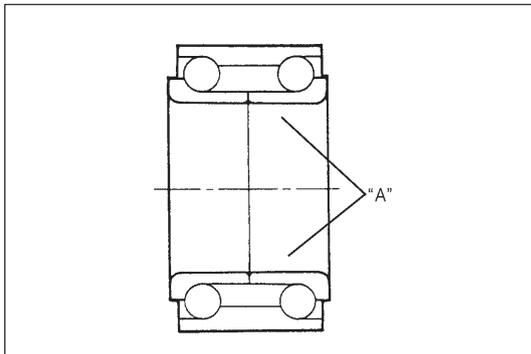
7) Apply lithium grease inside wheel bearing thin.
