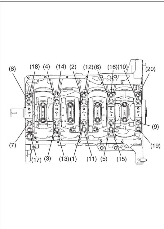
Tighten bearing cap No.1 bolts (1) – (10) and No.2 bolts (11) – (20) gradually as follows.
