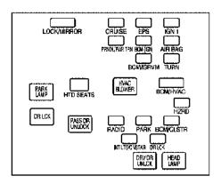
The instrument panel fuse block is located on the passenger's side of the instrument panel.
