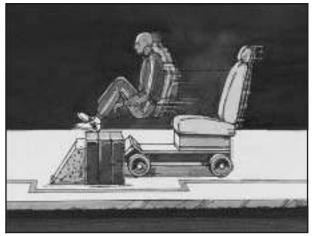
Get it up to speed. Then stop the vehicle. The rider does not stop.  $% \left\{ 1,2,\ldots,n\right\}$
