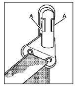
To move it up or down, squeeze the release buttons (A) together and move the height adjuster to the desired position.
