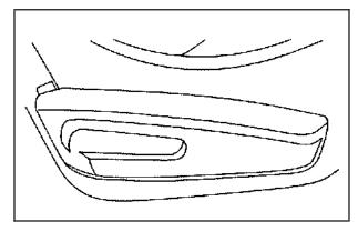
Lift the recliner lever, located on the outboard side of the seat, up fully and fold the seatback forward.
