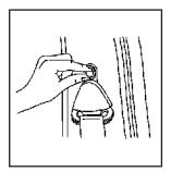
To move it down, press the release button and move the height adjuster to the desired position. You can move the height adjuster up just by pressing up on the shoulder belt quide.
