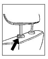
Press the button on the side of the head restraint to adjust it.
