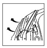
Gently pull the radiator cover/front grill toward you and pull the front grill trim bar away from the headlamp lens. The front grill bar is attached to the headlamp lens with a hidden clip.
