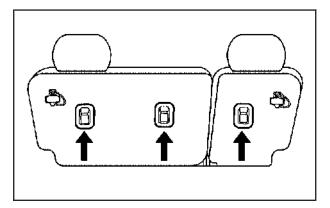
Your vehicle has top strap anchors in the rear seating positions. The anchors are located on the back of the rear seatback. Be sure to use an anchor point located on the same side of the vehicle as the seating position where the child restraint will be placed. You may need to fold down the plastic panel in the rear cargo area to access the anchors. If the position you are using has an adjustable head restraint, raise the head restraint and route the top strap under it.
