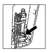
Install the jack in the left side panel of cargo area and secure with the wing bolt.
