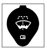
Open the cap with the washer symbol on it. Add washer fluid until the tank is full. See *Engine Compartment Overview on page 5-12* for reservoir location.
