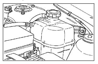
The surge tank is located on the driver's side of the engine compartment. See *Engine Compartment*Overview on page 5-12 for more information on location.
