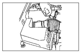
3. Disconnect the crank case ventilation tube.
