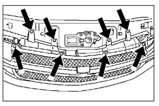
Remove the fastener plugs from the top of the radiator cover/front grill.
