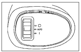
(Off): The lamp will not come on as long as the switch is in this position.
