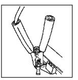
To access the remote positive (+) terminal, remove the fuse block cover.
