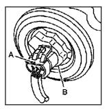
6. Press the clip (A) on the electrical connector when replacing the low-beam or high-beam bulb, then pull it straight off. Turn the bulb retaining ring (B) counterclockwise to remove it and then pull the bulb assembly straight out.
