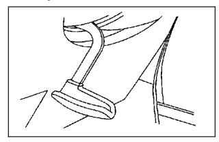
The lever to tilt the steering wheel is located on the left side of the steering column.
