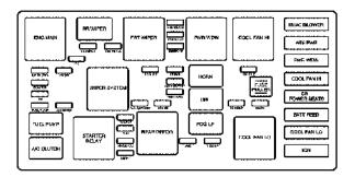
The engine compartment fuse block is located on the driver's side of the engine compartment.
