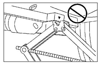
Do not lift the vehicle using the plastic lower body panel.
