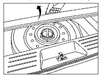
Lift the load floor up and pull it out of the vehicle and set it aside.
