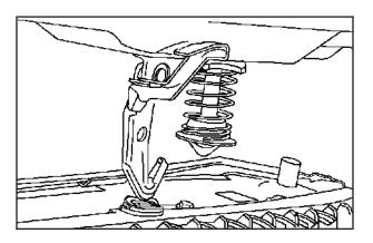
Then go to the front of the vehicle and lift up on the secondary hood release lever.
