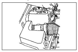
2. Disconnect the air flow sensor electrical connector.
