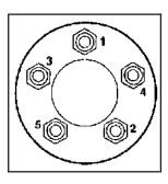
15. Tighten the wheel nuts firmly in a crisscross sequence, as shown.
