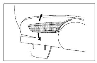
If your vehicle has a manual driver seat height adjuster, it is located on the outboard side of the seat toward the front of the seat cushion. To raise the seat, move the lever upward repeatedly until the seat is at the desired height. To lower the seat, move the lever downward repeatedly until the seat is at the desired height.
