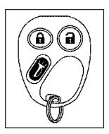
button on the remote keyless entry transmitter one time to lock the doors. The headlamps will flash once. This also arms the content theft-deterrent system.
