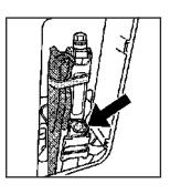
Remove the wing-bolt on the jack and then remove it.
