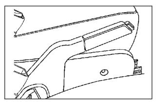
The parking brake lever is located to the right of the driver's seat.
