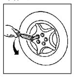
Loosen all five hex-shaped plastic caps by turning the wrench counterclockwise. Do not try to remove plastic caps from the cover or center cap.
