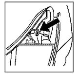
Carefully slide the taillamp assembly outward to clear the stud (see arrow) and then rearward and away from the body of the vehicle.
