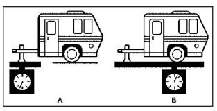
If you are using a weight-carrying or a weight-distributing hitch, the trailer tongue weight (A) should be 10 percent to 15 percent of the total loaded trailer weight (B). Do not exceed the maximum allowable tongue weight for your vehicle.
