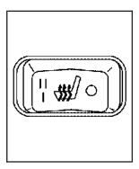
The switches for the heated seats, if equipped, are located on the outboard sides of the front seats.
