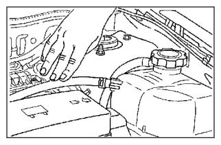
4. With the coolant surge tank pressure cap off, start the engine and let it run until you can feel the upper radiator hose getting hot. Watch out for the engine cooling fans.
