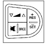
If your vehicle has this feature, some audio controls can be adjusted at the steering wheel. They include the following:  $\nabla$  **SEEK**  $\triangle$ : Press the up or the down arrow to go to the next or to the previous radio station and stay there. The radio will only seek stations with a strong signal that are in the selected band.
