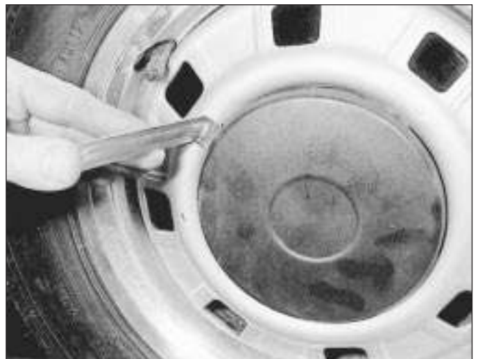
Levering off the hub cover
