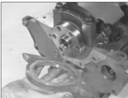
15.15 Use new gasket when refitting left-hand oil seal carrier
