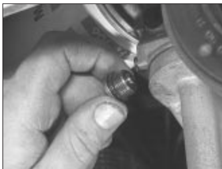
14.9a Unscrew threaded plug - seen through right-hand wheel arch . . .
