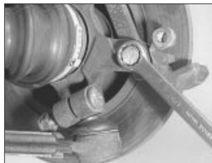
3.6 Undoing a brake caliper anchor bracket bolt
