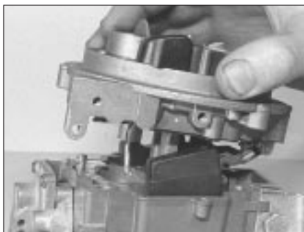
20.5b ... then detach the carburettor upper body
