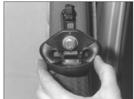
41.11 Removing a seat belt upper anchor cover
