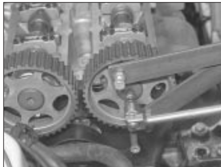
11.3 Using forked holding tool while camshaft toothed pulley bolt is slackened
