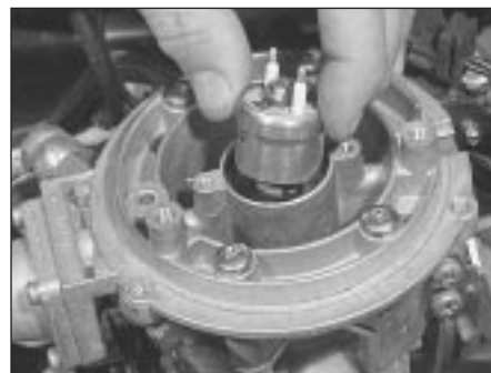
14.5c Withdrawing the injector from the CFI unit
