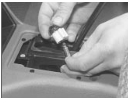
6.3a Remove the selector illumination bulb cover . . .
