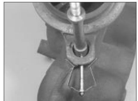
2.2e Release the spring clip to extract the securing bolt from the manifold, when required
