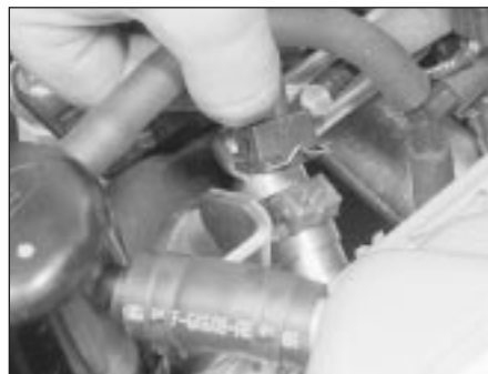
14.9a Disconnect the wiring multi-plug from each injector . . .
