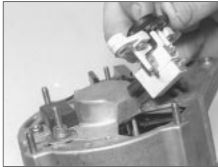
7.3b . . . withdraw the brush box/regulator unit (Bosch alternator)
