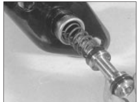
9.8b . . . followed by the secondary piston assembly
