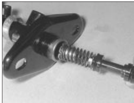
9.8a Removing the primary piston assembly from the master cylinder . . .
