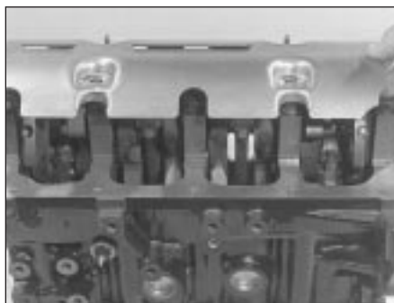
11.6 Removing the oil baffle to provide access to crankshaft and bearings
