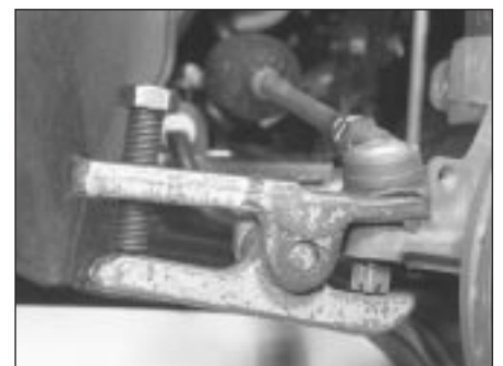
28.3 Balljoint separator tool in position. Note that the nut should be left loosely in position to protect the thread for re-use
