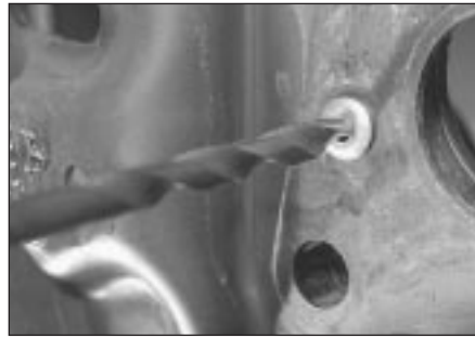
8.6 Drilling out a pop-rivet securing the brake backplate to the axle flange
