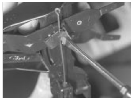
11.7c Releasing inner cable core from heater control lever
