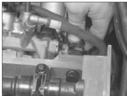
14.41 Disconnecting the camshaft position sensor wiring multi-plug (Zetec engine shown)
