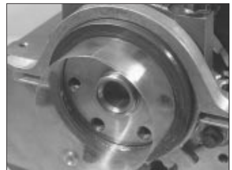
15.18 Using guide made from thin sheet of plastic to slide oil seal lips over crankshaft shoulder
