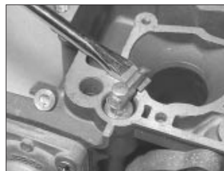
24.10 Carefully prising out the accelerator pump discharge tube assembly
