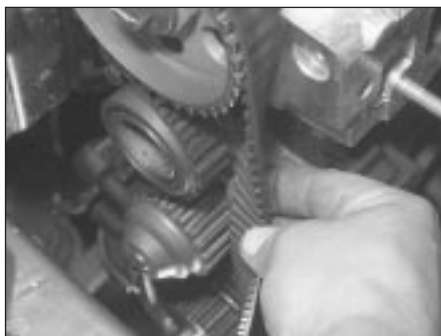
8.13 Checking the tension of the timing belt
