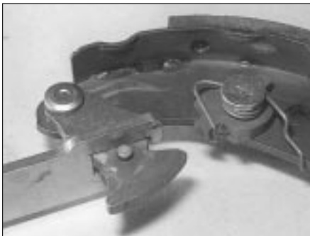
6.7a Release the automatic brake adjuster cam and pawl
