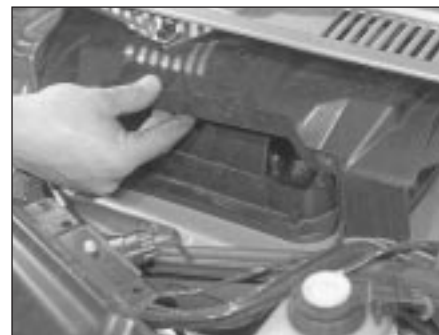
11.16 Removing the cover from the heater fan motor assembly
