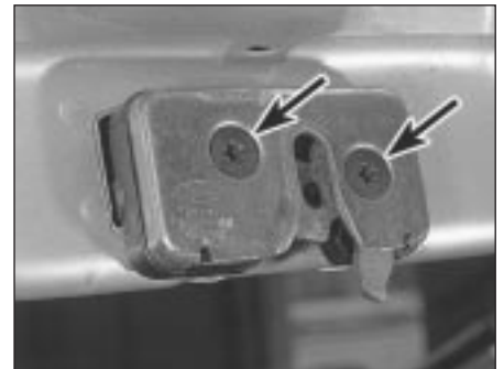
27.2 Tailgate latch and its Torx securing screws (arrowed)
