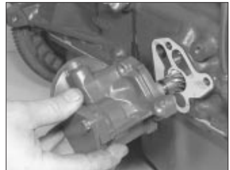
12.7 Refitting the oil pump. Note the new gasket
