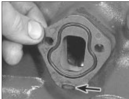
7.11 Gasket/spacer fitment on HCS engine. Note position of the lug (arrowed)
