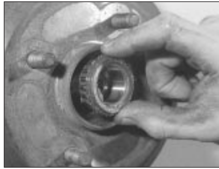
9.7 Removing a bearing cone from the hub bore
