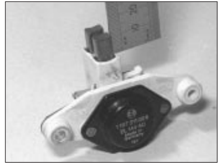
7.4 Measuring the brush lengths (Bosch alternator)
