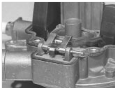
20.6a Slide out the float retaining pin ...
