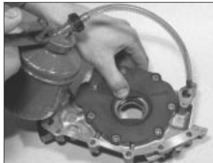
14.8 Prime the oil pump prior to fitting
