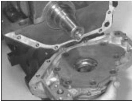
14.9a Refit the oil pump
