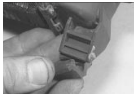
7.6b Rubber insulator on radiator locating lug
