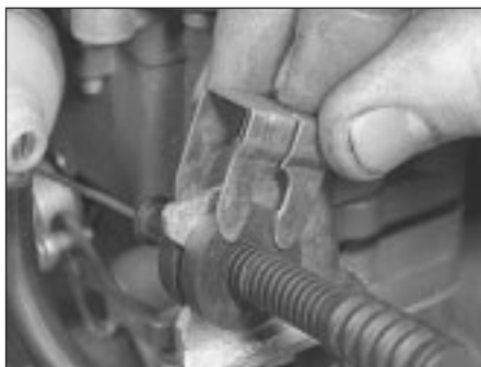
3.5a Remove the accelerator outer cable securing clip . . .
