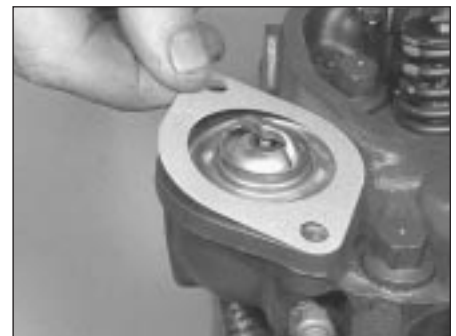
4.7a Removing the gasket and thermostat from an HCS engine
