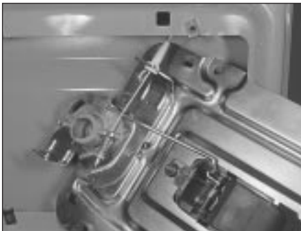
30.2b Latch assembly released - disconnect cables to withdraw
