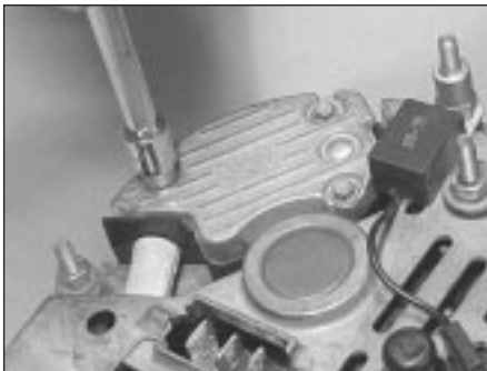
7.7a Removing the regulator and brushbox assembly securing screws (Magnet-Marelli alternator)
