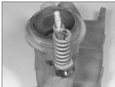
2.2c Showing securing bolts - note coil spring, and shoulder on bolt
