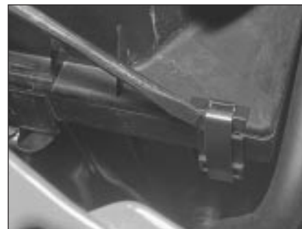
24.6 On EFI fuel injection engines, release the retaining clips and lift off the air cleaner lid
