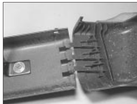
16.19b ... Courier rear bumper end moulding unclipped
