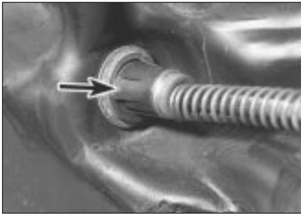
8.3 Compress the retaining lugs (arrowed), and release the handbrake cable from the backplate
