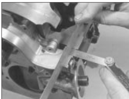
14.13 Oil pump must be positioned accurately
