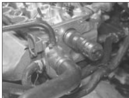
11.12 Withdraw the camshaft from the cylinder head
