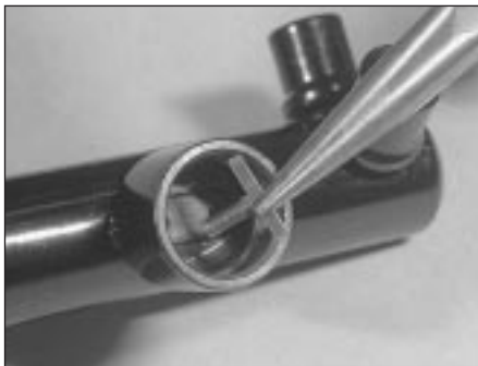
9.7 Removing the secondary piston retaining pin
