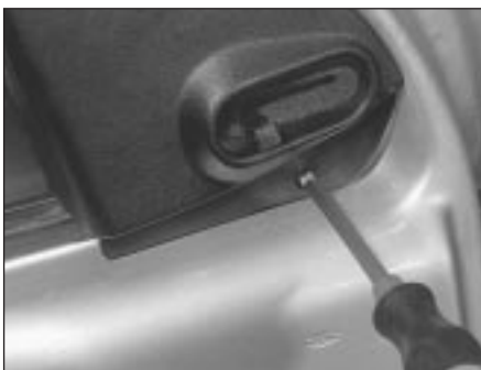
18.7 Removing the mirror trim retaining screw
