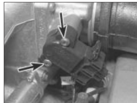
14.46 Throttle position sensor mounting screws (arrowed)
