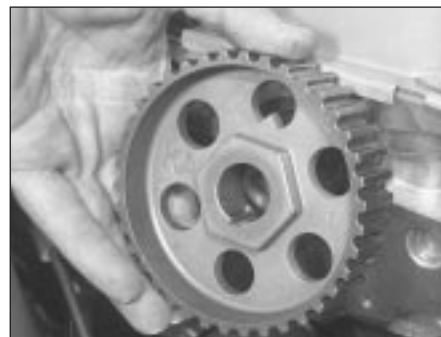
9.13a Refit the camshaft sprocket ...
