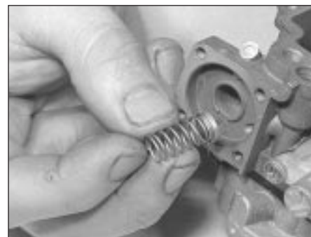
24.11c ... and the return spring and valve assembly
