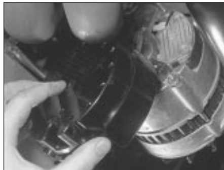
6.8 Removing the splash cover from the inner end of the alternator
