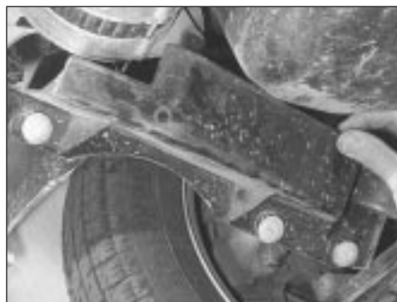
6.3 Removing the drivebelt splash guard (where fitted)
