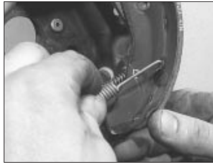
6.4a Detach the lower pull-off spring
