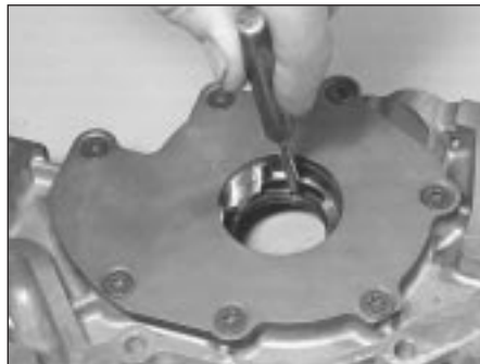
15.2 Driving out crankshaft right-hand oil seal
