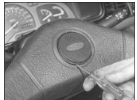
19.2 Removing the motif from the steering wheel
