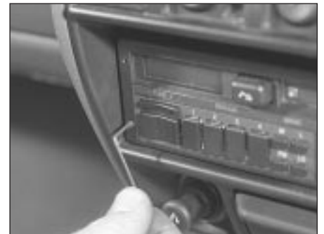
22.2 Unscrewing the securing pins from the radio/cassette player
