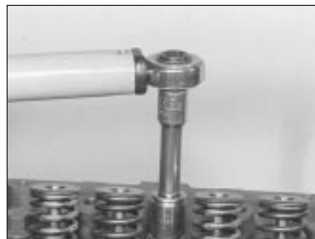
7.27b Tightening the cylinder head bolts (Stage 1)
