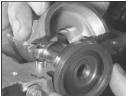
10.6 Alternatively, seal can be inserted when camshaft bearing cap is unbolted
