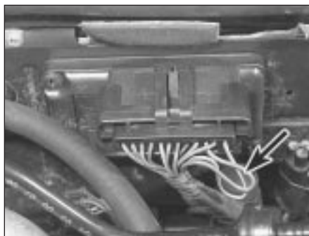
7.19 Pulse-air solenoid valve location (arrowed) under ignition module
