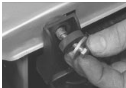
7.6a Radiator securing bolt, insulator and washer
