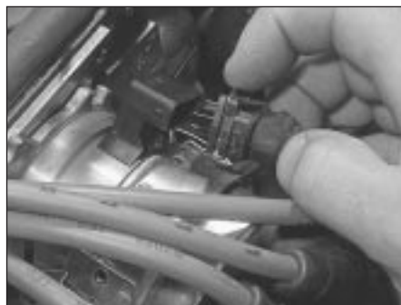
7.4a Disconnecting the distributor multi-plug
