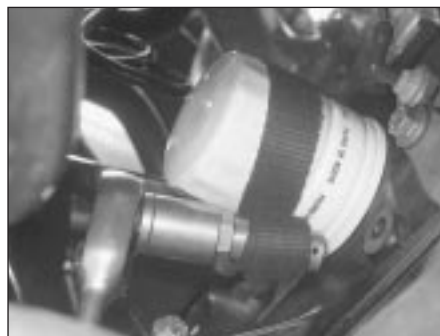
3.9 Removing the oil filter on the CVH engine using a strap wrench
