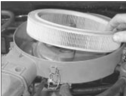
24.10a Removing the air filter element on carburettor engine models . . .
