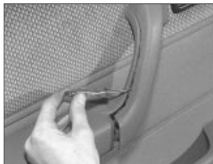
21.4a Detaching armrest/doorpull removable panel
