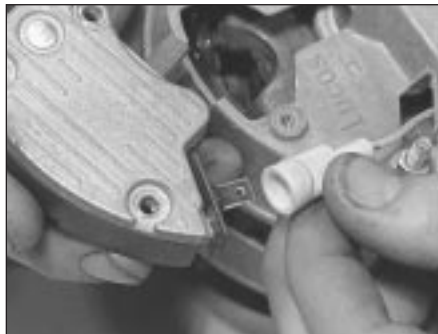
7.7b Disconnecting the field connector (Magnet-Marelli alternator)
