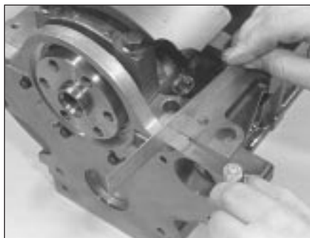
15.16 Oil seal carrier must be positioned accurately
