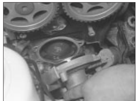
10.5b . . . and remove the Zetec engine water pump
