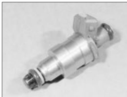
14.13 Remove the seals from the injectors
