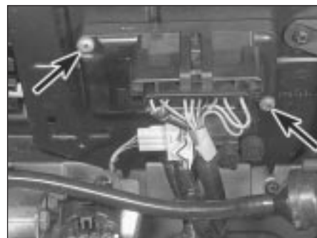
5.5 Ignition module location on bulkhead panel. Note retaining screws (arrowed)
