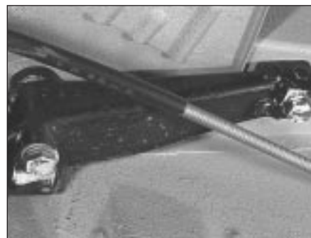
17.7 Courier rear suspension pivot brackets locate on dowels in underbody
