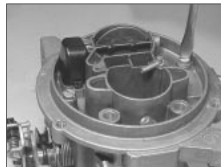
20.5a Remove the carburettor upper body securing screws . . .
