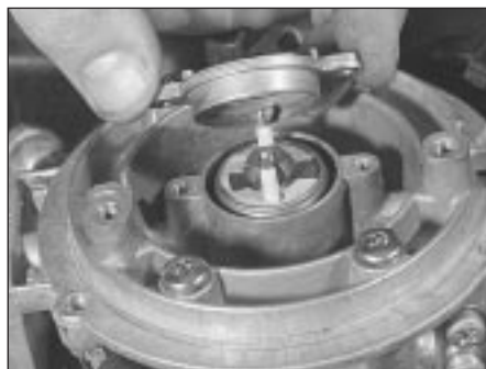
14.5b Removing the injector retaining collar
