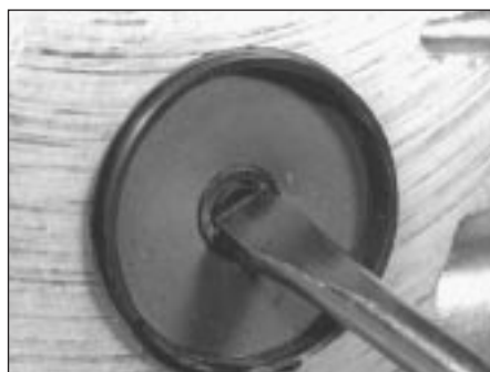
11.11a Pierce the centre of the blanking plug ...
