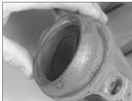
2.2d Renew the exhaust system downpipe-to-manifold gasket to prevent leaks
