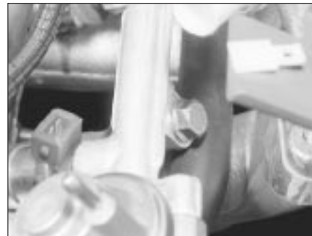
14.12a Remove the fuel rail retaining bolts . . .
