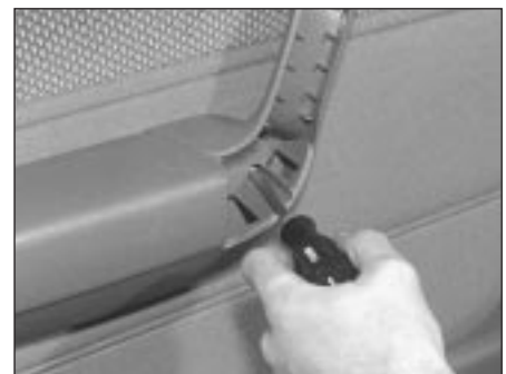
21.4b Undoing armrest/doorpull retaining screws
