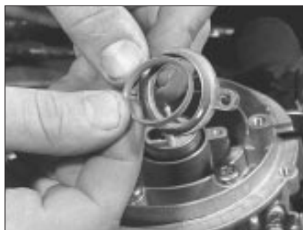
14.5e Withdrawing the seal from the injector retaining collar
