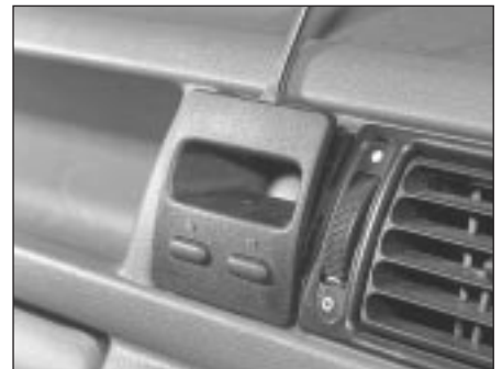
13.2 Carefully prise the clock out of the facia
