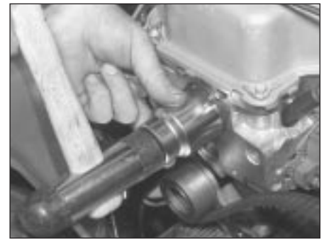
10.3 Using a socket to tap the camshaft oil seal into place
