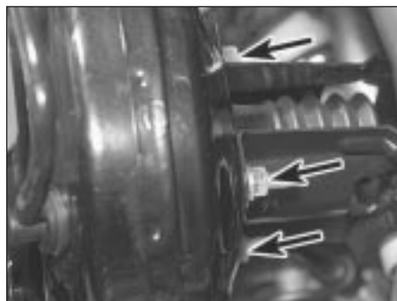
15.6 Nuts securing servo unit to its mounting bracket assembly (arrowed)
