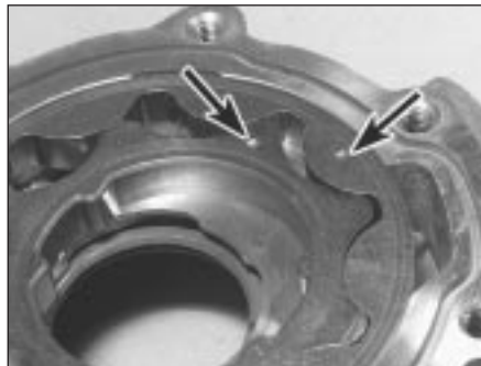
15.4 Inner and outer rotor matchmarks (arrowed)
