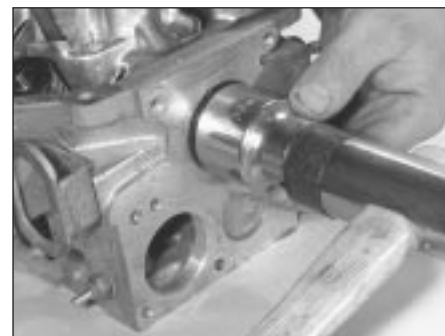
11.22 Driving a new blanking plug into position
