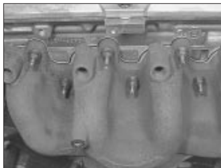
3.13 Exhaust manifold retaining nuts (Zetec engine models)
