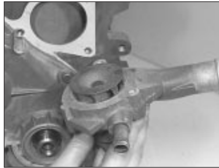
8.6 HCS engine water pump removal
