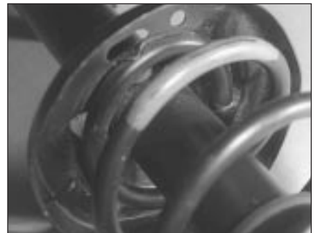
5.9 Correct spring location in its lower seat
