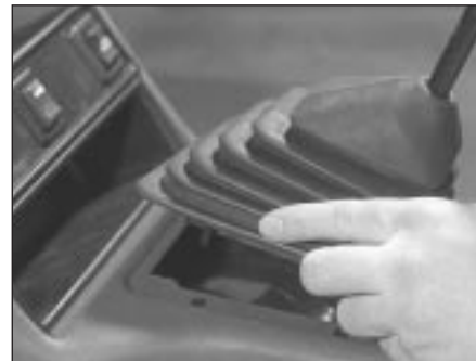
45.3 Removing the gear lever gaiter from the centre console
