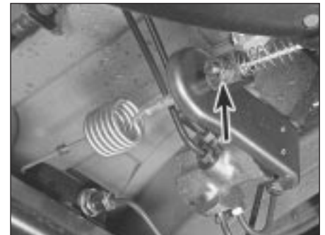
22.3 Light-laden valve linkage adjustment locknut (arrowed)
