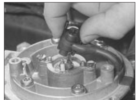
14.4 Disconnect the multi-plug from the injector
