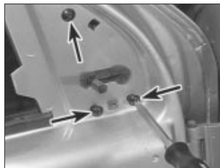
18.8 Removing the three mirror retaining screws (arrowed)
