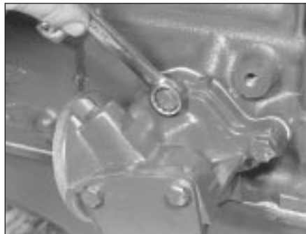
12.4 Unscrewing the oil pump retaining bolts
