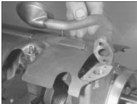
14.16 Use new gasket when refitting oil pick-up pipe to pump
