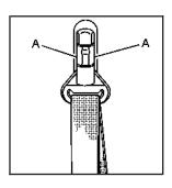
To move it up or down, squeeze the release buttons (A) together and move the height adjuster to the desired position.
