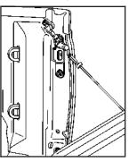
Remove the retaining cable from the passenger side of the tailgate by pulling the clip away from the bolt head while pushing the cable bracket forward.
