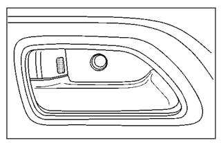
To lock a door from the inside, push the manual lever on the door forward. To unlock a door from the inside, push the lever on the door rearward.
