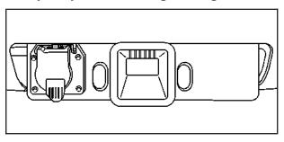
If your vehicle is equipped with a trailer towing package, the rear bumper harness will have a seven-pin universal heavy-duty trailer connector attached to a bracket on the hitch platform.
