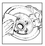
Remove any rust or dirt from the wheel bolts, mounting surfaces and spare wheel. 9. Install the spare tire.
