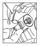
10. Put the wheel nuts back on with the rounded end of the nuts toward the wheel. Tighten each wheel nut by hand. Then use the wheel wrench to tighten the nuts until the wheel is held against the hub.
