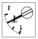
This gage shows the engine coolant temperature.
