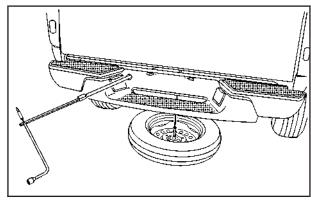
4. Insert the hoist end of the extension through the hole in the rear bumper and into the funnel-shaped guide.
