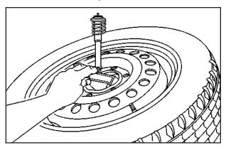
Tilt the retainer downward and through the wheel opening. Make sure the retainer is fully seated across the underside of the wheel.
