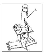
Place the bottom edge of the jack (A) on the wheel blocks (B), separating them so that the jack is balanced securely.
