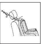
If the position you are using has an adjustable headrest or head restraint and you are using a single tether, raise the headrest or head restraint and route the tether under the headrest or head restraint and in between the headrest or head restraint posts.
