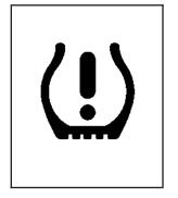
When a low tire pressure condition is detected, the TPMS illuminates the low tire pressure warning light located on the instrument panel cluster.
