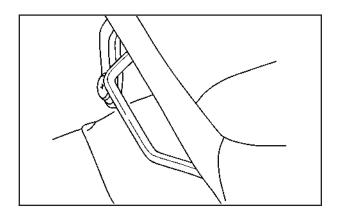
Lift the bar located under the front of the seat to unlock it. Slide the seat to where you want it and release the bar. Try to move the seat with your body to make sure the seat is locked into place.
