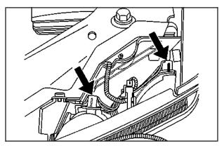
Reach in to access either one of the bulb sockets in the engine compartment.
