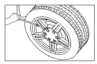
Remove the center cap by placing the chisel end of the wheel wrench (E) into one of the slots on the wheel and gently prying the cap out.
