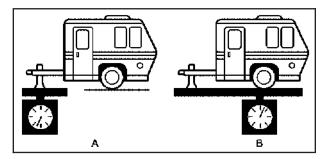
The trailer tongue weight (A) should be 10 percent to 15 percent of the total loaded trailer weight (B), up to a maximum of 600 lbs (272 kg) with a weight carrying hitch.
