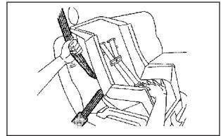
6. To tighten the belt, push down on the child restraint, pull the shoulder portion of the belt to tighten the lap portion of the belt and feed the shoulder belt back into the retractor. If you are using a forward-facing child restraint, you may find it helpful to use your knee to push down on the child restraint as you tighten the belt. You should not be able to pull more of the belt from the retractor once the lock has been set.
