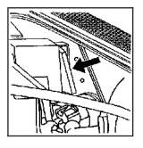
Remove the turn signal/parking lamp assembly by pressing the release clip on the outboard side of the assembly and pulling the outboard end of the assembly toward you.
