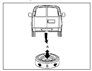
Make sure the tire is stored securely. Push, pull (A), and then try to turn (B) the tire. If the tire moves, use the wheel wrench to tighten the cable. Reinstall the spare tire lock (if equipped). To store the tools, follow these steps:
