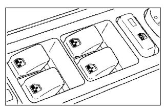
The controls for the power windows are located on the armrest on each of the side doors. The switches operate the windows when the ignition is in RUN, ACCESSORY or while Retained Accessory Power (RAP) is active. See *Retained Accessory Power (RAP)* on page 2-27.
