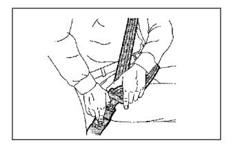
To unlatch the belt, push the button on the buckle.
