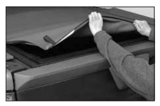
2. Pull the back of the cover out from the rear rail (D).
