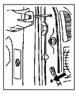
Remove the two rear lamp assembly screws near the tailgate latch and pull out the lamp assembly. 4. Locate the bulb you wish to change.
