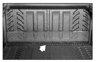
The midgate drain grate is located near the base of the midgate in the cargo area. You will find a removable drain grate covering the drain.
