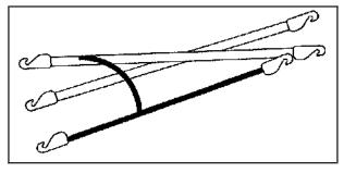
1. Extend the six strap ends on a flat surface.
