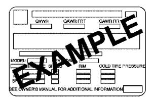
A vehicle specific Certification/Tire label is attached to the rear edge of the driver's door. The label shows the size of your vehicle's original tires and the inflation pressures needed to obtain the gross weight capacity of your vehicle. This is called Gross Vehicle Weight Rating (GVWR). The GVWR includes the weight of the vehicle, all occupants, fuel and cargo.
