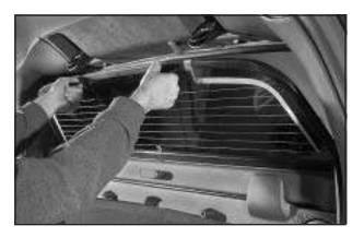
With the rear glass tilted at an angle, place the bottom edge in the lower channel of the window frame.
