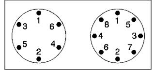
11. Tighten the nuts firmly in a crisscross sequence as shown by turning the wheel wrench clockwise.
