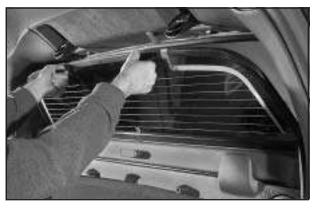
4. With the rear glass tilted toward you, lift it out from the lower window frame channel. Use the grab handles to assist you in removing the rear glass.
