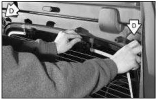
6. Turn both glass lock knobs (D), located at both top corners of the storage pocket, to the locked position. Push in on the corner of the rear glass to allow the lock knob to engage more easily.
