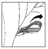
Pull the seat loop located where the seatback and seat cushion meet. The seat cushion will release and allow you to tilt it toward the front of the vehicle.
