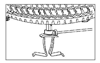
Attach the jack handle, extension, and wheel wrench to the jack and place it (with the wheel blocks) under the vehicle towards the front of the rear bumper.
