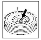
15. Tilt the retainer at the end of the cable and pull it through the wheel opening. Pull the tire out from under the vehicle.
