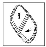
(Trip Information): Press this button to display the odometer, trip odometers, tire pressure for vehicles with a tire pressure monitor, timer, and engine hours.
