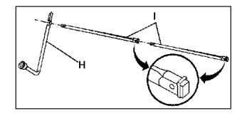
Attach the wheel wrench (H) and extensions (I) together.
