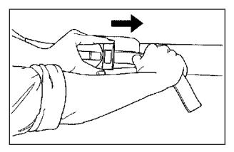
6. Tighten all straps by pulling on the free end of each strap.
