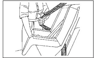
5. Pull the rest of the shoulder belt all the way out of the retractor to set the lock.
