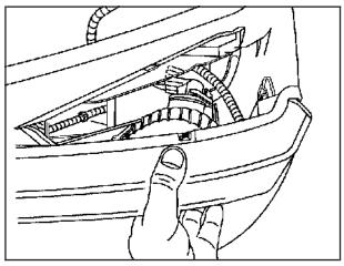
3. Pull the turn signal assembly out from the vehicle.
