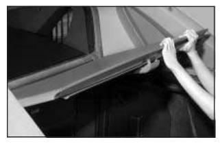
Starting with cargo panel 1, place the latches in the unlocked position. Place cargo panel 1 on the cargo area rails while holding the back of the cargo panel up.
