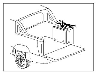
3. Store cargo panel 2 by loading the cargo panel with latches down and facing toward you.
