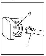
Insert the hoist end (F) through the hole (G) in the rear bumper and into the hoist shaft.
