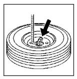
Tilt the retainer downward and through the wheel opening. Make sure the retainer is fully seated across the underside of the wheel.
