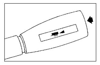
Your vehicle is equipped with a tow/haul mode. The button is located on the end of the column shift lever. You can use this feature to assist when towing or hauling a heavy load. See "Tow/Haul Mode" under Towing a Trailer on page 4-62 for more information.
