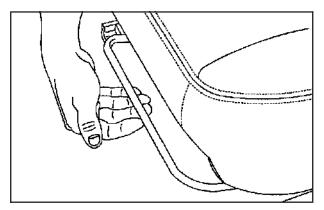
If your vehicle has a manual front passenger split bench seat, you can adjust it with this lever located at the front of the seat.
