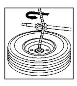
Use the hook on the wheel wrench to pull the hoist cable towards you to assist in reaching the spare tire.
