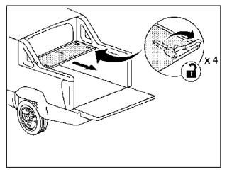
4. If cargo panel 1 needs to be removed. There are latches on both sides that need to be released.
