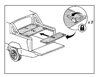
7. Push the latches away from you, starting with the left latch, to lock the panel in place. You should hear a click when each latch locks.
