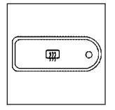
If the vehicle has heated mirrors, the button to turn this function on or off is located on the climate control panel.
