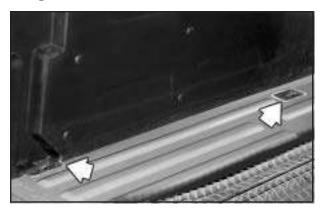
Your vehicle also has four cargo-area floor drains located under the cargo mat near the sides of the cargo area. These drains should be cleaned periodically to allow water to drain from the cargo area.
