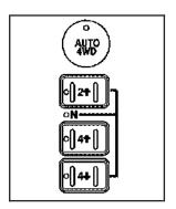
The transfer case buttons are located to the left of the instrument panel cluster.
