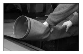
3. Roll the cover toward the front of the vehicle. The plastic lip (E) will release from the siderails (C) as you roll the cover forward.
