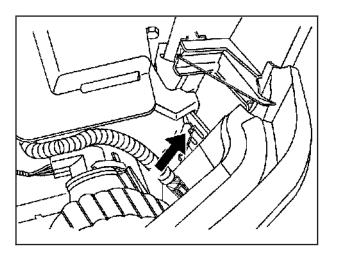
Press the retainer clip (arrow), located behind the turn signal assembly, towards the outside of the vehicle.
