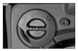
Push both latch levers up to the locked position. You should hear a click when each latch lever locks correctly.
