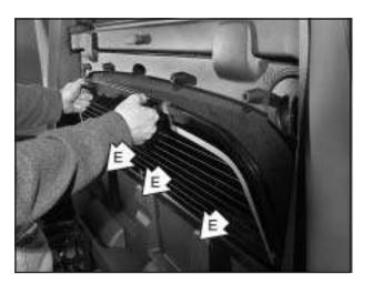
Load the rear glass into the storage pocket in the midgate, guiding the lower edge of the rear glass behind the three rear glass retaining tabs (E).
