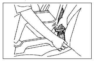
Buckle the belt. Make sure the release button is positioned so you would be able to unbuckle the safety belt guickly if you ever had to.
