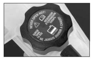
You can remove the coolant surge tank pressure cap when the cooling system, including the coolant surge tank pressure cap and upper radiator hose, is no longer hot. Turn the pressure cap slowly counterclockwise about one full turn.
