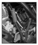
The remote positive (+) terminal is located near the engine accessory drive bracket. On some vehicles, the terminal may be under a red plastic cover. To access the remote positive (+) terminal, open the red plastic cover, if equipped.
