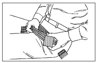
When you sit in a center front seating position, you have a lap safety belt, which has no retractor. To make the belt longer, tilt the latch plate and pull it along the belt.
