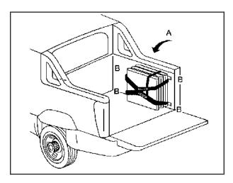
5. Move the rest of the strap system inside the cargo box, covering the three cargo covers (A). Fasten the four strap clips (B).
