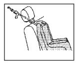
If the position you are using has an adjustable head restraint and you are using a single tether, raise the head restraint and route the tether under the head restraint and in between the head restraint posts.
