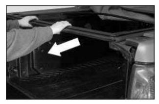
Remove the rear rail by pulling it straight out from the side rails. Set the rail aside.
