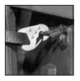
Secure the storage strap system in the cargo storage area by attaching the six clips included on the cargo strap system to the tie down locations on either side of the storage area.
