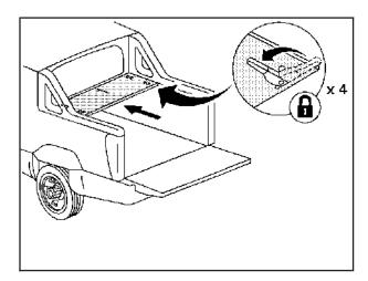
Push both left latches away from you to lock the latches. Remember that there are two latches on each side for panel 1. You should hear a click when each latch locks. Lock the remaining two right latches on panel 1.
