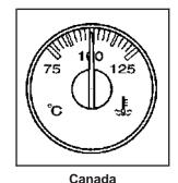
This gage shows the engine coolant temperature.
