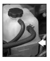
When the engine is cold, the coolant level should be at or above the FULL COLD mark. If it is not, you may have a leak at the pressure cap or in the radiator hoses, heater hoses, radiator, water pump or somewhere else in the cooling system.
