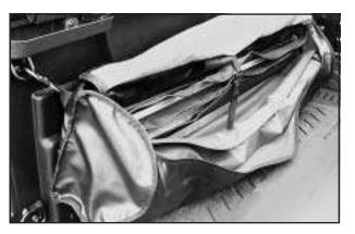
Stow both bows and the front and rear rails in the storage bag. When all components of the tonneau cover are secured in the bag properly, zip the bag shut.
