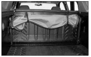
4. Stow the cover using the buckles and the straps attached to the front rail.
