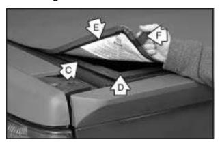
Starting at the rear corner of the driver's side of the vehicle, pull the loop (F) toward you and then pull up so the plastic lip (E) releases from the channel in the rear rail (D) and the side rail (C).
