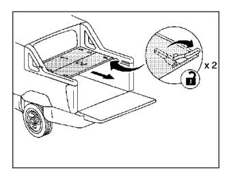
Pull each cargo panel up and then out from the side rails and set it aside. Remove as many cargo panels as needed.
