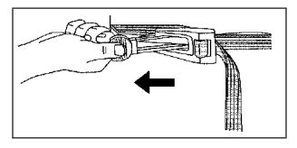
7. Close both cross locks at the center of the strap system to secure tightly.
