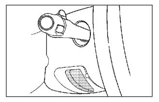
The tilt lever is located on the driver's side of the steering column under the turn signal lever.
