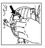
Press the release tab and turn the bulb socket counterclockwise to remove it from the taillamp assembly.
