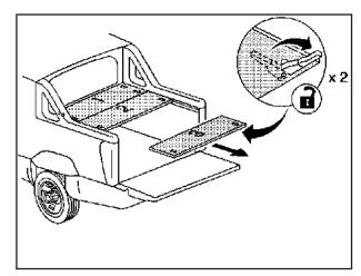
Remove cargo panel 3 by pulling the left and right cargo panel latches, located on the bottom of each cargo panel, forward to unlock the cargo panel latches.
