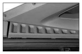
The top drain grates are located near the rear glass on both sides of the vehicle. You may need to clean the grates and drains if there seems to be a blockage. To remove each drain grate, do the following:
