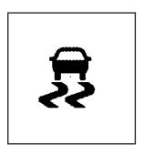
StabiliTrak® and part of the traction control system can be turned off or back on by pressing the StabiliTrak® button on the instrument panel.
