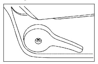
If the seats have manual reclining seatbacks, the lever is located on the outboard side of the seat cushions. To adjust the seatback, lift the lever. Release the lever to lock the seatback where you want it.
