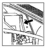
Remove the turn signal/parking lamp assembly by pressing the release clip on the outboard side of the assembly and pulling the outboard end toward you.
