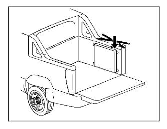
2. Starting with cargo panel 1, load the cargo panel with latches up and facing away from you.
