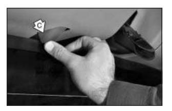
While holding the rear glass in place, press the glass-catch release button (C) and pull the top of the rear glass toward you using the grab handle(s) (B) located at the top of the rear glass.
