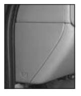
The fuse block access door is on the driver's side edge of the instrument panel. Pull off the cover to access the fuse block.
