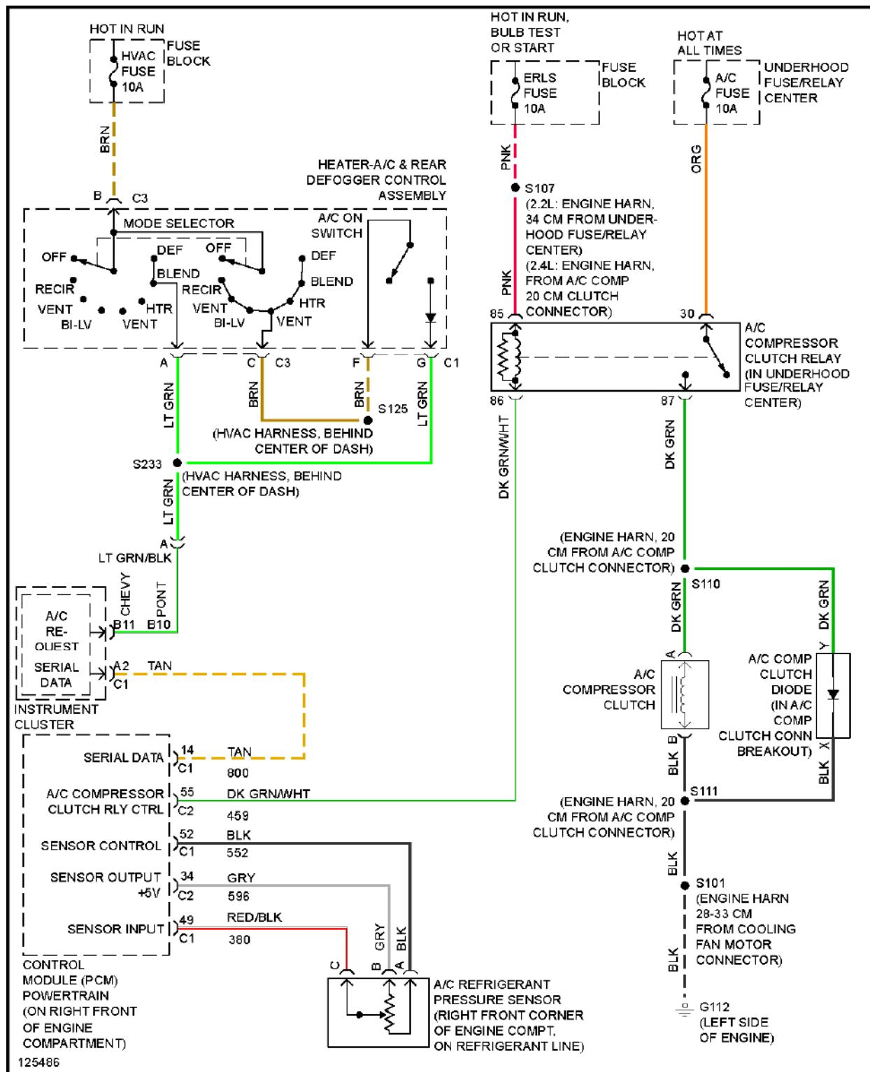
**Fig. 1: Compressor Circuit**
