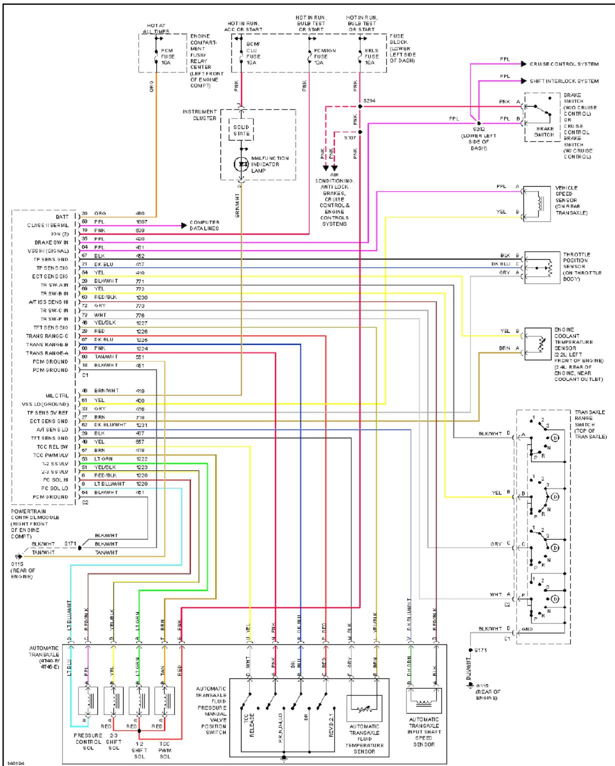
**Fig. 45: 2.4L VIN T, A/T Circuit**
