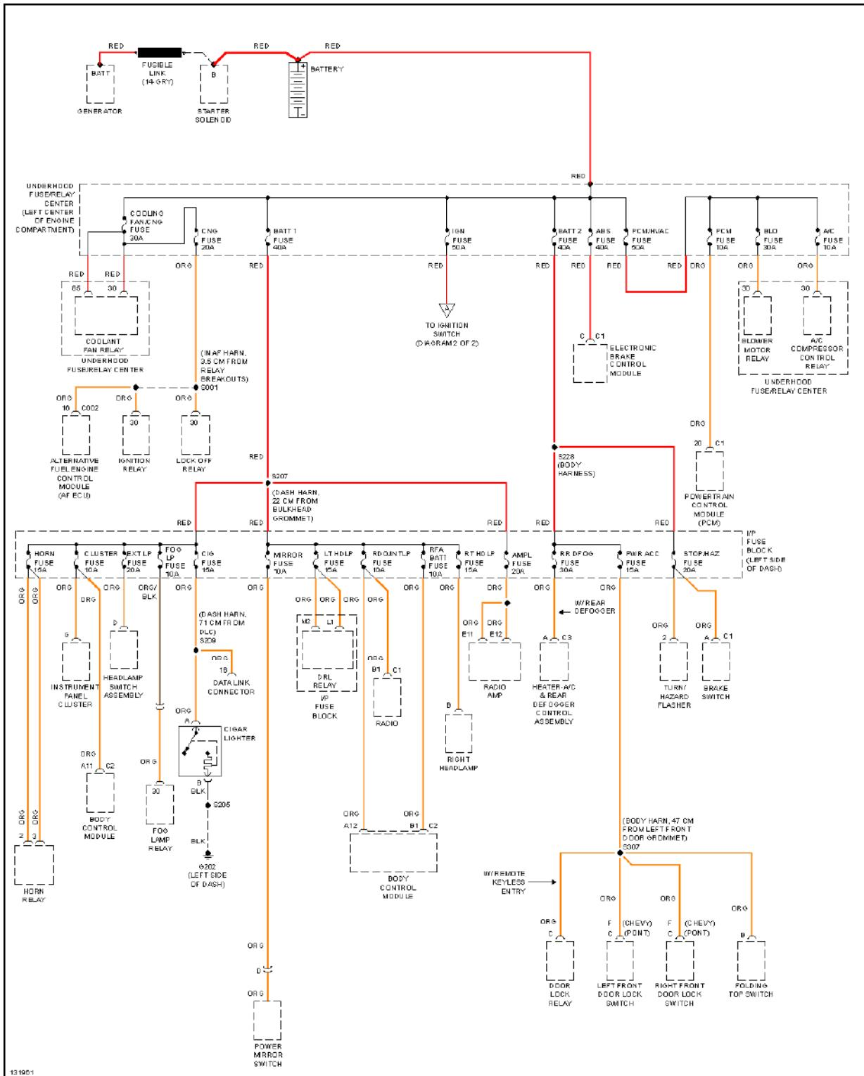
**Fig. 28: Power Distribution Circuit (1 of 2)**
