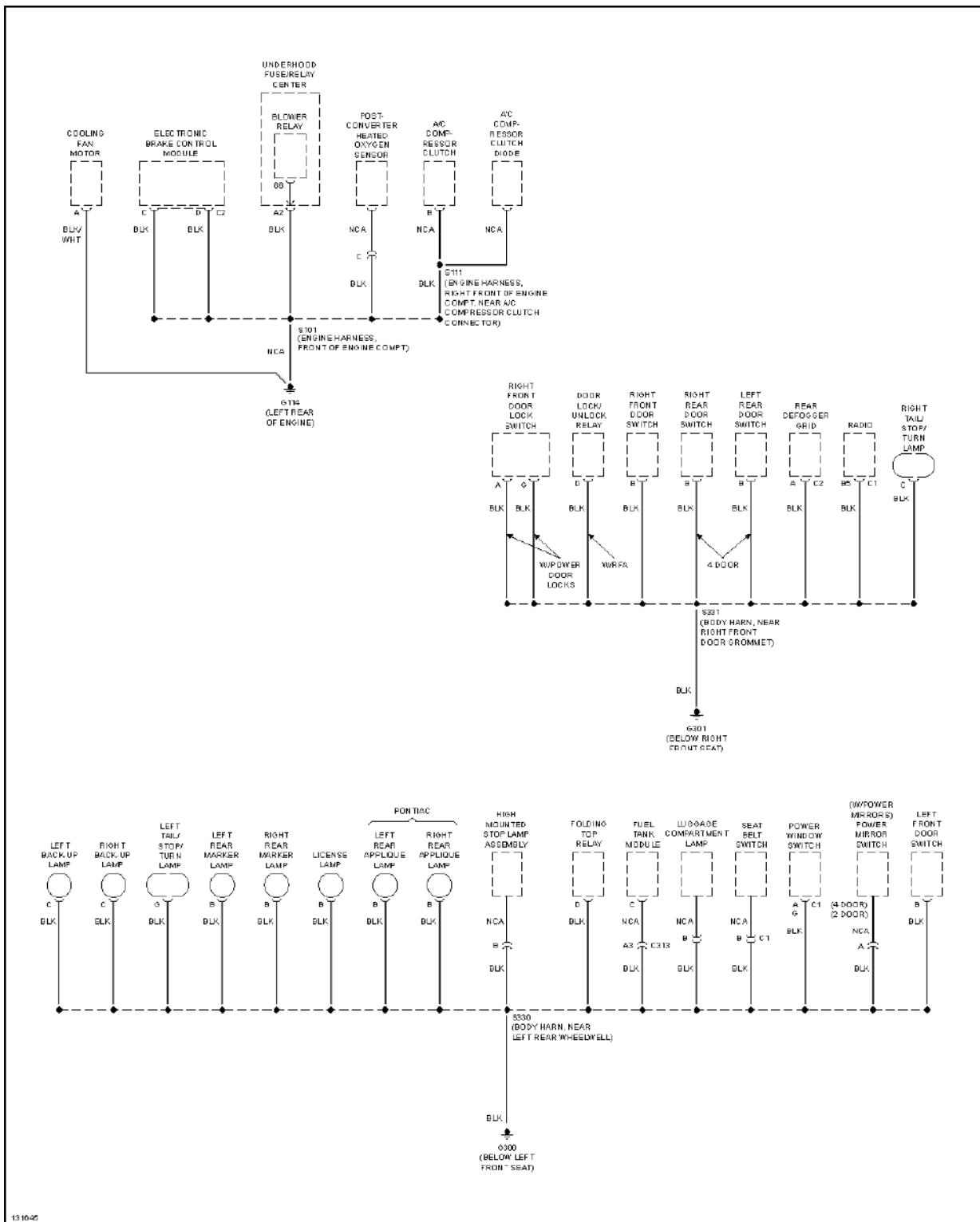
**Fig. 21: Ground Distribution Circuit (3 of 3)**
