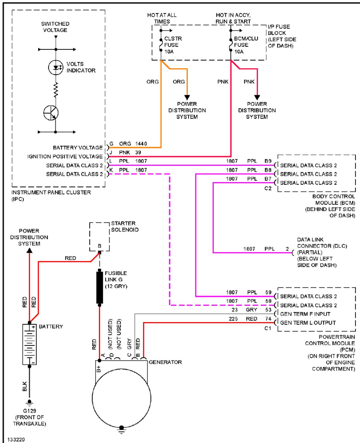
**Fig. 40: Charging Circuit**
