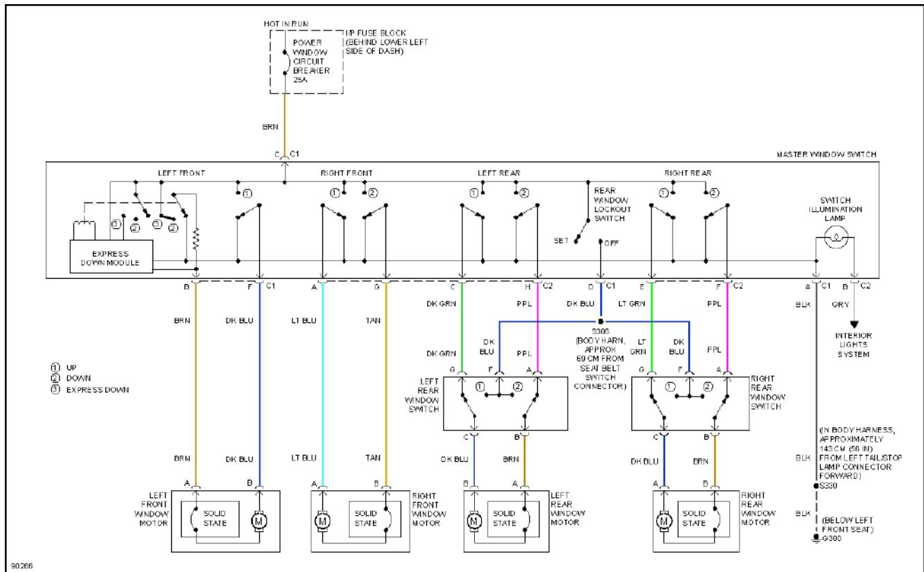
**Fig. 36: Power Window Circuit, 4 Door**
