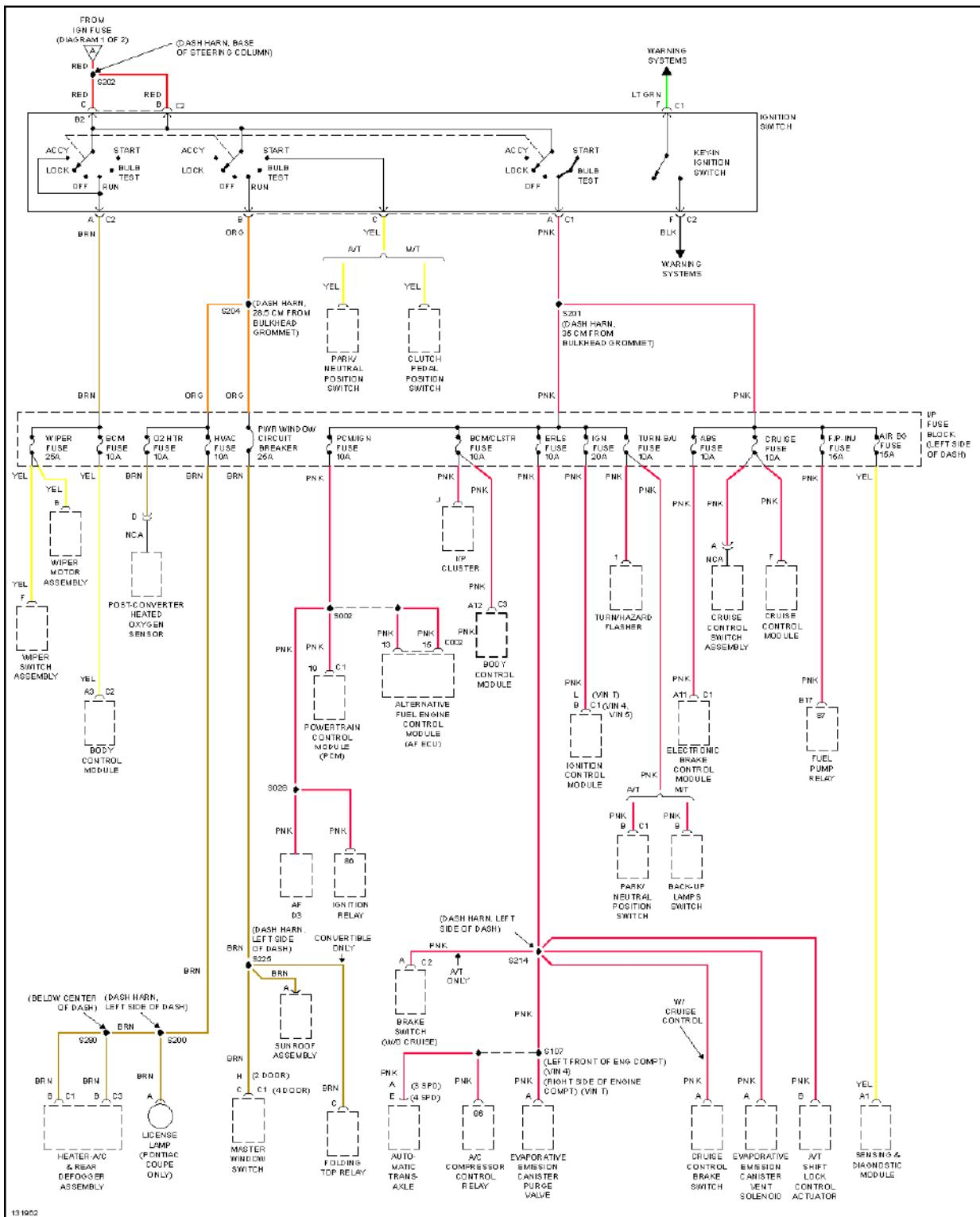
**Fig. 29: Power Distribution Circuit (2 of 2)**
