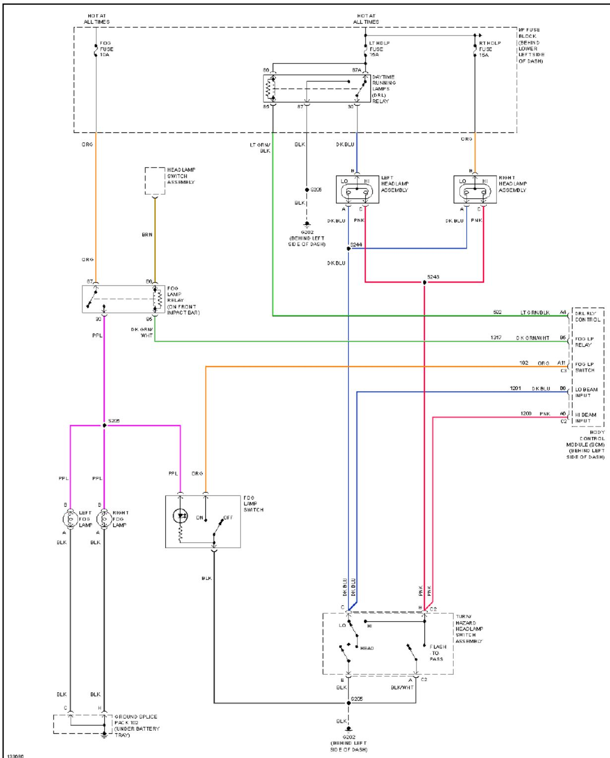
**Fig. 22: Headlight Circuit**
