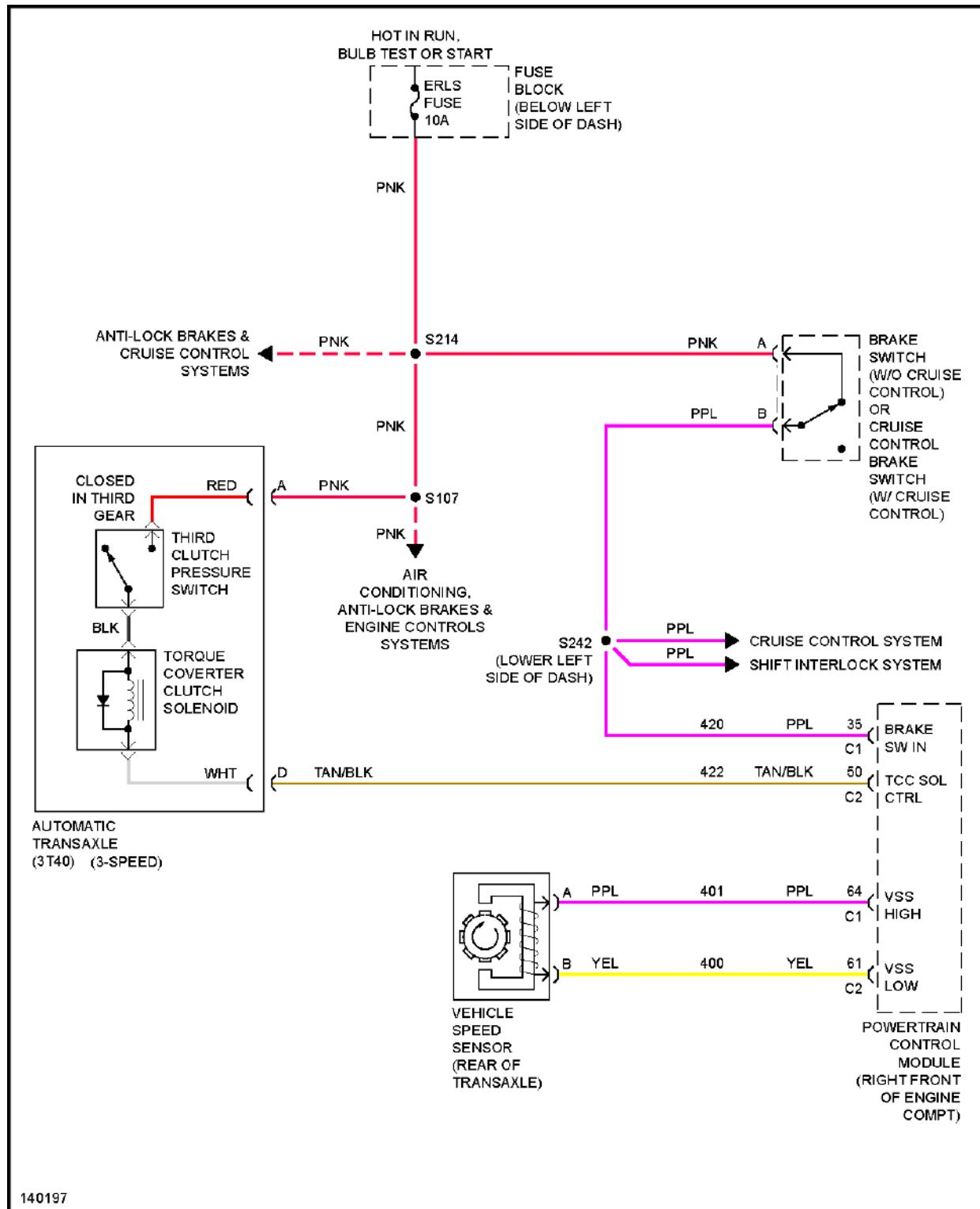
**Fig. 44: 2.2L VIN 4, TCC Solenoid Circuit**
