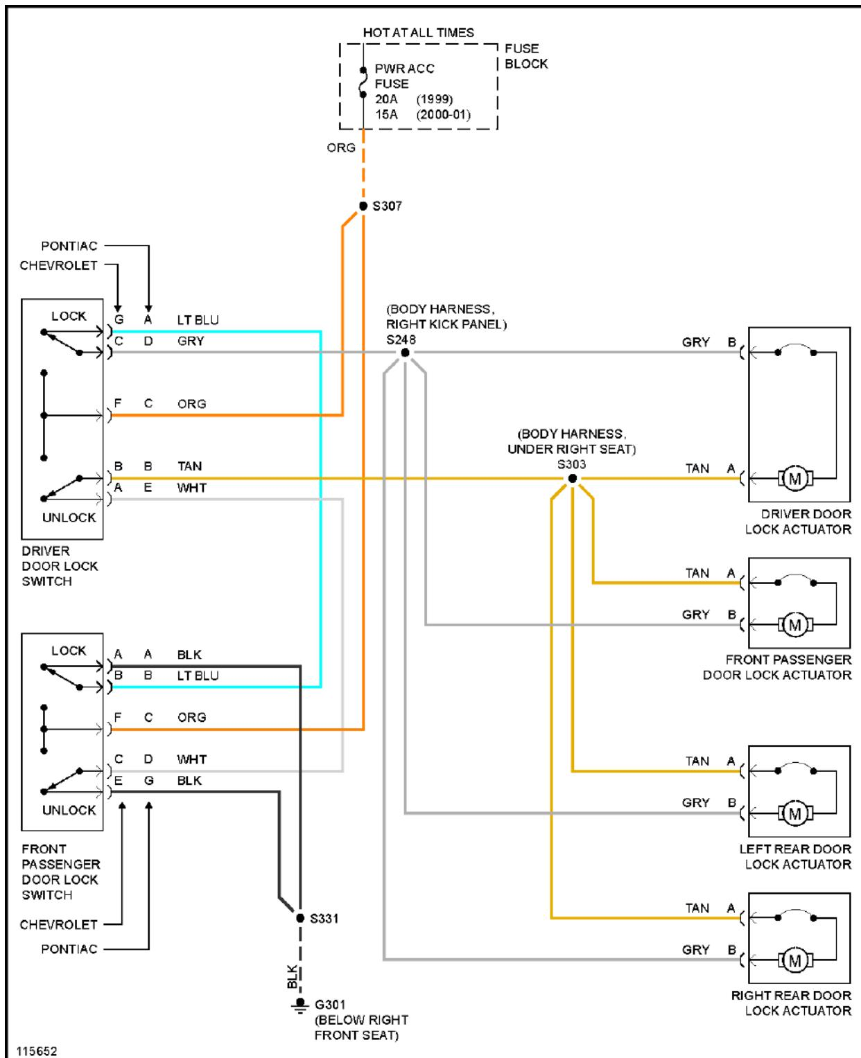
**Fig. 31: Power Door Lock Circuit, W/O Keyless Entry**
