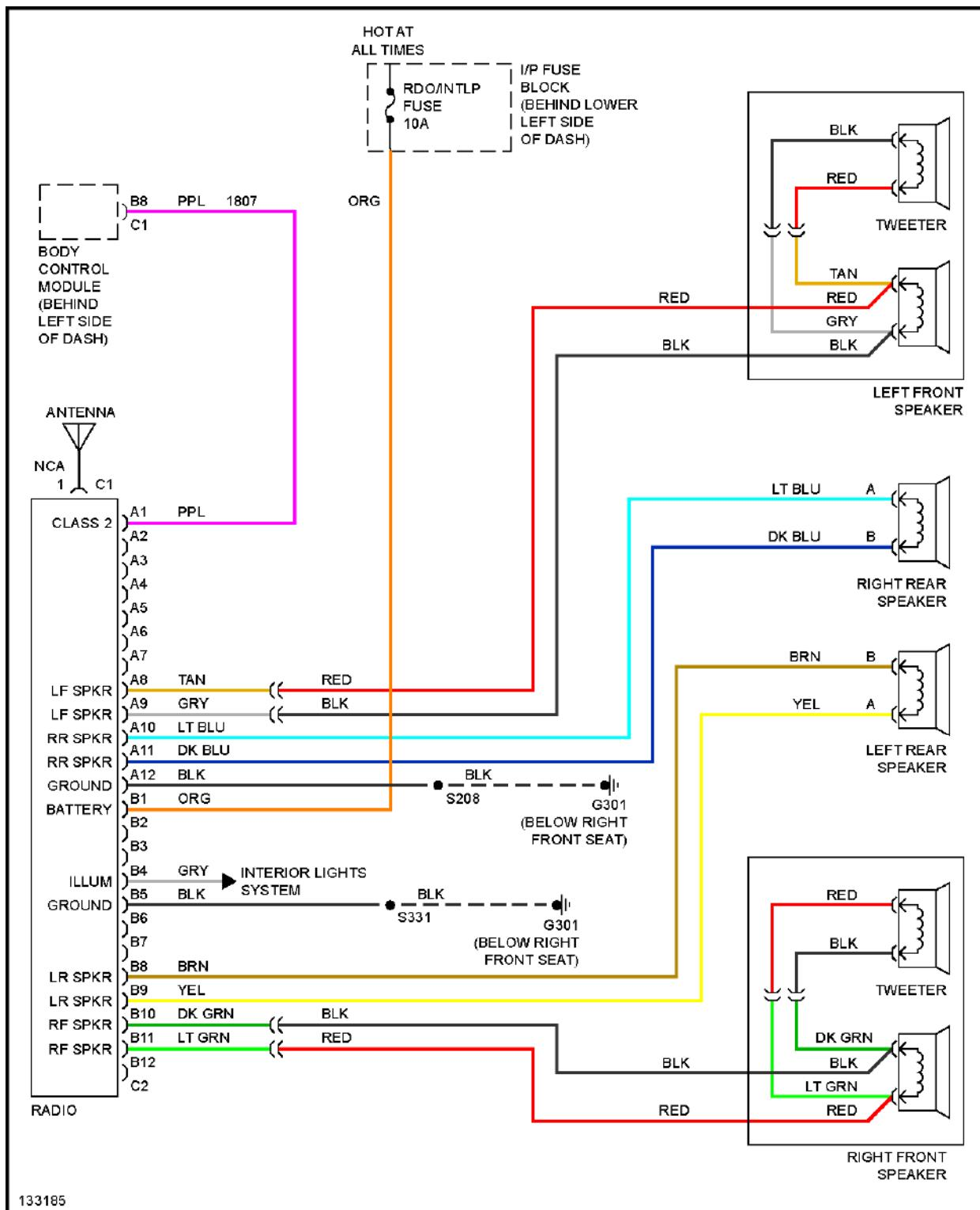
**Fig. 38: Radio Circuits, W/O Amplifier**
