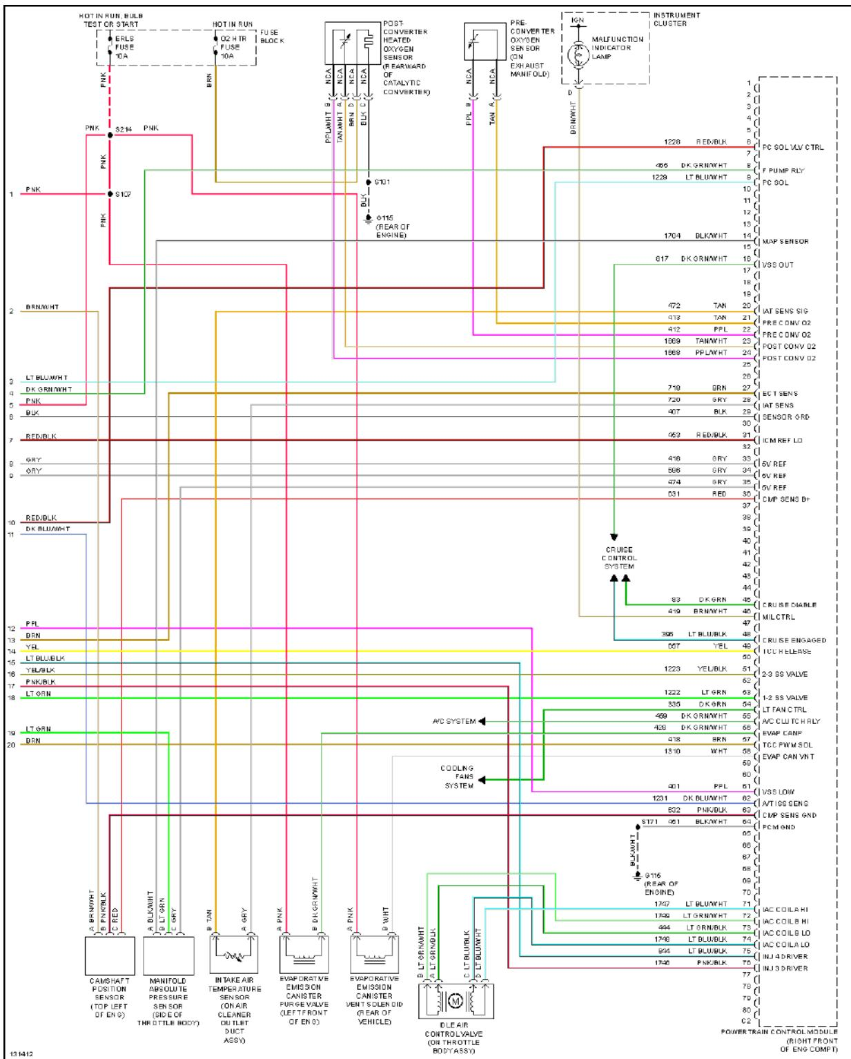
**Fig. 16: 2.4L VIN T, Engine Performance Circuits (3 of 3)**
