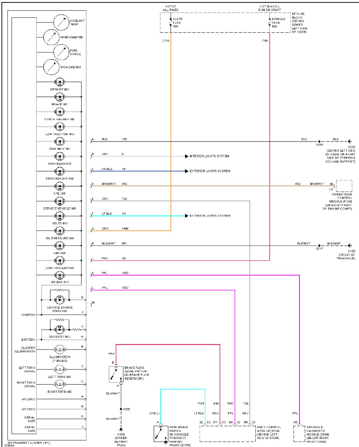
**Fig. 24: Instrument Cluster Circuit**
