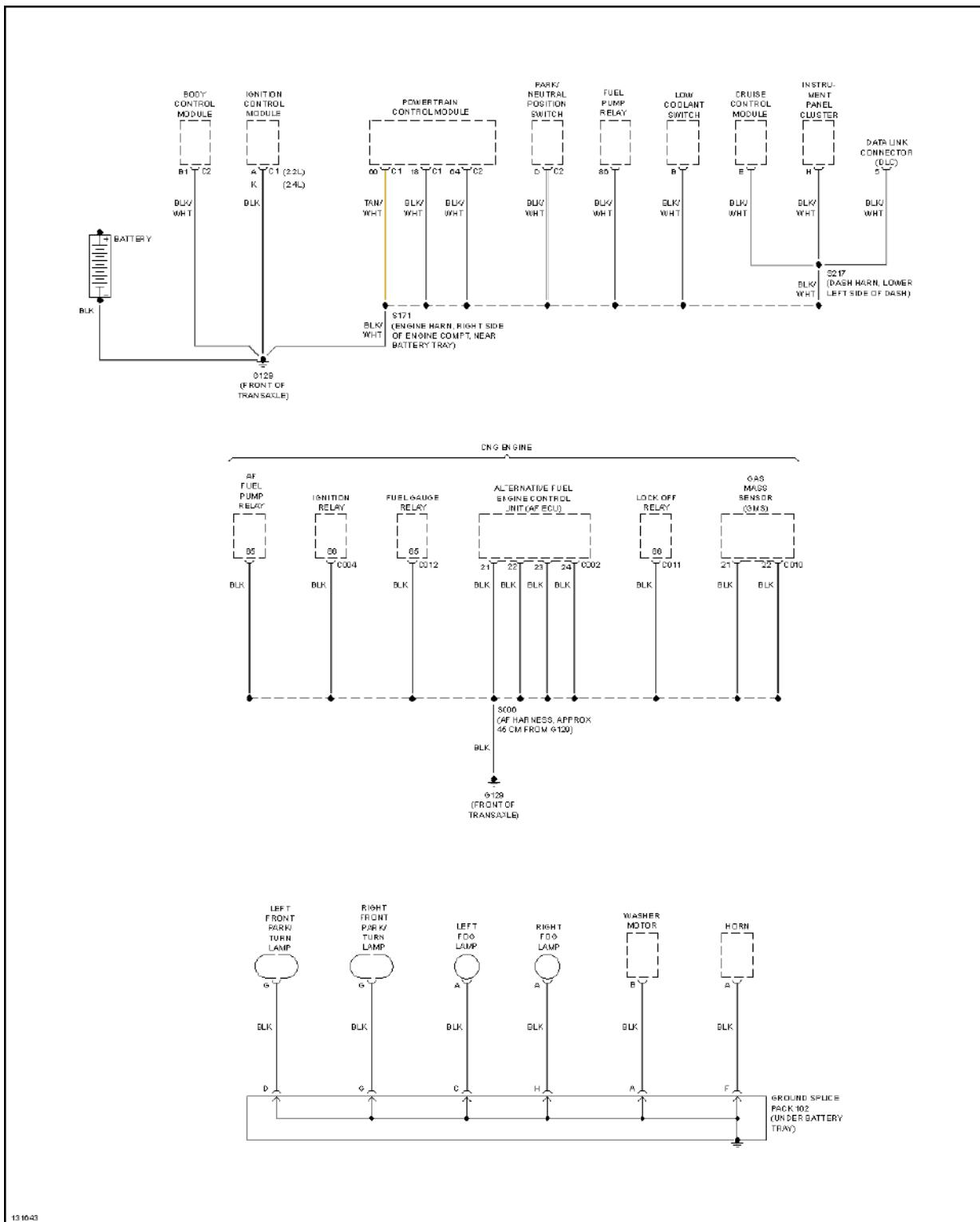
**Fig. 19: Ground Distribution Circuit (1 of 3)**
