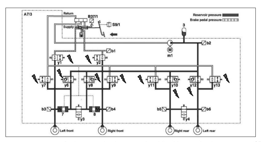
• Outlet control valves y7, y9, y11, y13 energized
