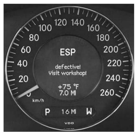
Complete ESP control module failure - Instrument cluster will scroll through failure displays
