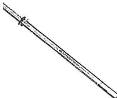
30.2 Checking the stop washer position on the oil pump driveshaft
