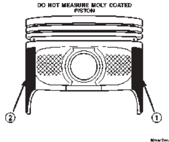
Fig. 18 Moly Coated Piston
