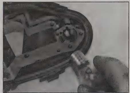
5.21 Push and twist out the bayonet bulb
