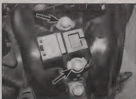
12.59b ... undo the retaining bolts and remove the sensor
