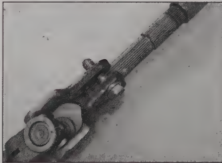
15.16 Remove the retaining bolt to remove the joint from the column
