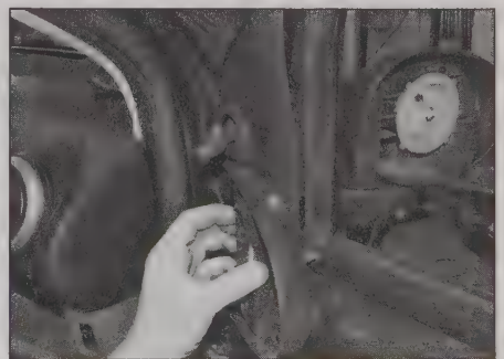
18.2b ... and remove the trim panel from inside the door frame
