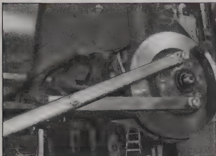
2.5 Using a home-made holding tool to prevent the front hub from turning
