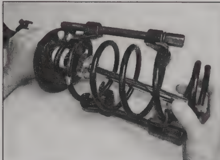
4.13 Remove the compressed spring from the strut
