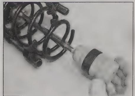
4.12b ... and the rubber bump stop
