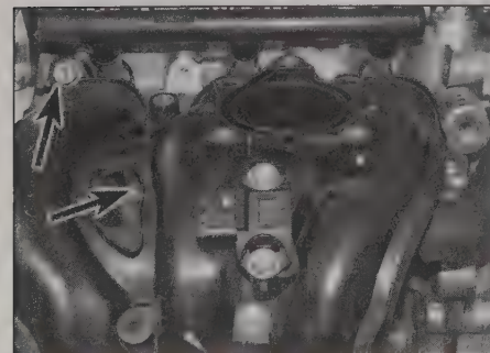
13.9b . . . left-hand side mounting bolts . . .
