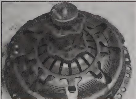
4.17a Centralise the clutch plate . . .
