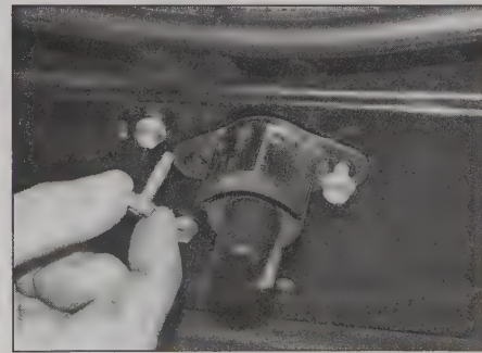
15.6a Undo the lock button retaining bolts ...
