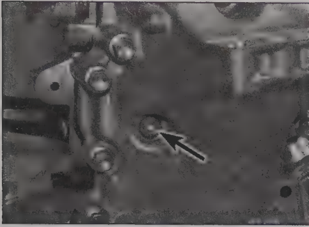
7.2 Access plug for timing chain tensioner
