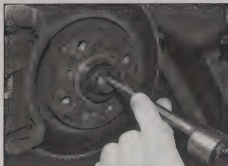
2.2 Tap up the deformed portion of the nut so it can be unscrewed
