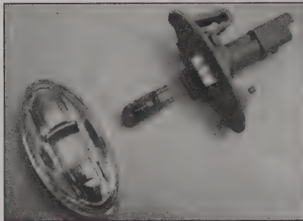
5.15a The side repeater can be split in two to renew the wedge-base bulb
