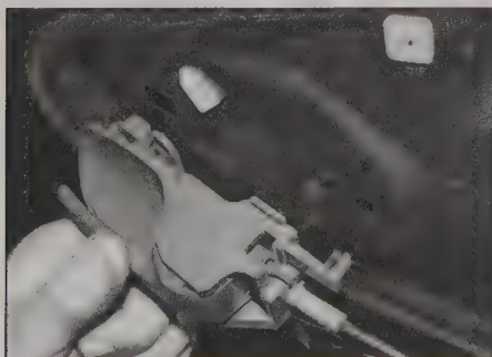
12.2 Unclip the door lock handle from the door panel
