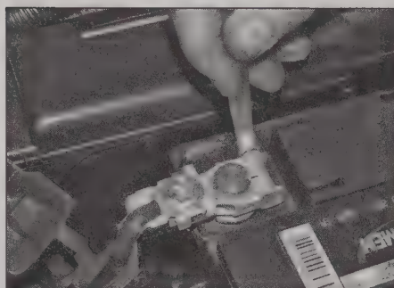
4.3b ... loosen the clamp nut and disconnect the positive lead
