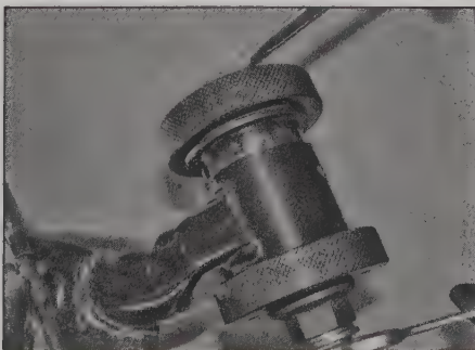
13.9 Using a threaded rod and spacers to press the bearing into the axle
