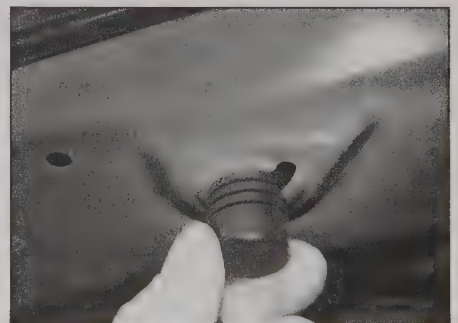
7.9 Adjust bump stop for bonnet closure height
