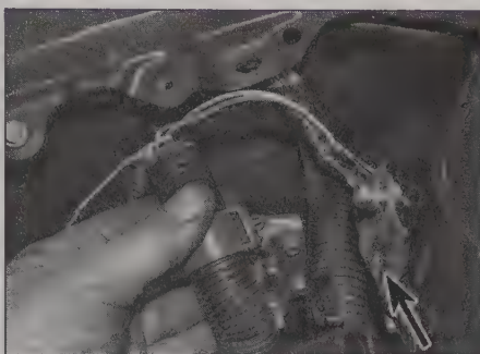
4.10b ... and unclip the wiring loom from the bracket (arrowed)
