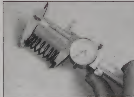
7.19 Checking the valve spring free length
