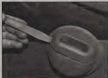
4.31a Unclip the switch trim from the door panel ...
