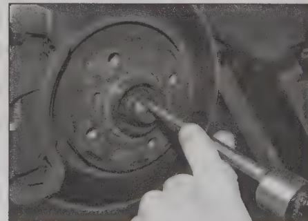
2.2 Tap up the deformed portion of the nut so it can be unscrewed
