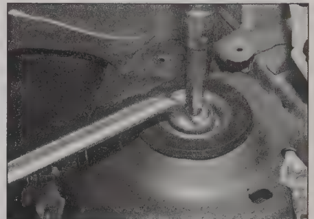
4.25 Hold the piston rod with an Allen key and tighten the retaining nut
