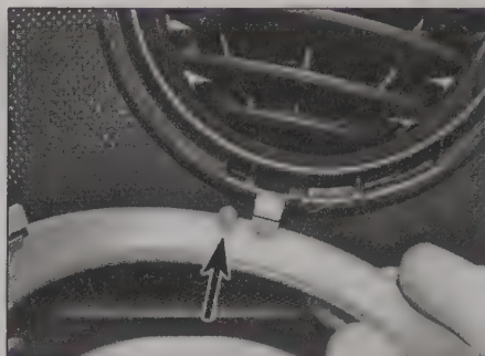
9.58b . . . noting its locating peg for refitting
