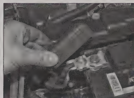
4.3a Unclip the red plastic cover ...
