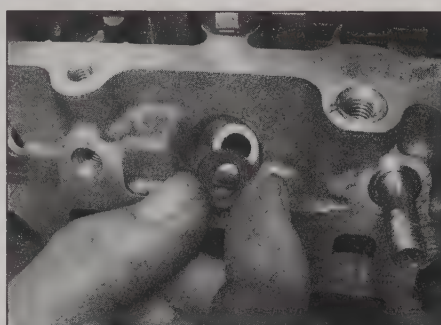
12.32a Fit new seals/dampers to the cylinder head ...
