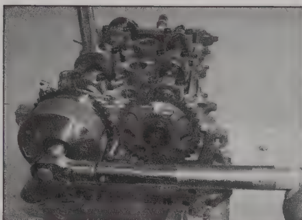
5.33 Holding the inlet camshaft using the hex casting
