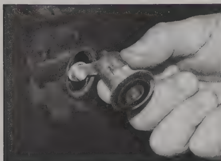
12.14b ... and withdraw the lock barrel from the door
