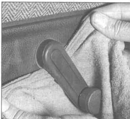
10.3a Work a cloth up behind the regulator handle and move it back-and-forth ...
