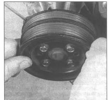
7.5 If there's play in the shaft, replace the water pump
