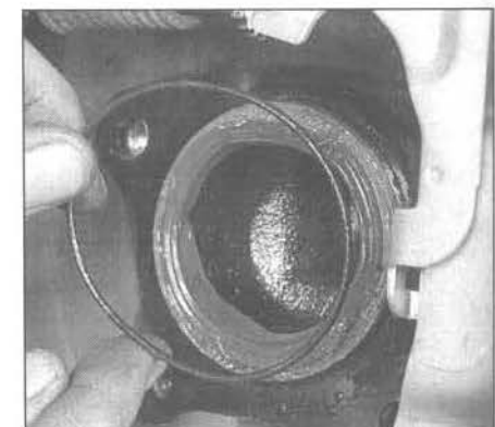
13.5 Be sure to replace this O-ring on the hub seat
