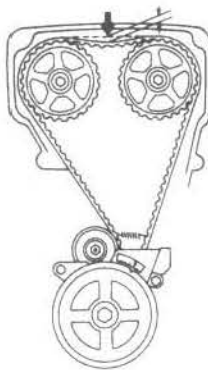
7.35b On 4A-GE engines, check the timing belt deflection at the top (arrow)
