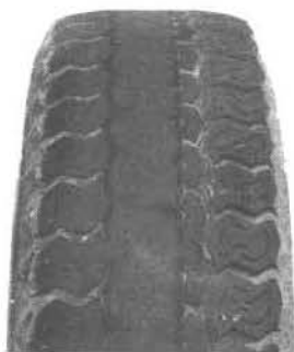
INCORRECT TOE-IN OR EXTREME CAMBER
