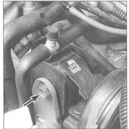
19.8a Remove the through-bolt (arrow)
