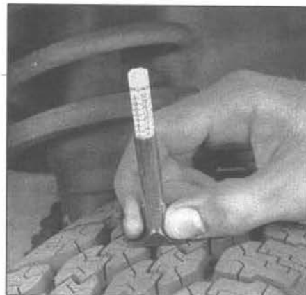
5.2 A tire tread depth indicator should be used to monitor tire wear - they're available at auto parts stores and service stations and cost very little
