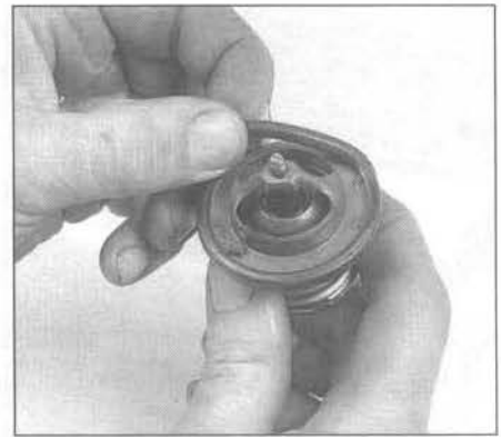
3.13 The thermostat gasket fits over the edge of the thermostat
