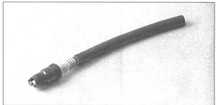
25.10 A length of 3/16-inch ID rubber hose will save time and prevent damaged threads when installing the spark plugs
