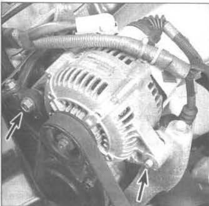
16.3 To remove the alternator, loosen the adjustment bolts shown on other side of adjustment bracket in the previous illustration, then remove the adjustment bolt and pivot bolt (arrows) shown here
