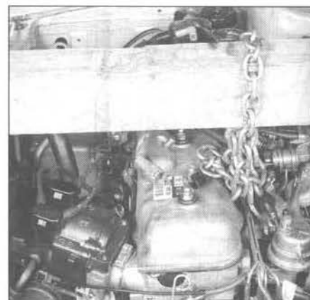
9.11 If you don't have a regular engine hoist, lay a 4 x 4 post across the engine compartment like this and support the engine with a heavy chain
