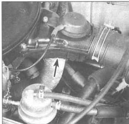
28.3 The air control valve is located in the air cleaner housing snorkel (arrow)
