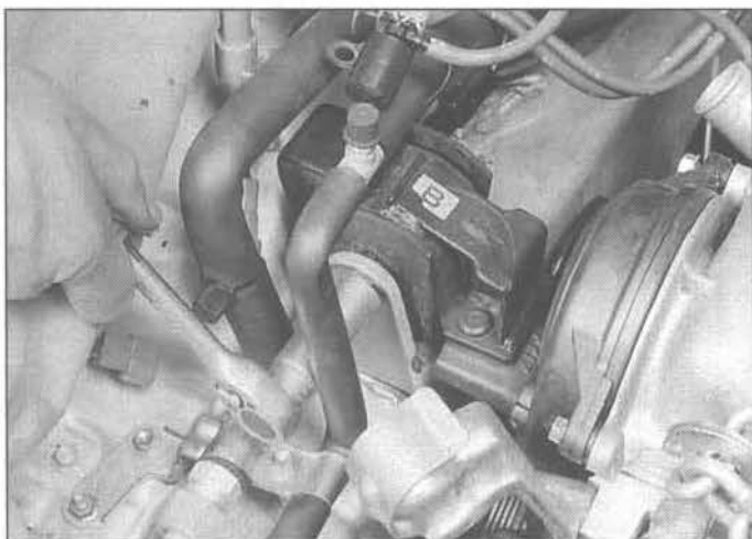
5.18 Remove the through-bolt from the engine mount
