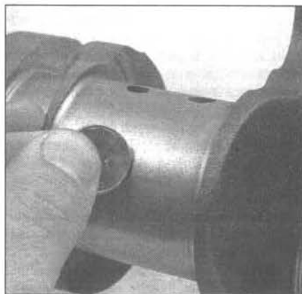
18.4 Rubbing a penny lengthwise on each journal will give you a quick idea of its condition - if copper rubs off the penny and adheres to the crankshaft, the journals should be reground
