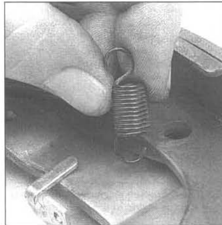
5.4q Install the adjuster lever spring
