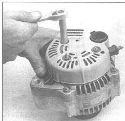
17.2a Remove the three nuts from the rear cover
