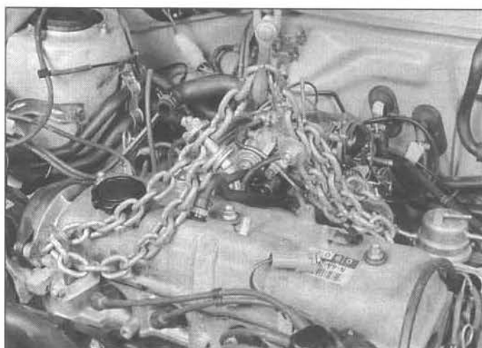
5.16 Attach a sling to the lifting brackets on the engine
