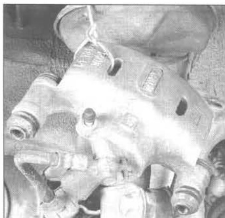
2.6c Once the caliper is removed from the torque plate, hang it from the coil spring with a piece of wire - DON'T let it hang by the brake hose!
