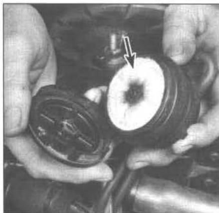
8.24 Remove the HAC cover, peel the filter out, clean it with compressed air, inspect it and, if necessary, replace it
