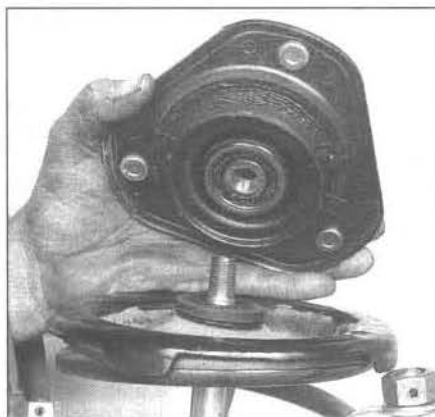
4.6 Lift the suspension support off the damper shaft
