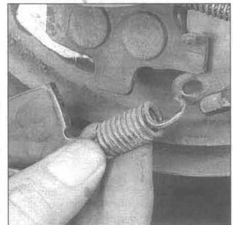
5.4u Connect the anchor spring to the bottom of each shoe and mount the front shoe to the backing plate - install the hold-down spring into the hole in the front shoe
