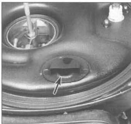
8.21a With the engine running, listen for a burbling noise from the air suction valve inlet (arrow)
