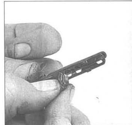
9.6b . . . then pull the element tab out of the hold (note the relationship to the frame) and slide the element out of the frame
