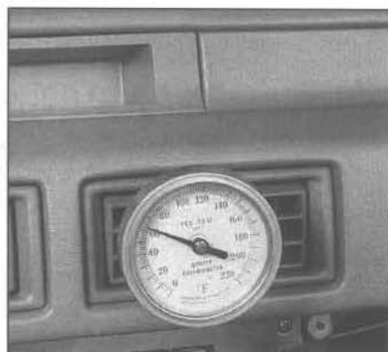
14.11 Place the thermometer in the dash vent
