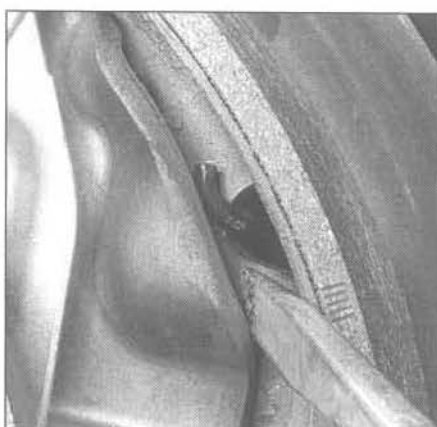
5.4w Pry the parking brake lever forward and check to see that the return spring didn't come unhooked from the rear shoe
