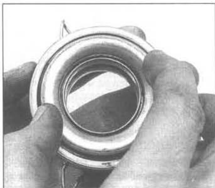
4.4 To check the bearing, hold it by the outer cage (hub) rotate the inner race while applying pressure - the bearing should turn smoothly - if it doesn't, replace it
