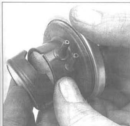
6.8a To remove the EGR vacuum modulator filters for cleaning, remove this cap ...
