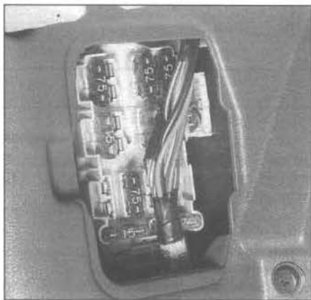
3.1a This fuse block is located in the left kick panel
