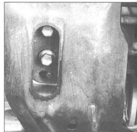
9.24c ... remove the rear mount bolts ...
