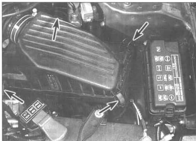
17.3 On fuel-injected models, the air cleaner cover may be secured by screws or clips (arrows)
