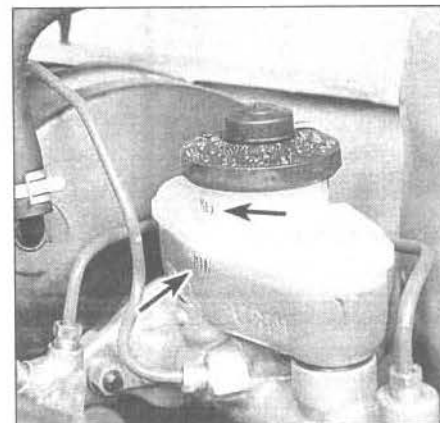
4.19a The brake fluid level should be kept between the Max and Min marks (arrows) - pry the cap off to add fluid
