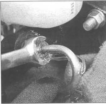
7.27 Have an assistant depress the brake pedal and hold it down, then loosen the fitting nut, allowing the air and fluid to escape - repeat this procedure on both fittings until the fluid is free of bubbles
