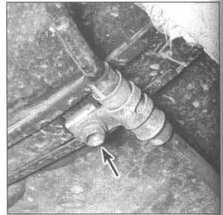
6.7 Remove the bracket bolt (arrow) and detach the parking brake cable from the fuel tank strap
