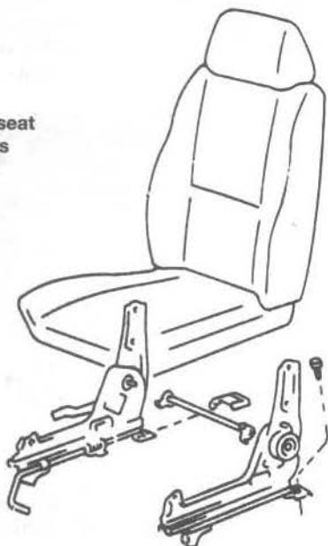
17.2a Squeeze expansion-type retaining clips with needle-nose pliers to remove them from their brackets
