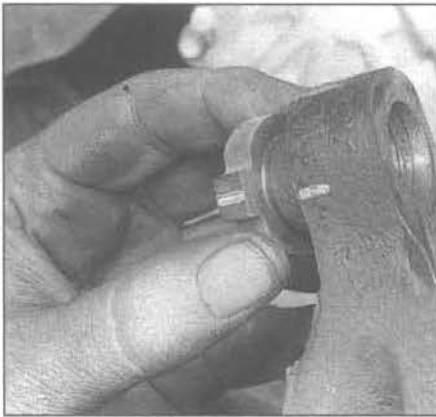
3.13 The camber adjuster (1984 through 1987 models only) slides into the upper hole in the steering knuckle - don't forget to install it
