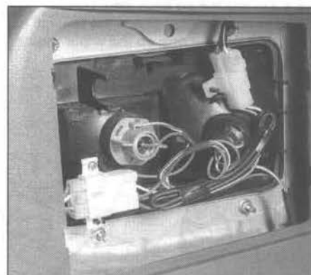
14.7a To replace a rear light on early models, open the small access door, turn the locking bulb holder counterclockwise, pull it out and pull the bulb straight out of the holder
