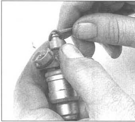
11.30a Even if you plan to reinstall the same injector(s), be sure to remove and discard the old O-rings and replace them with new ones
