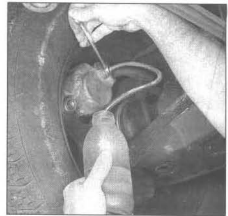
9.8 When bleeding the brakes, a piece of clear tubing is connected to the bleeder valve at the caliper or wheel cylinder and then submerged in brake fluid - air will be seen as bubbles in the tubing and container (all air must be expelled before moving to the next wheel)
