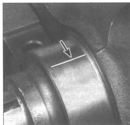
22.10 Lay the Plastigage strips (arrow) on the main bearing journals parallel to the crankshaft centerline
