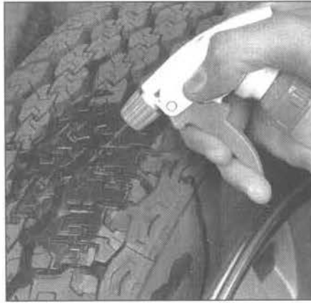
5.4b If the valve core is tight, raise the corner of the vehicle with the low tire and spray a soapy water solution onto the tread as the tire is turned slowly - leaks will cause bubbles to appear
