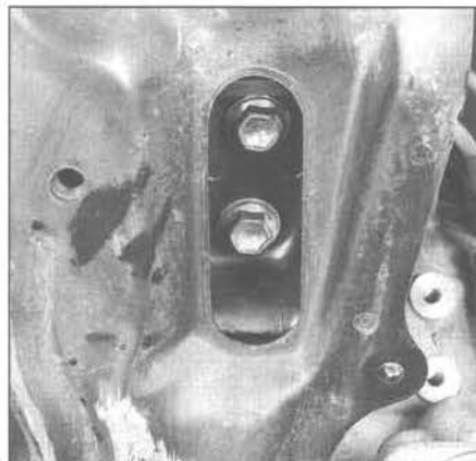
9.244b ... remove the front mount bolts ...
