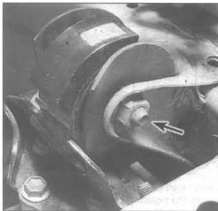
9.7 Remove the through-bolt (arrow) from the upper transaxle mount
