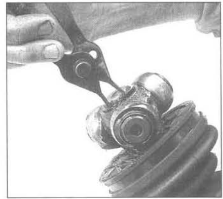
11.6b Use snap-ring pliers to remove the snap-ring that retains the inner joint tripod
