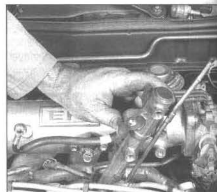
11.28 Carefully remove the fuel rail assembly through the space between the valve covers and the air intake chamber
