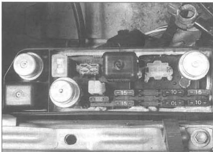
3.1b The engine compartment fuse block is located next to the battery, under a cover
