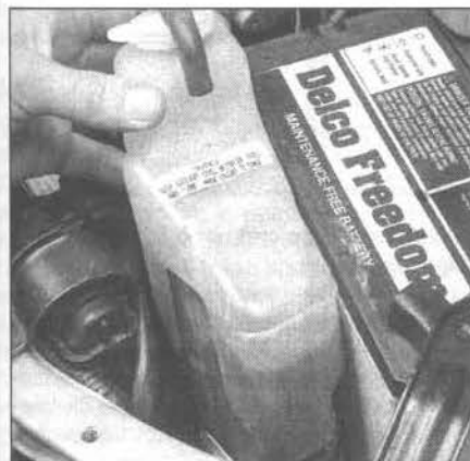
6.3 The reservoir is slipped onto a bracket - pull straight up to remove it
