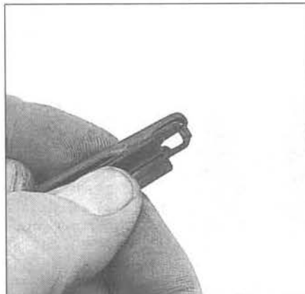
9.6a To remove the old wiper blade element, pull the top end of the element down until you can see the replacement hole in the frame . . .
