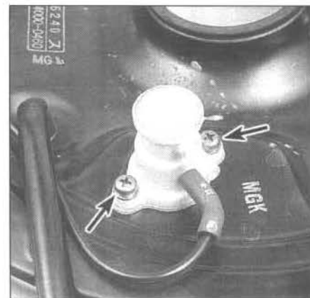
8.28 Label and detach the vacuum hoses from the HIC valve, then remove the mounting screws (arrows)
