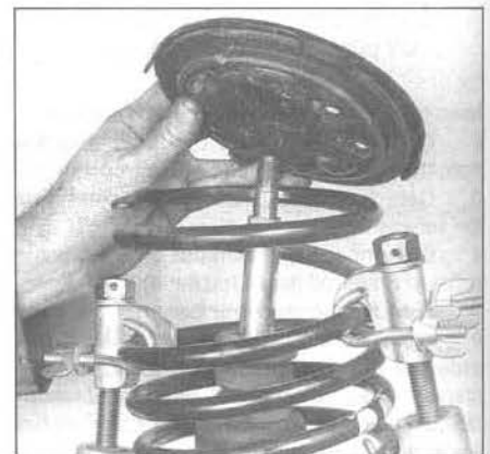
4.7 Remove the spring seat from the damper shaft
