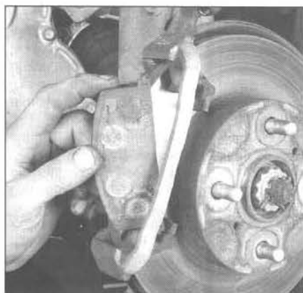
2.6f To remove the pads, slide them to the side, then straight out of the torque plate
