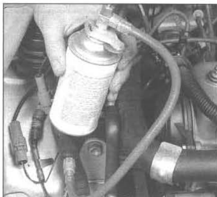
14.9 Connect the charging kit to the low pressure port - easily identified because the tubing is larger in diameter than the high pressure side
