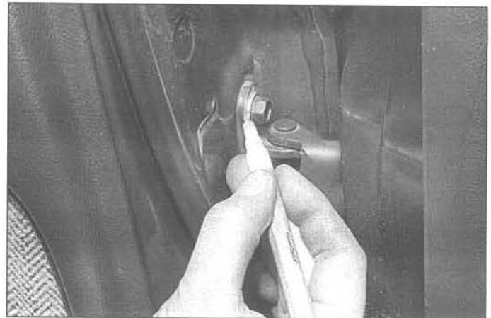
12.3 Before loosening or removing them, mark the door bolt locations
