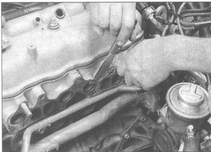
5.8 Be very careful when scraping the gasket mounting surfaces - the aluminum gouges very easily
