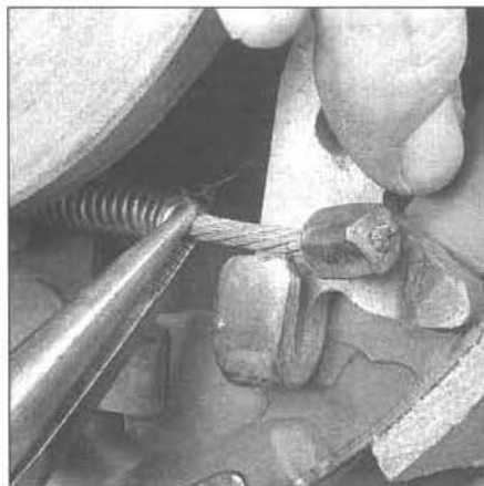
5.4s Pull the parking brake cable spring back and hold it there with a pair of pliers, then place the cable in the hooked end of the parking brake lever
