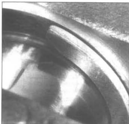
22.19a Rotate the thrust bearing into position on the number three crankshaft journal with the oil grooves facing OUT (against the crank throw)
