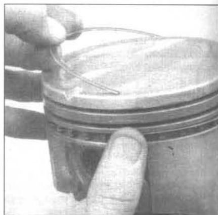
21.9b DO NOT use a piston ring installation tool when installing the oil ring side rails
