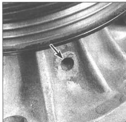
7.4 If coolant is leaking from the weep hole (arrow) the water pump must be replaced
