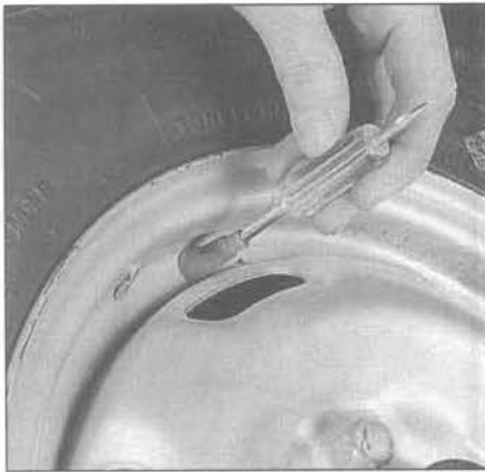
5.4a If a tire loses air on a steady basis, check the valve core first to make sure it's snug (special inexpensive wrenches are commonly available at auto parts stores and service stations)
