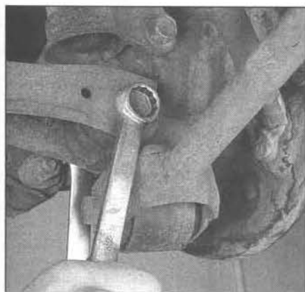
11.2 Remove the control arm-to-spindle bolt - use a back-up wrench on the nut
