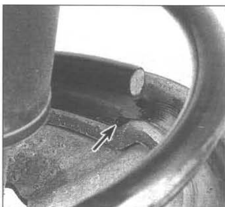
4.13 When installing the spring, make sure the end fits into the recessed portion of the lower seat (arrow)
