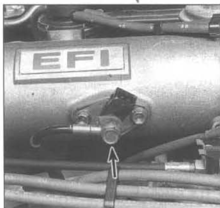
11.23 Unplug the electrical connector, remove the banjo bolt (arrow) and sealing washers, then separate the line from the cold start injector (4A-GE engine shown, 4A-FE engine similar)
