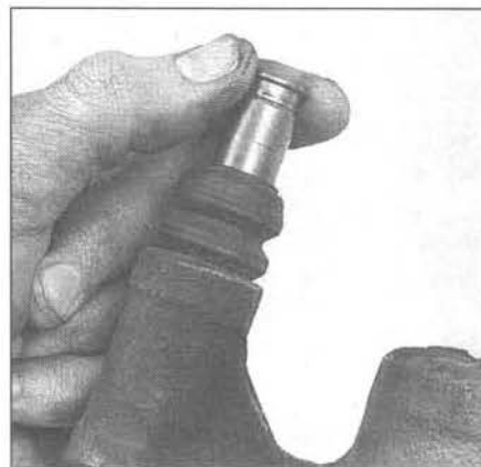
3.8a Push the sliding bushing on each side of the caliper up through the boot and pull it free, then remove the dust boots
