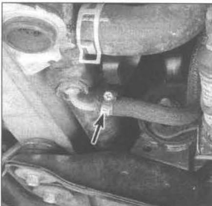
5.7 On automatic transaxle models, disconnect the cooler lines (arrow) from the bottom of the radiator (viewed from below)
