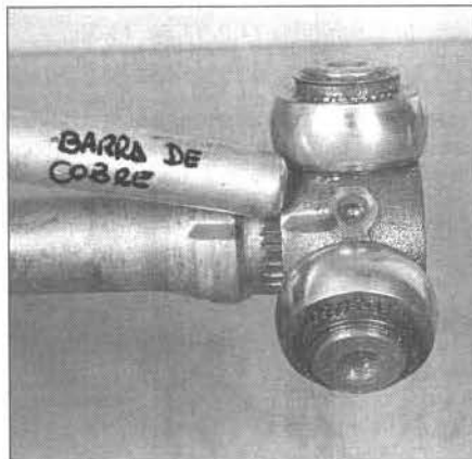
11.8 Drive the tripod joint from the driveaxle with a brass drift punch and hammer - be careful not to damage the bearing surfaces or the splints on the shaft
