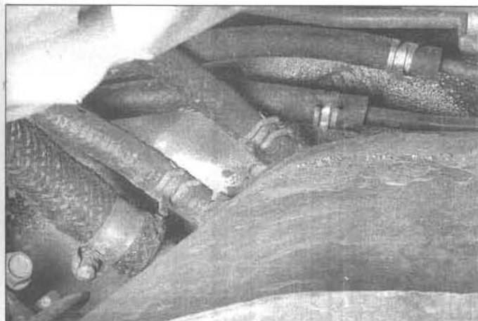
6.8b Label and disconnect the fuel lines
