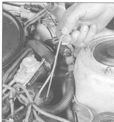
4.2 The engine oil dipstick is at the drivebelt end of the engine
