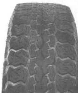
FEATHERING DUE TO MISALIGNMENT
