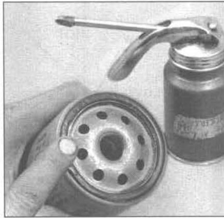
8.18 Lubricate the gasket with clean oil before installing the filter on the engine
