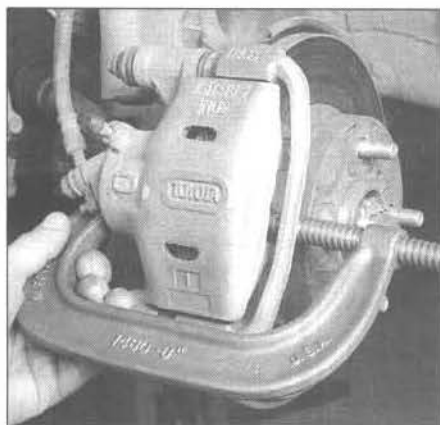
2.5 On front calipers only, use a large C-clamp to push the piston back into the caliper bore - note that one end of the clamp is on the flat area near the brake hose fitting and the other end (screw end) is pressing against the outer brake pad
