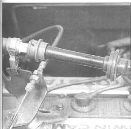
6.1 To use a calibrated ignition tester (available at most auto parts stores), simply disconnect a spark plug wire, attach the wire tester and clip the tester to a good ground - if there is enough power to fire the plug, sparks will be clearly visible between the electrode tip and the tester body as the engine is turned over
