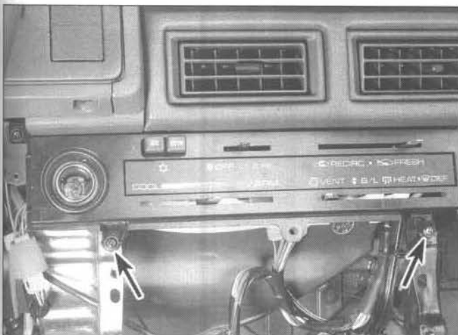
13.4 Remove the mounting screws (arrows)
