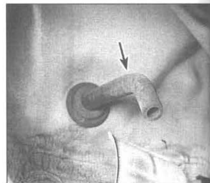
14.1 The evaporator housing drain tube (arrow) is located on the lower portion of the firewall in the engine compartment - insert a thin wire to check for blockage
