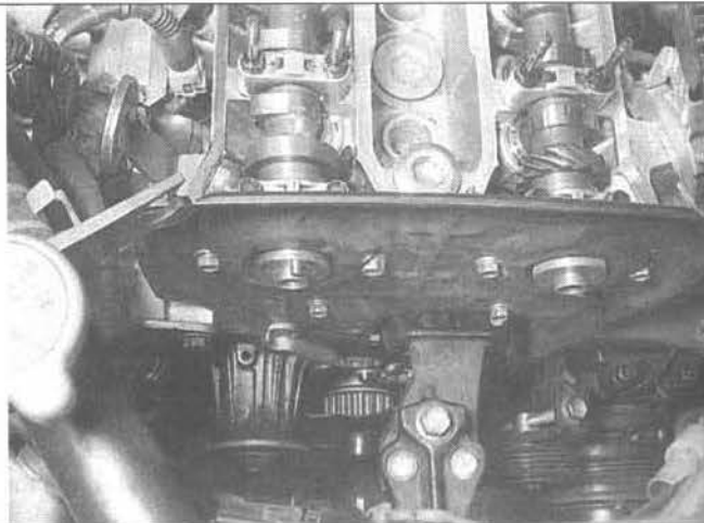
7.16c On 4A-GE engines, the knock pins (arrows) on the camshafts should be positioned as shown, with the pin on the intake camshaft at 12 o'clock and the pin on the exhaust camshaft at 5 o'clock
