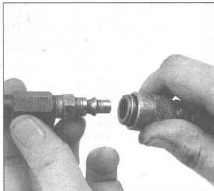
12.4 This is what the air hose adapter that threads into the spark plug hole looks like - they're commonly available from auto parts stores
