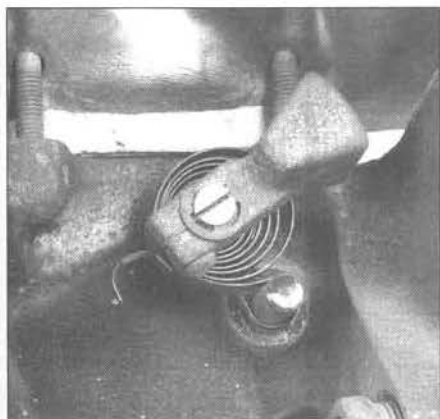
8.34 When the engine is cold, make sure the weight on the valve is in the upper position - when the engine is hot, make sure the weight is in the lower position
