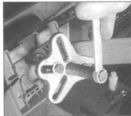
16.4 Use a steering wheel puller to separate the steering wheel from the column - DON'T attempt to remove the wheel with a hammer!
