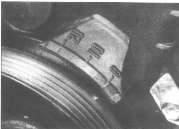
9.4 Typical 4A-C engine ignition timing marks
