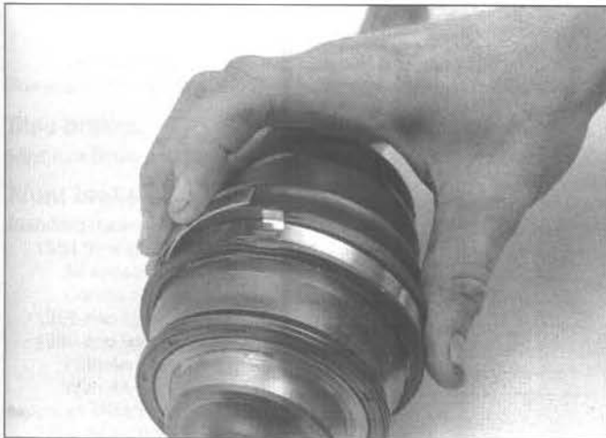
11.15c To install the new clamps, bend the tang down. . .
