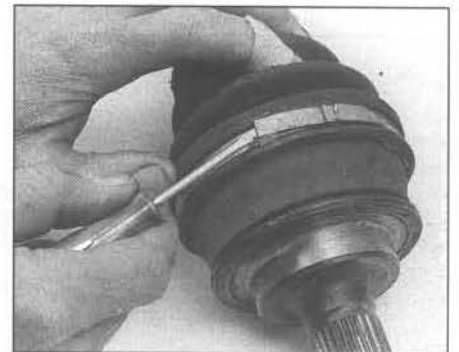
11.3a On Toyota type driveaxles, the large boot clamps can be pried open with a small screwdriver
