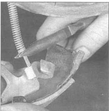
5.4j Pull back the spring on the parking brake cable and detach the cable from the lever
