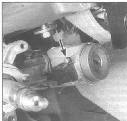
9.5 Remove the screw for the warning buzzer switch (arrow), then detach the switch
