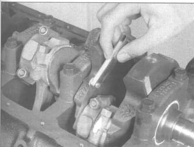
12.3 Check the connecting rod side clearance with a feeler gauge as shown here
