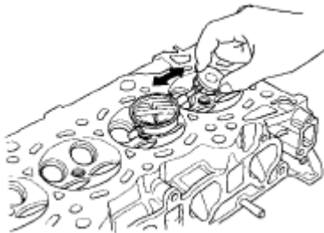
Fig. 250: Checking Intake Valve Stem-To-Guide Clearance Courtesy of AMERICAN HONDA MOTOR CO., INC.
