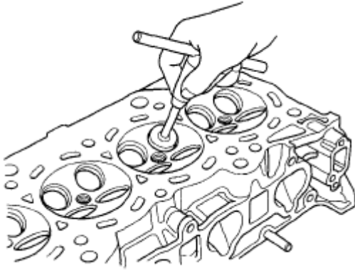
Fig. 256: Cutting Valve Seats Using Valve Seat Cutter Courtesy of AMERICAN HONDA MOTOR CO., INC.
