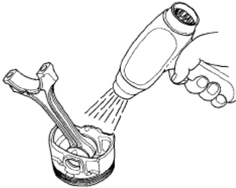
Fig. 111: Heating Piston And Connecting Rod Assembly Courtesy of AMERICAN HONDA MOTOR CO., INC.
