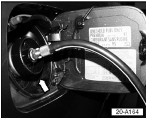
Fig. 291: Checking Leak Detection Pump -V144- For Internal Leaks Courtesy of VOLKSWAGEN UNITED STATES, INC.
