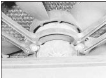
6.1b Radiator cooling fan to frame mounting bolts
