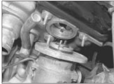
4.9b . . . and remove the distributor
