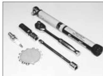
7.4 Tools required for spark plug removal, gap adjustment and refitting
