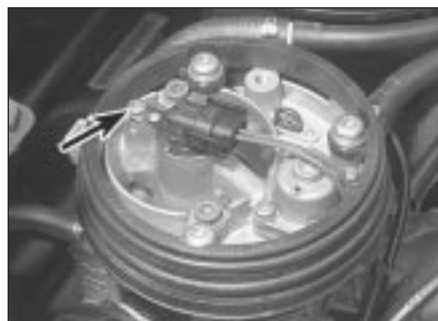
12.5 Fuel injector retaining plate securing screw (arrowed)
