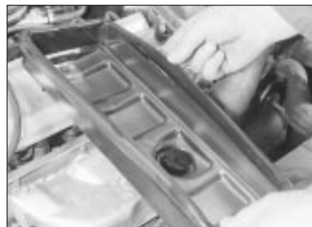
4.8 Ensure the rubber seal is correctly located on the cover when refitting
