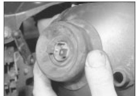
8.6 . . . remove the rubber cover . . .
