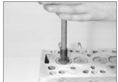
6.21 Grinding-in a valve
