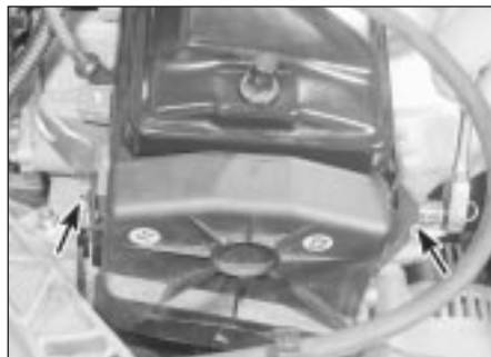
6.1a Undo the two retaining bolts (arrowed) . . .
