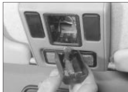
9.5 Removing the map reading light and extract the bulb
