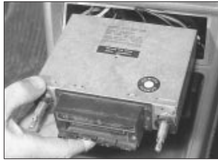
22.3 Removing the radio on early models
