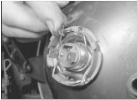
8.7a ... release the spring clips ...
