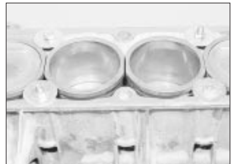
8.17 Cylinder liners clamped with washers and bolts
