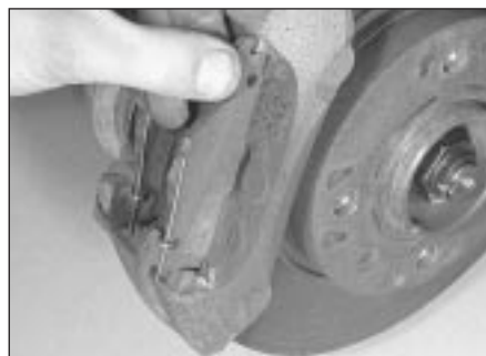
4.5 Removing the outer pad (DBA Bendix caliper)
