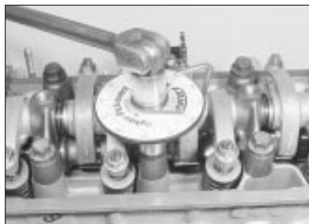
11.38 ... then with an angle tightening gauge
