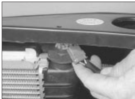
5.4b . . . and low coolant level sensor wiring
