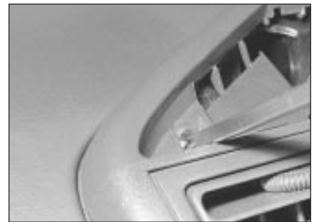
26.22a Removing the central vent assembly upper . . .
