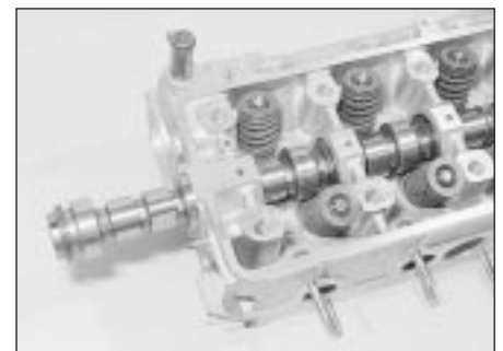
6.8 Removing the camshaft
