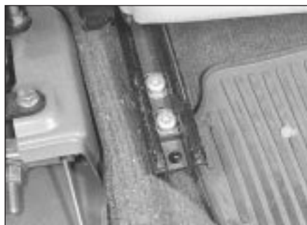
21.1 Front seat rear inner mounting bolts
