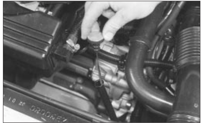
5.1 Withdrawing the automatic transmission fluid dipstick
