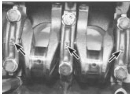
8.14 Main bearing cap identification markings (arrowed)
