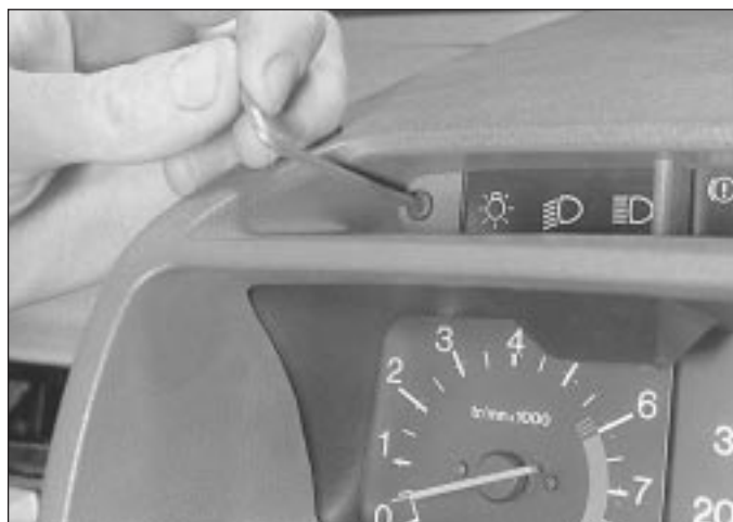
5.2 Removing the instrument panel upper ...
