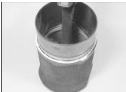
9.11 Cylinder liner with paper base seal
