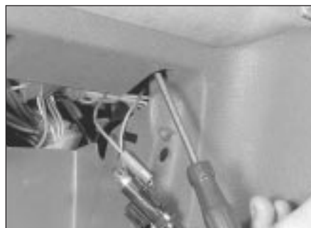
26.11 Removing a facia mounting screw
