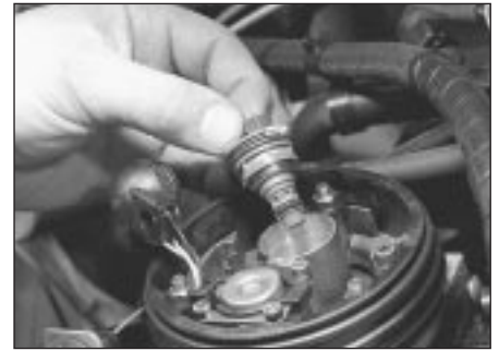
11.7 Withdrawing the fuel injector
