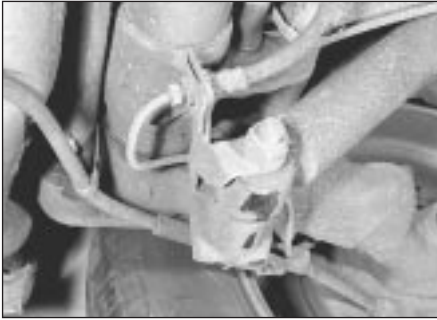
10.2 Rear shock absorber bottom mounting
