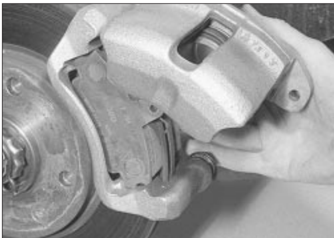
4.20a Swivel the caliper upwards . . .
