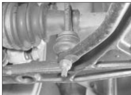
7.9 Anti-roll bar link arm bottom mounting on GTI models
