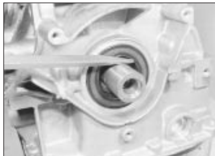
14.2 Using a screwdriver to lever out the crankshaft front oil seal
