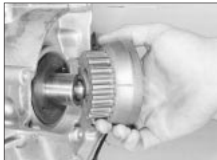
8.11b . . . then slide off the sprocket
