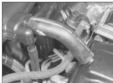
2.6a Disconnect the crankcase ventilation hose from the valve cover . . .
