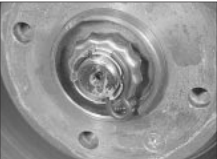
2.1 R-clip and locking collar fitted to hub nut on later models
