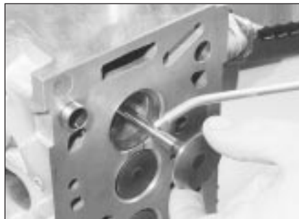
6.27 Lubricate the valve stems prior to refitting
