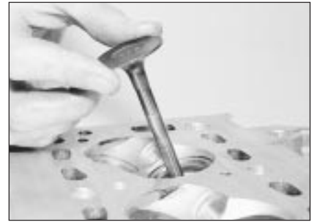
6.6 Withdraw the valve through the combustion chamber
