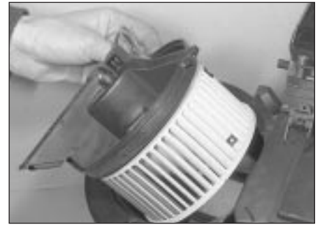
9.7 Removing the heater blower motor
