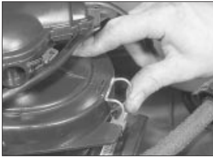
2.7a Release the spring clips . . .
