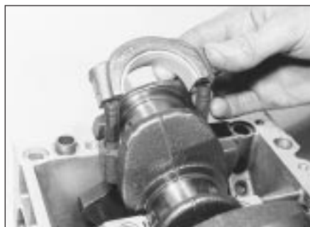
7.5 Remove the big-end bearing caps
