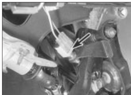
4.35 Brake stop light switch wiring connector (arrowed)
