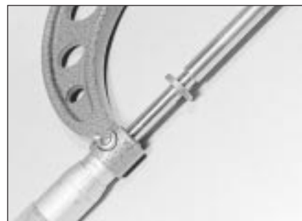
2.12b ... then measure the shim thickness with a micrometer
