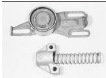
5.12 Spring loaded timing belt tensioner components
