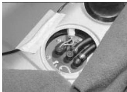
5.3 Fuel pump locations and connections
