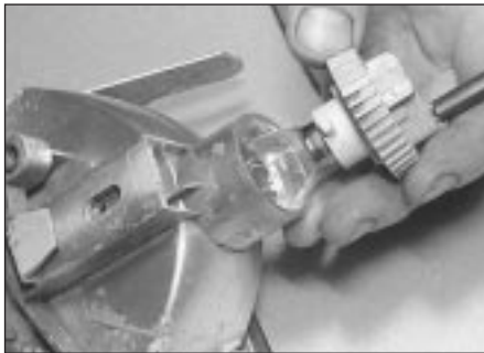
8.10 Remove the front direction indicator light bulbholder ...
