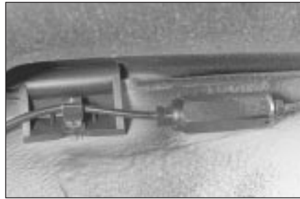
13.7 Rear brake compensator fitted to 1.9 GTI models
