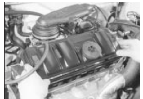
4.5 . . . and lift off the cylinder head cover
