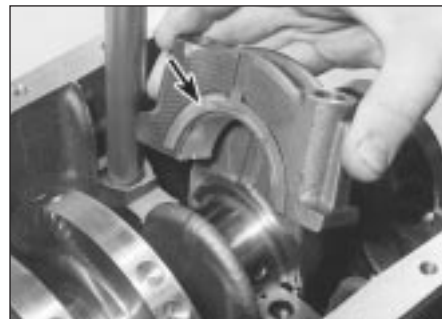
8.16 Removing the main bearing cap and thrustwashers (arrowed)
