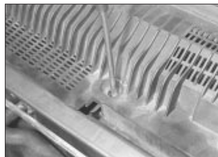
15.3 Removing the air intake grille screws
