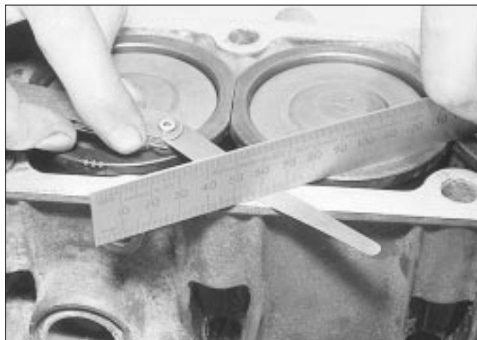
9.24 Measuring cylinder liner protrusion
