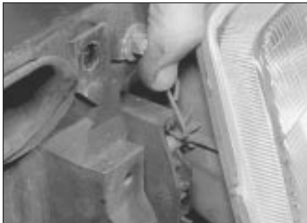
10.3 Releasing the headlight spring clips
