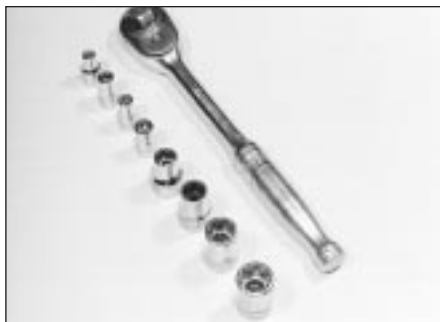
Sockets and reversible ratchet drive
