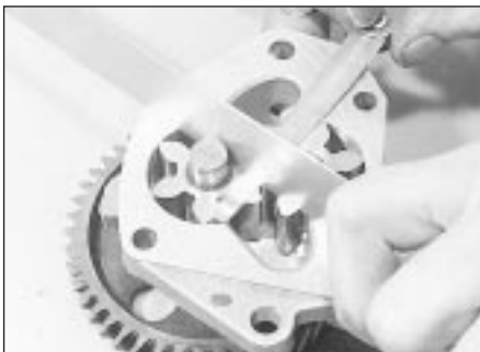
5.5 Checking oil pump gear endfloat
