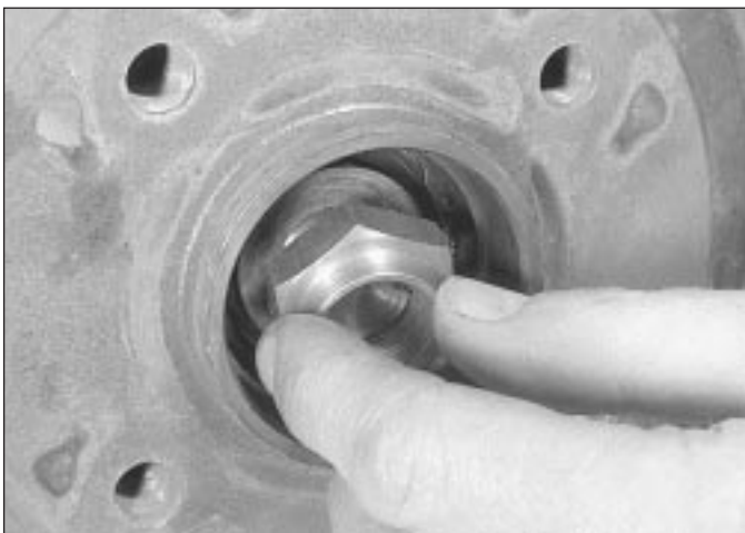
11.2a Unscrew the rear hub nut . . .
