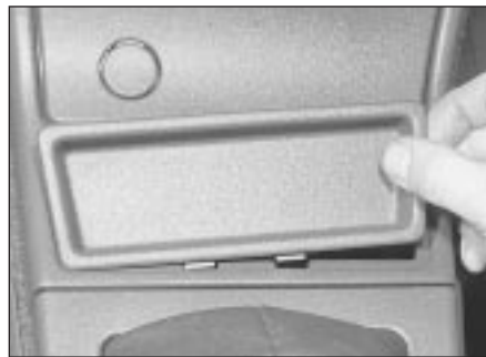
26.32 Removing the centre console tray
