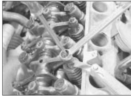
2.7 Adjusting the valve clearances
