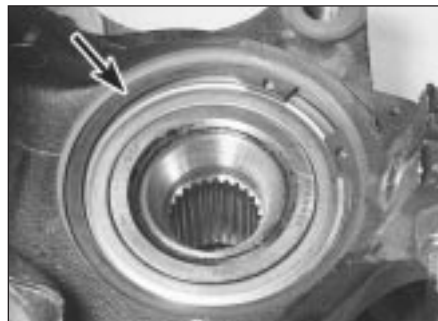
3.3 Front hub bearing retaining circlip (arrowed)
