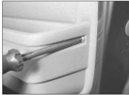
11.3 Removing the side pocket
