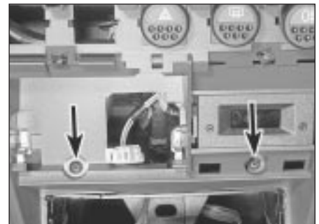
26.36 Front facia panel screws (arrowed)
