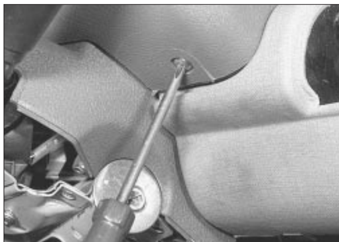
5.4 ... and lower retaining screws
