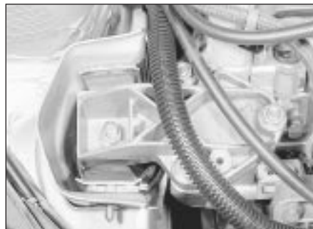
8.6 Right-hand engine mounting and cylinder head bracket
