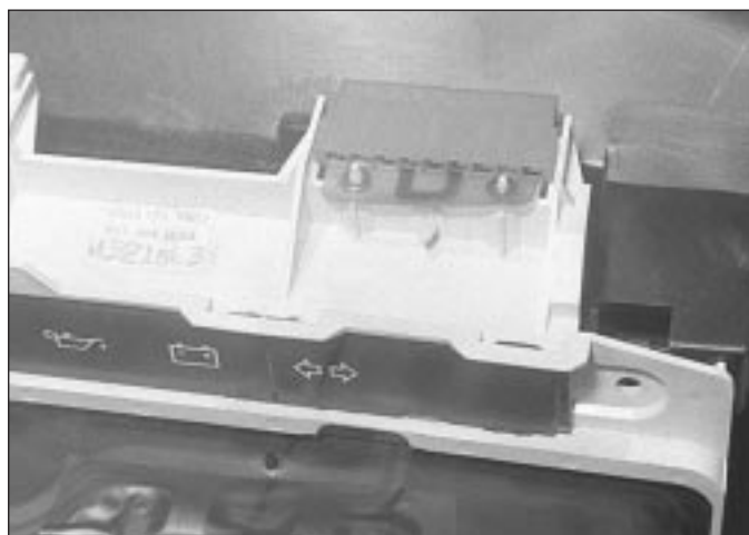
5.6b Instrument panel right-hand upper multiplug
