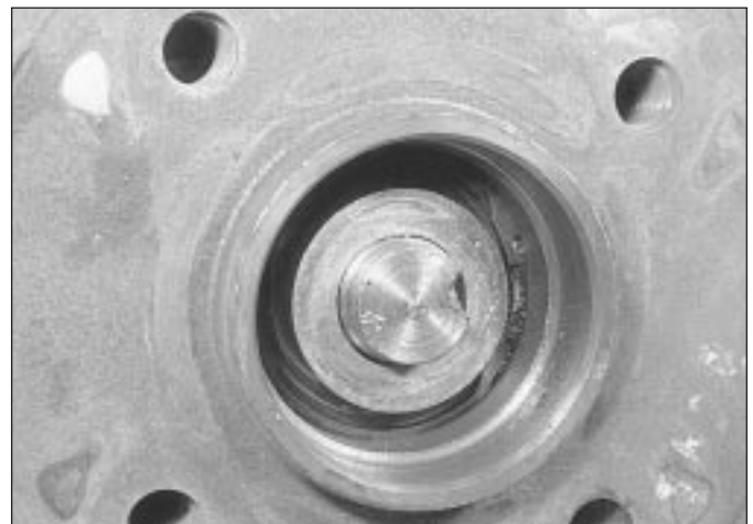
11.2b . . . and remove the washer
