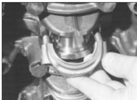
7.11 Removing a big-end bearing cap and shell
