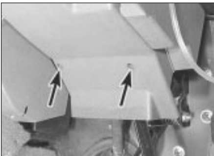
14.2 Steering column lower trim panel screws (arrowed)
