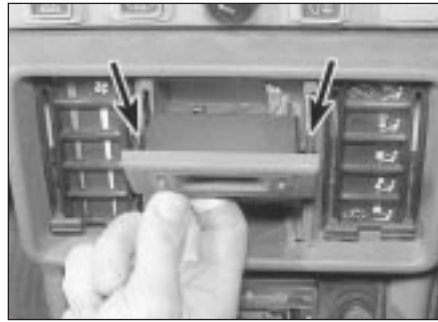
26.5 Digital clock and retaining barbs (arrowed)
