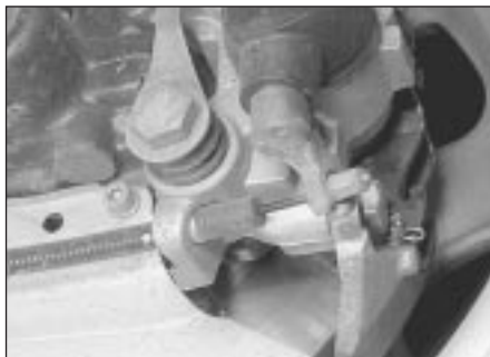
8.4 Handbrake cable attachment at rear brake caliper
