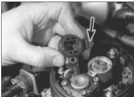
11.13 Intake air temperature sensor (arrowed)
