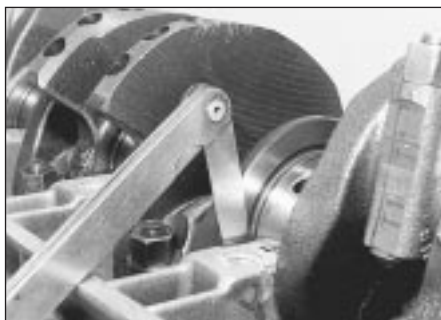
8.7 Checking crankshaft endfloat using feeler blades
