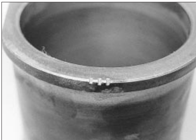
9.18 Cylinder liner size group marking
