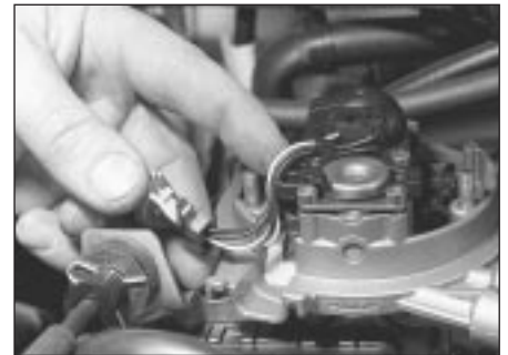
11.12b . . . then release wiring from clip
