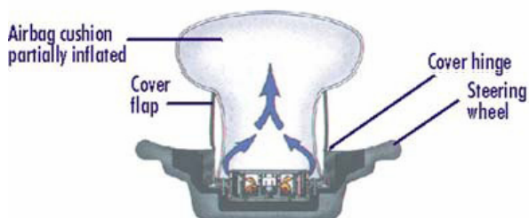
Figure E Cushion deploys and begins to fill. Time sequence: 15-25 milliseconds.
