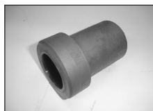
Fork oil seal fitment punch :
