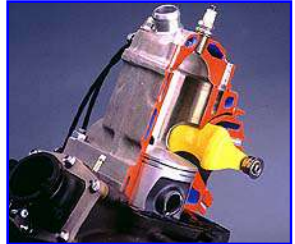
The curved yellow valve rotates on a pivot to open and close the exhaust port; it is shown in the closed position.
