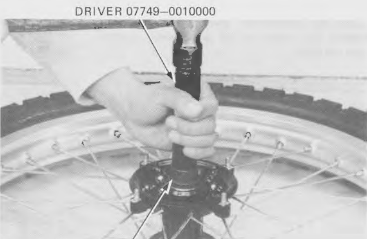
DRIVER 07749-0010000 ATTACHMENT, 32 x 35 mm 07746-0010100 PILOT, 15 mm 07746-0040300
