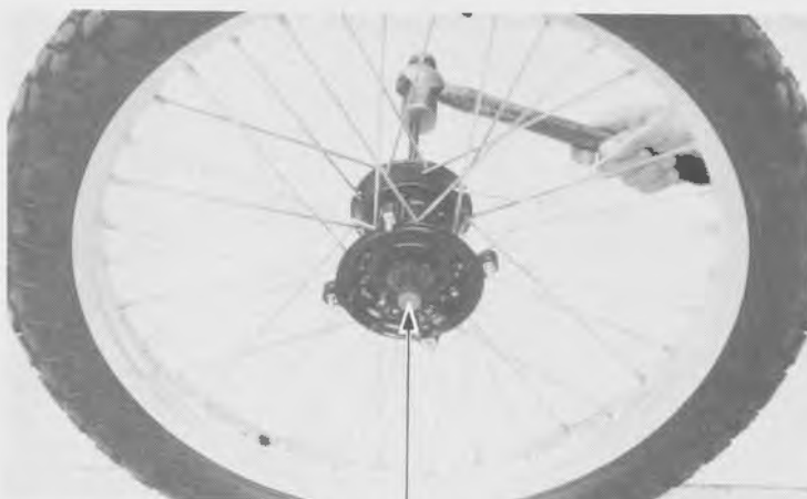
WHEEL BEARING REMOVER HEAD 15 mm 07746-0050400 WHEEL BEARING REMOVER SHAFT 07746-0050100 OR EQUIVALENT COMMERCIALLY AVAILABLE IN U.S.A.
