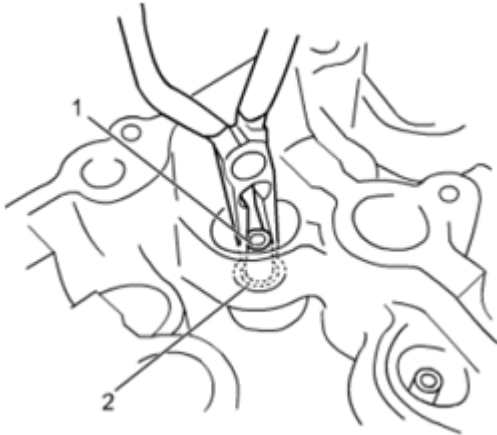
Fig. 124: Removing Valve Stem Seal Courtesy of SUZUKI OF AMERICA CORP.
