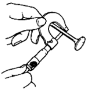
Fig. 133: Checking Valve Stem Inside Diameter Courtesy of SUZUKI OF AMERICA CORP.
