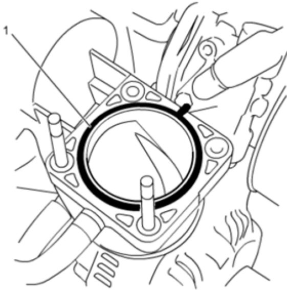
Fig. 19: Identifying Throttle Body Gasket To Intake Manifold Courtesy of SUZUKI OF AMERICA CORP.
