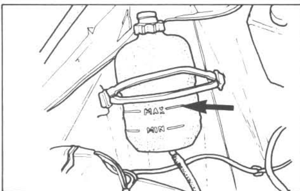
Fig. A:17 Check/top up coolant level to MAX mark
