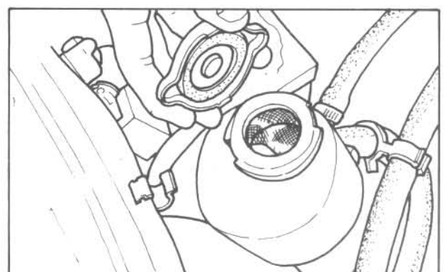
Fig. A:26 Check/top up power steering fluid level
