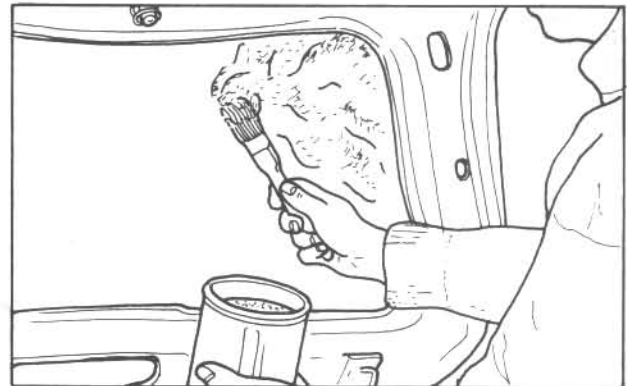
Fig. P:23 Applying adhesive to bonnet
