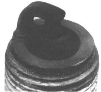
Fig. B:2 Check and adjust plug electrode gap
