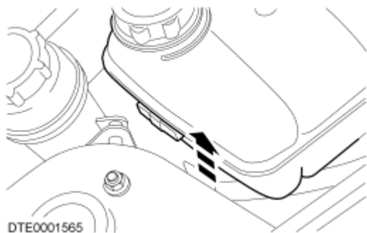
Fig. 202: Removing Coolant Expansion Tank Courtesy of FORD MOTOR CO.
