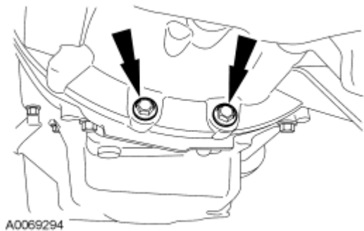
Fig. 530: Locating Lower Bellhousing Bolts Courtesy of FORD MOTOR CO.
