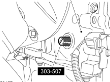
Fig. 2: Installing Crankshaft TDC Timing Peg
