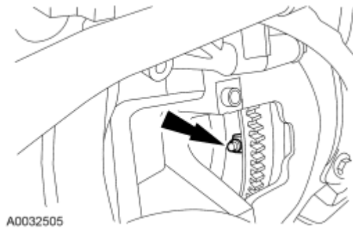
Fig. 271: Locating Torque Converter Nut Courtesy of FORD MOTOR CO.
