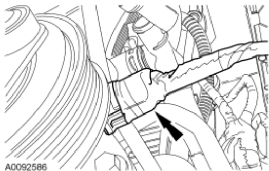
Fig. 247: Locating A/C Compressor Electrical Connector Courtesy of FORD MOTOR CO.
