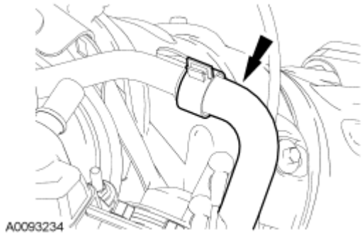
Fig. 210: Locating Secondary Air Injection (AIR) Hose Courtesy of FORD MOTOR CO.
