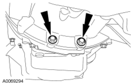
Fig. 265: Locating Lower Bellhousing Bolts Courtesy of FORD MOTOR CO.
