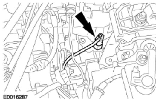
Fig. 558: Locating Reversing Lamp Switch Electrical Connector Courtesy of FORD MOTOR CO.
