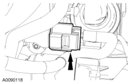
Fig. 302: Locating Manifold Absolute Pressure Sensor Electrical Connector Courtesy of FORD MOTOR CO.
