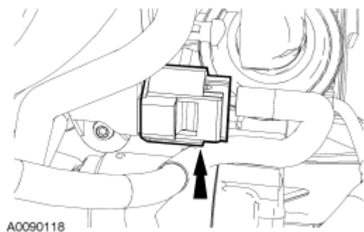
Fig. 490: Locating Manifold Absolute Pressure Sensor Electrical Connector Courtesy of FORD MOTOR CO.
