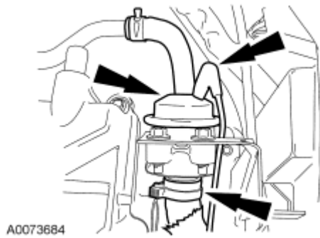
Fig. 173: Locating Secondary Air Injection Vacuum Regulator Electrical Connector And Vacuum Hose Courtesy of FORD MOTOR CO.
