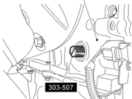
Fig. 410: Installing Crankshaft TDC Timing Peg
