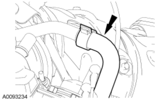
Fig. 582: Locating AIR Hose Courtesy of FORD MOTOR CO.
