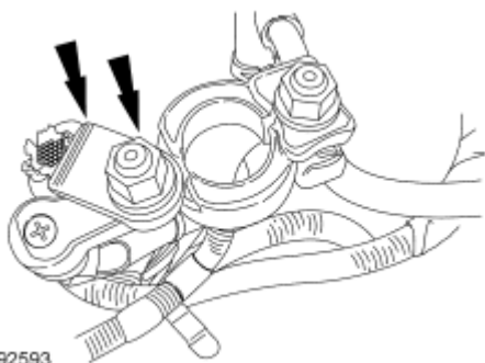
Fig. 563: Locating Power Distribution Wiring Harness Eyelet And Nut Courtesy of FORD MOTOR CO.
