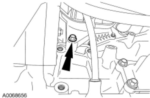
Fig. 296: Locating Lower Intake Manifold Bolt Courtesy of FORD MOTOR CO.
