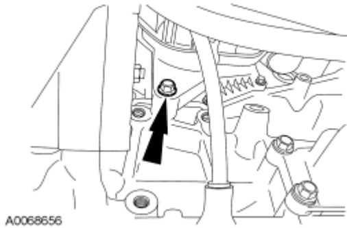
Fig. 39: Locating Lower Intake Manifold Bolt Courtesy of FORD MOTOR CO.
