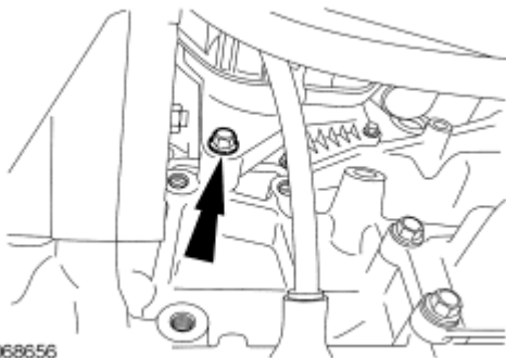
Fig. 496: Locating Lower Intake Manifold Bolt Courtesy of FORD MOTOR CO.
