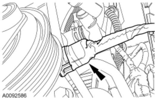
Fig. 545: Locating A/C Compressor Electrical Connector
