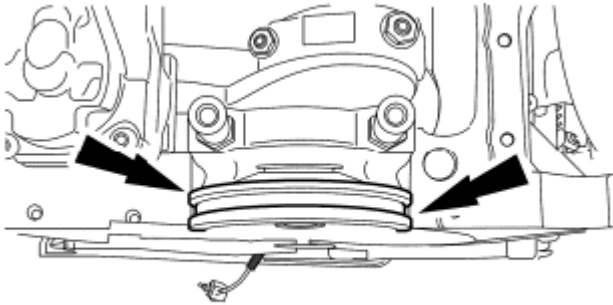
Fig. 173: Locating Gasket Mating Surfaces Courtesy of FORD MOTOR CO.
