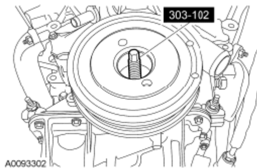
Fig. 403: Installing Crankshaft Pulley
