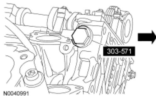
Fig. 141: Identifying Timing Chain Tensioner Courtesy of FORD MOTOR CO.
