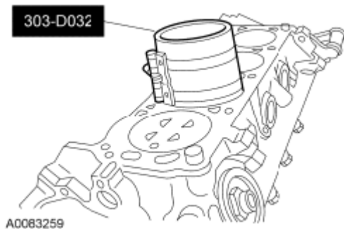
Fig. 354: Installing Piston Using Piston Ring Compressor Courtesy of FORD MOTOR CO.
