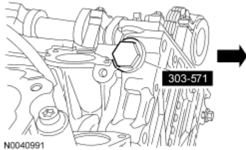
Fig. 18: Identifying Timing Chain Tensioner Courtesy of FORD MOTOR CO.
