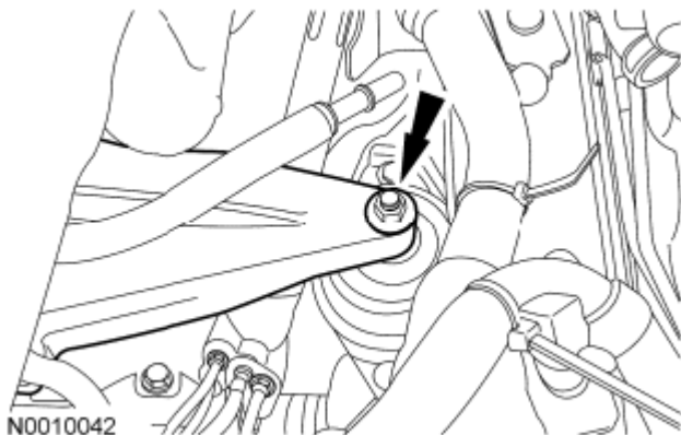
Fig. 478: Locating Engine Mount Nut Courtesy of FORD MOTOR CO.
