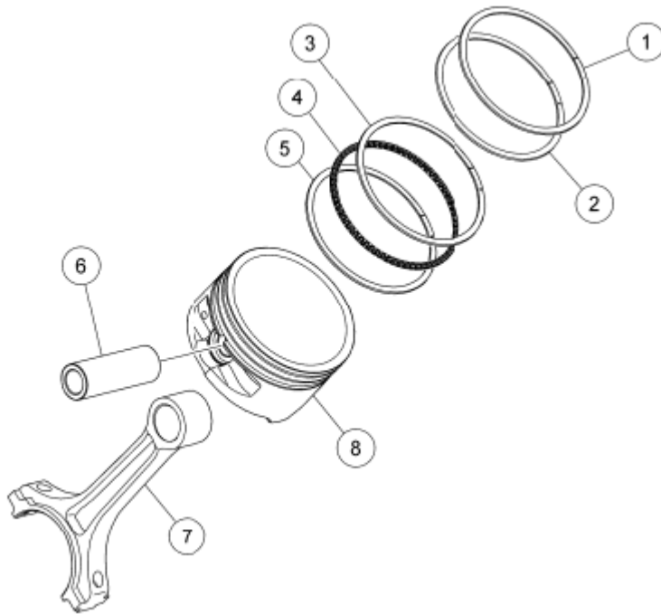
Fig. 340: Exploded View Of Piston Courtesy of FORD MOTOR CO.
