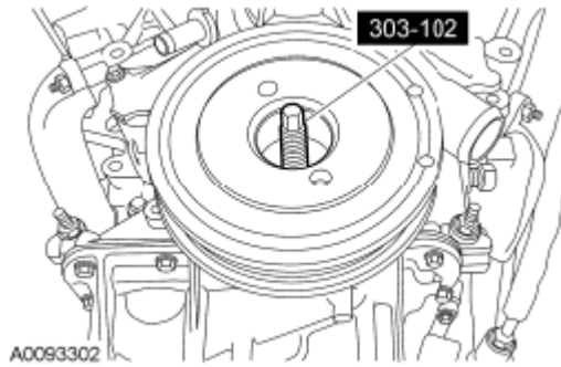
Fig. 33: Installing Crankshaft Pulley Using Crankshaft Vibration Damper Installer Courtesy of FORD MOTOR CO.
