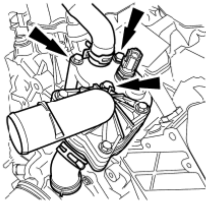
Fig. 443: Locating Thermostat Housing Hoses And Coolant Tube Courtesy of FORD MOTOR CO.
