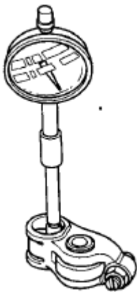
Fig. 106: Measuring Inside Diameter Of Rocker Arm Courtesy of AMERICAN HONDA MOTOR CO., INC.
