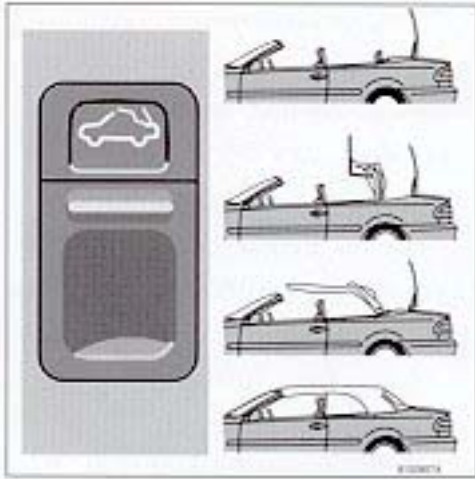
Electrically operated convertible top
