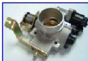
Profile of a throttle position sensor
