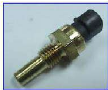
Profile of a coolant temperature sensor
