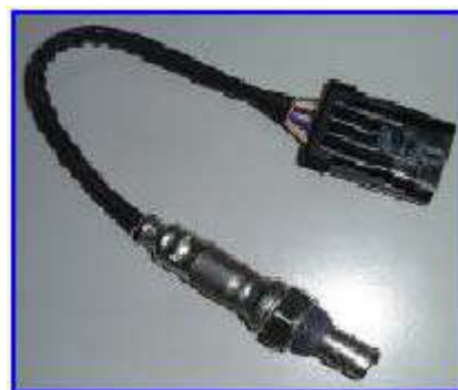
Profile of a oxygen sensor
