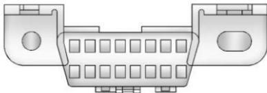
The DLC is under the instrument panel to the left of the steering wheel. Connecting devices that are not used to perform an Emissions Inspection/Maintenance test or to
