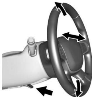
To adjust the tilt and telescoping steering wheel, if equipped:
