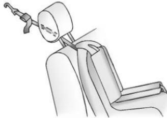
If you are using a single tether, raise the headrest or head restraint and route the tether under the headrest or head restraint and in between the headrest or head restraint posts.
