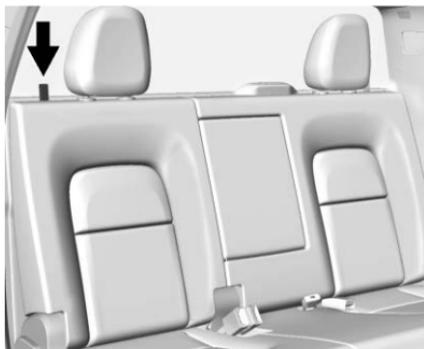
3. Pull the release strap on the outboard side of the seatback.
