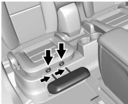
3. Insert the headrest posts into the holes on the front of the passenger side seat cushion to install the seat cushion extension. The notches on the posts should face the passenger side of the vehicle. Try to move the headrest to make sure it is locked in place.
