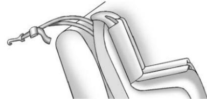
If the position you are using does not have a head restraint and you are using a dual tether, route the tether over the seatback.
