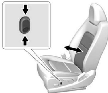
If equipped, press and hold the top of the control to increase lumbar support. Press and hold the bottom of the control to decrease lumbar support. Release the control when the seatback reaches the desired level of lumbar support.
