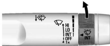
**INT** : Move the lever up to INT for intermittent wipes, then turn the
