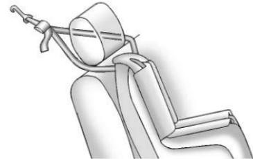
If the position you are using has a fixed head restraint and you are using a dual tether, route the tether around the sides of the head restraint.
