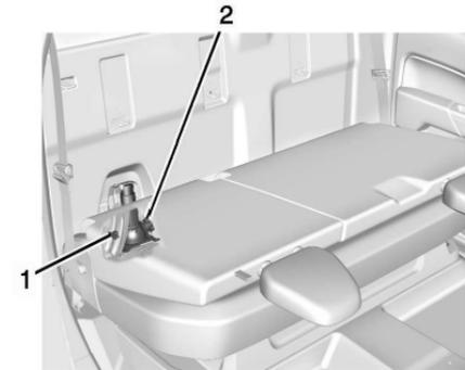
4. Turn the knob on the jack (2) counterclockwise to lower the jack head to release the jack from its holder.
