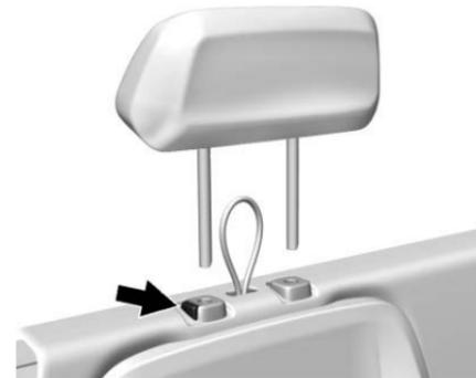
2. Press the button for the passenger side headrest at the top of the seatback and pull up.
