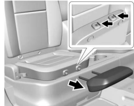
1. If installed as a seat cushion extension, first press both buttons on the front of the seat cushion to remove the headrest.
