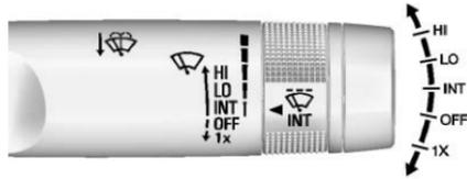
The windshield wiper/washer lever is on the right side of the steering column. With the ignition on or in ACC/ACCESSORY, move the windshield wiper lever to select the wiper speed.
