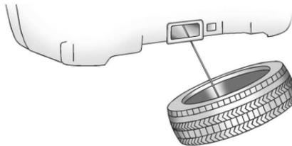
6. Tilt the tire toward the vehicle with some slack in the cable to access the tire/wheel retainer.
