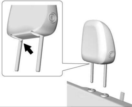
1. Insert the posts into the holes in the top of the seatback. The notch on the post should face the driver side of the vehicle.
