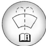
Open the cap with the washer symbol on it. Add washer fluid until the tank is full. See *Engine Compartment Overview* ⇨ 239 for reservoir location.
