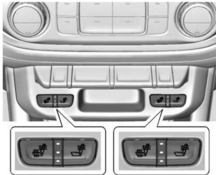
If equipped, the buttons are on the center stack. To operate, the engine must be running.
