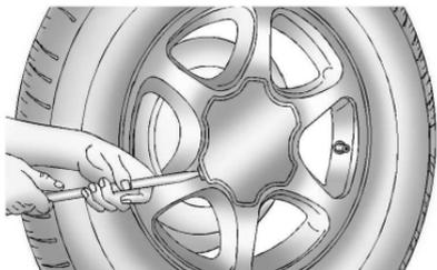
2. If the wheel has a center cap that covers the lug nuts, place the chisel end of the wheel wrench in each of the slots in the cap, and gently pry it out.
