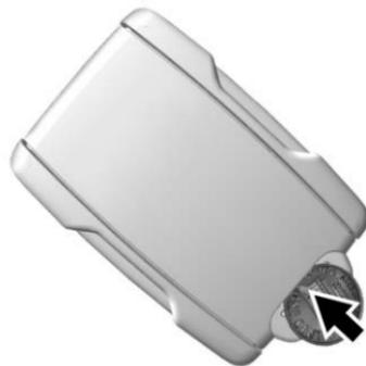
1. Separate and remove the back cover of the transmitter with a flat, thin object, such as a coin.
