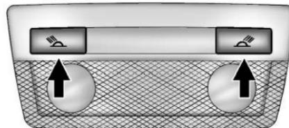
The rear reading lamps, if equipped, are in the headliner.
