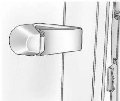
If the vehicle has this feature, squeeze the latch in the center of the window and slide the glass to open it.
