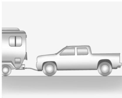
Only dinghy tow four-wheel-drive vehicles that have an N (Neutral) and a Four-Wheel Drive Low (4 ↓) setting.
