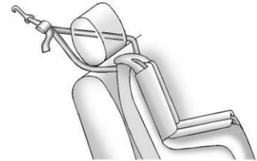
If you are using a dual tether, route the tether around the headrest or head restraint.
