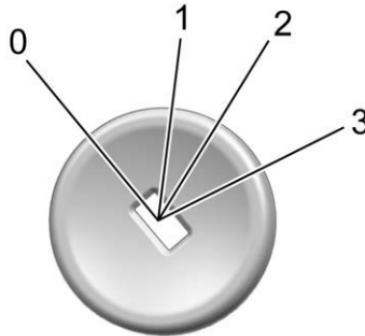
0. Stopping the Engine/LOCK/OFF
