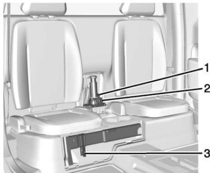
3. Turn the knob on the jack (1) counterclockwise to lower the jack head to release the jack from its holder.
