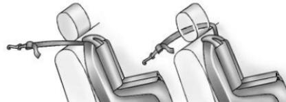
If the position you are using has a fixed head restraint and you are using a single tether, route the tether around the inboard or outboard side of the head restraint.
