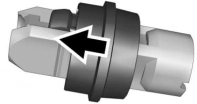
8. Verify the retainer ring is in the proper position. If the retainer ring is out of position, it will not engage. Reset the retainer by pulling it forward with a tool.
