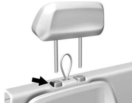
2. Press the button on the passenger side headrest and pull up.
