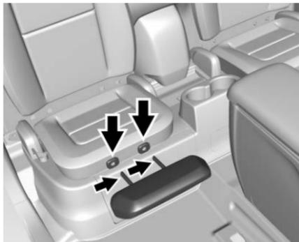
3. Insert the headrest posts into the holes on the front of the passenger side seat cushion to install the seat cushion extension. The notches on the post should face the passenger side of the vehicle. Try to move the headrest to make sure it is locked in place.
