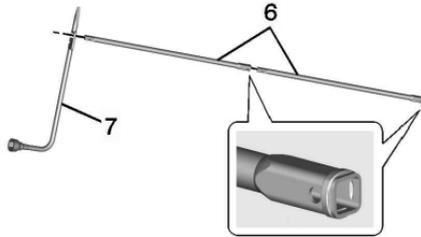
2. Assemble the wheel wrench (7) and the two jack handle extensions (6), as shown.
