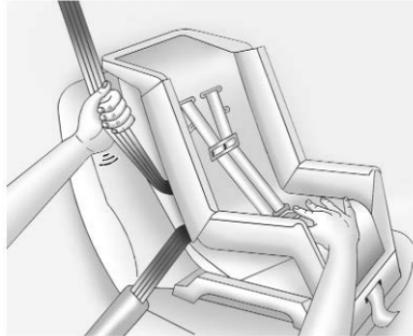
9. To tighten the belt, push down on the child restraint, pull the shoulder portion of the belt to tighten the lap portion of the belt, and feed the shoulder belt back into the retractor. When installing a forward-facing child restraint, it may be helpful to use your knee to push down on the child restraint as you tighten the belt.
