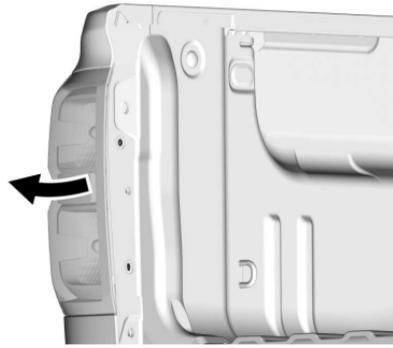
4. Pull the rear lamp assembly straight back to remove it from the vehicle.
