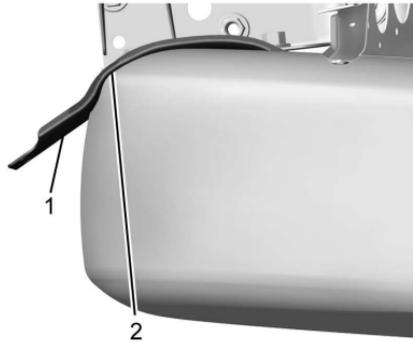
7. Make sure the tire is stored securely and flush in the radius (2) of the spare tire support bracket (1). Push, pull, and then
