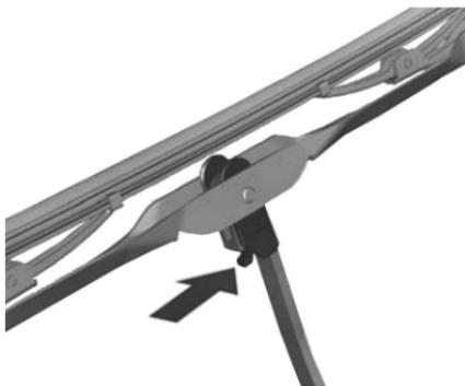
2. Press the release lever in the middle of the wiper blade where the wiper blade attaches.
