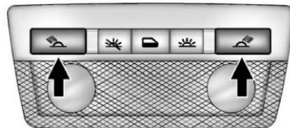
The front reading lamps, if equipped, are in the overhead console.
