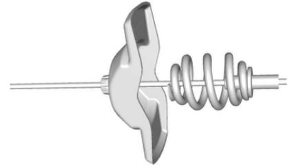
Tilt the retainer and pull it through the center of the wheel along with the cable and spring.
