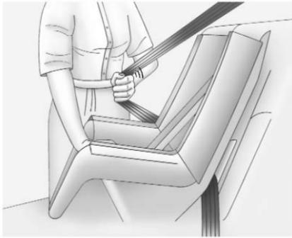
8. Pull the shoulder belt all the way out of the retractor to set the lock. When the retractor lock is set, the belt can be tightened but not pulled out of the retractor.
