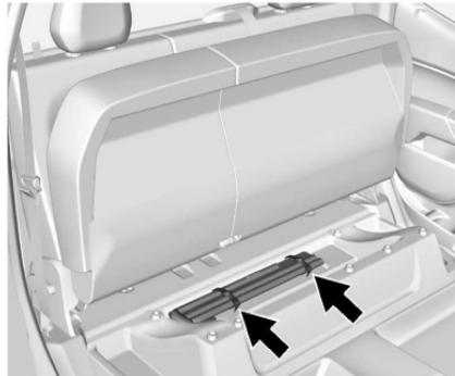
1. Lift the rear seat to access the tool bag.
