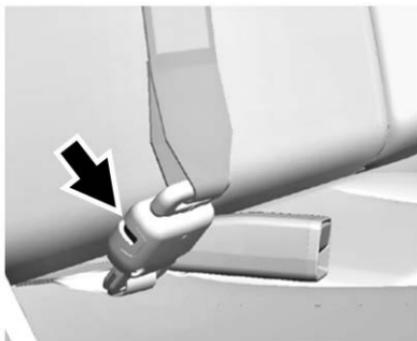
2. Disconnect the rear center seat belt latch from the mini-buckle by inserting the tip of the seat belt tongue into the slot on the buckle. Let the belt retract.
