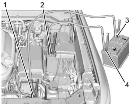
1. Discharged Battery Negative (-) Grounding Point
