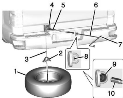
1. Spare Tire (Valve Stem Pointed Down for All Except ZR2 Models. Valve Stem Pointed Up for ZR2 Models.)
