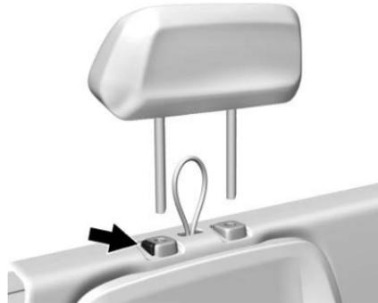
1. Press the button on the side of the headrest post on the top of the seatback and pull up.
