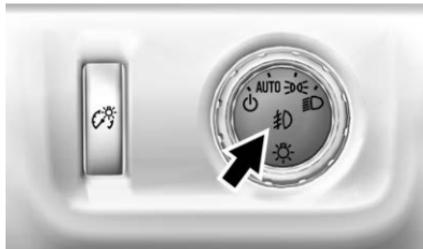
If equipped, the control is on the center of the exterior lamp control, to the left of the steering column.
