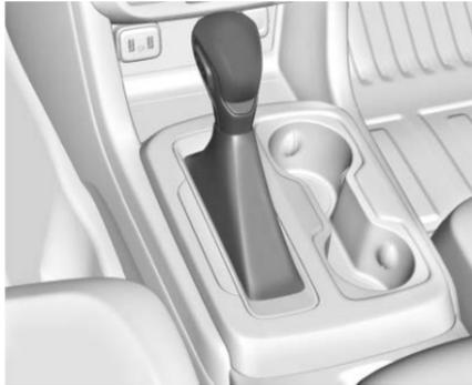
**P** : This position locks the drive wheels. Use P (Park) when starting the engine because the vehicle cannot move easily. When parked on a hill, especially when the vehicle has a heavy load, you might notice an increase in the effort to shift out of P (Park). See “Torque Lock” under *Shifting Into Park* ⇨ 188.
