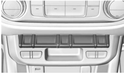
Turn the Tow/Haul Mode on and off by pressing the button on the center stack. When the Tow/Haul Mode is enabled, a light on the instrument cluster will come on.
