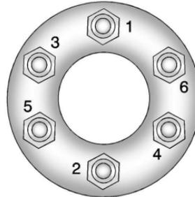
13. Tighten the nuts firmly in a crisscross sequence, as shown, by turning the wheel wrench clockwise.
