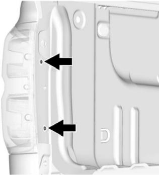
2. Remove the two rear lamp assembly screws.
