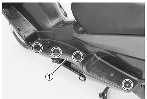
**SIDE LEG SHIELD (RH)****REMOVAL**
