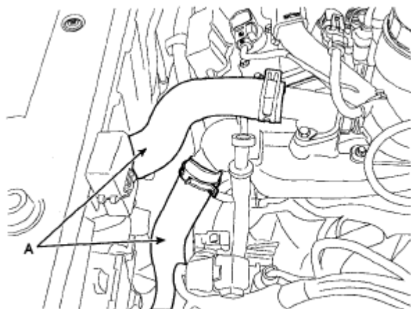
Fig. 103: Locating OCV (Oil Control Valve) Filter Courtesy of HYUNDAI MOTOR CO.
