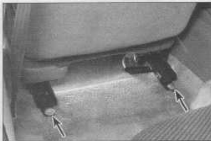
29.2 Front seat - rear mounting bolts (arrows)
