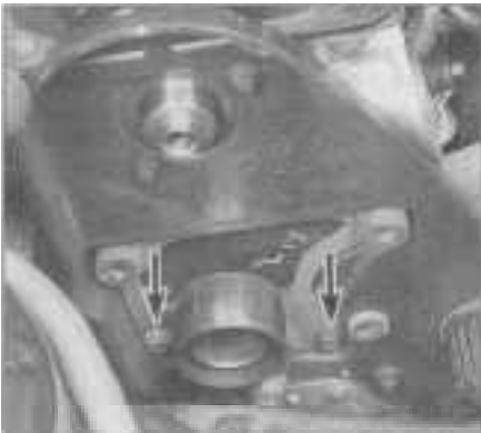
8.4a Remove the hydraulic tensioner pulley/plate assembly mounting bolts (arrows) ..
