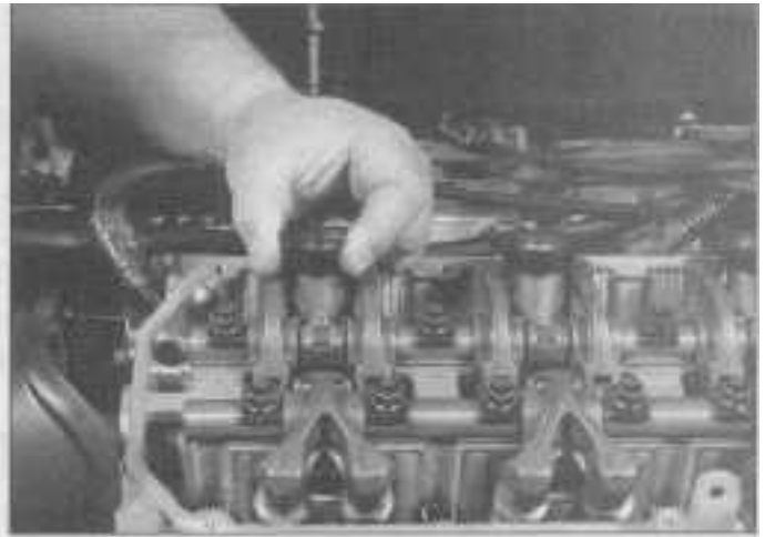
3.7 Remove and replace the seal from each spark plug tube
