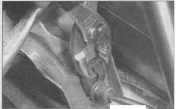
4.13 Use pliers to remove the shift cable retaining clip
