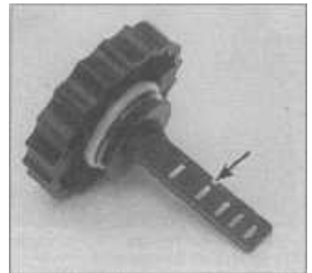
7.5 The power steering fluid dipstick on most models is marked on both sides for checking the fluid level (the arrow is pointing to the COLD level mark)
