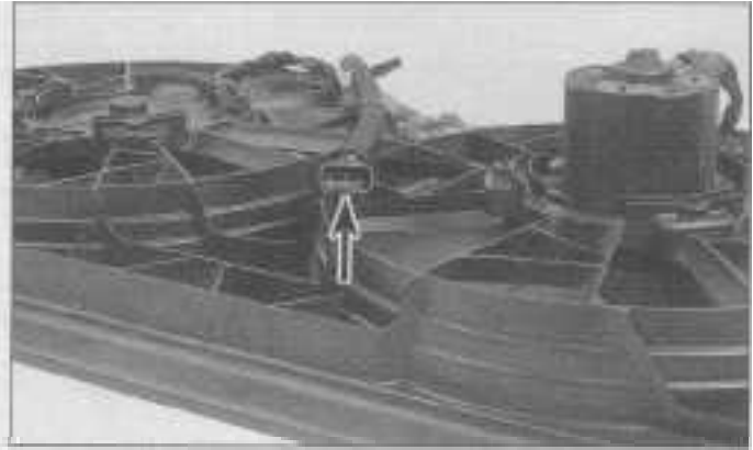
4.1 b Disconnect the fan connector (arrow) and try operating the fan with a fused battery-voltage jumper wire and a ground wire
