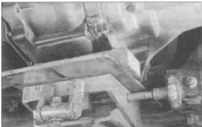
6.28 Place a jack under the transaxle (transmission jack shown) and secure the transaxle to the jack using chains or straps
