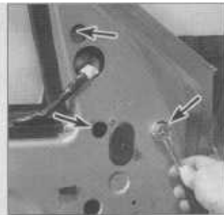
27.8 Remove the exterior mirror mounting nuts through these holes (arrows)
