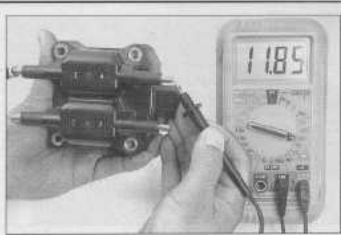
7.5 Checking the secondary resistance of coil "1" - repeat the test for coil "2". The secondary resistance of each coil should be within specifications
