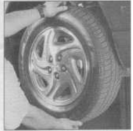
14.10 Checking the wheel bearing freeplay
