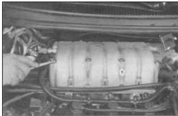
4.7a Starting in the center and working outwards, remove the upper intake manifold mounting bolts in a criss-cross pattern . . .
