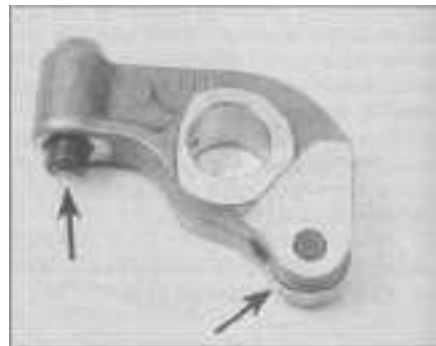
9.8 Visually inspect the hydraulic lash adjuster and roller (arrows) for damage and excessive play - check the rocker arm shaft bore for score marks or excessive wear
