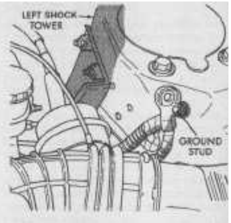
1.4b . . . then detach the cable and push the hole in the cable insulator over the stud
