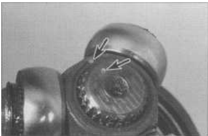
9.25 Use a centerpunch to mark (arrows) the tripod spider to the axleshaft
