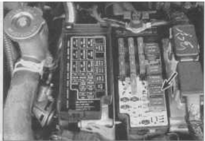
3.20b The fuel pump relay (arrow) is located in the Power Distribution Center under the rectangular cover
