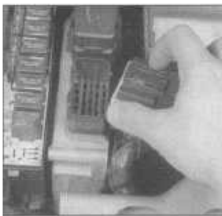
4.3 Disconnecting one of the two Powertrain Control Module (PCM) 40-pin connectors
