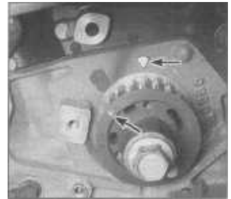
6.21b ... then back it off counterclockwise 3 teeth BTDC (arrows)
