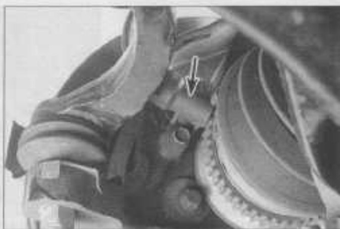
2.9 Wheel Speed Sensor (arrow)
