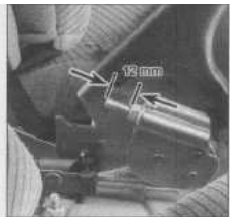
13.12 Tighten the output cable adjusting nut onto the cable until 12 mm of threads are exposed as shown
