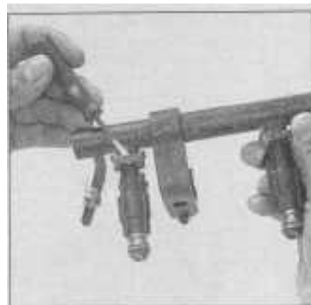
16.26a Using a screwdriver or pliers, remove the injector retaining clip securing the injector to the fuel rail ...
