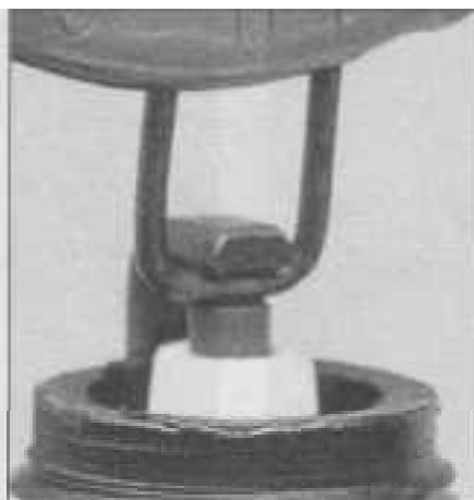
27.5a Spark plug manufacturers recommend using a wire-type gauge when checking the gap - if the wire does not slide between the electrodes with a slight drag, adjustment is required
