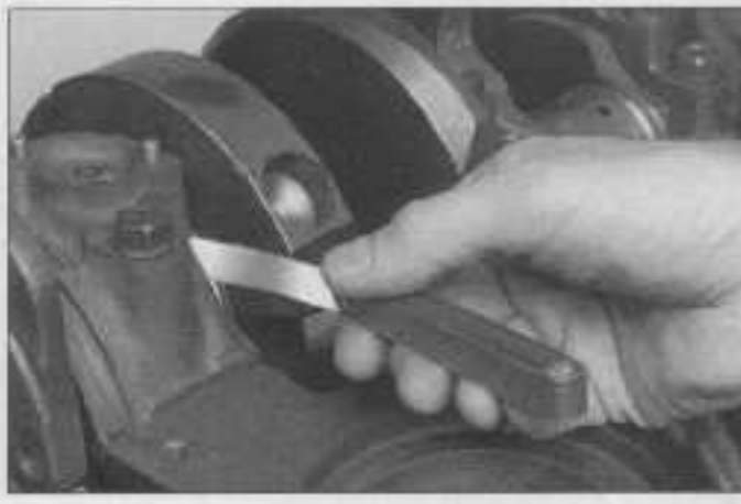
16.3 Checking the crankshaft endplay using feeler gauges at the thrust bearing journal
