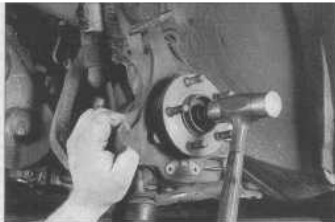
8.8b If the driveaxle is stuck in the wheel hub, apply some penetrating oil to the hub splines then install the hub nut onto the driveaxle a few turns (to protect the threads) and strike the end of the driveaxle with a soft-faced hammer to break it loose - DO NOT attempt to drive the driveaxle out of the hub using a hammer!
