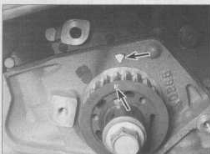
6.21c Rotate the crankshaft timing sprocket clockwise to 1/2-tooth BTDC (arrows)
