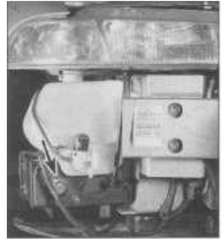
7.12 On 1995 models, the EVAP system charcoal canister (arrow) is located behind the right front bumper fascia (removed for clarity)
