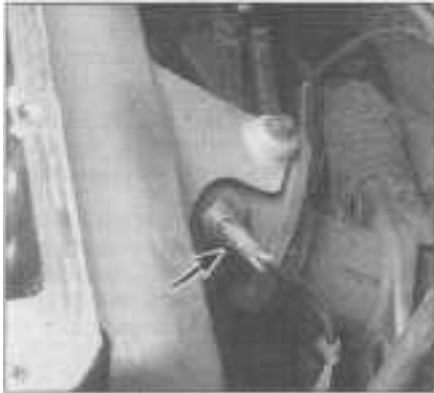
5.4 Follow the harness from the upstream oxygen sensor (arrow) and disconnect it at the connector
