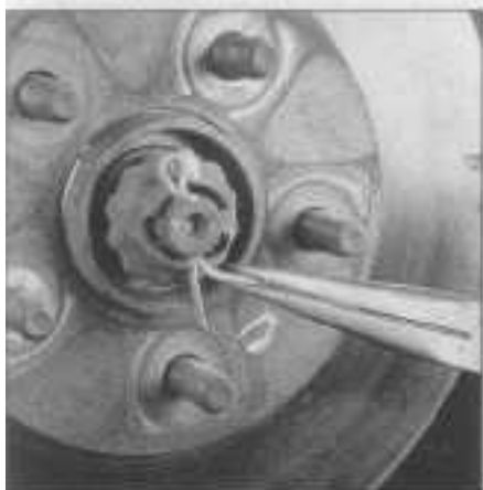
8.2a Remove the hub nut cotter pin ..
