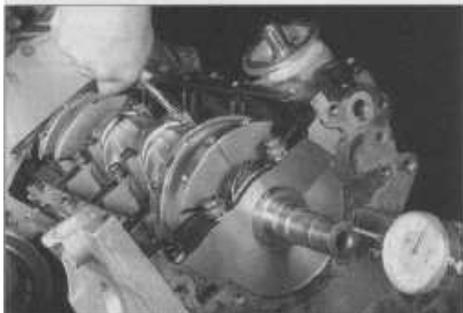
16.1 Checking the crankshaft endplay using a dial indicator
