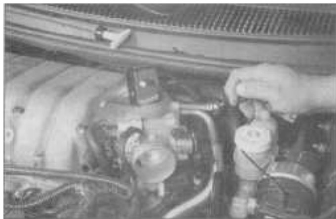
4.6 Remove the EGR tube
