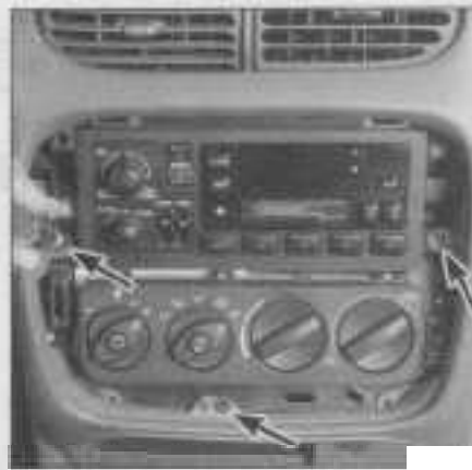
22.6 Remove the three screws (arrows) holding the instrument cluster hood to the instrument panel
