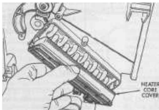
10.6 Remove the heater core cover
