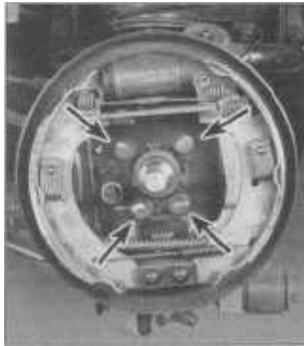
18.5a Remove the brake backing plate bolts (arrows)
