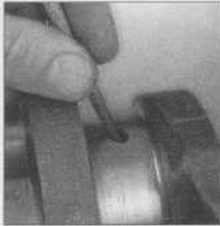
21.1 Using a fine file, break the edge on the crankshaft journal oil passages so sharp edges won't gouge or scratch the new bearings
