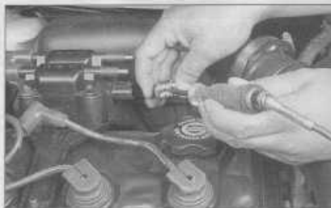
6.9 On four-cylinder engines, connect a test light between the coil electrical connector center terminal and one of the outer terminals. Crank the engine. The test light should blink on-and-off
