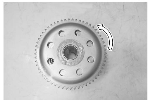
Inspect the starter clutch gear bushing and outer race for any damages.
