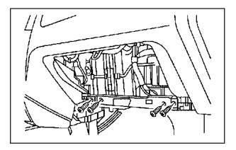
3. Remove the four screws on the knee bolster.
