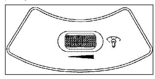
The thumbwheel for this feature is located on the instrument panel to the left of the steering column. Turn the thumbwheel clockwise to brighten the lights or counterclockwise to dim them.
