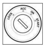
With the key in the ignition switch, you can turn the key to four different positions.
