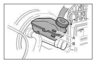
To check the fluid level, look on the side of the reservoir. If the fluid reaches the MAX (A) mark on the reservoir, the fluid level is correct. The reservoir is located near the back of the engine compartment on the driver's side of the vehicle. See *Engine Compartment Overview on page 5-12* for more information on location.
