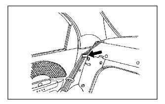
4. Hook the safety belts in the outboard seating positions into the retaining clips.
