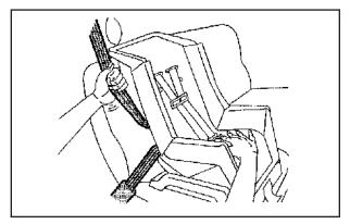
6. To tighten the belt, push down on the child restraint, pull the shoulder portion of the belt to tighten the lap portion of the belt and feed the shoulder belt back into the retractor. If you are using a forward-facing child restraint, you may find it helpful to use your knee to push down on the child restraint as you tighten the belt. You should not be able to pull more of the belt from the retractor once the lock has been set.
