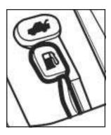
Open the trunk from inside your vehicle by pulling up the release lever located to the left side of the driver's seat.
