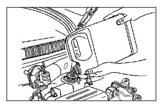
3. Fill the coolant surge tank with the proper mixture to the Maximum mark on the coolant surge tank. Wait about five minutes, then check to see if the level is below the mark. If the level is below the Maximum mark, add additional coolant to bring the level up to the mark. Repeat this procedure until the level remains constant at the Maximum mark for at least five minutes.
