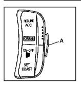
The cruise control pad is located on the right side of the steering wheel.
