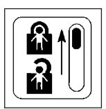
Your vehicle has rear door security locks on each rear door that help prevent passengers from opening the rear doors on your vehicle from the inside.
