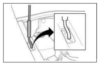
Place the hood prop into the slot on the inner fender. Before closing the hood, be sure all the filler caps are on properly. Then lift the hood to relieve pressure on the hood prop. Remove the hood prop from the slot in the inner fender and return the prop to its retainer. Lower the hood 12 inches (30 cm) above the vehicle and release it to latch fully. Check to make sure the hood is closed and repeat the process if necessary.
