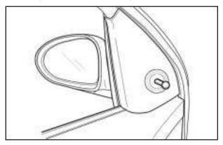
Adjust the outside manual mirrors using the control lever located next to the mirror.
