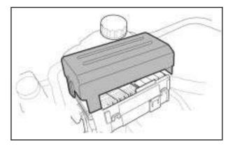
The engine compartment fuse block is located on the driver's side of the vehicle, near the battery. See *Engine Compartment Overview on page 5-12* for more information on location. To access the fuses, pull out the top and bottom flaps to release the cover. To reinstall the cover, push the cover until it is secure.
