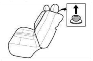
Pull up the release knob, located on the top of the seatback, and fold the seatback forward and down. Notice: Folding a rear seat with the safety belts still fastened may cause damage to the seat or the safety belts. Always unbuckle the safety belts and return them to their normal stowed position before folding a rear seat.
