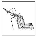
If the position you are using has a head restraint and you are using a dual tether, route the tether under the head restraint and in between the head restraint posts.
