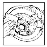
Remove any rust or dirt from the wheel bolts, mounting surfaces and spare wheel. 12. Place the compact spare tire on the wheel-mounting surface.
