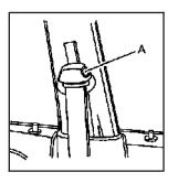
To move it down, press the release button (A) and move the height adjuster to the desired position.
