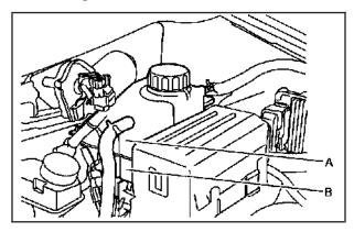
The engine coolant surge tank is located in the rear of the engine compartment on the driver's side of the vehicle. See *Engine Compartment Overview on page 5-12* for more information on location.
