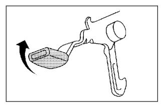
Then go to the front of the vehicle and lift up on the secondary hood release lever, located under the front center of the hood. 3. Lift the hood and release the hood prop from its retainer located on the underside of the hood.
