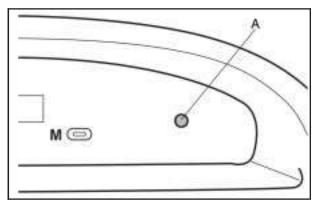
The security light (A) will flash once every second to indicate that the theft-deterrent system is armed. The security light is located on the secondary information center (SIC) on the center of the instrument panel. To avoid activating the alarm by accident, do one of the following:
