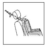
If the position you are using has an adjustable head restraint and you are using a single tether, route the tether under the head restraint and in between the head restraint posts.
