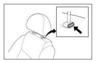
Pull the head restraint up to raise it. To lower it, press the button, located on the top of the seatback, and push the head restraint down.
