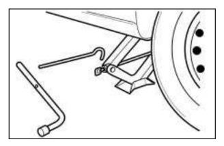
7. Insert the jack handle into the jack and the wheel wrench onto the end of the jack handle.
