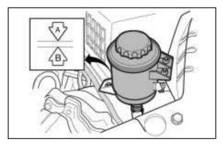
The level should be between the MIN (B) and MAX (A) marks on the reservoir. If the level drops below the MIN (B) mark, add power steering fluid.
