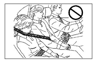
move the child toward the center of the vehicle. If the child is sitting in the center rear seat passenger position, move the child toward the safety belt buckle. In either case, be sure that the shoulder belt still is on the child's shoulder, so that in a crash the child's upper body would have
