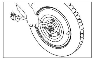
3. Use the wheel wrench to loosen all the wheel nuts. Do not remove them yet.
