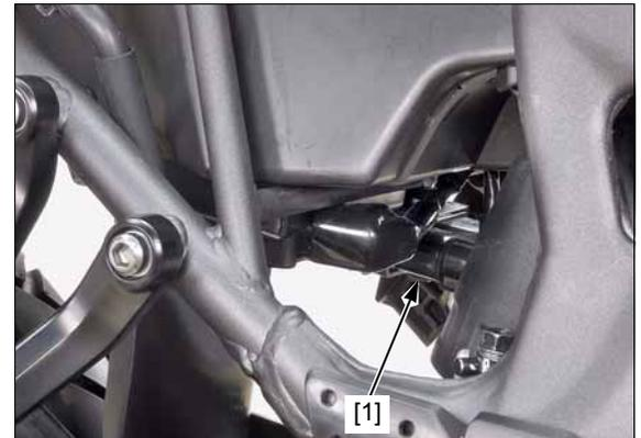
CRF1000: Release the turn signal light relay [1].
