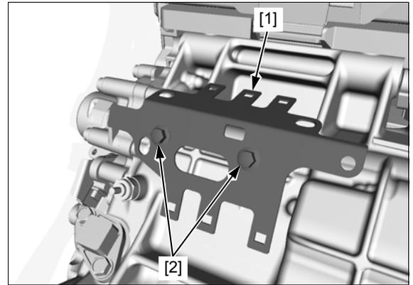
Install the O<sub>2</sub> sensor wire clip [1] to the connector clip stay.
