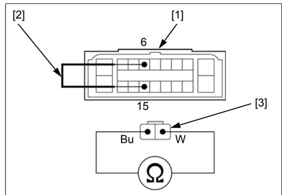
**4. Failure Reproduction with a New Speed Sensor**
