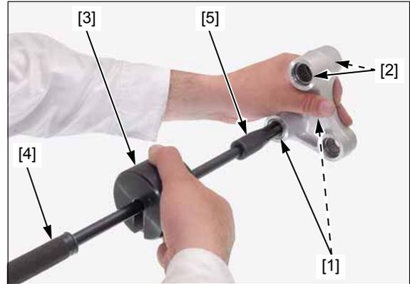
Remove the needle bearing (17 x 24 x 17 mm) [1] using the special tools and hydraulic press.
