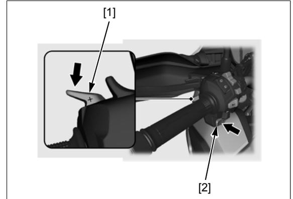
4. The self-diagnostic memory is erased if the shift indicator "-" goes off and starts blinking as shown.
