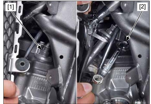
Replace new spark plugs as set. Install and hand tighten the spark plug to the cylinder head, then tighten the spark plug to the specified torque using the equipped spark plug wrench.
