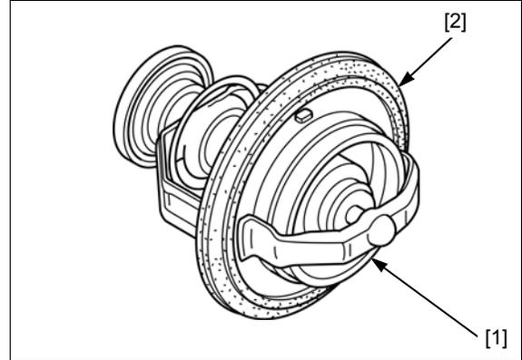
Visually inspect the thermostat [1] for damage.
