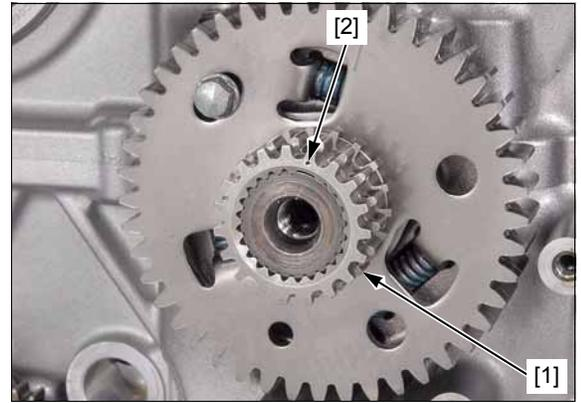
Temporarily install the clutch outer [1].
