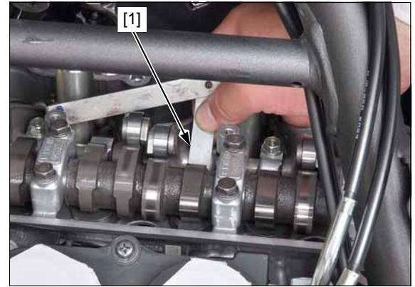
Check the No.2 cylinder exhaust valve clearances by inserting a feeler gauge [1] between the rocker arm roller and cam lobe.
