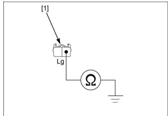
**DTC 7-2 (ECT SENSOR HIGH VOLTAGE)**
