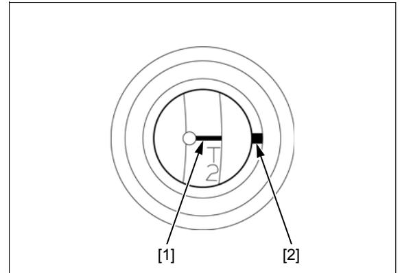
Install the valve lifters [1] and shims [2].
