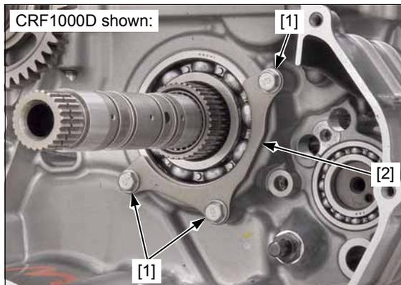
Remove the right mainshaft bearing [1] from the upper crankcase.
