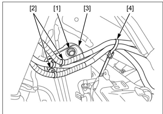
Connect the immobilizer receiver 4P (Black) [1] and ignition switch 2P (Brown) [2] connectors and install them to the ignition coil tray.
