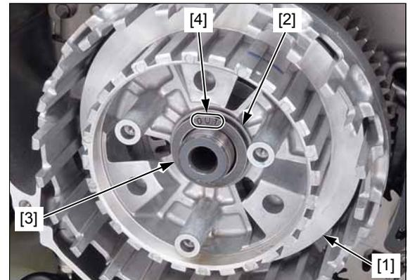
Apply engine oil to a new clutch center lock nut threads and seating surface.
