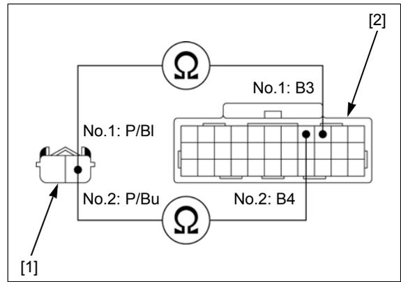
**5. Fuel Injector Signal Line Short Circuit Inspection**
