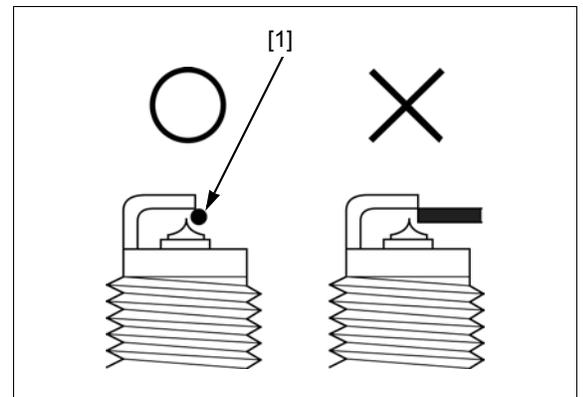
*Do not adjust the spark plug gap. If the gap is out of specification, replace it with a new one.*
