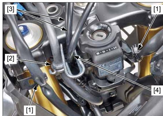
Remove the steering stem nut [1].
