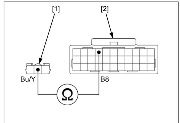
**6. TP Sensor Signal Line Short Circuit Inspection**
