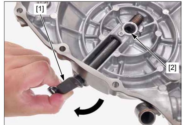
Install the right crankcase cover [1] by holding the clutch lifter lever [2].
