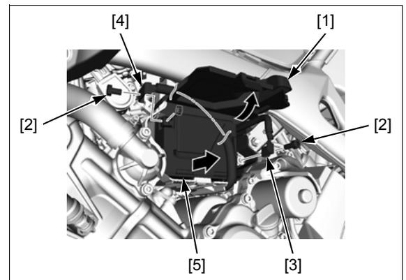
Remove the bolt [1] and battery negative (-) cable [2].
