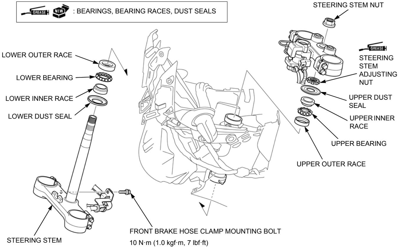
Apply specified grease (page 1-23) to the upper and lower bearings and bearing races.
