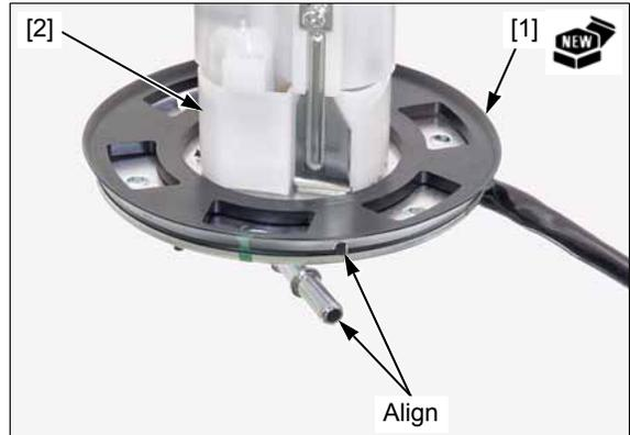
Install the fuel pump unit [1] into the fuel tank.
