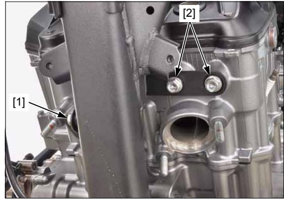
Tighten the rear upper bolts (8 x 25 mm) [1] to the specified torque.
