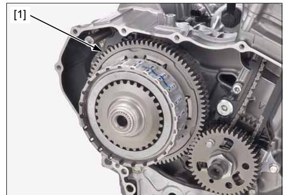
Remove the seal rings [1] from the mainshaft grooves.
