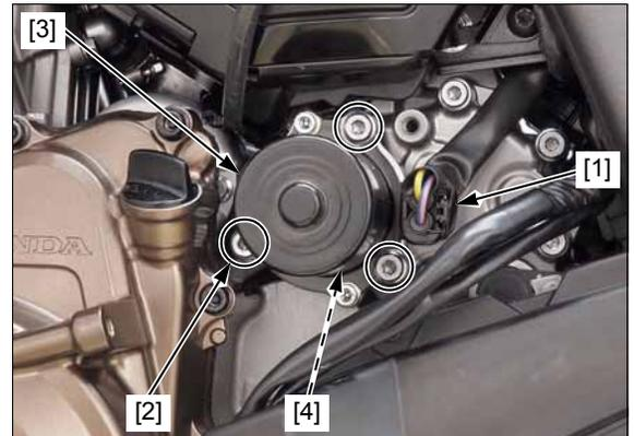
Remove the torx bolts [1] and reduction gear cover [2].
