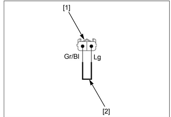
**3. ECT Sensor Output Line Open Circuit Inspection**
