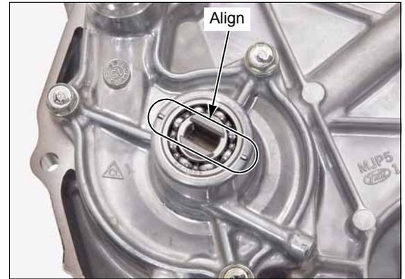
Turn the clutch lifter lever [1] clockwise so that the lever slit [2] is in position as shown.
