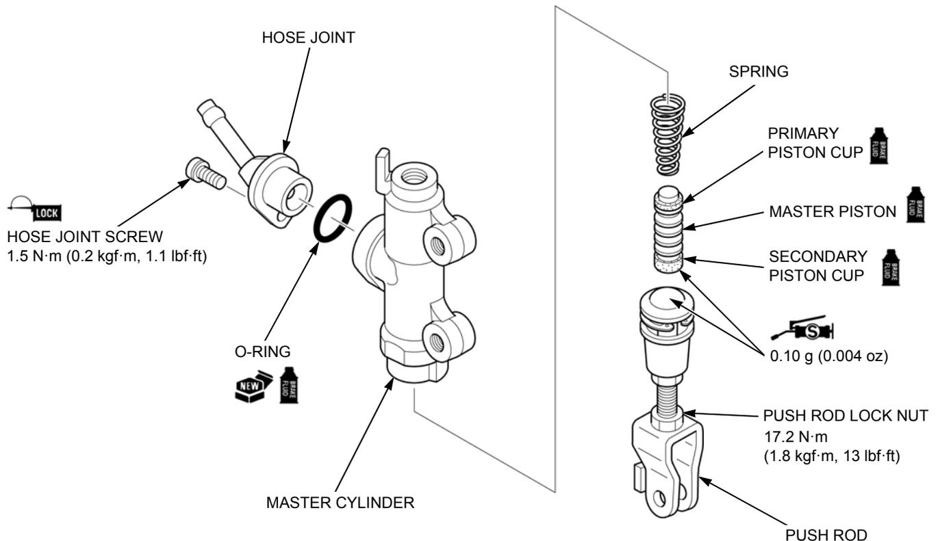
When the push rod has been disassembled, adjust the push rod length so that the distance from the center of the master cylinder lower mounting bolt hole to the center of the joint pin hole is standard length as shown.
