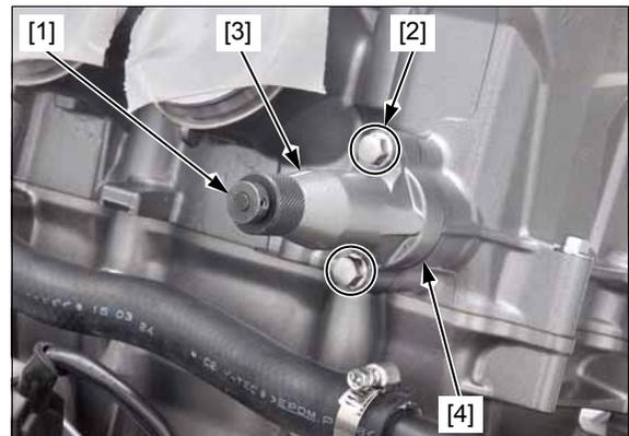
Install a new gasket [1] on the cam chain tensioner lifter [2] and install them to the cylinder.
