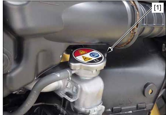
Wet the sealing surfaces of the cap, then install the cap onto the tester [1].
