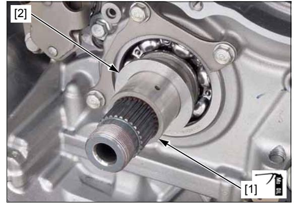
Apply engine oil to the clutch outer needle bearing.
