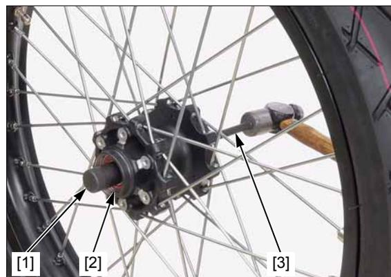
*Never install the old bearings. Once the bearings have been removed, the bearings must be replaced with new ones.*
