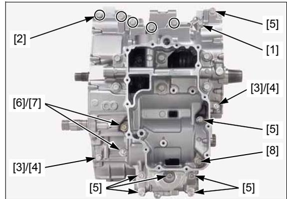
Loosen the crankcase main journal bolts [1] in a crisscross pattern in 2 or 3 step, and remove them.
