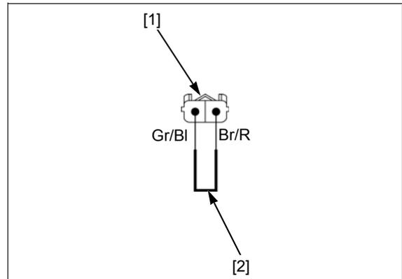
**3. IAT Sensor Output Line Open Circuit Inspection**
