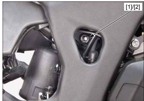
Remove the rear shock absorber [1] by lifting the swingarm [2].
