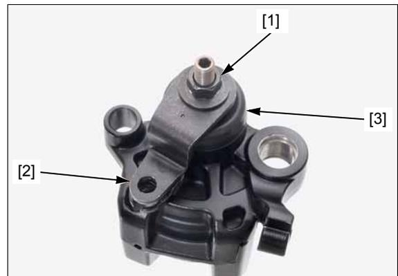
Remove the push rod [1] while holding the brake shaft [2].
