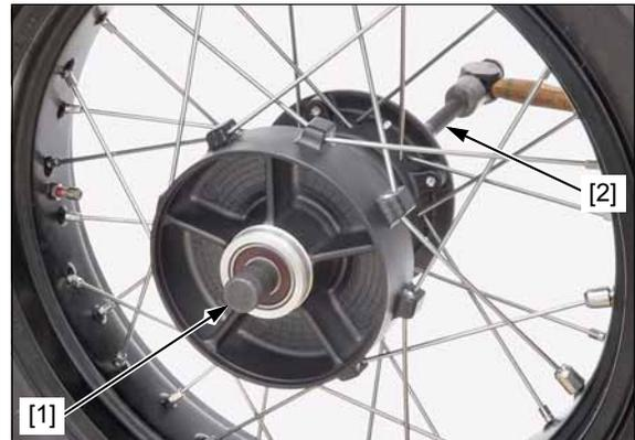
*Never install the old bearing, once the bearing has been removed, the bearing must be replaced with new ones.*
