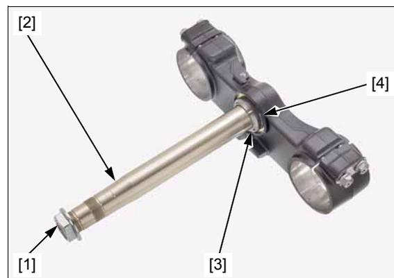
Apply specified grease to a new lower dust seal lips (page 1-23).
