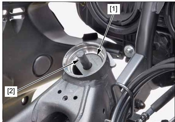
Remove the lower outer race using the special tool and suitable shaft.
