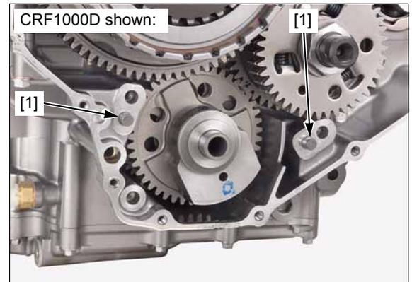
Install the bolts [1] and rear balancer shaft holder [2] and tighten the bolts to the specified torque.
