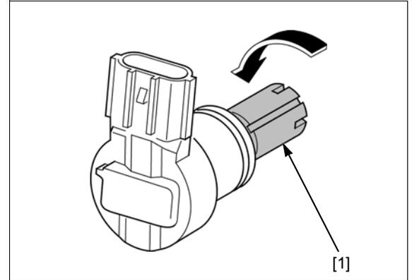
Install a new O-ring [1] onto the IACV [2].
