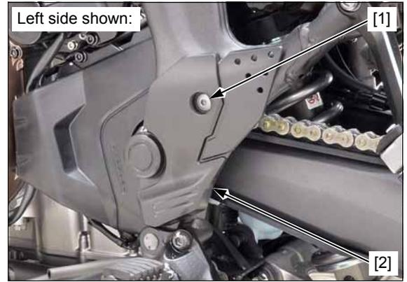
Remove the bolt [1] and brake hose clamp [2].
