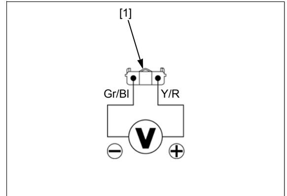
**3. MAP Sensor System Inspection with Jumper Wire**
