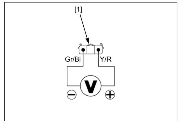
**2. MAP Sensor Input Voltage Inspection**
