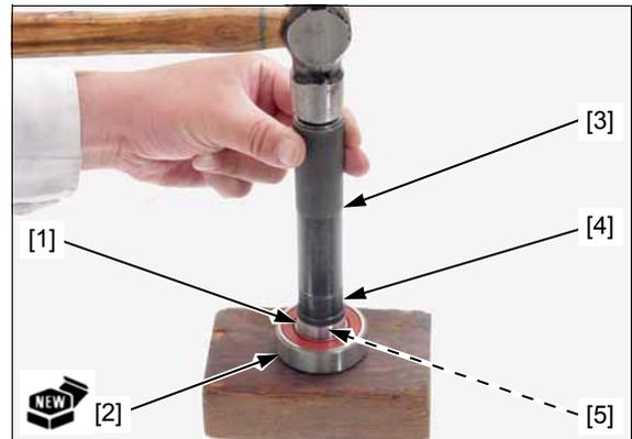
Drive in the bearing/collar [1] squarely with its collar side facing down until it is fully seated.
