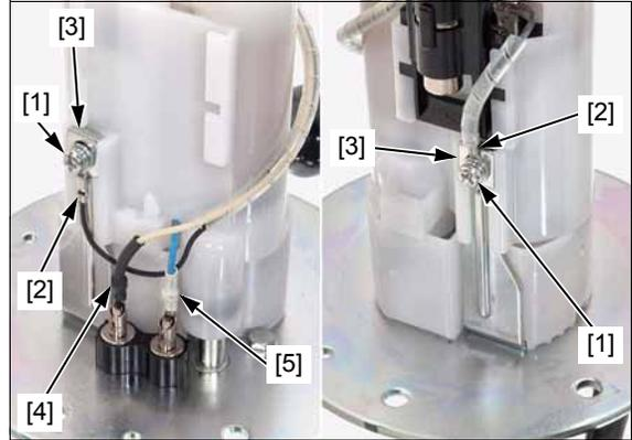
Remove the fuel pump filter assembly [1] and O-ring [2] from the fuel pump stay [3].
