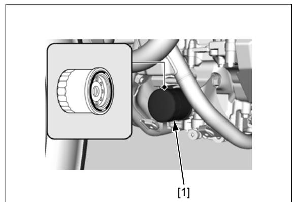
Check the oil filter boss [1] protrusion from the crankcase is within the specified length as shown.
