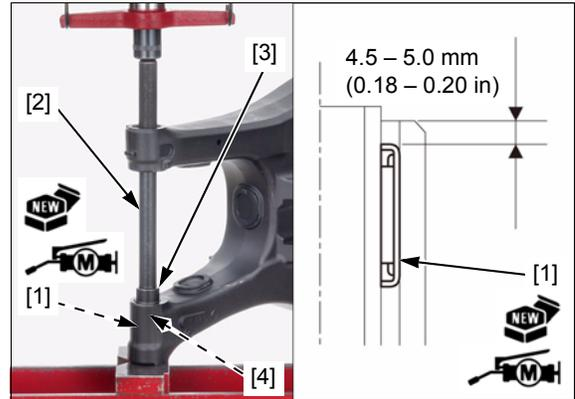
Apply molybdenum disulfide grease to a new ball bearing rotating area.
