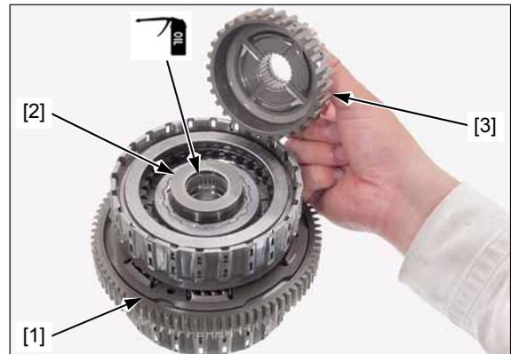
Turn over the dual clutch assembly while holding clutch guide 1.
