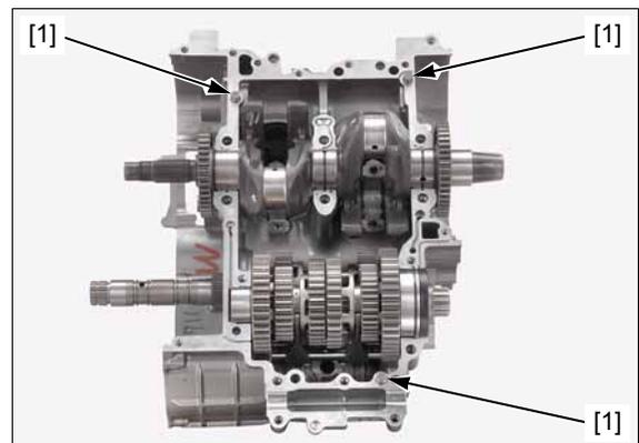
Install the lower crankcase onto the upper crankcase. Make sure that the upper and lower crankcase are seated securely.
