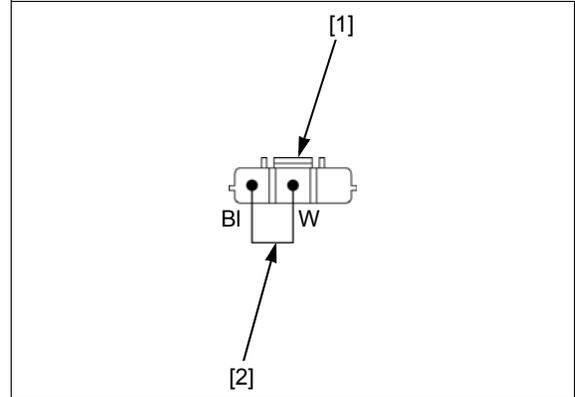
**3. EOP Sensor Ground Line Open Circuit Inspection**
