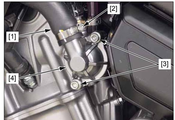
Remove the thermostat [1] from the upper crankcase.
