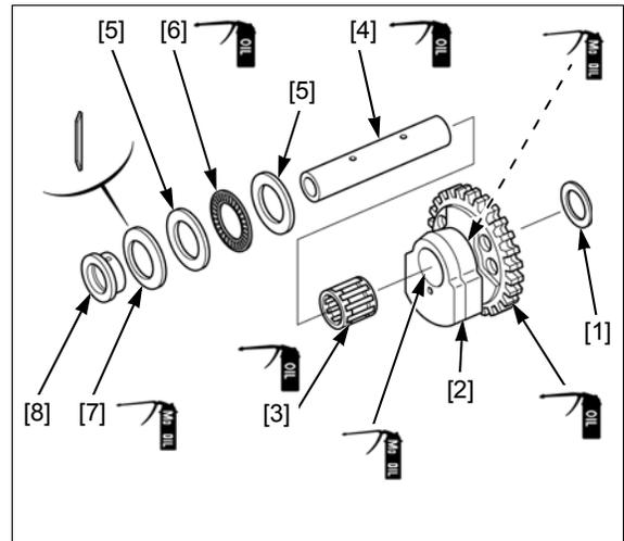
Insert the rear balancer driven gear assembly shaft end [1] into the hole [2] of the lower crankcase.
