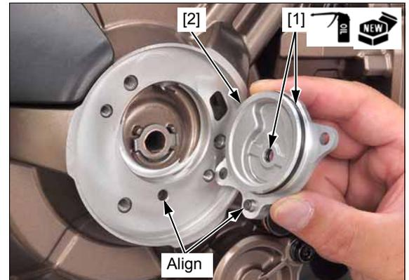
Install and tighten the bolts [1] to the specified torque.
