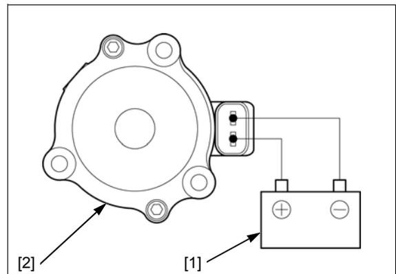
**4. Shift Spindle Angle Sensor System Inspection**
