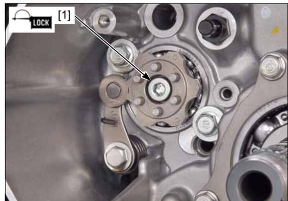
Install the thrust washer [1] onto the gearshift spindle [2].
