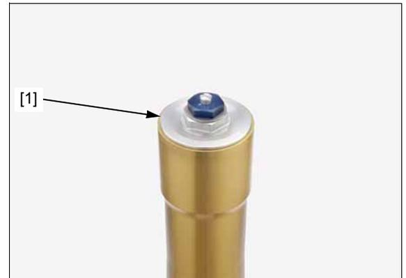
Push the outer pipe [1] slowly down, and gently seat the dust seal [2] onto the axle holder [3].
