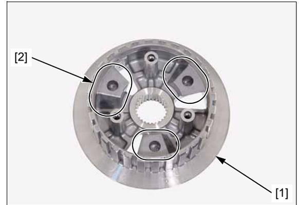
Check the following of the clutch outer [1] for scratch, damage, abnormal wear and deformation.
