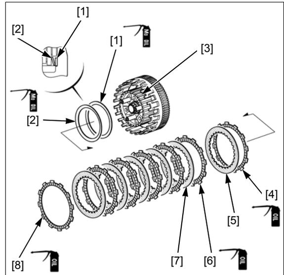
Install the clutch lifter pin [1].
