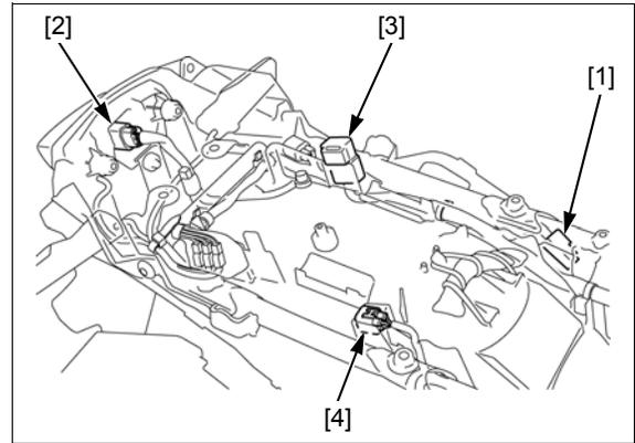
CRF1000A/D: Release the rear speed sensor wire clip [1].
