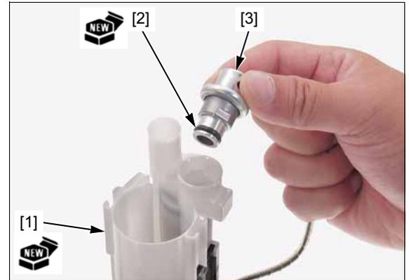
Install a new O-ring [1] to the fuel pump [2].
