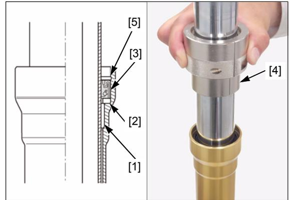
*Do not scratch the fork pipe sliding surface.*
