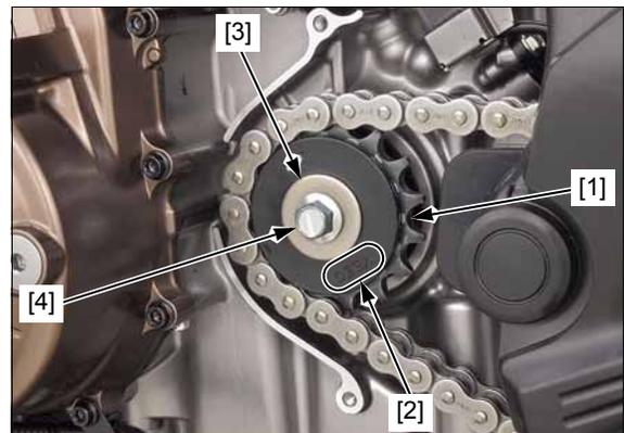
Install the stay [1] and bolt [2], and tighten the bolt securely.
