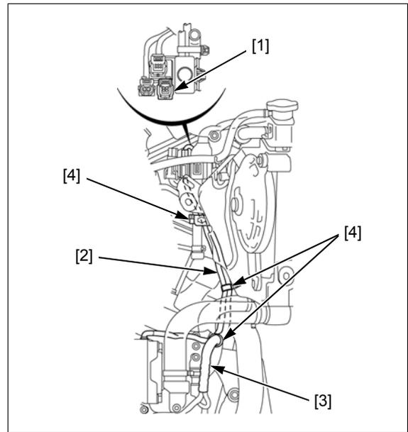
Install the wire stay [1] and bolt [2], and tighten the bolt to the specified torque.
