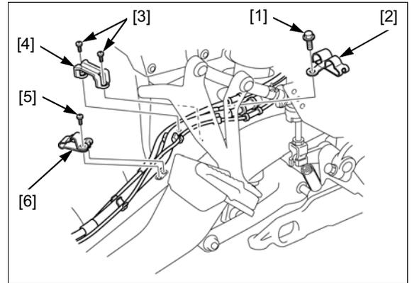
*CRF1000D:* Remove the bolt [1] and parking brake cable guide [2].
