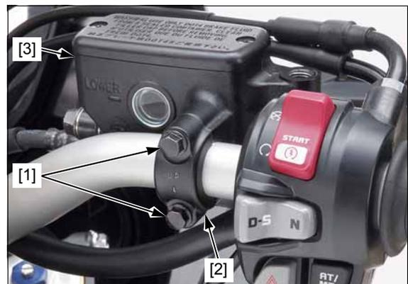
Remove the screw/washers [1] and separate the right handlebar switch housing [2].
