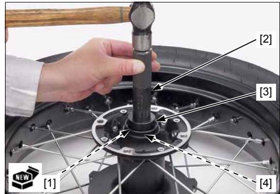
Drive in the rear wheel distance collar B [1] to a new bearing [2].
