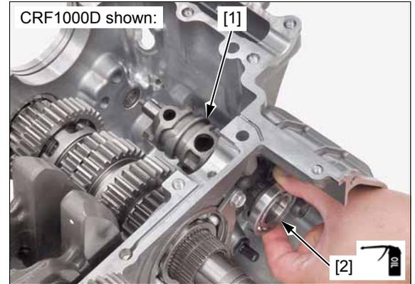
Apply locking agent to the shift drum bearing setting bolt threads (page 1-20).
