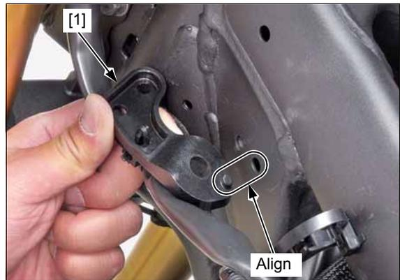
Install the bolt [1] and tighten it securely.
