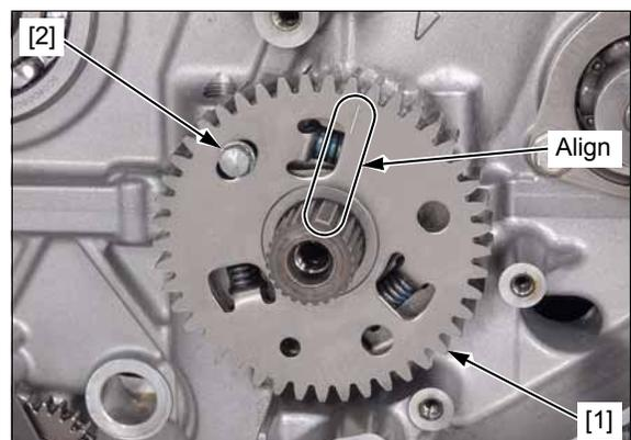
Install the timing sprocket [1] with its punch mark [2] facing out as shown
