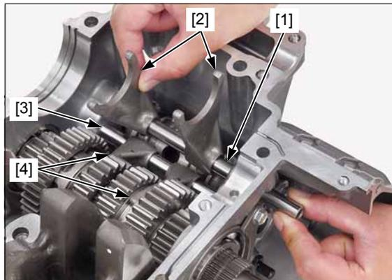
Remove the shift drum bearing setting bolt [1] and washer [2].
