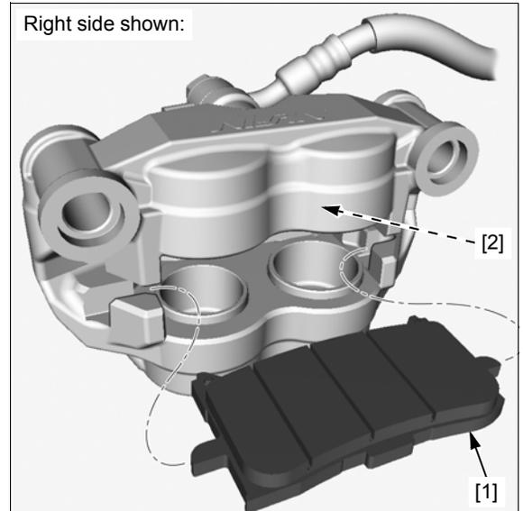
Install the brake caliper [1] and new mounting bolts [2].
