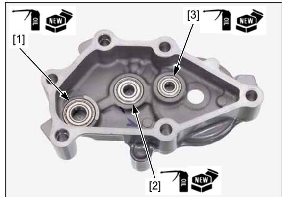
Check the bearings and replace if necessary (page 14-19).
