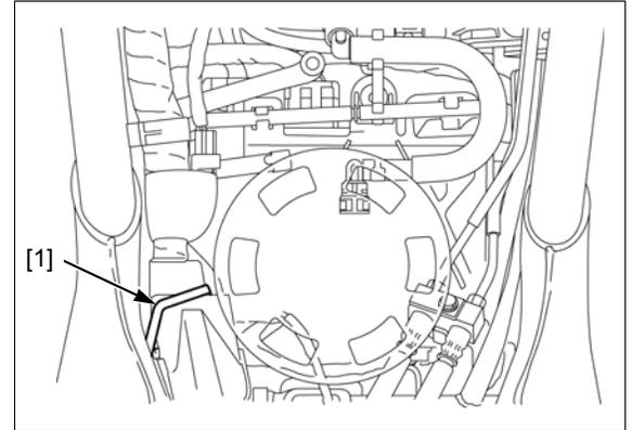
Disconnect the turn signal light relay 18P (Black) connector [1].
