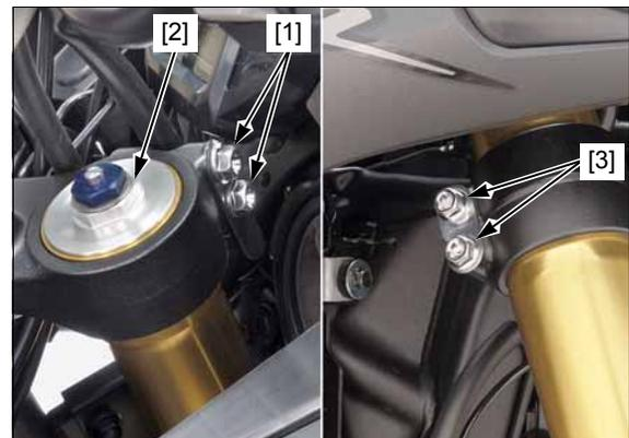
When disassembling the fork, turn the pre-load adjuster [1] and rebound adjuster [2] counterclockwise to the softest position (be sure to record the number of turns from the starting position).
