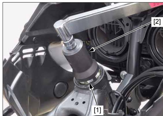
Install the brake hose clamp [1] and bolt [2] and tighten the bolt to the specified torque.
