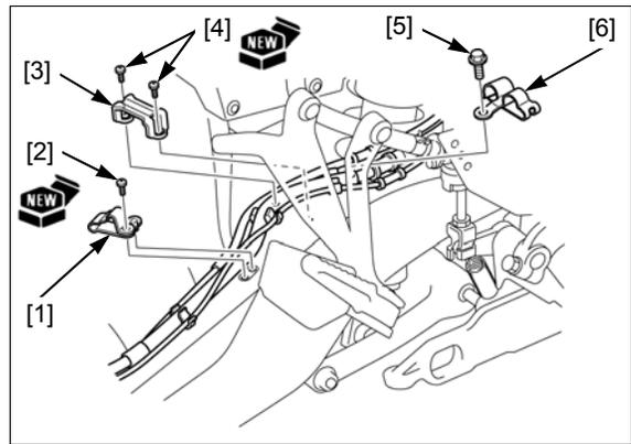
Install the left/right heel guards [1] and socket bolts [2] and tighten the bolts securely.
