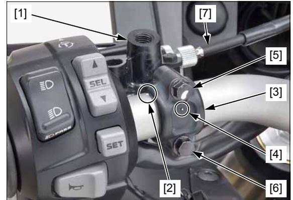
Connect the parking brake switch connectors [1].
