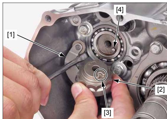
Apply locking agent to the threads of the shift drum center bolt [1] (page 1-21). Install the shift drum center bolt and tighten it to the specified torque.
