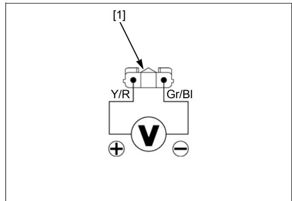
**4. TP Sensor Input Line Open Circuit Inspection**
