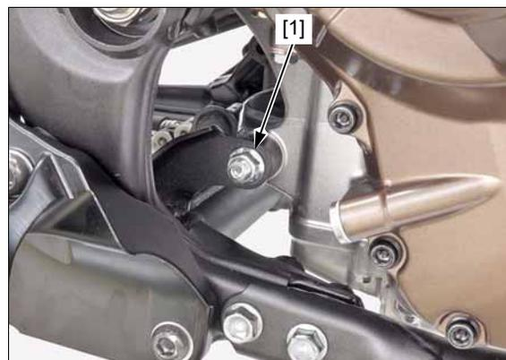
Tighten the front lower nut (10 mm) [1] to the specified torque.
