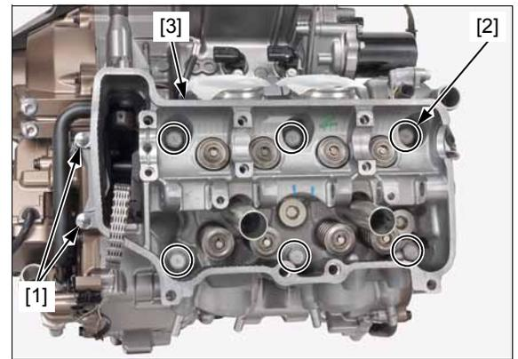
Remove the gasket [1] and dowel pins [2].
