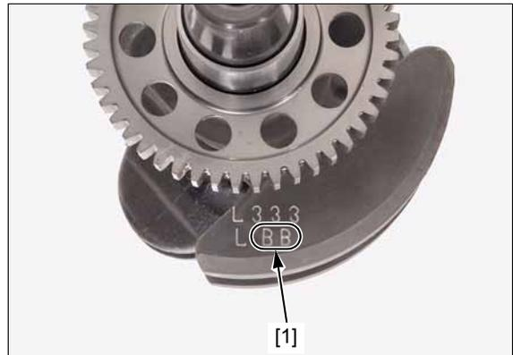
Cross-reference the connecting rod and crankpin codes to determine the replacement bearing color code [1].
