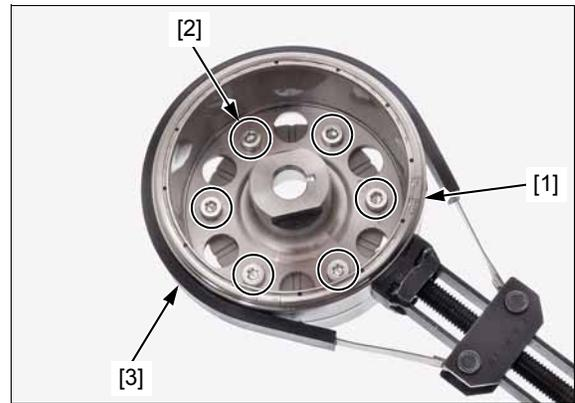
Remove the starter clutch assembly [1].
