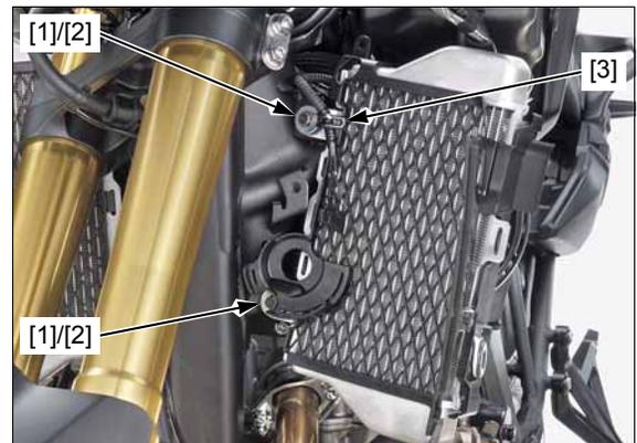
Release the connector clip [1] from the radiator shroud.
