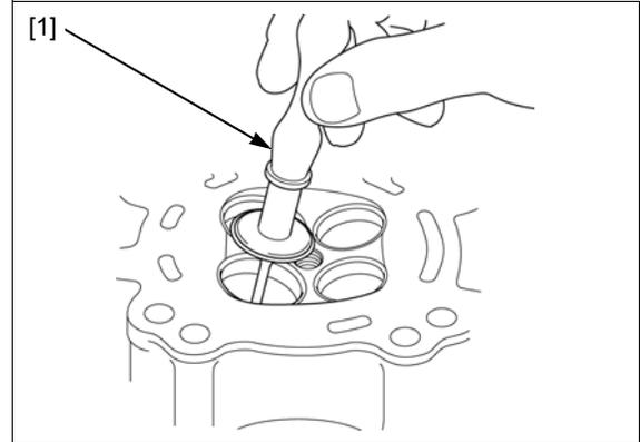
*The valves cannot be ground. If the valve face is burned, badly worn, or if it contacts the seat unevenly, replace the valve.*
