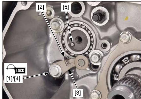
Hold the stopper arm [1] using a screwdriver.
