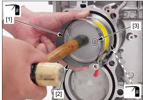
*Make sure the piston ring compressor tool sits flush on the top surface of the cylinder.*
