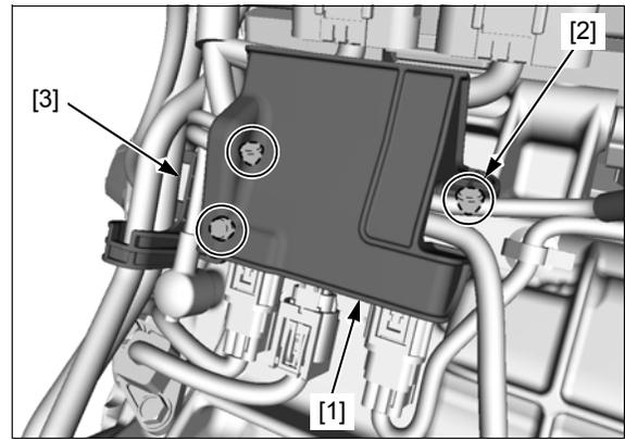
Install the alternator assembly wire onto the frame:
