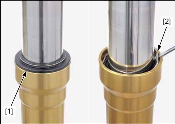
Pull the slide pipe assembly [1] out until you feel resistance from the slider bushing. Then move it in and out, tapping the bushing lightly until the outer pipe [2] separates from the slide pipe assembly. The guide bushing will be forced out by the slider bushing.
