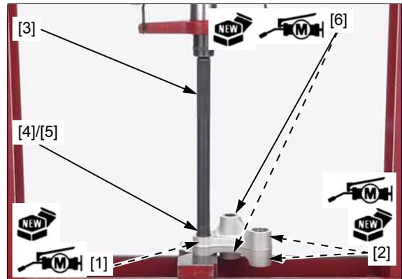
Install the needle bearings (17 x 24 x 30 mm) [6] with its marked side facing up until it is flush with the cushion arm surface using the special tools and hydraulic press.
