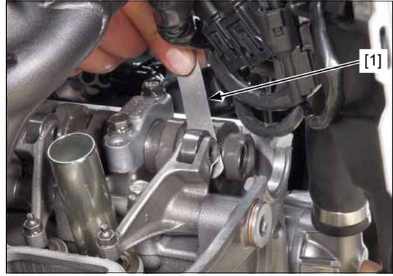
Adjust the No.1 cylinder exhaust valve clearance by loosening the lock nut [1] and turning the adjusting screw [2] until there is a slight drag on the feeler gauge [3].
