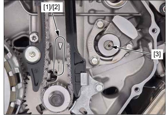
Rotate the water pump shaft and align the shaft slit with the pump cover index lines as shown.
