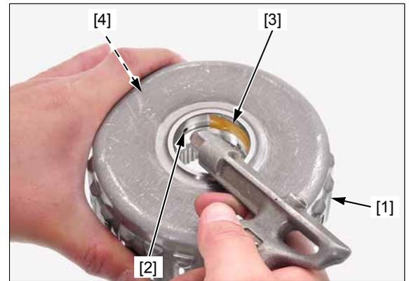
Remove the clutch piston [1] and O-rings [2].
