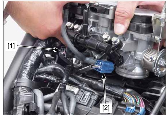
Loosen the throttle cable A adjuster lock nut [1] and adjusting nut [2] then disconnect the throttle cable A [3] from the throttle drum and cable stay.
