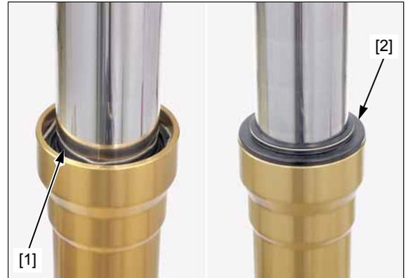
Install the fork damper assembly [1] and centering plate [2].
