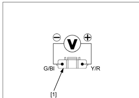
**4. Clutch EOP Sensor Input Line Open Circuit Inspection**
