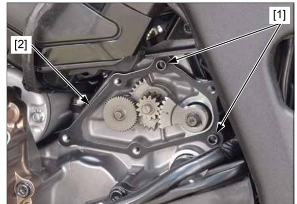
Install the reduction gear cover [1] and torx bolts [2], then tighten the torx bolts.
