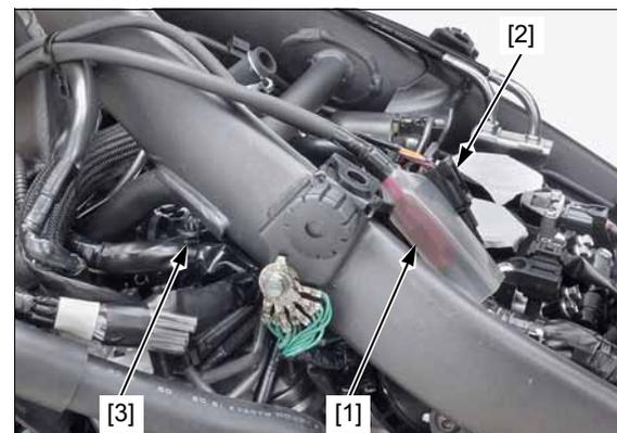
Loosen the band screws (throttle body side) [1].
