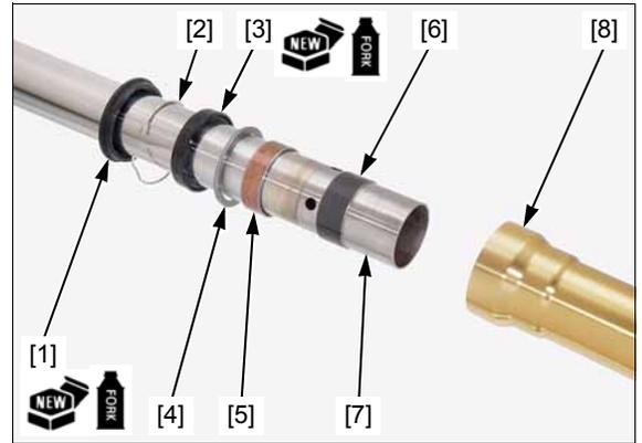
Put the guide bushing [1], back-up ring [2] and oil seal [3] on the outer pipe.
