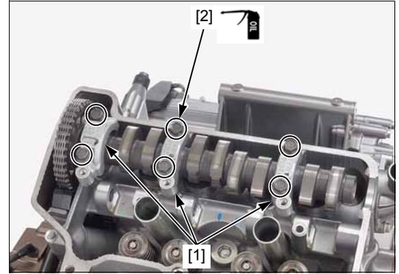
Remove the camshaft holders and measure the compressed plastigauge at its widest point on the camshaft to determine the oil clearance.
