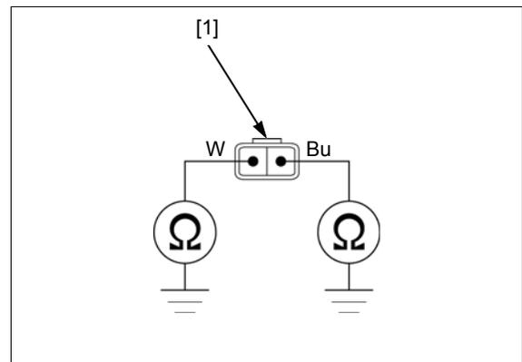
**2. Front Wheel Speed Sensor Line Short Circuit Inspection**
