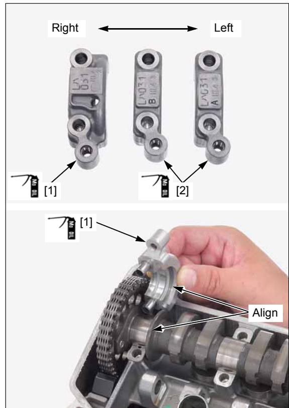
Apply engine oil to the camshaft holder bolt [1] threads and seating surfaces and install them.
