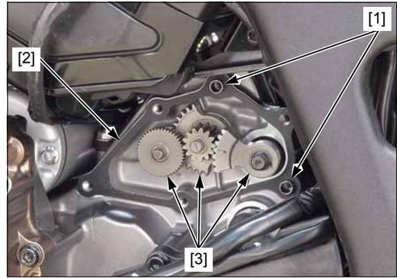
Check the bearings and replace if necessary.
