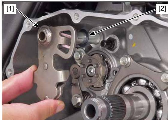
Remove the shift drum center bolt [1].
