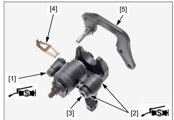
Tighten the parking brake caliper pin bolt [1] to the specified torque.
