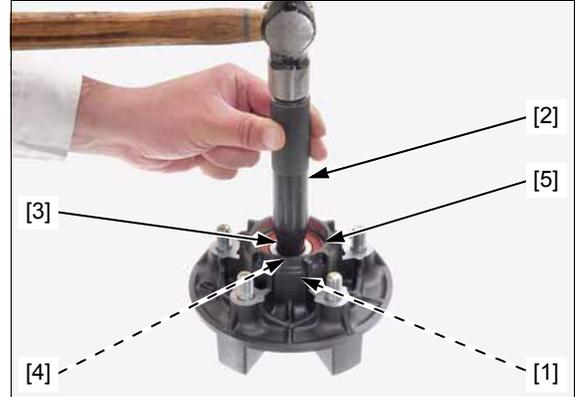
*Replace the wheel bearings in pairs. Do not reuse old bearings.*
