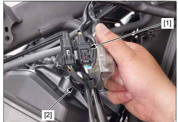
*CRF1000D:* Remove the bolts [1] and clutch EOP sensor cover [2].
