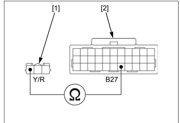
**5. TP Sensor Signal Line Open Circuit Inspection**
