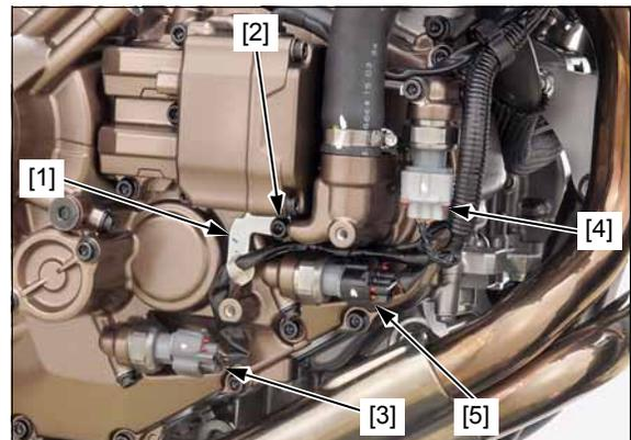
Install the clutch EOP sensor cover [1] and bolts [2] and tighten the bolts to the specified torque.
