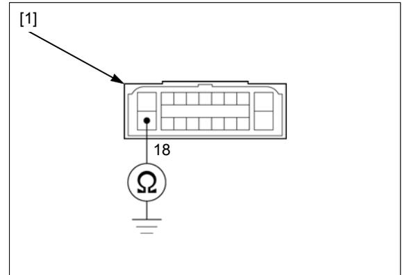
**3. Motor Power Input Line Open Circuit Inspection**
