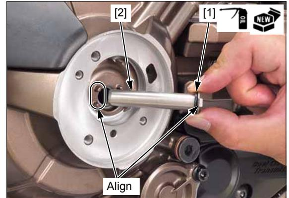
Apply engine oil to new O-rings [1] and install them to the feed pipe guide plate grooves.
