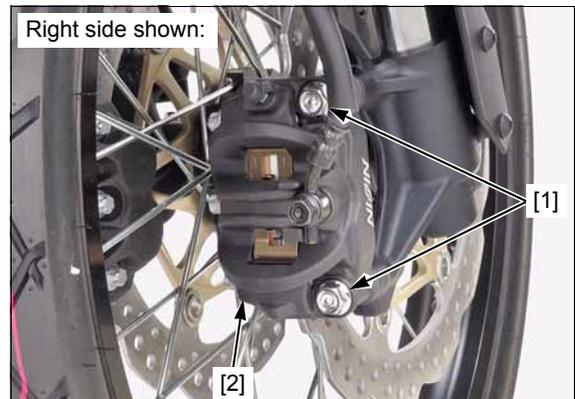
Remove the brake pads [1].
