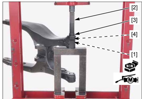
Install the snap ring [1] into the right pivot groove securely.
