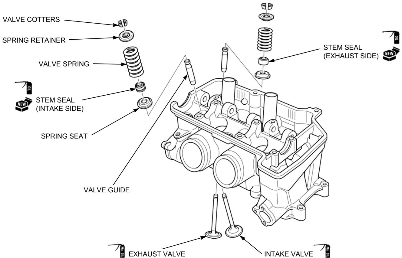
Blow through the oil passage in the cylinder head with compressed air.
