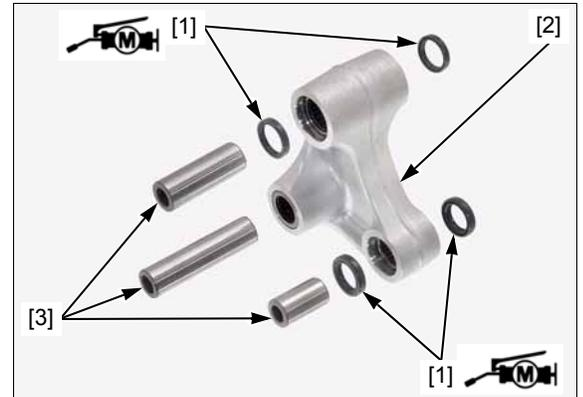
Install the collar [1] into the cushion connecting rod [2].
