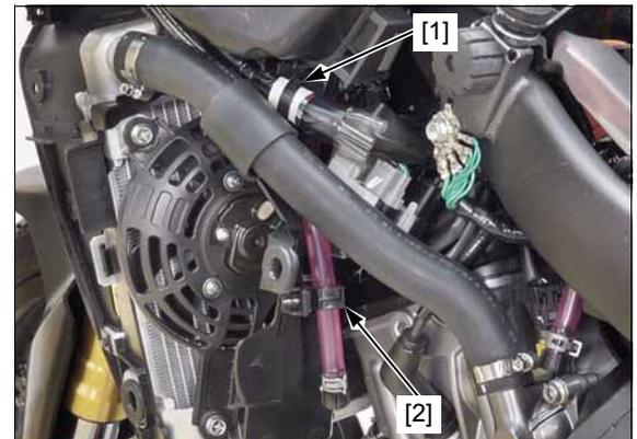
CRF1000D: Release the wire band [1] and clamp [2].
