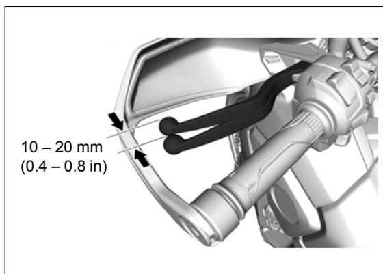
*The adjuster may be damaged if it is positioned too far out, leaving minimal thread engagement.* Minor adjustment is made with the upper adjuster at the clutch lever. Loosen the lock nut [1] and turn the adjuster [2].
