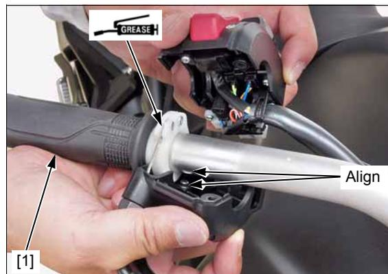
Tighten the upper screw/washer [1] first, then the lower screw/washer [2] to the specified torque.
