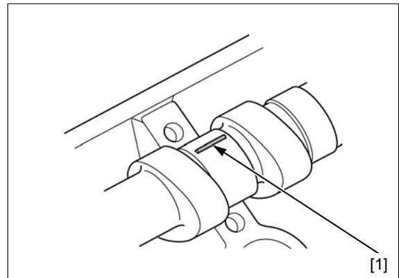
Install camshaft holders/dowel pins [1] in the correct locations, being careful not to drop the plastigauge.
