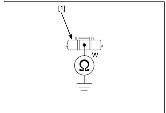
**DTC 83-2 (EOP SENSOR HIGH VOLTAGE)**
