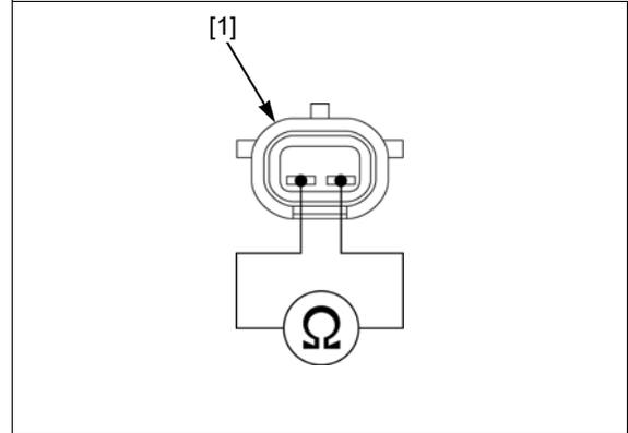
**4. Fuel Injector Signal Line Open Circuit Inspection**
