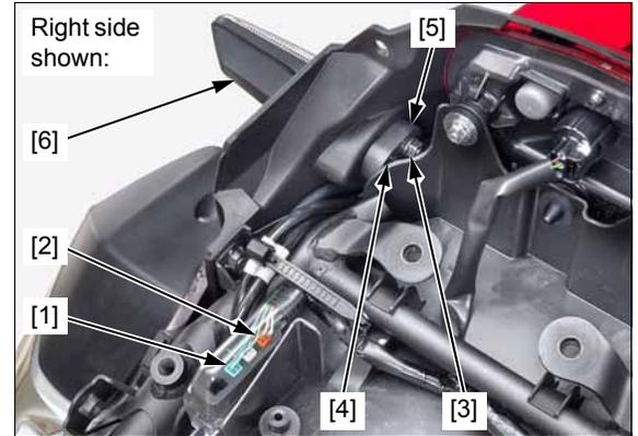
**TURN SIGNAL RELAY REMOVAL/ INSTALLATION**
