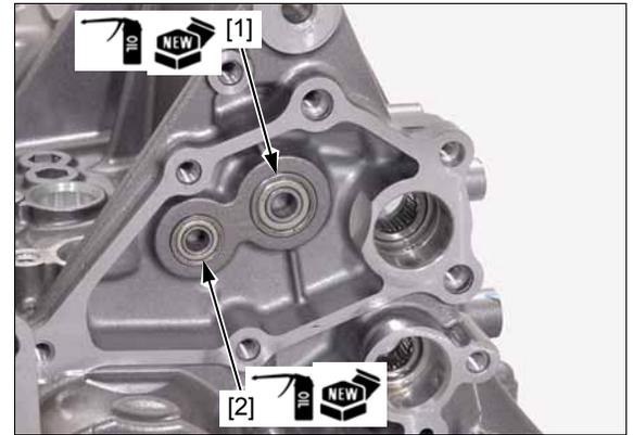
**GEARSHIFT SPINDLE NEEDLE BEARING (CRF1000D)**
