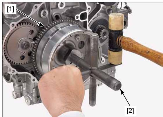
Remove the needle bearing [1].
