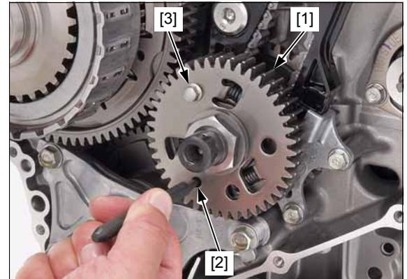
Remove the dual clutch assembly [1] from the mainshaft.
