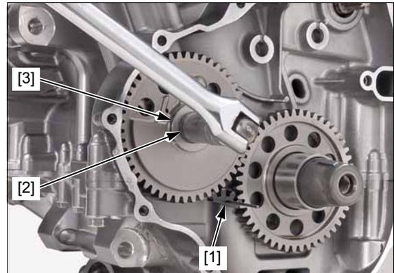
Line up the front balancer driven gear and sub gear teeth by inserting a suitable pin [1] into the holes of gears.
