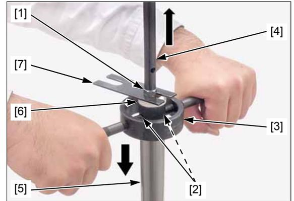
When installing the fork bolt assembly [1], turn the rebound adjuster [2] counterclockwise to the softest position.
