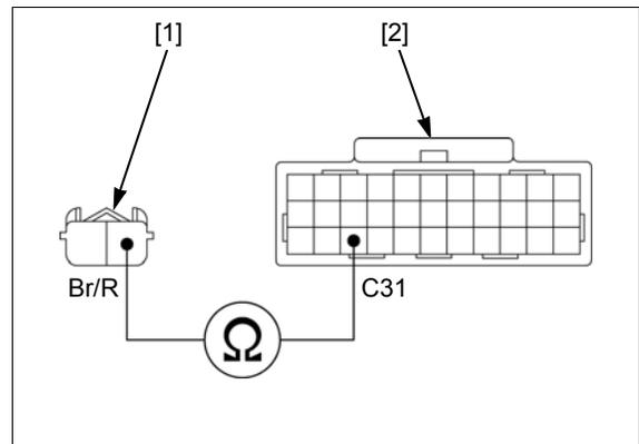
**4. IAT Sensor Ground Line Open Circuit Inspection**
