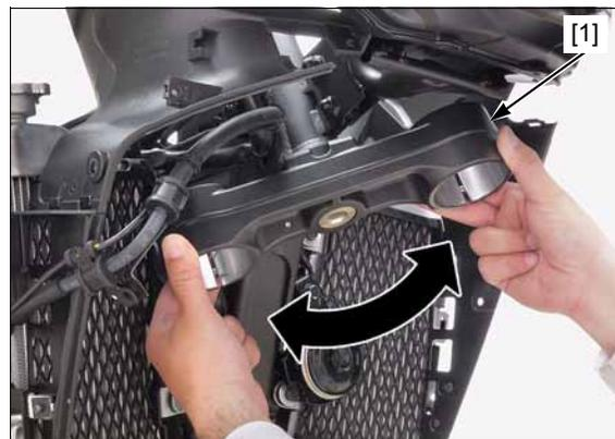
Retighten the steering stem adjusting nut [1] to the specified torque using a special tool.
