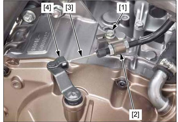
*CRF1000D:* Disconnect linear solenoid 4P (Black) connector [1].
