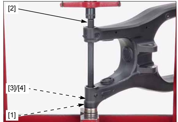
Remove the needle bearing (24 x 31 x 28 mm) [1] out of the right pivot using the special tool.
