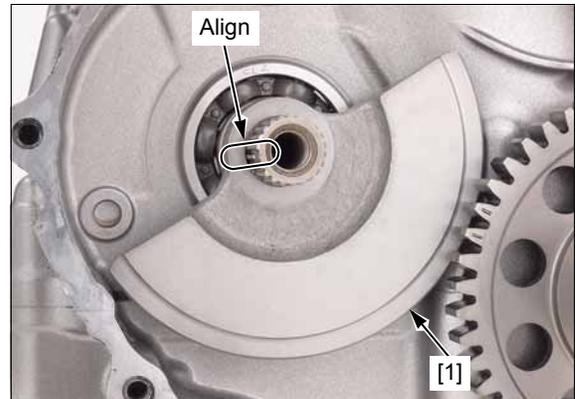
Apply molybdenum oil solution to the front balancer driven gear sliding area and thrust surface.
