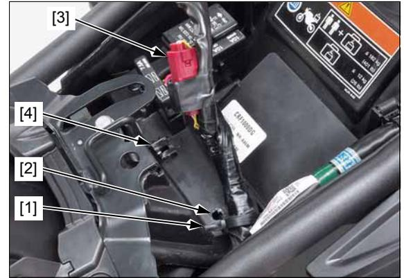
Connect the special tools to the wire harness side 2P (Red) connector.
