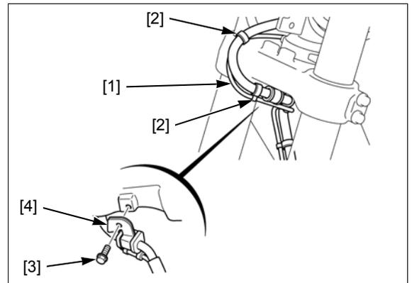
Remove the bolt [1] and front wheel speed sensor [2].
