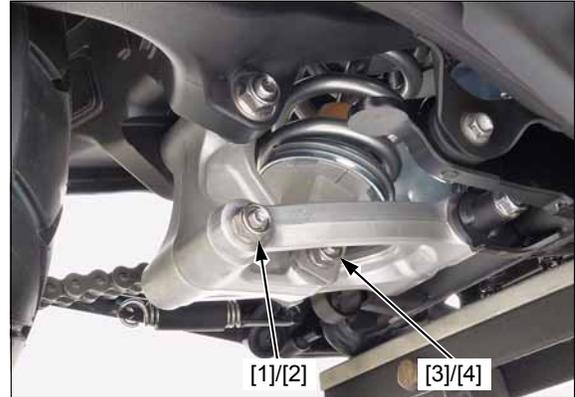
Remove the shock absorber upper mounting bolt [1] and nut [2].
