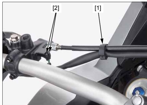
*CRF1000D:* Remove the wire clamp [1] and disconnect the parking brake switch connectors [2].
