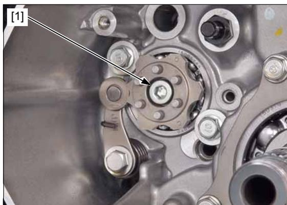
Remove the shift drum center [1] while holding the stopper arm [2] using a screwdriver as shown.
