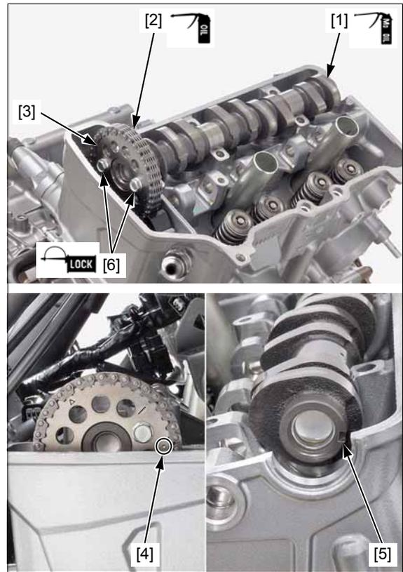
Apply molybdenum oil solution to the camshaft holders inside and install them in their original locations.
