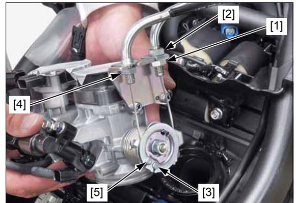
Loosen the throttle cable B lock nut [4] then disconnect the throttle cable B [5] from the throttle drum and cable stay.
