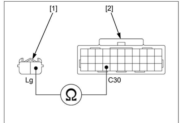
**4. ECT Sensor Ground Line Open Circuit Inspection**
