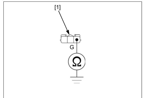
**3. VS Sensor Input Line Open Circuit Inspection**
