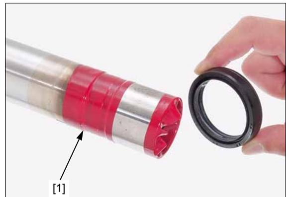
Apply fork fluid to new dust seal and oil seal lips.
