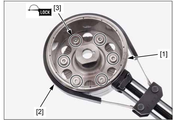
Install the starter driven gear [1] into the starter clutch outer while turning the starter driven gear counterclockwise.
