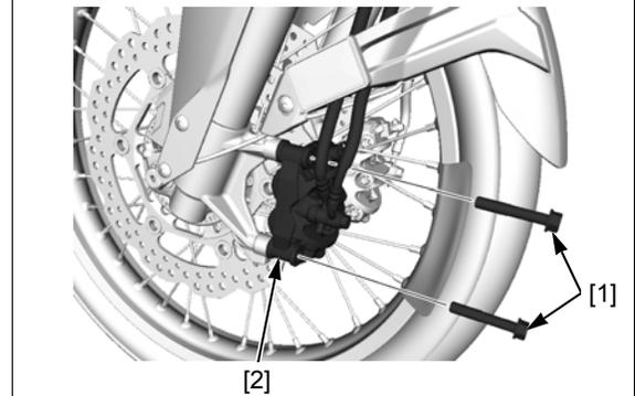
ED model: Remove the axle cap [1].
