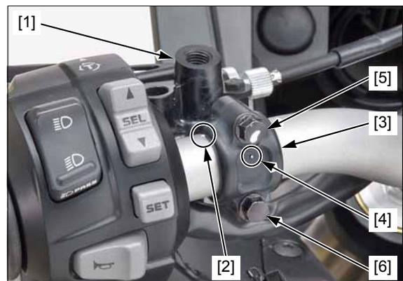
*CRF1000A:* Install the wire clamp [1] and connect the clutch switch connectors [2].
