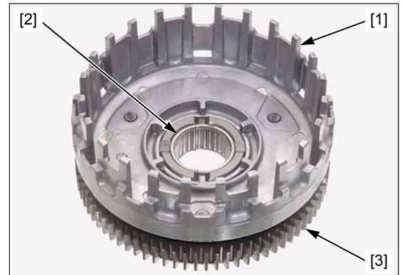
Inspect the following parts for scratch, damage, abnormal wear and deformation. Replace if necessary.
