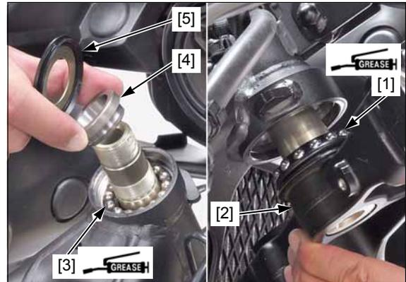
Apply 0.10 – 0.30 g (0.004 – 0.011 oz) of urea based multi-purpose extreme pressure grease NLGI #2 (EXCELITE EP2 manufactured by KYODO YUSHI CO., LTD. or equivalent) to the steering stem adjusting nut [1] threads.
