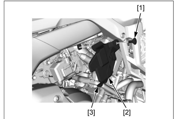
Release the starter relay switch [1] from the battery box.
