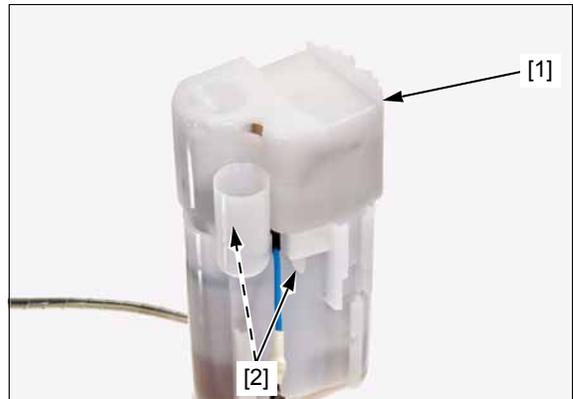
Remove the fuel pump [1] and O-ring [2].
