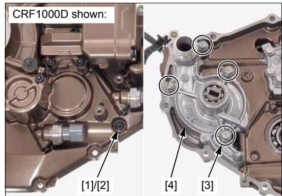
Install a new O-ring [1] into the groove in the water pump body [2].
