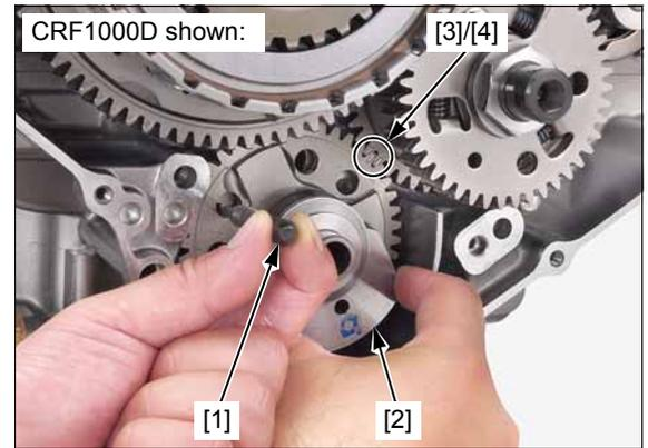
Install the dowel pins [1].
