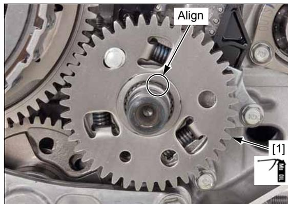
Apply engine oil to the primary drive gear nut threads and seating surface.
