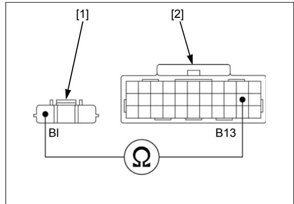
**4. EOP Sensor Output Line Open Circuit Inspection**
