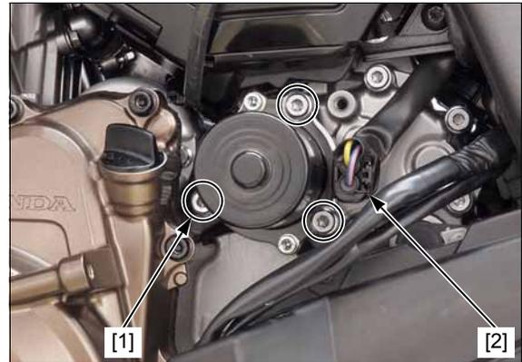
Install the shift control motor cover [1] and bolts [2] and tighten the bolts to the specified torque.
