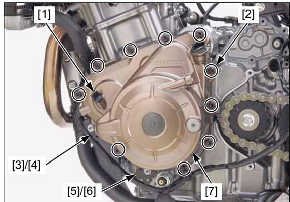
Remove the dowel pins [1] and oil joint [2].
