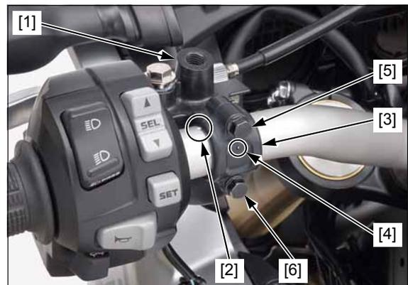
*CRF1000D:* Install the parking brake lever assembly [1] by aligning its end with the paint mark [2] on the handlebar. Install the holder [3] with its punch mark [4] facing up. Tighten the upper bolt [5] first, then the lower bolt [6].
