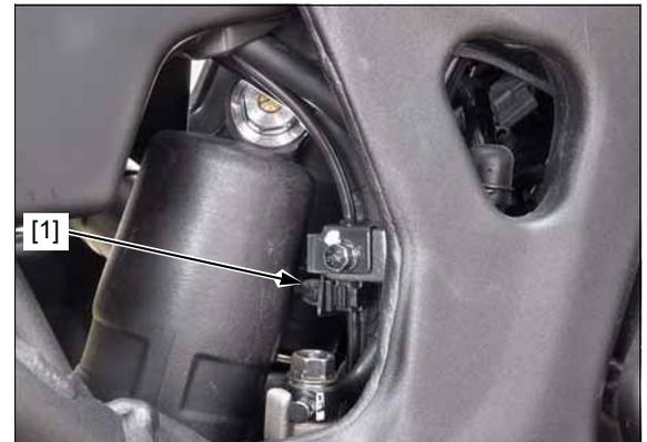
Install the rear brake hose B [1] and rear wheel speed sensor 2P (Black) connector [2] through the hole [3] of rear fender B.
