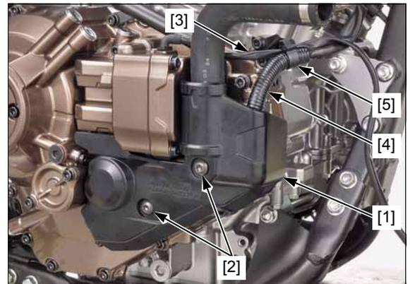
CRF1000D: Connect linear solenoid 4P (Black) connector [1].
