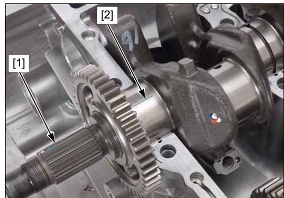
Install the dowel pins [1].
