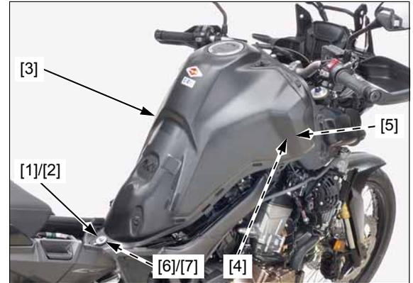
Check the fuel line [1] for deterioration, damage or leakage. Replace the fuel line if necessary.
