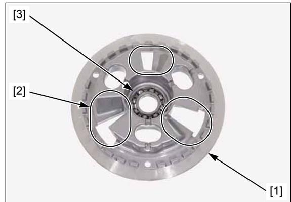
Check the following of the clutch center [1] for scratch, damage, abnormal wear and deformation.
