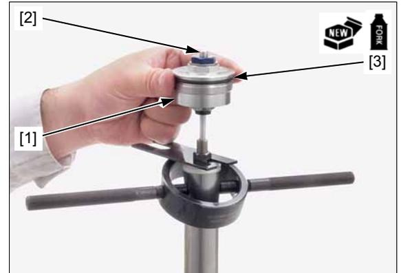
*Be careful not to damage the fork bolt when tightening it.*
