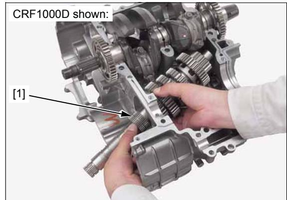
Apply engine oil to the right mainshaft bearing [1].
