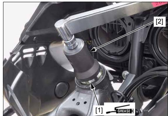
Move the steering stem [1] right and left, lock-to-lock, five times to seat the bearings.
