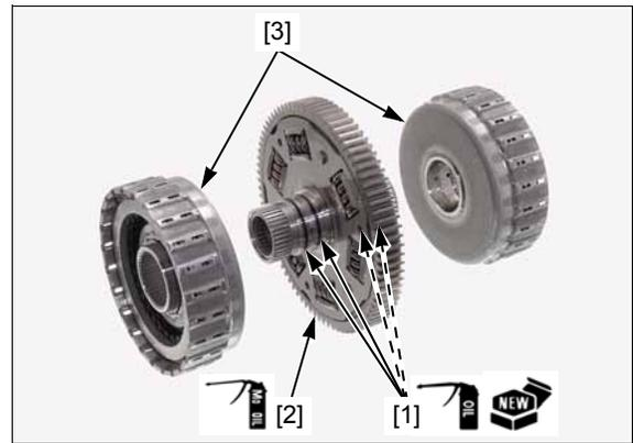
Apply engine oil to the needle bearings in the primary driven gear.
