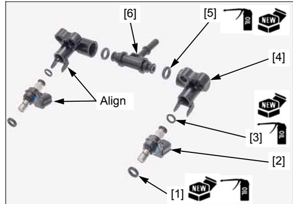
Install the fuel injector assembly [1].
