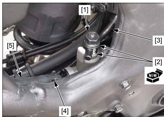
Remove the cotter pin [1] and joint pin [2], and disconnect the brake rod joint [3] from the middle arm [4].
