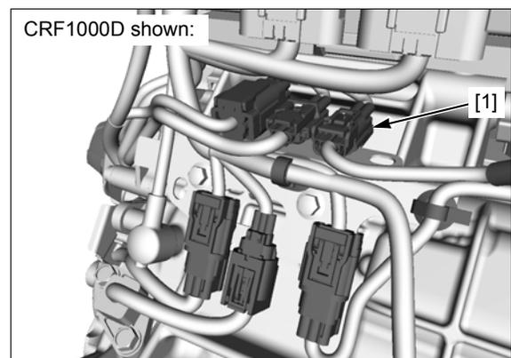
Check for continuity between the rear brake light switch 2P (Gray) connector [1] terminals.
