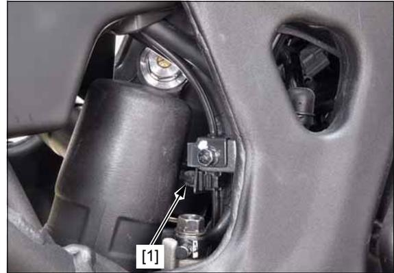
CRF1000A/D: Remove the oil bolt [1], rear brake hose A [2], and sealing washers [3].
