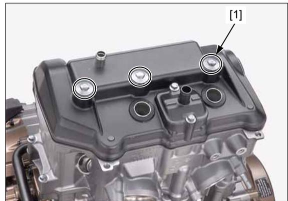
Remove the cylinder head cover [1] to the right side as shown.
