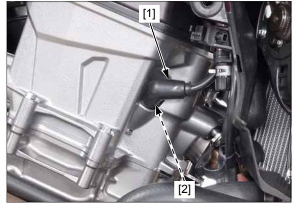
Remove the spark plug cap [1].
