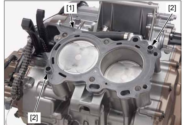
Remove the cam chain guide [1].
