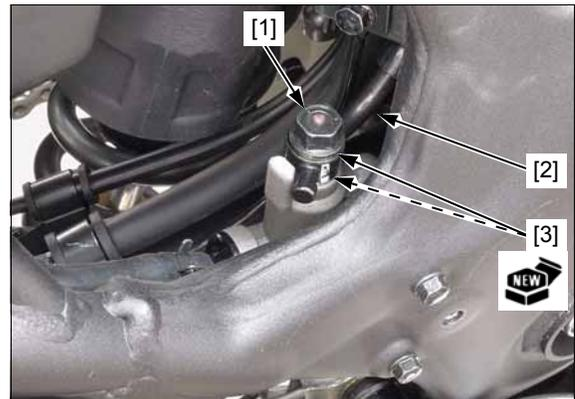
CRF1000A/D: Disconnect the rear brake hose B [1] from the ABS modulator by removing the oil bolt [2] and sealing washers [3].
