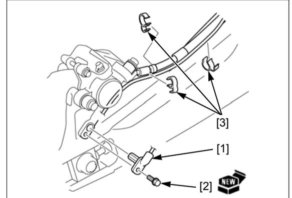
Clamp the sensor wire [1] with the brake hose clamps.
