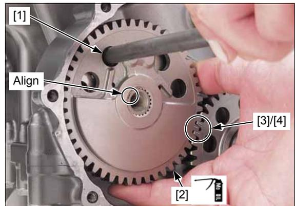
Install the special tool between the front balancer drive and driven gears.
