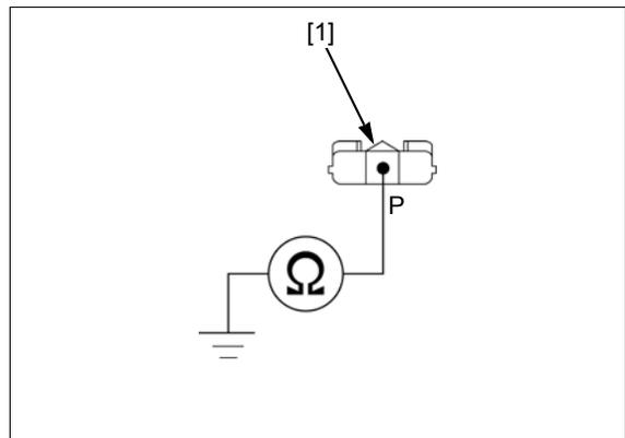
**5. VS Sensor Signal Line Open Circuit Inspection**
