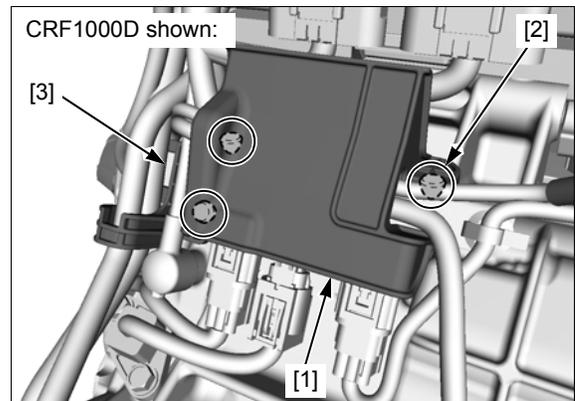
Disconnect the Alternator assembly 6P (Black) connector [1].
