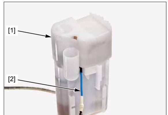
Install a new O-ring [1] to the fuel pump stay [2].
