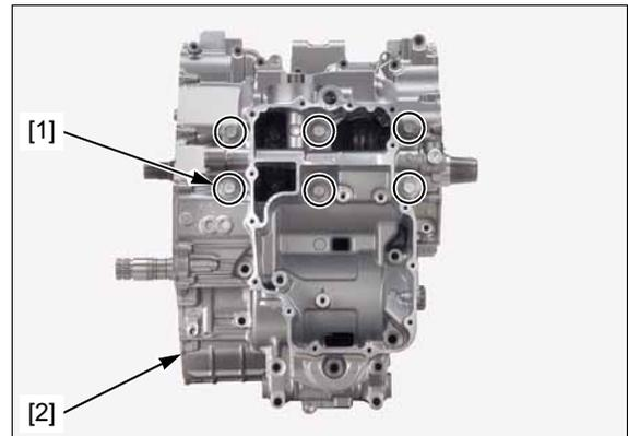
Remove the dowel pins [1], oil joint A [2], and oil joint B [3].
