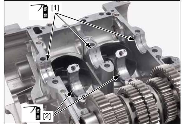
Apply molybdenum oil solution to the thrust surfaces of the crankshaft as shown.
