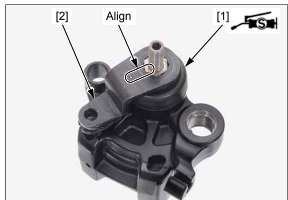
Install the adjuster lock nut [1].
