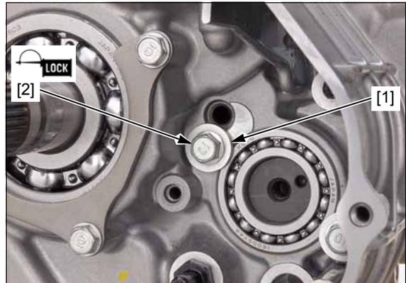
**CRF1000D:** Apply locking agent to the shift drum bearing setting bolt threads (page 1-20).
