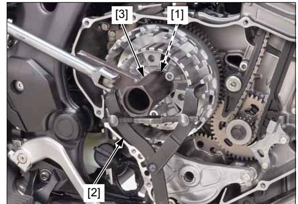
Remove the lock washer [1], washer [2], and clutch center [3].
