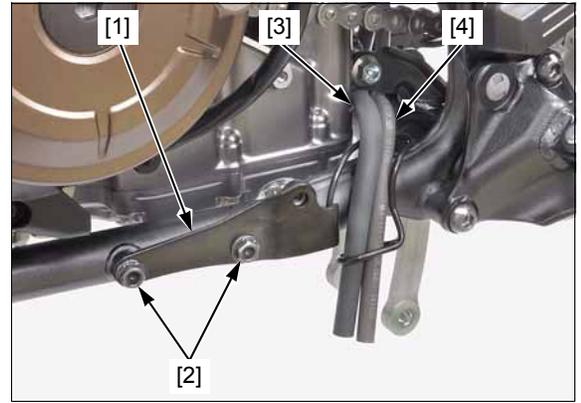
Install the connector clip stay [1] and bolts [2], and tighten the bolts securely.
