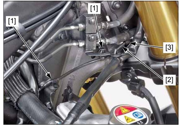
Release the sensor wire [1] from the clamps [2].
