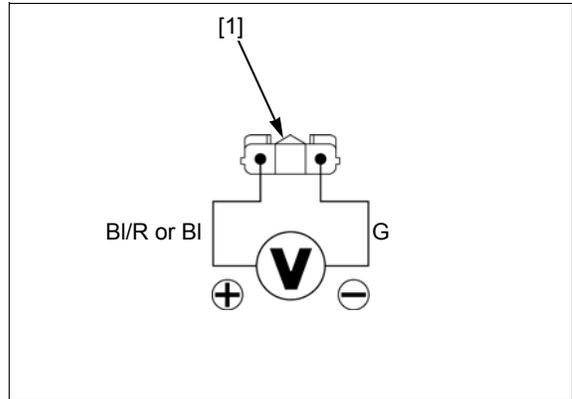
**4. VS Sensor Signal Line Short Circuit Inspection**
