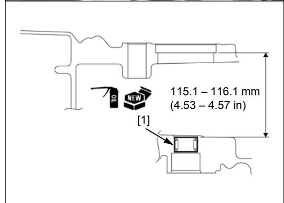
**SHIFT CONTROL MOTOR REDUCTION GEAR BEARING (CRF1000D)**
