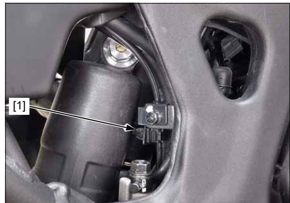
Remove the bolt [1] and release the sensor wire [2] from the brake hose clamp [3].
