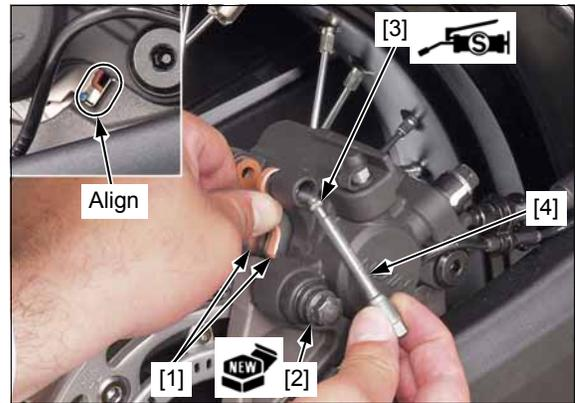
Tighten the rear brake caliper mounting bolt [1] to the specified torque.
