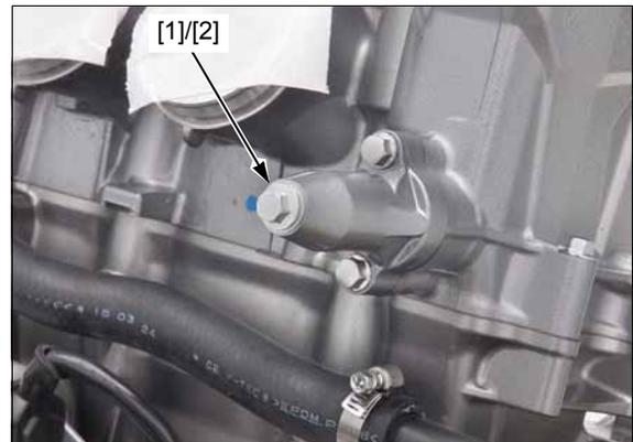
Turn the cam chain tensioner lifter shaft fully in (clockwise) and secure it using the special tool.
