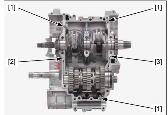
Apply molybdenum oil solution to the main journal bearing sliding surfaces on the lower crankcase.
