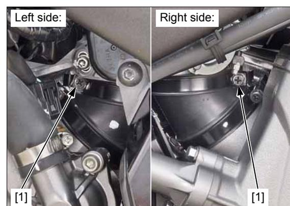
Disconnect the ignition coil wire sub harness 6P (Black) connector [1].
