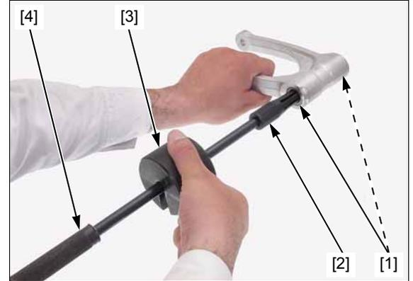
*Never install the old bearing, once the bearing has been removed, the bearing must be replaced with a new one.*
