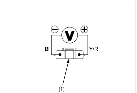
**4. EOP Sensor Output Line Short Circuit Inspection**
