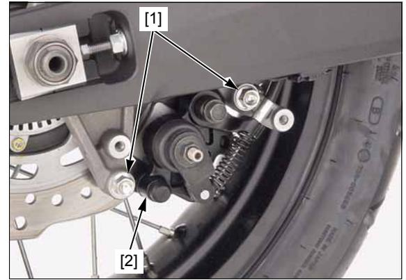
Remove the pad pins [1] and pads [2].
