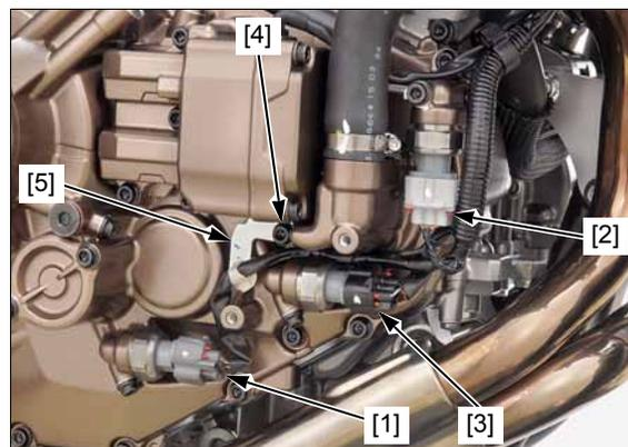
Release the linear solenoid valve wire [1] and main wire harness [2] from the clamps [3].
