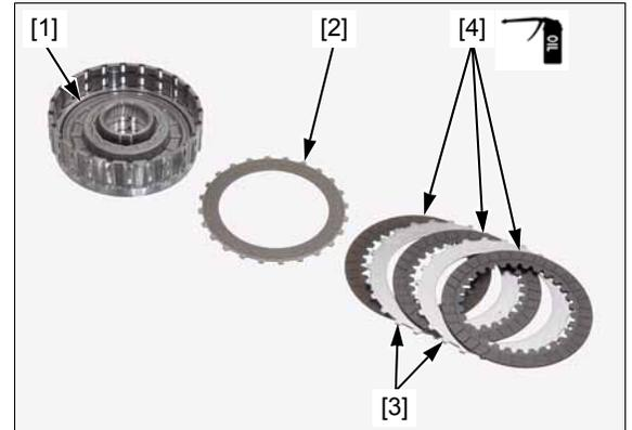
Install end plate [1] with the marking side facing out.
