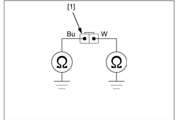
**3. Front Wheel Speed Sensor Line Open Circuit Inspection**
