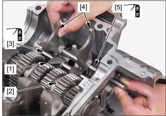
**CRF1000/A:** Apply locking agent to the shift drum bearing setting bolt threads (page 1-20).
