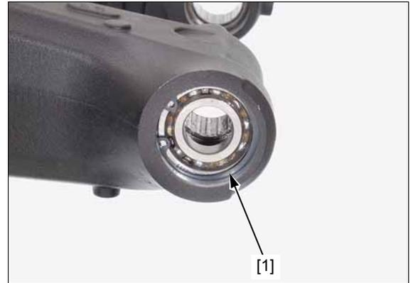
Remove the ball bearing 6003 [1] out of the right pivot using a hydraulic press and special tool.
