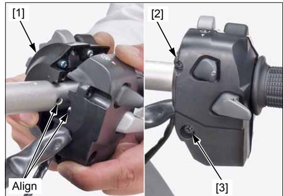
*CRF1000/A:* Install the clutch lever assembly [1] by aligning its end with the paint mark [2] on the handlebar. Install the holder [3] with its punch mark [4] facing up. Tighten the upper bolt [5] first, then the lower bolt [6].
