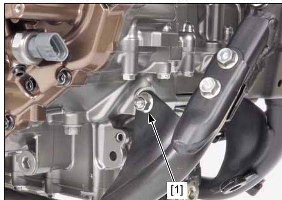
Tighten the front middle nuts (8 mm) [1] to the specified torque.
