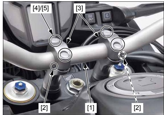
Install the left handlebar switch housing [1] by aligning its locating pin with the hole in the handlebar.
