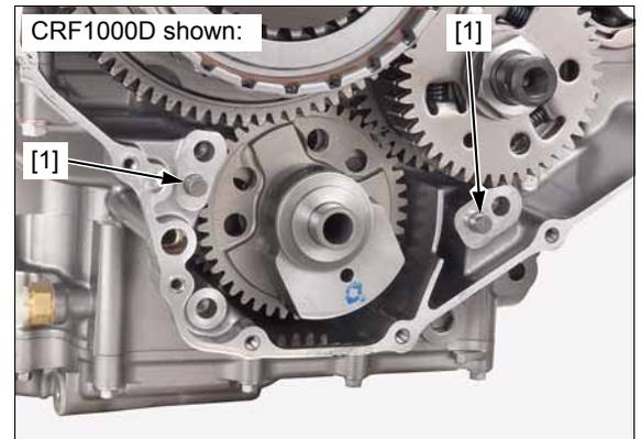
Line up the rear balancer driven gear and sub gear teeth by inserting a suitable pin [1] into the holes of gears.
