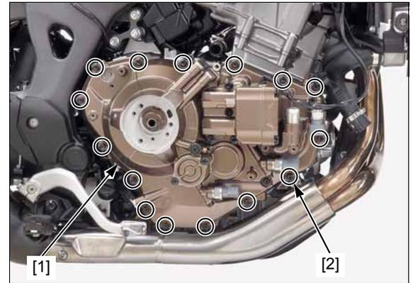
Coat a new O-ring [1] with engine oil and install it onto the water pipe [2].
