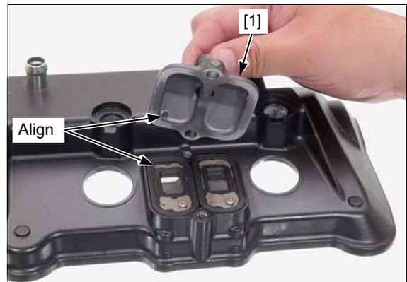
Remove the PAIR reed valves [1] and port plates [2].
