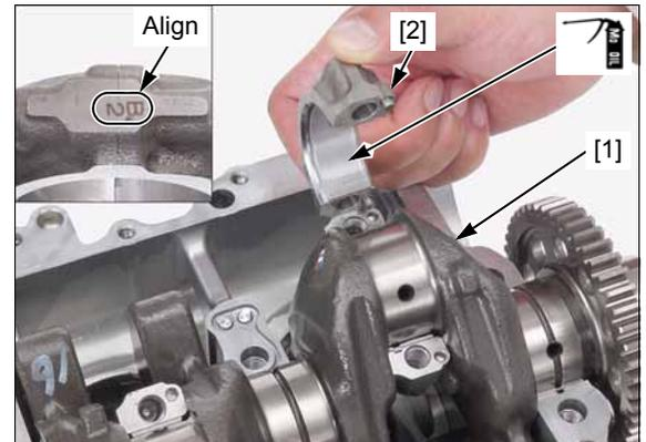
Apply engine oil to new crankpin bearing cap bolt threads and seating surfaces.
