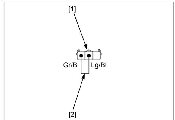
**4. MAP Sensor Signal Line Open Circuit Inspection**
