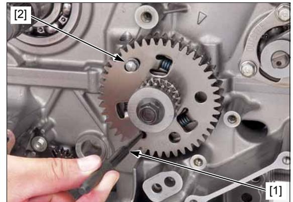
Temporarily install the clutch outer [1].
