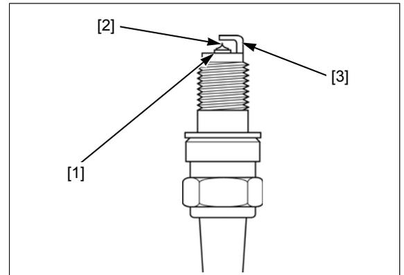
*To prevent damaging the iridium center electrode, use a wire type feeler gauge to check the spark plug gap.*
