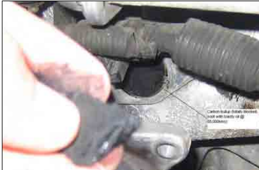
In case you can not read the text it states; “Carbon buildup (totally blocked, soot with toasty oil @ 85,000 klms)”
