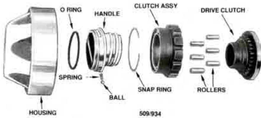
Manual free wheeling hub components.
