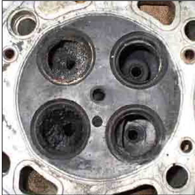
A picture of a cylinder head from a forum member (GUHOON) notice how carboned up the two left ports are.
