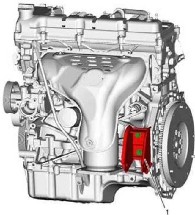
Fig. 162: Removing Engine Front Mounting Bracket Courtesy of SUZUKI OF AMERICA CORP.
