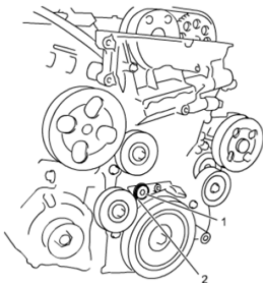
Fig. 32: Removing Timing Chain Cover Plug And Gasket Courtesy of SUZUKI OF AMERICA CORP.
