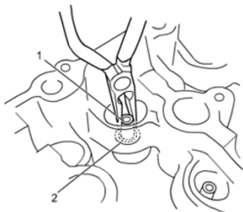
Fig. 113: Removing Valve Stem Seal And Valve Spring Seat Courtesy of SUZUKI OF AMERICA CORP.
