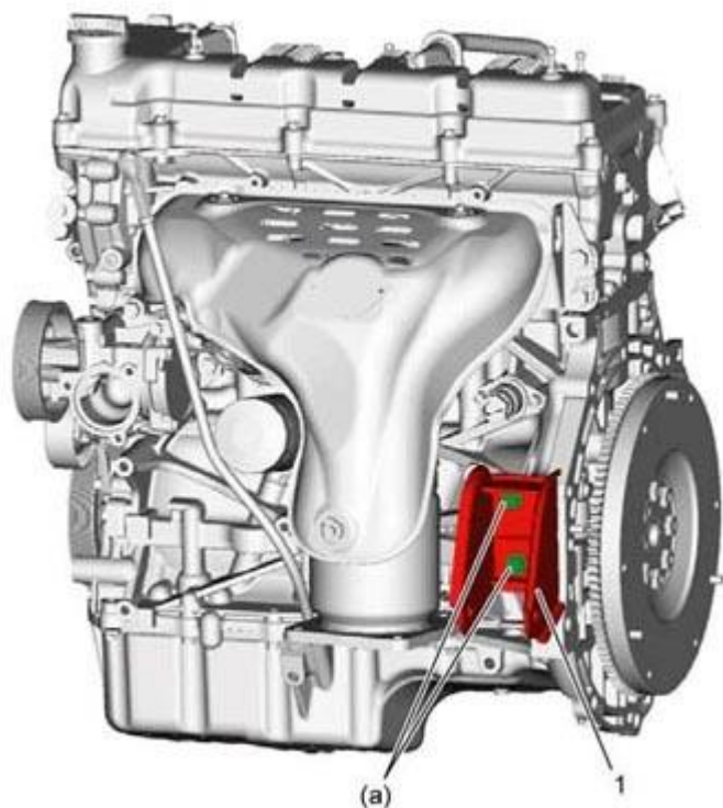
Fig. 176: Identifying Engine Front Mounting Bracket Bolt Courtesy of SUZUKI OF AMERICA CORP.
