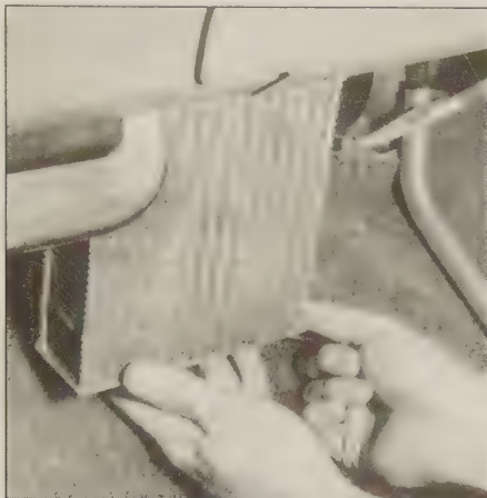
13.9 Pull the heater core to the rear and down to remove it from the plenum
