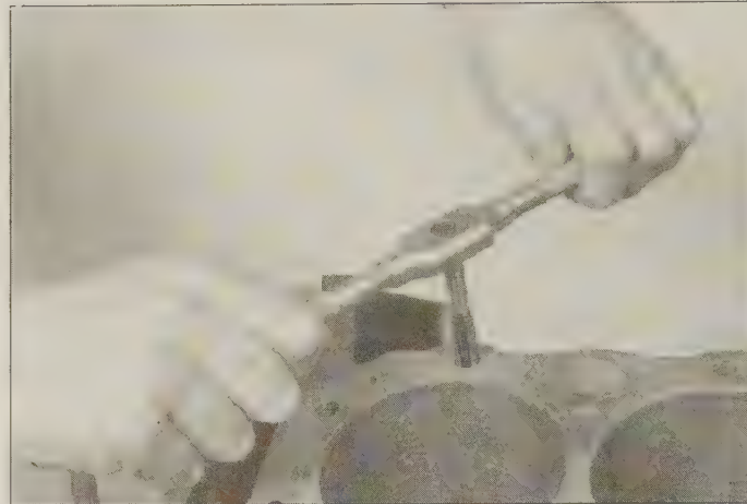
14.8 All bolt holes in the block - particularly the main bearing cap and head bolt holes - should be cleaned and restored with a tap (be sure to remove debris from the holes after this is done)
