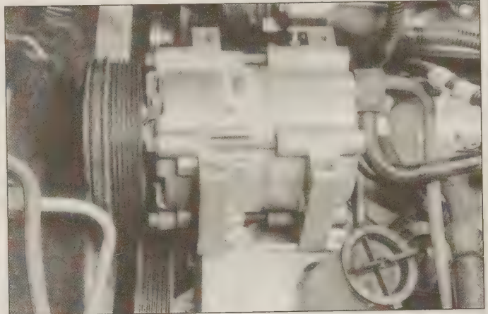
4.12 Disconnect the compressor electrical connector from the back of the compressor, then remove the mounting bolts and shift the compressor forward as shown - DO NOT disconnect any refrigerant lines
