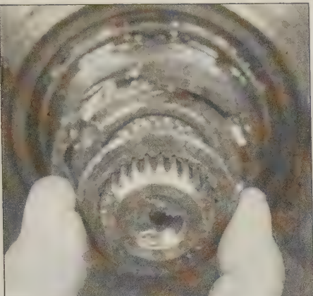
28.26 Remove the axle shaft spacer
