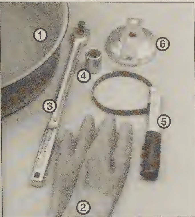
6.2 These tools are required when changing the engine oil and filter
