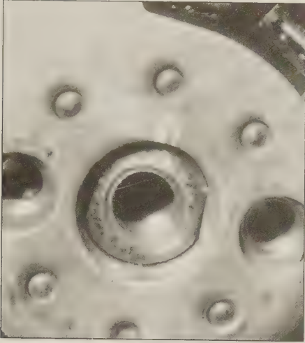
20.6 There should be factory alignment marks on the steering wheel and shaft; if not, make your own
