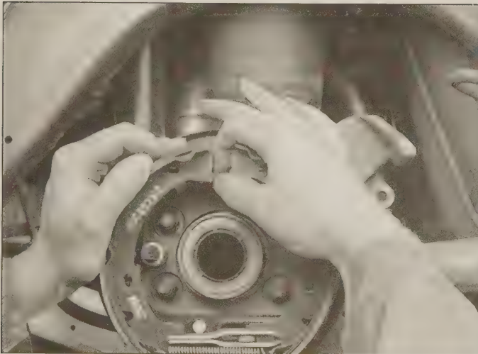
13.5d Detach the upper return spring from the parking brake shoes (it's in the back)
