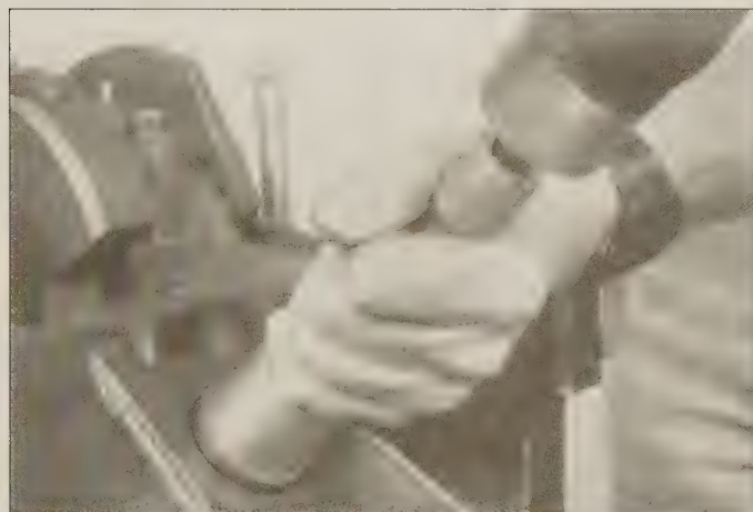
14.10 A large socket on an extension can be used to drive the new core plugs into the bores
