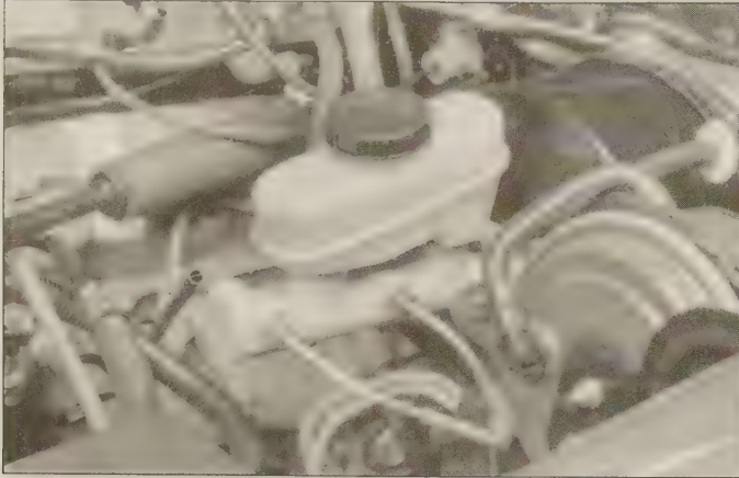
3.16 Check the brake fluid level by looking through the translucent plastic reservoir
