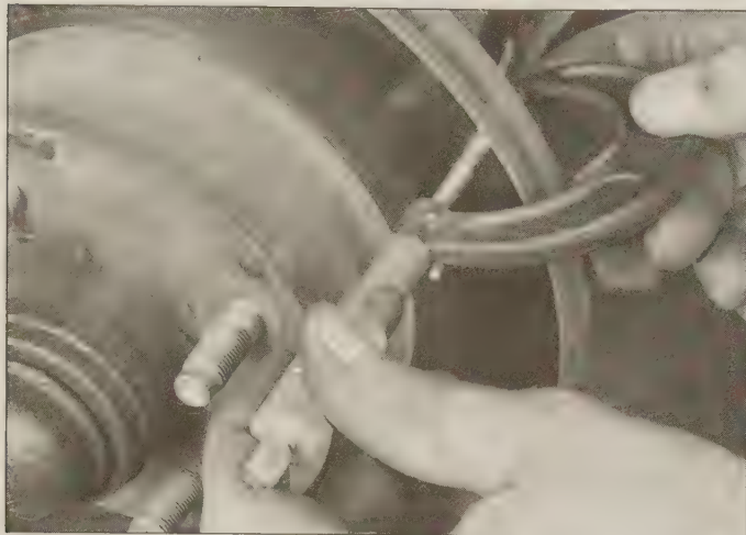
5.6b Use a micrometer to measure disc thickness at several points, about 1/2-inch from the edge
