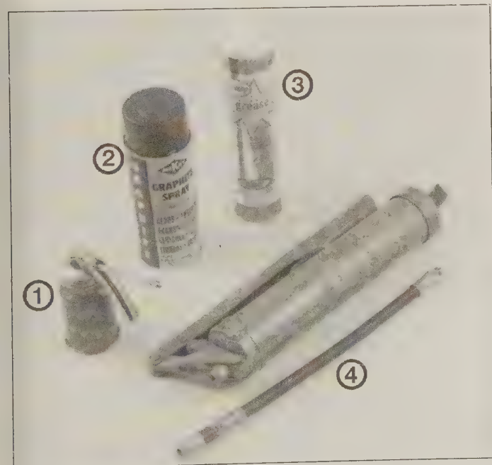
15.1 Materials required for chassis and body lubrication
