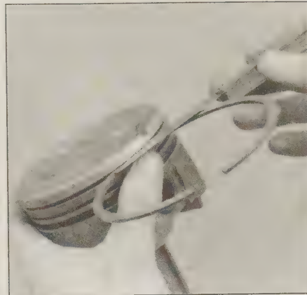
17.10 Check the ring side clearance with a feeler gauge at several points around the groove
