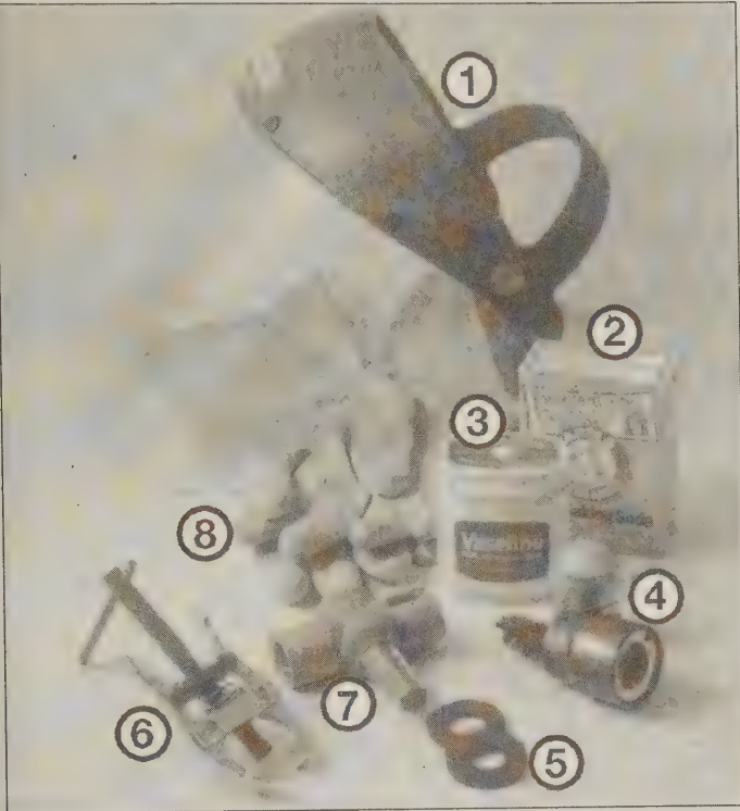
12.1 Tools and materials required for battery maintenance
