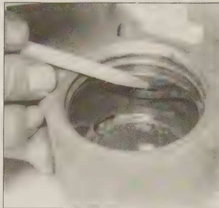
4.7 To remove the seal from the caliper bore, use a plastic or wooden tool, such as a pencil
