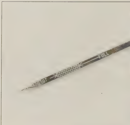
3.4b The oil level should appear between the ADD 1 QT and SAFE marks; don't overfill the crankcase
