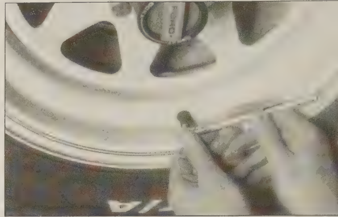
4.8 To extend the life of the tires, check the air pressure at least once a week with an accurate gauge (don't forget the spare!)
