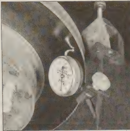
5.5a To check disc runout, mount a dial indicator as shown and rotate the disc
