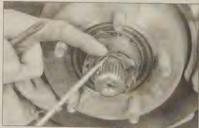
28.25b The snap-ring can be lifted off with a screwdriver if snap-ring pliers aren't available - hold the center of the snap-ring with a finger as shown so it doesn't fly off
