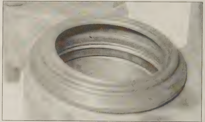
4.18 Install the dust boot in the upper groove in the caliper bore, making sure it's completely seated
