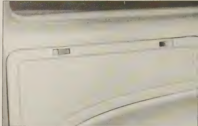
3.23a To check the rear windshield washer fluid level, lift the tabs and remove the access panel in the luggage compartment . . .
