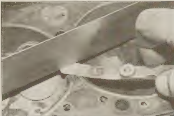
9.12a Check the cylinder head gasket surface for warpage by trying to slip a feeler gauge under the straightedge (see this Chapter's Specifications for the maximum warpage allowed and use a feeler gauge of that thickness)
