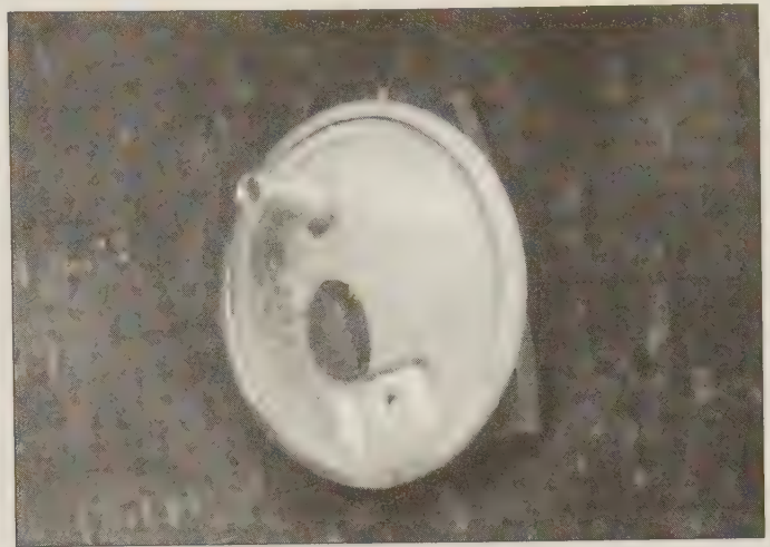
5.21 The bimetal sensor is mounted inside the air cleaner housing
