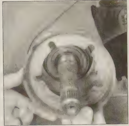
21.6 Take the spindle seat off
