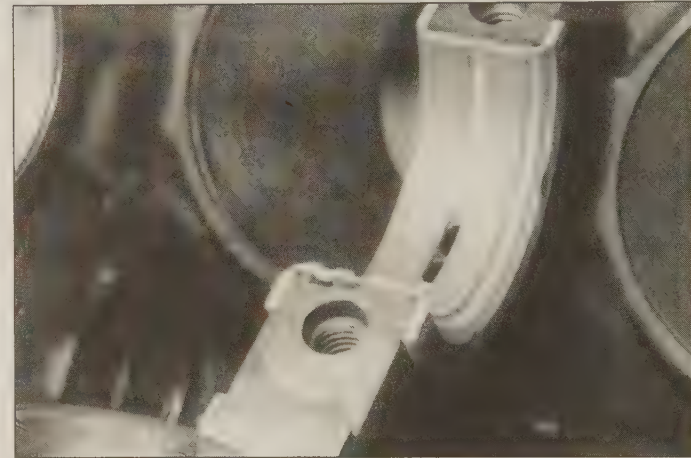
22.5 The upper main bearing in position (flanged thrust bearing shown) - the oil hole in the bearing must align with the oil hole(s) in the block
