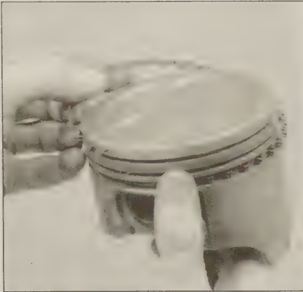
21.9a Installing the spacer/expander in the oil control ring groove
