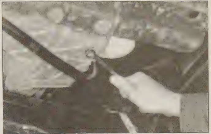
6.7 Remove the oil pan drain plug with a box-end wrench or socket - an open-end or adjustable wrench shouldn't be used, since it may round off the corners of the drain plug
