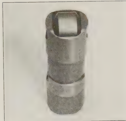
12.8b The roller on roller lifters must turn freely - check for wear and excessive play as well
