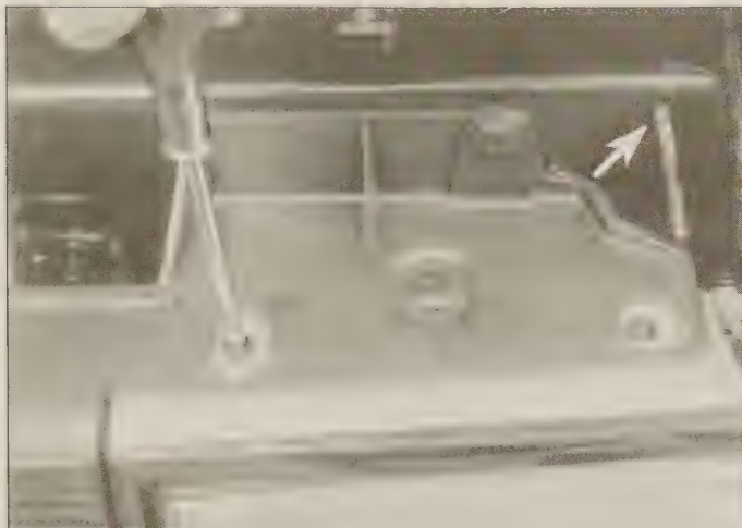
17.2 Remove two screws that secure the top of the lamp housing (the screw indicated by the arrow is the headlight adjustment screw that affects the vertical position of the headlight beam)
