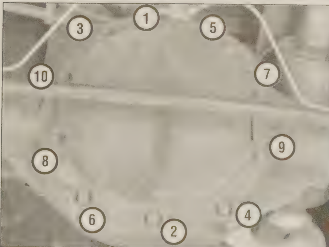
17.12 Tighten the cover bolts in a criss-cross pattern - don't overtighten the bolts, or the cover may be distorted, causing it to leak
