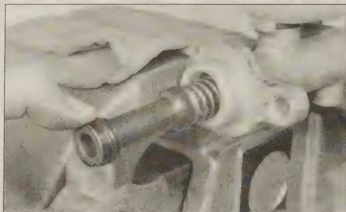
8.8 Remove the primary piston assembly from the cylinder
