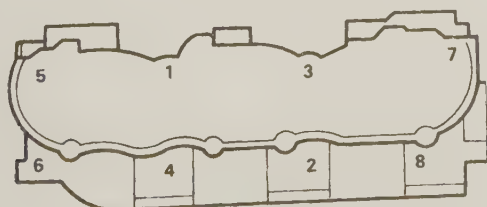
9.23 Cylinder head tightening sequence
