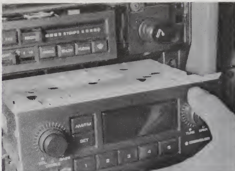
11.4a Pull the radio out, support it and . . .
