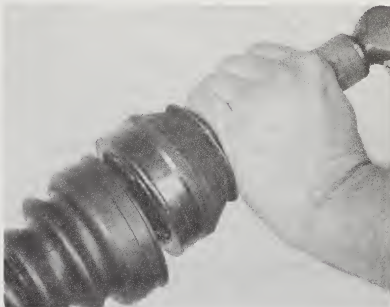
19.45 Strike the end of the housing shaft with a soft-faced hammer to engage it with the shaft circlip
