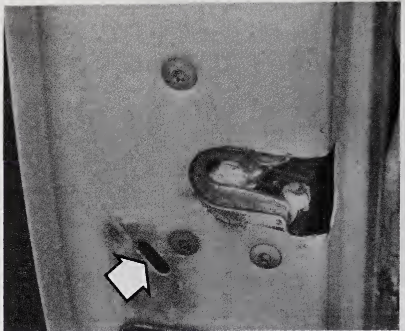
11.4 Insert a screwdriver through the access hole (arrow) to adjust the linkage
