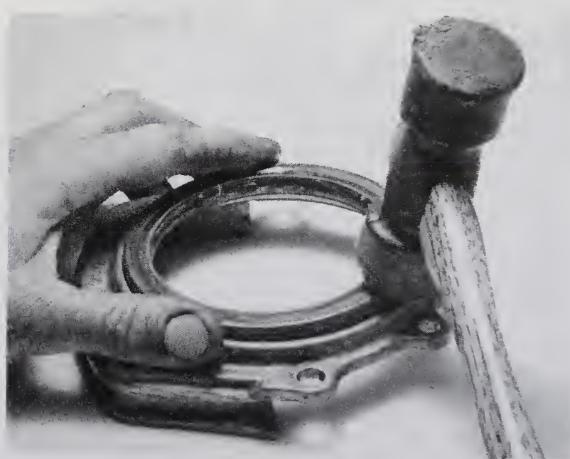
13.6 Tap the new rear oil seal squarely into place with a soft-face hammer
