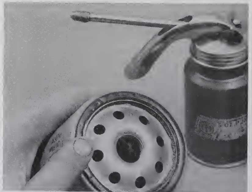
12.18 Lubricate the gasket with clean oil before installing the filter on the engine
