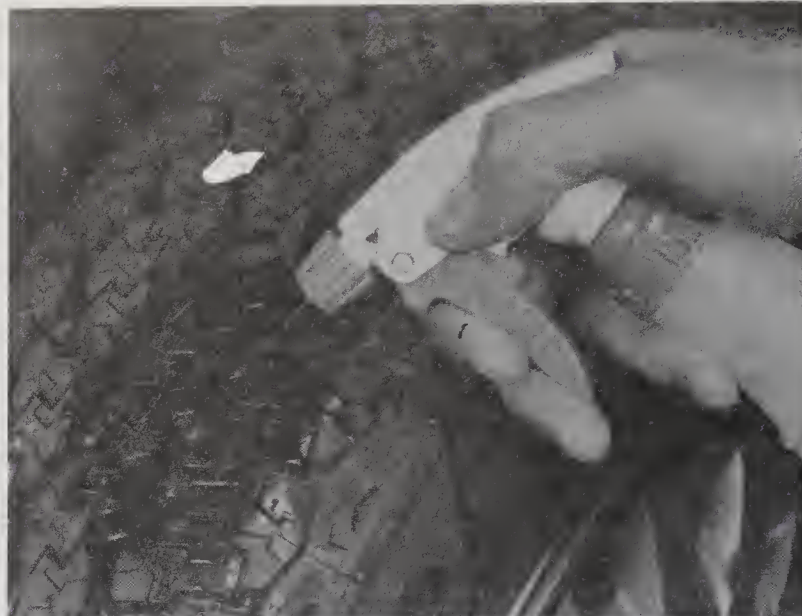
5.4b If the valve core is tight, raise the corner of the vehicle with the low tire and spray a soapy water solution onto the tread as the tire is turned – slow leaks will cause small bubbles to appear
