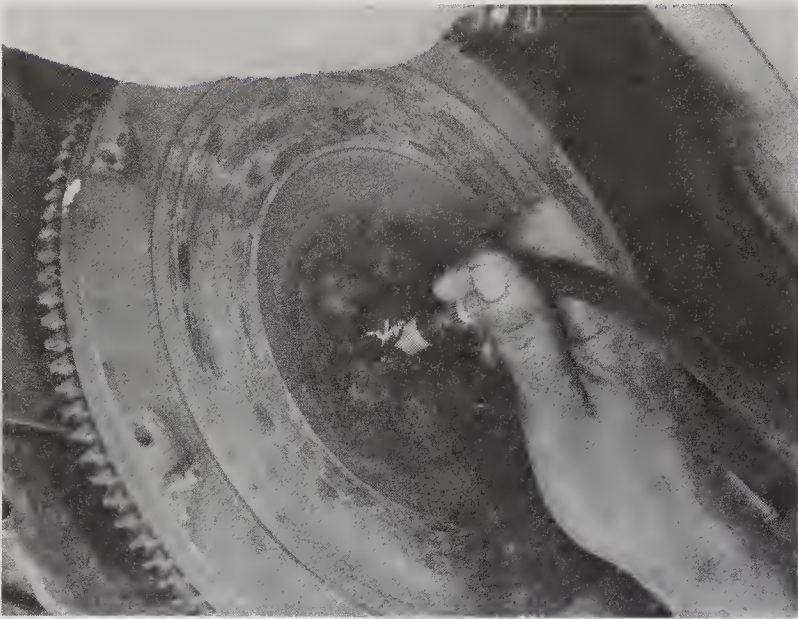
6.8 Fill the cavity behind the pilot bushing with grease . . .
