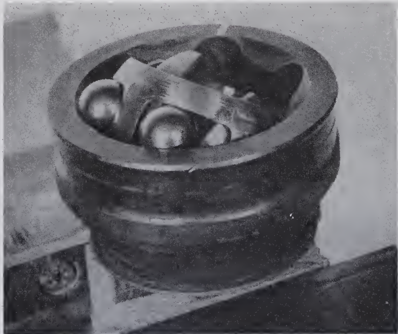
19.31 With the cage and cross tilted, the balls can be removed one at a time
