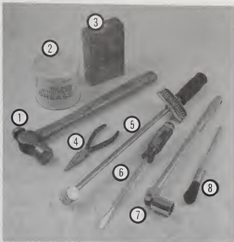
33.1 Tools and materials needed for front wheel bearing maintenance
