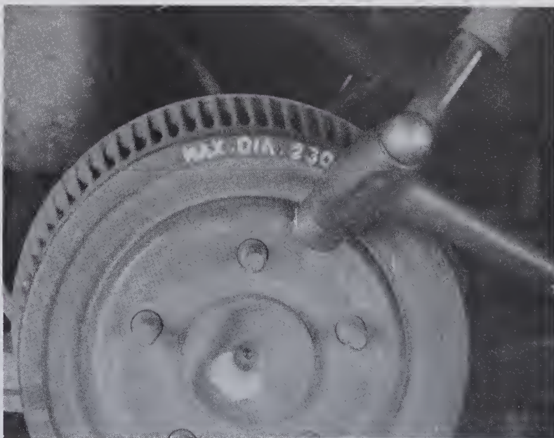
5.4a If the brake drum cannot be easily pulled off, apply some penetrating oil at the hub-to-drum joint and allow it to soak in, lightly tap the drum to break it loose . . .
