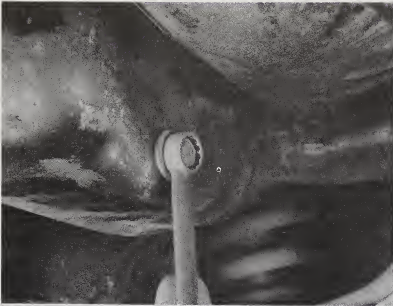
12.9 The oil drain plug is located at the bottom of the pan and should be removed with a socket or box-end wrench – DO NOT use an open-end wrench (the corners on the hex can be easily rounded off)
