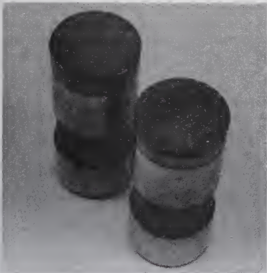
10.18c If the lifters are pitted or rough, they shouldn't be reused
