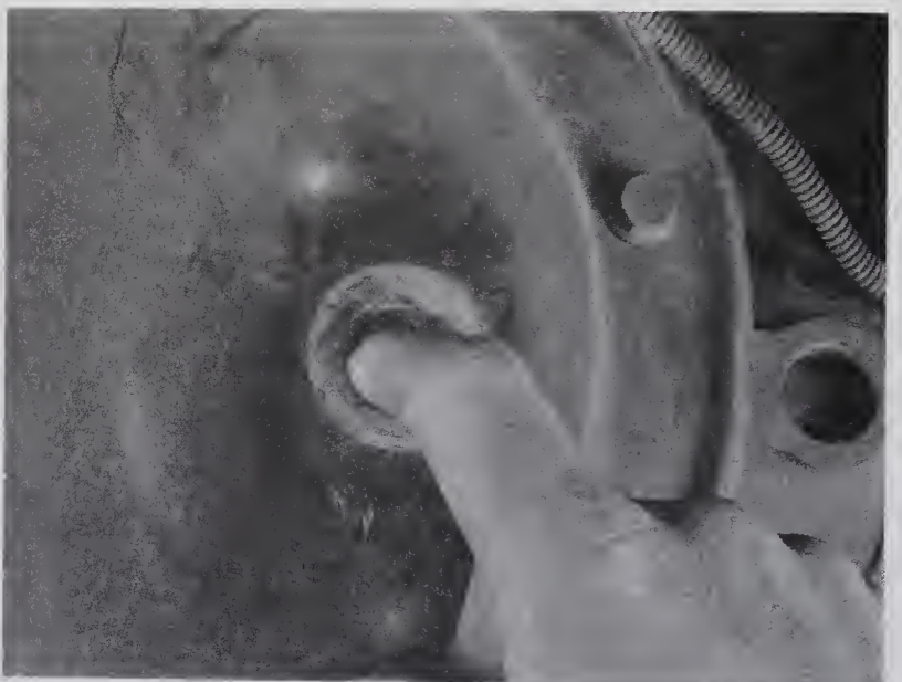
18.3 Use your finger as a dipstick to check the lubricant level
