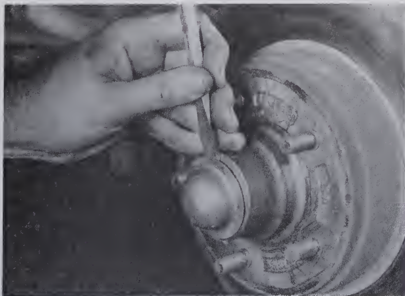
33.6 Dislodge the dust cap by working around the outer circumference with a hammer and chisel
