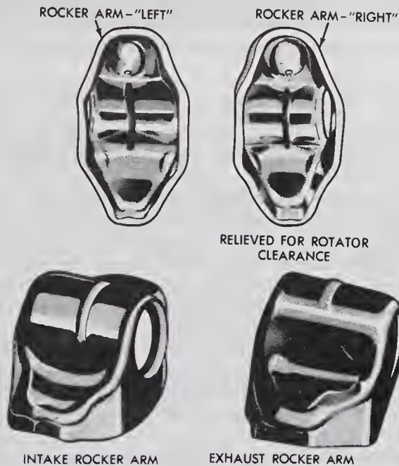
4.10 Rocker arm identification details (1987 through 1991 models)
