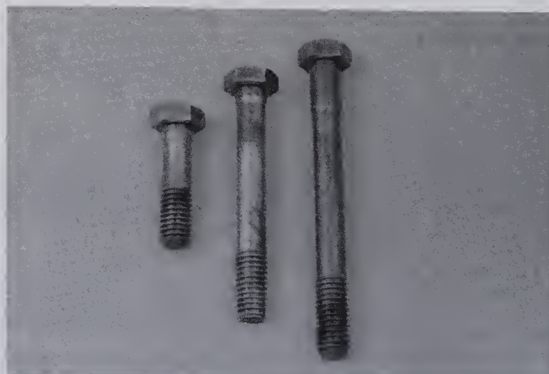
8.16a The two long bolts go in positions 1 and 3, the middle length bolts go in positions 5 and 7 and the short bolts go in positions 2, 4, 6 and 8 in the tightening sequence (1987-1991 V6 engine)
