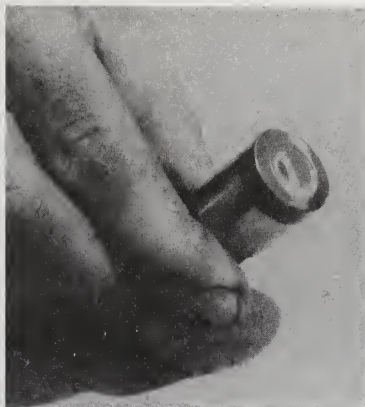
10.18a If the bottom of any lifter is worn concave, scratched or galled, replace the entire set with new lifters
