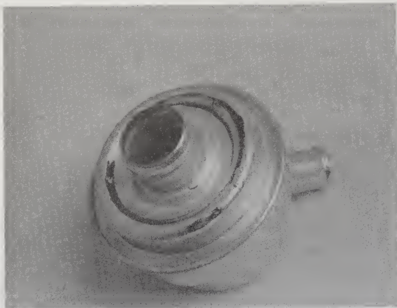
39.3 Lubricate the filter by pouring clean engine oil into the large opening until it drains out of the smaller opening (V6 and V8 models only)
