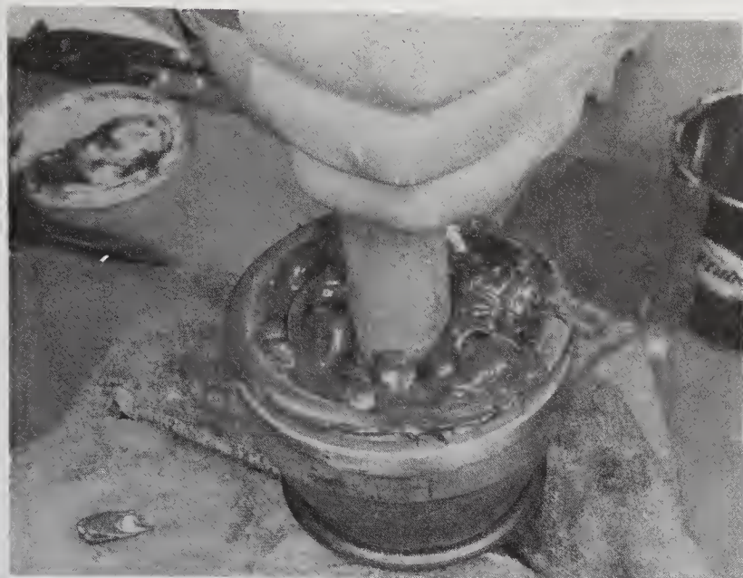
19.43 Apply grease through the splined hole, then insert a wooden dowel into the hole and push down – the dowel will force the grease into the joint
