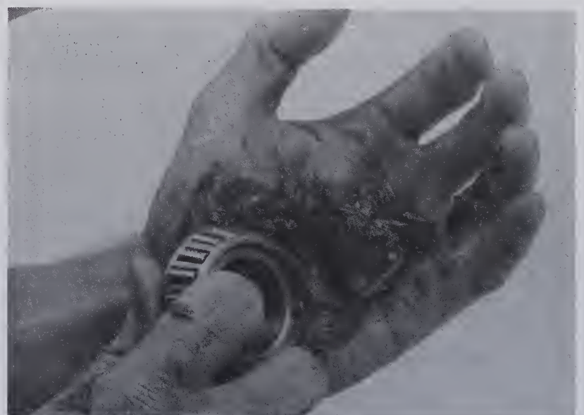
33.15 Work the grease into each bearing until it's full
