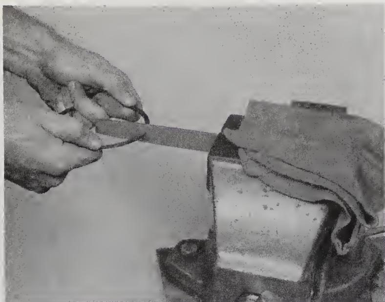
22.5 If the end gap is too small, clamp a file in a vise and file the ring ends (from the outside in only) to enlarge the gap slightly
