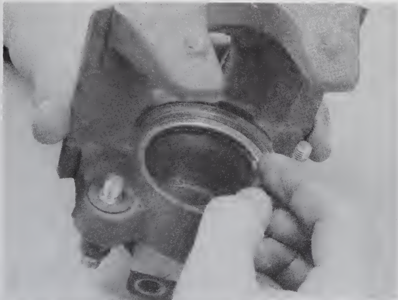
3.10 Position the new seal in the cylinder groove – make sure it isn't twisted
