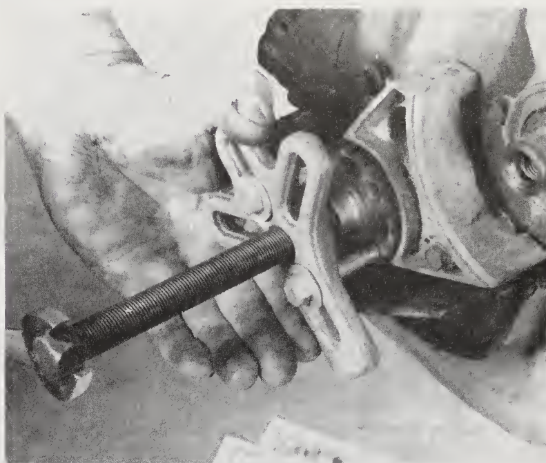
6.6 A puller must be used to remove the crankshaft sprocket
