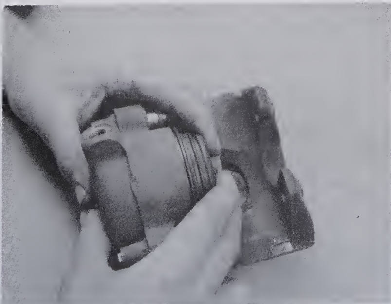
3.11b Push the piston straight into the cylinder – make sure it doesn't become cocked in the bore
