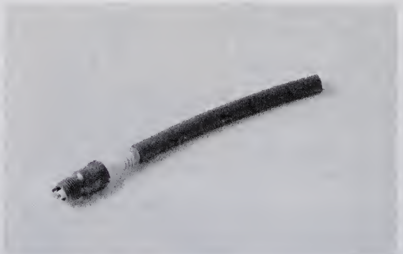
43.10 A length of 3/16-inch ID rubber hose will save time and prevent damaged threads when installing the spark plugs
