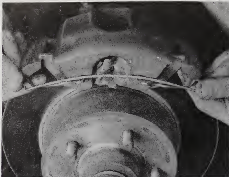
2.4 On 2WD models, remove the hold-down spring by depressing the ends and pulling the spring out
