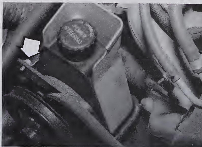
17.3 Remove the cover bolts (arrow) and detach the cover
