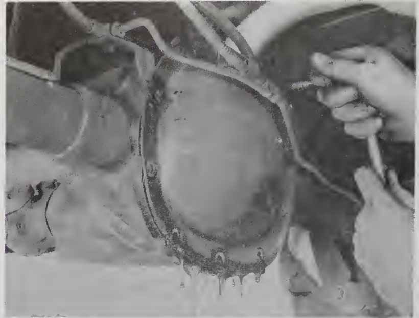
32.4b . . . then loosen the top bolts and let the lubricant drain
