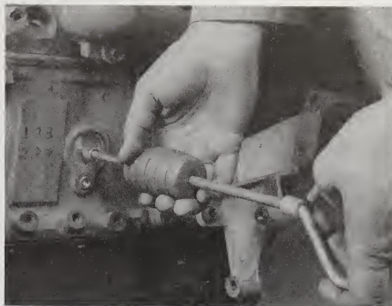
15.1 Remove the core plugs with a puller – if they're driven into the block, they may be impossible to retrieve
