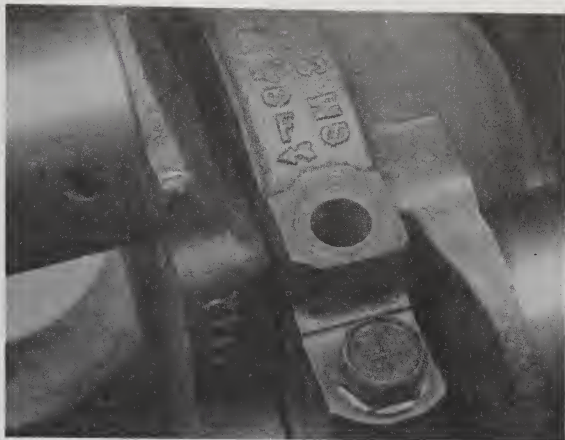
14.4c The arrow on the main bearing cap indicates the front of the engine
