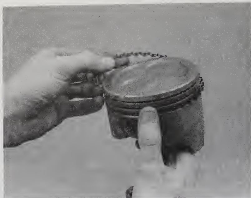
22.9a Install the three-piece oil control ring first, one part at a time beginning with the spacer/expander . . .
