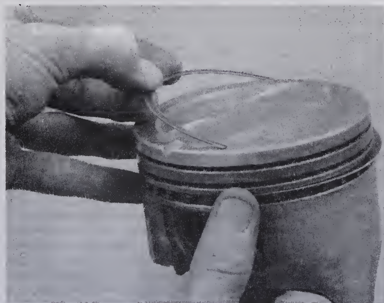
22.9b . . . followed by the side rails – DO NOT USE a piston ring installation tool to install the oil ring side rails
