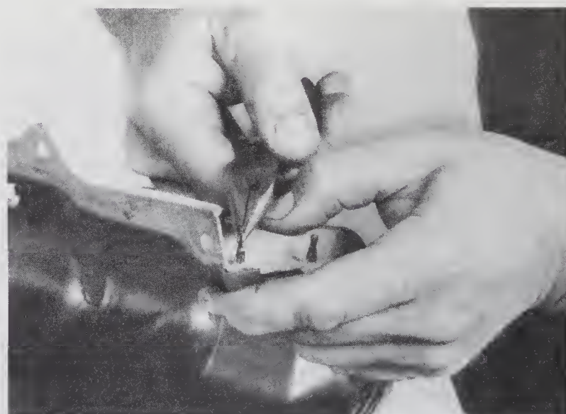
3.10b Seat the new end seals in the valve cover by pulling the tabs through the holes with pliers
