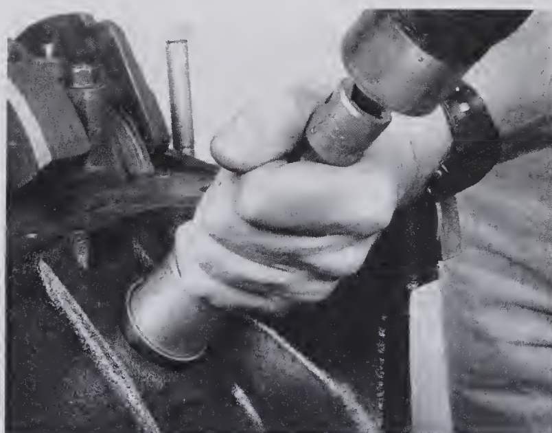
15.10 A large socket on an extension can be used to drive the new core plugs into the bores
