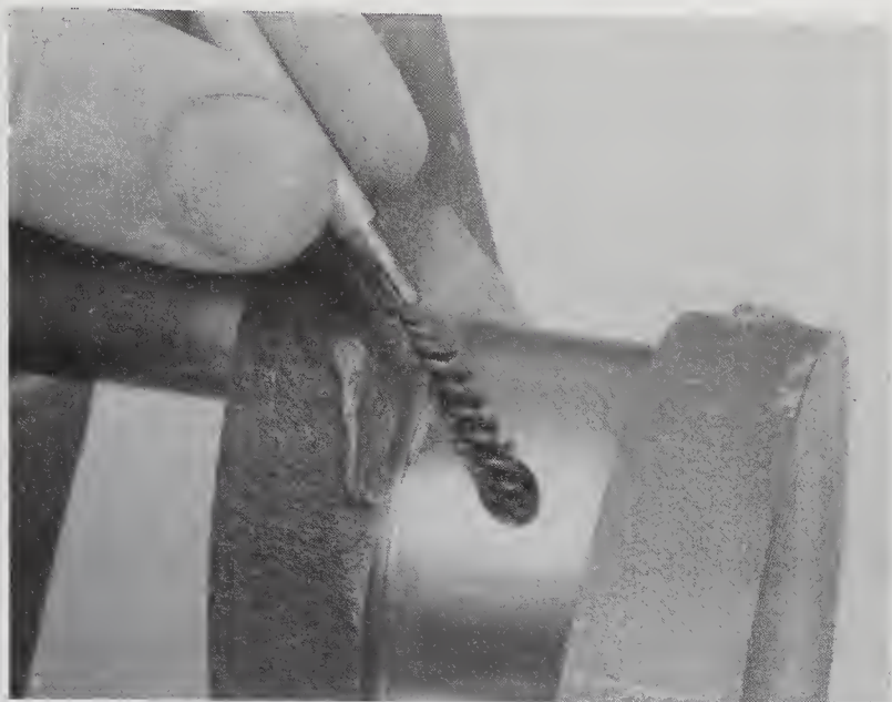
19.1 Clean the crankshaft oil passages with a wire or stiff plastic bristle brush and flush them out with solvent
