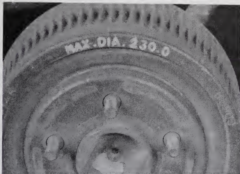
5.5 The maximum allowable inside diameter is cast into the outer edge of the drum
