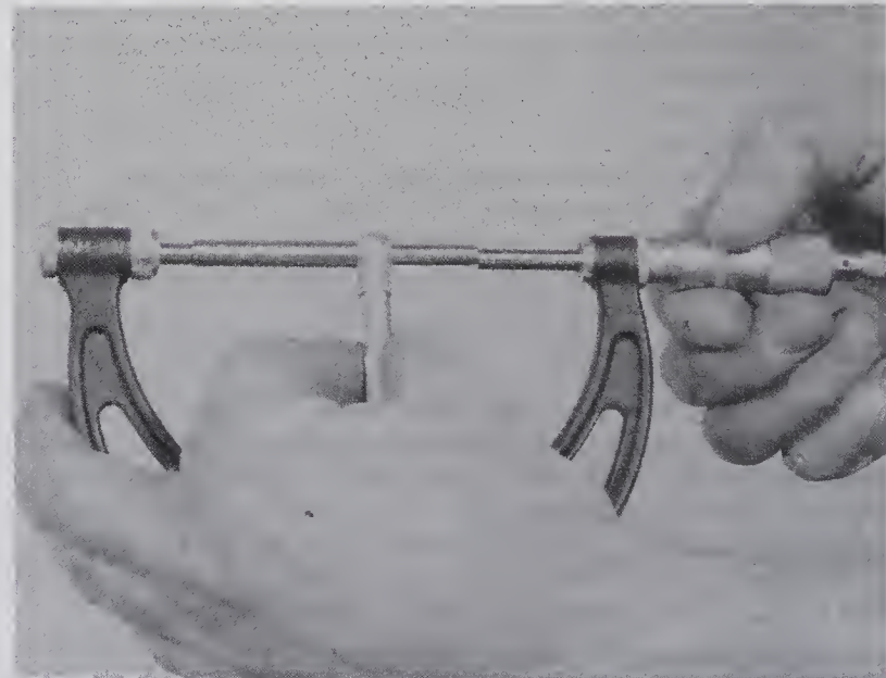
16.4c The gauge is then measured with a micrometer to determine bore size
