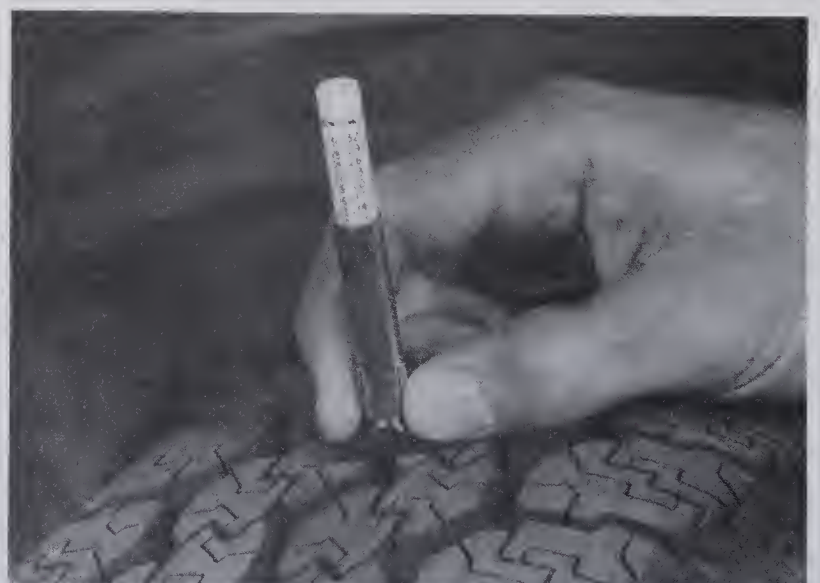
5.2 A tire tread depth indicator should be used to monitor tire wear – they're available at auto parts stores and service stations and cost very little
