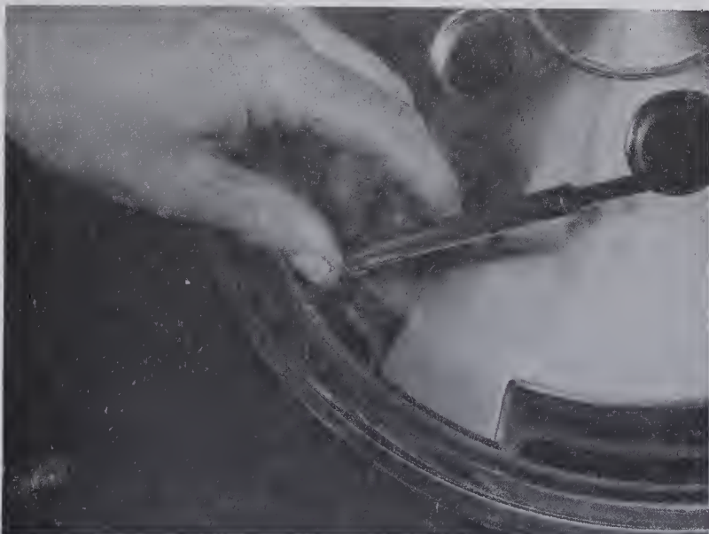
5.8 To extend the life of the tires, check the air pressure at least once a week with an accurate gauge (don't forget the spare!)
