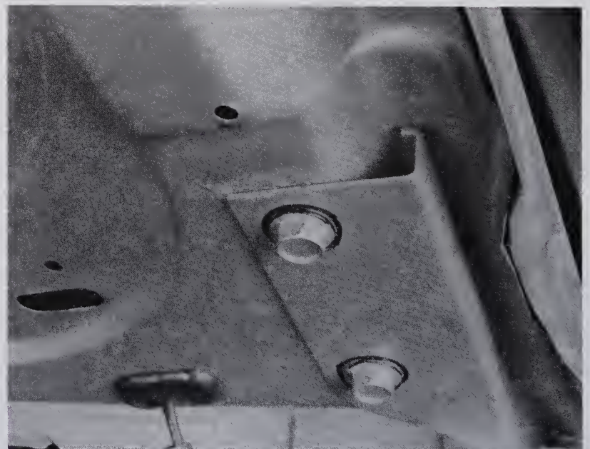
17.2 Scribe or mark around the mounting bolts on the hinge – mark around the entire hinge plate before removing the hood
