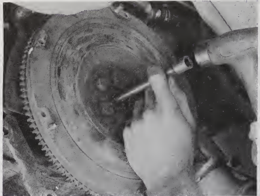
6.9 . . . then force the bushing out hydraulically with a steel rod slightly smaller than the bore in the bushing – when the hammer strikes the rod, the grease will transmit force to the backside of the bushing and push it out
