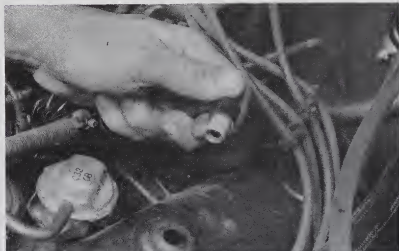
35.2 The PCV valve fits into the valve cover on V6 and V8 models
