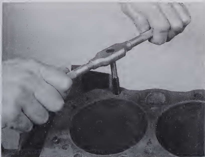
15.8 Clean and restore all threaded holes in the block – especially the main bearing cap and head bolt holes – with a tap (be sure to remove debris from the holes when you're done)
