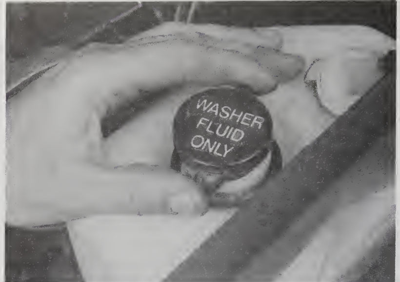
4.14 The windshield washer fluid level can be checked visually through the translucent plastic reservoir – do not overfill it
