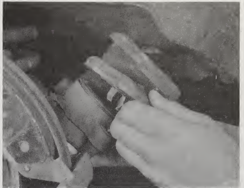
2.7a Unclip the inner pad from the caliper piston
