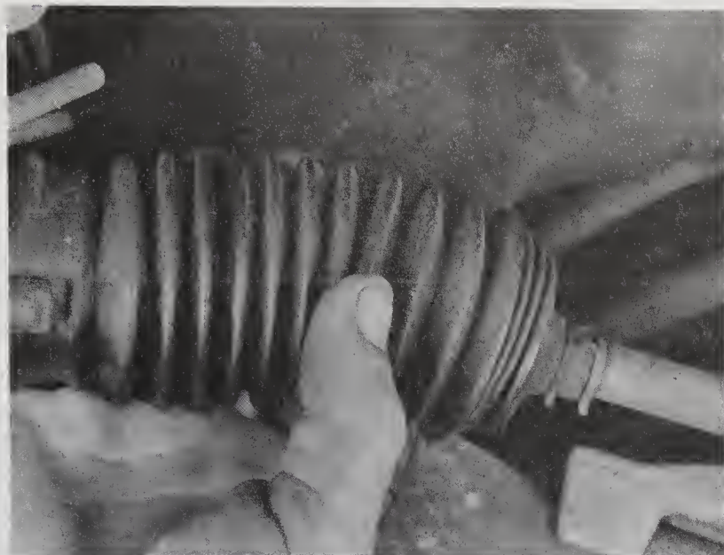
13.4 Push on the steering gear boots to check for cracks or leaking grease
