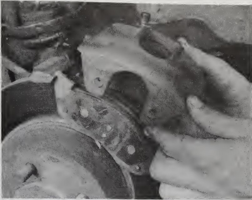
2.6 Lift the caliper straight up off the brake disc . . .
