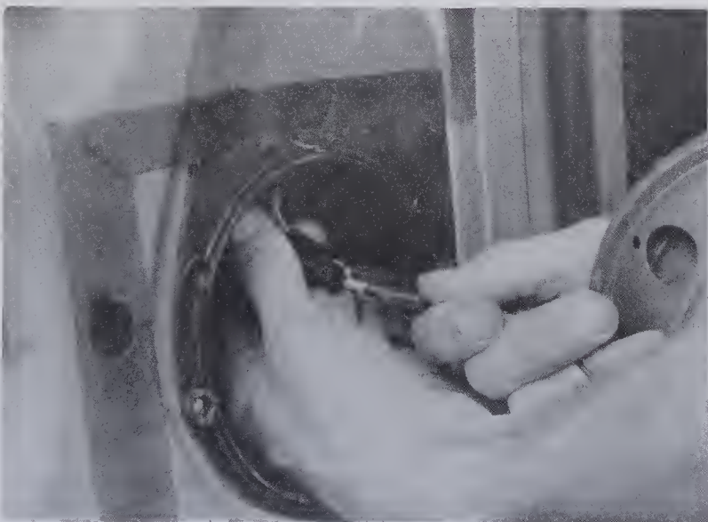
11.7b . . . then pull the speaker out and support it so you can use both hands to unplug the connector
