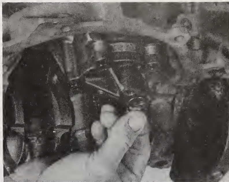
11.8 Lubricate the new O-ring and install it in the oil pump before attaching the pickup tube
