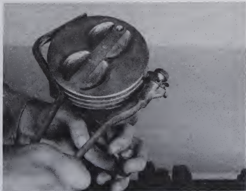
18.4a The piston ring grooves can be cleaned with a special tool, as shown here . . .
