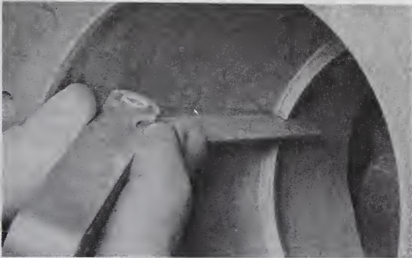
22.4 Once the ring is at the lower limit of travel and square in the cylinder, measure the end gap with a feeler gauge
