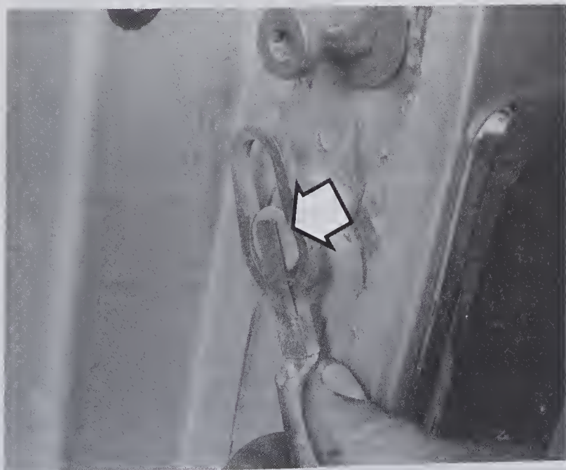
23.2 Slide the widest opening of the eyelet over the head of the pin and lift it off
