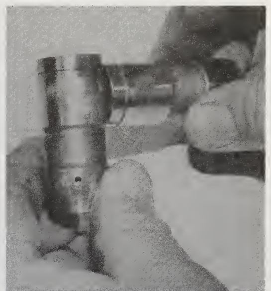
10.18b The foot of each lifter should be slightly convex – the side of another lifter can be used as a straightedge to check it; if it appears flat, it is worn and must not be reused
