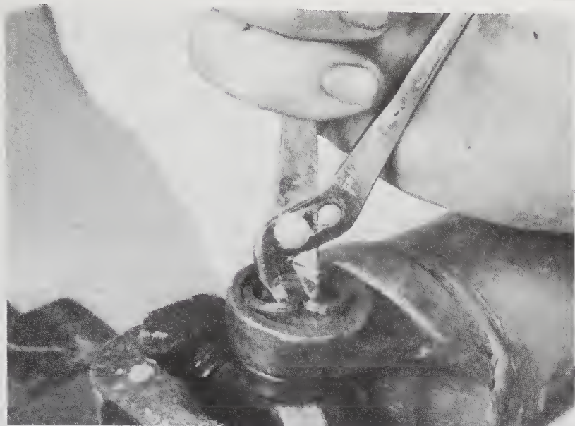
11.2 Use pliers to remove or install an external snap-ring from the U-joint
