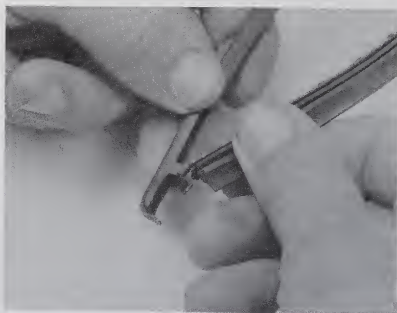
11.7 Squeeze the tabs on the end of the blade, pull the end out of the bridge claw, then slide the element out of the blade
