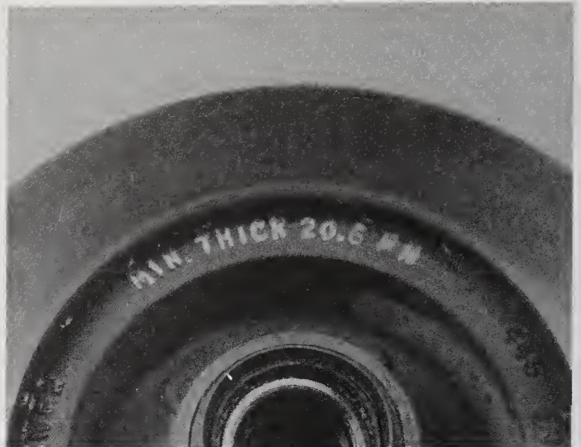
4.4a On some models, the minimum thickness is cast into the inside of the disc – on others, it's located on the outside of the disc
