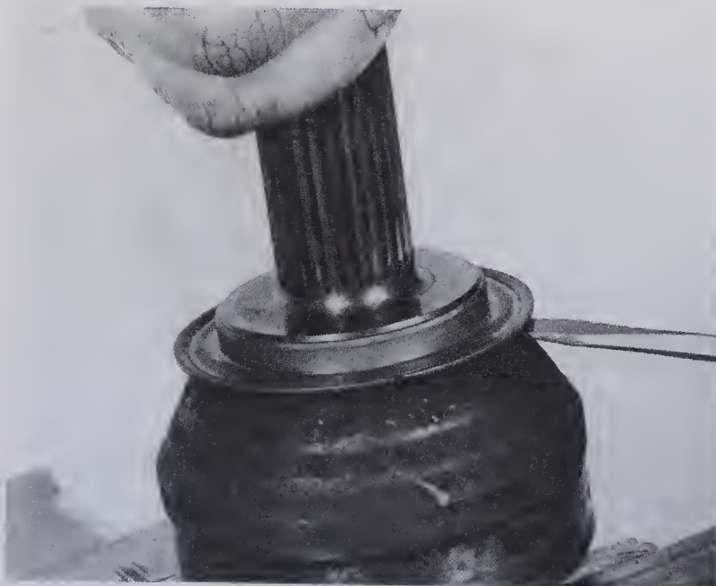
19.37 The wear sleeve can be pried off the housing with a large screwdriver if replacement is necessary
