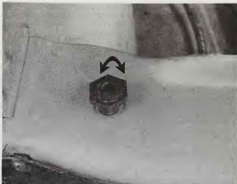
17.11 The hood bumpers can be screwed in or out to adjust the front edge of the hood in relation to the fenders
