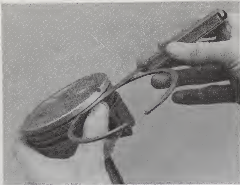
18.10 Check the ring side clearance with a feeler gauge at several points around the groove
