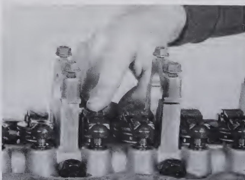
7.15 Seat the rocker arms on the valves and adjusters, then apply assembly lubricant to the cam lobe faces
