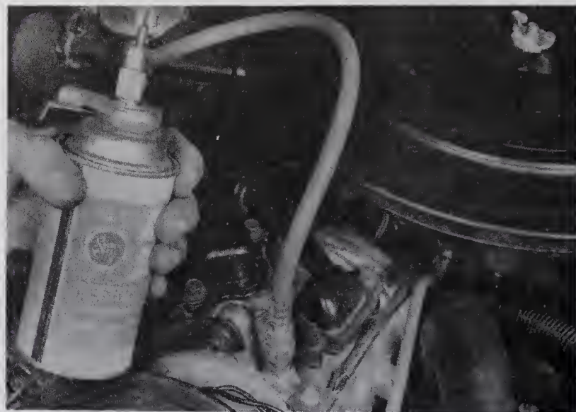
12.8 Connect the charging kit to the low side fitting on the compressor (marked "S" for suction)
