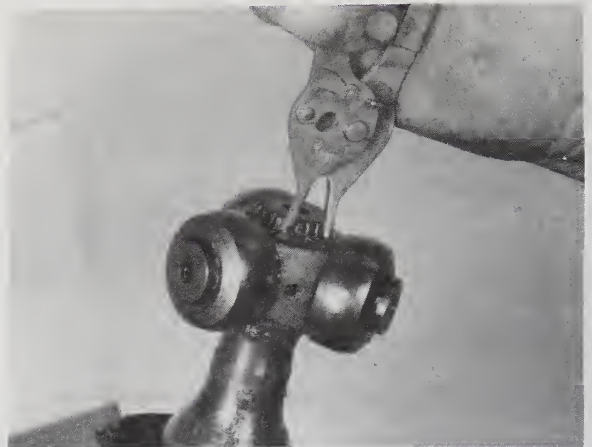
19.6 The tripod is held on the shaft with a snap-ring
