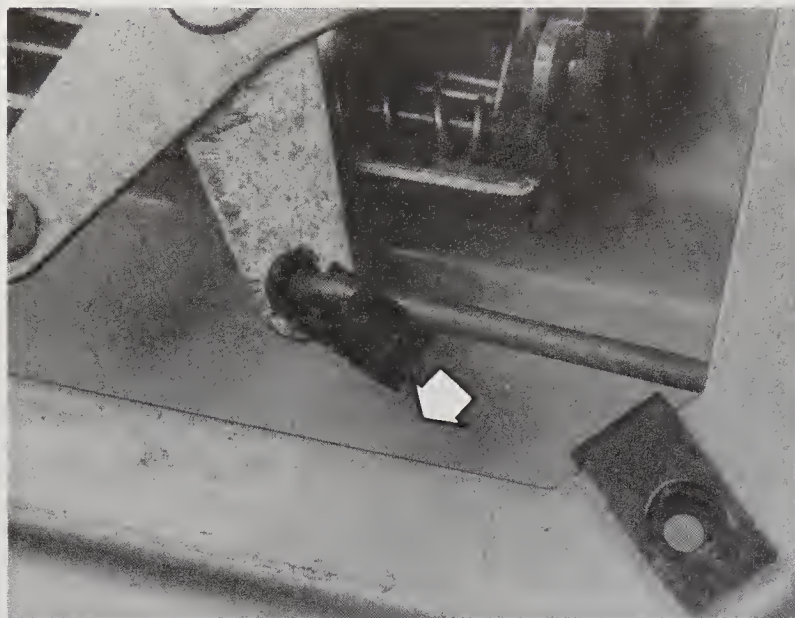
24.2 Slide the ends of the clips over, then lift the link straight up to disconnect it from the handle mechanism
