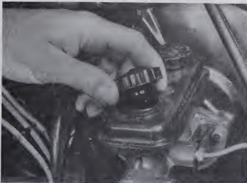
4.19 The brake fluid level is easily checked after unscrewing the cap – the level should be even with the ring at the base of the filler neck
