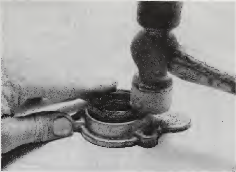
9.9 With the retainer on a flat surface, carefully tap the new seal into place with a soft-face hammer
