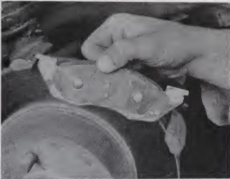
2.7b Remove the outer pad from the caliper adapter
