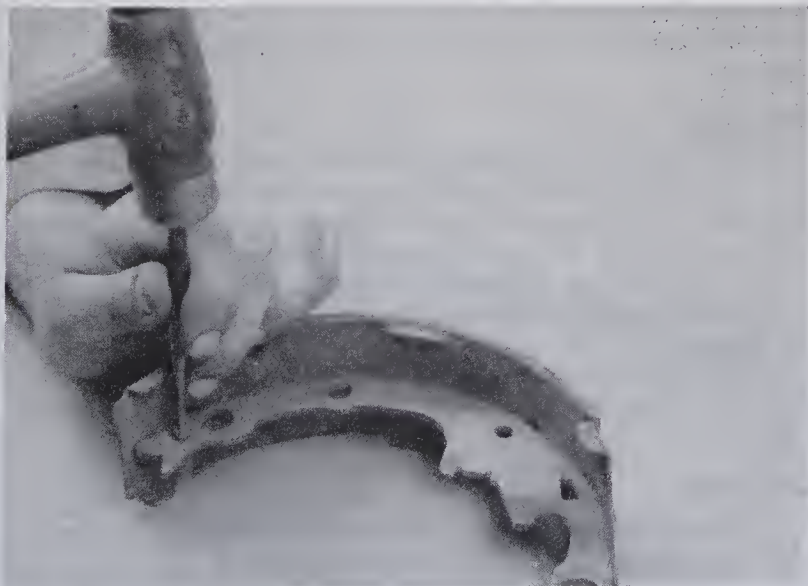
5.4k Install a new adjuster lever pin to the new shoe
