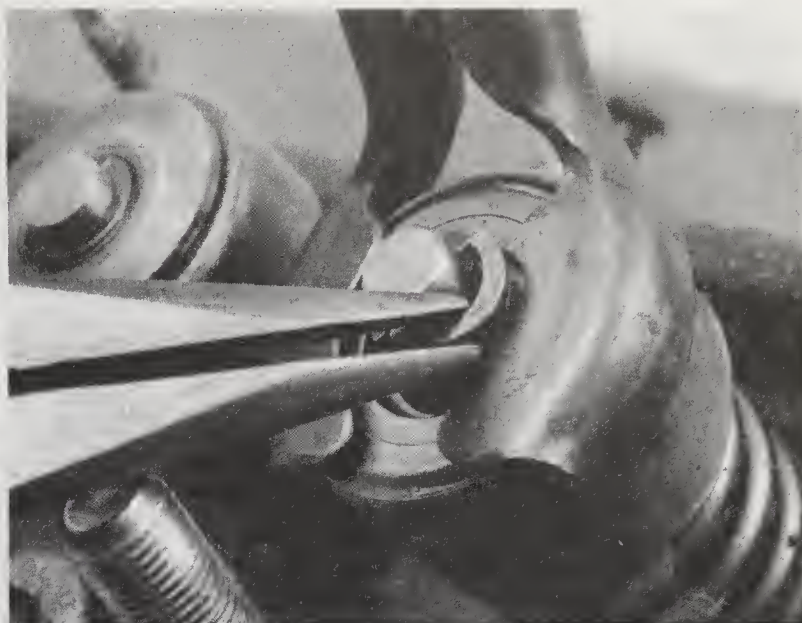
9.3a Use a valve spring compressor to compress the springs, then remove the keepers from the valve stem with a magnet or small needle-nose pliers
