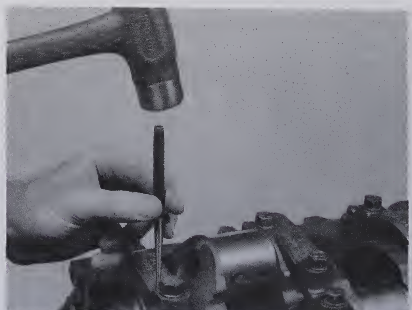
14.4b Use a center punch or number stamping dies to mark the main bearing caps to ensure installation in their original locations on the block (make the punch marks near one of the bolt heads)
