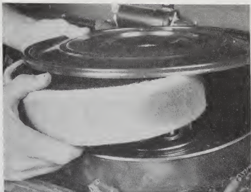
27.4a Remove the wingnut, release the clips (if equipped), then lift off the cover and pull out the filter element (V6 model shown, V8 similar)
