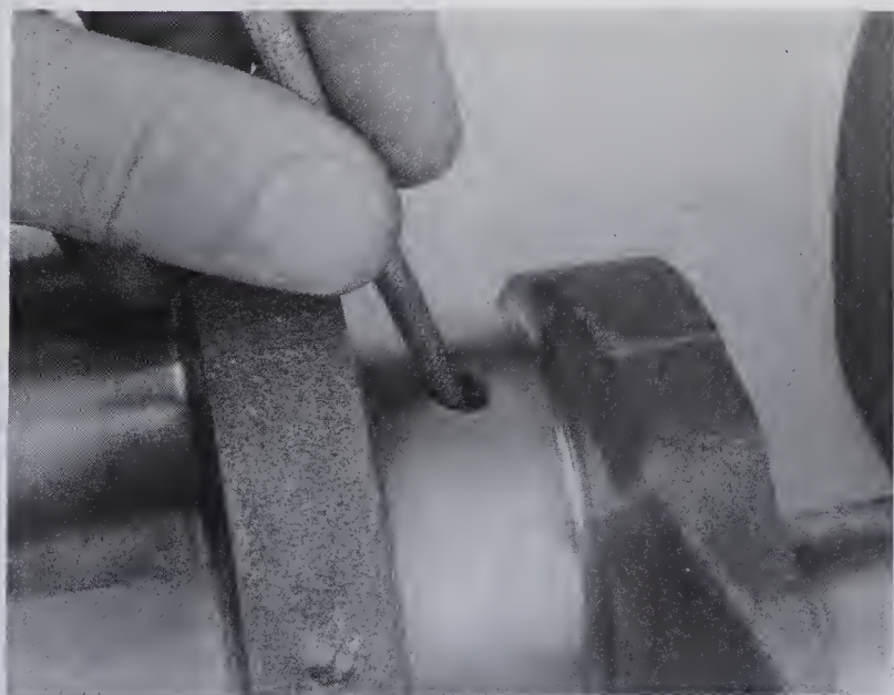
19.4 Chamfer the oil holes to remove sharp edges that might gouge or scratch the new bearings
