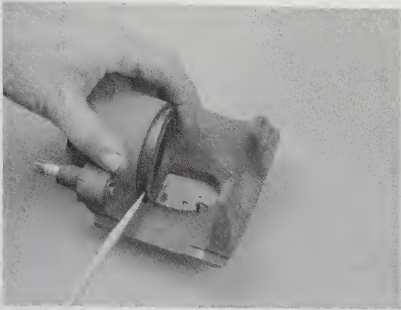
3.5b Carefully pry the dust boot out of the caliper
