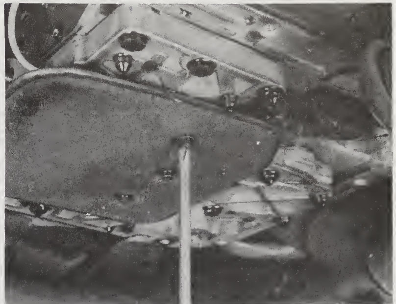
29.9 Use a Phillips screwdriver to remove the filter screws
