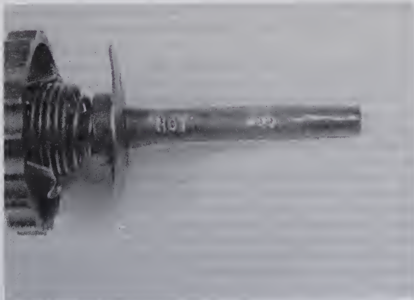
7.6a The power steering fluid dipstick has marks on both sides so the fluid level can be checked when hot ...
