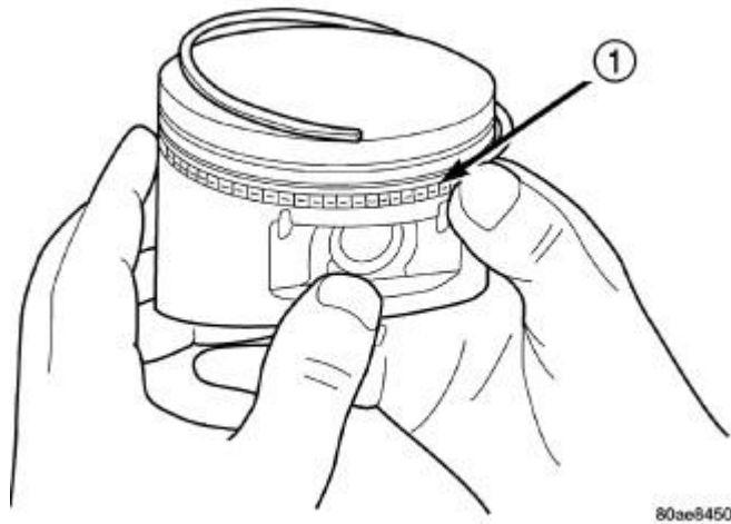
Fig. 400: Removing/Installing Piston Ring Side Rail Courtesy of CHRYSLER GROUP, LLC
