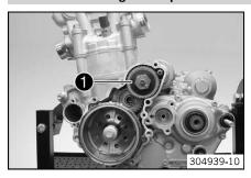
Remove torque limiter ①.
