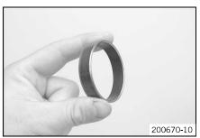
Roughen, clean, and grease the edges of the sliding bushings using 600 grit sandpaper.
