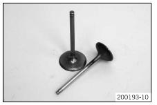
Check the valve plate for run-out.
