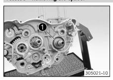
Remove spacer • of the crankshaft.
