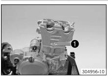
Remove nut • with the washer.
