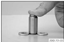
Place two compensating disks or similar aids next to the timing chain tensioner piston. This ensures that, when pressed in, the piston cannot go in all the way.
