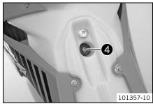
Remove screw 4 with the rubber bushing.
