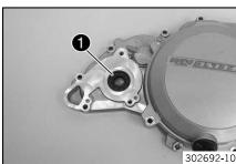
Press in shaft seal ring • all the way, with the open side facing outward.
