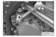
Remove screw connection on the clutch cover and fill up with engine oil.
