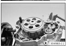
Mount pretension ring 3 with the Top marking facing up.
