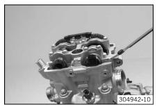
Check the valve clearance at all valves between the camshaft and cam levers.
