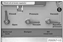
When the vacuum gauge reaches the required value, turn control lever **0il reservoir ⑤** to **Equalize pressure**.
