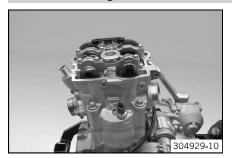
Grease the O-rings and mount the spark plug shaft insert.
