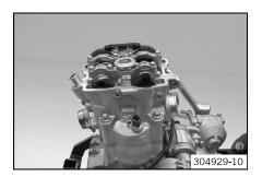
Remove the spark plug shaft insert.
