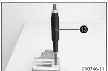
Screw on fluid barrier ® to the stop.
