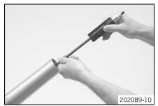
Lubricate the O-ring. Slide the cartridge all the way into the fork leg.
