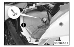
Insert both parts together, position them and fasten them using air filter holder ①.
