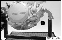
Remove screw • with the washer.
