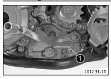
The engine number • is stamped on the left side of the engine under the engine sprocket.
