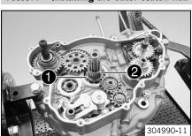
Mount collar sleeve 1 and both needle bearings 2.
