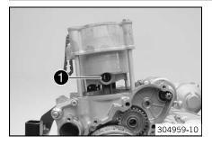
Push the cylinder upward.
