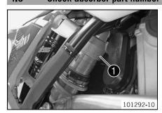
The shock absorber part number **1** is stamped on the top of the shock absorber above the adjusting ring on the engine side.
