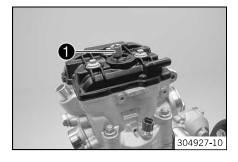
Mount and tighten the spark plug with special tool 1. Guideline
