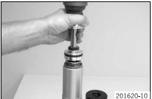
Grease the O-ring of the seal ring retainer.
