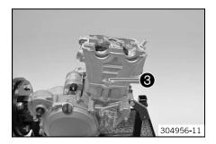
Mount and tighten nut **3** with the washer.
