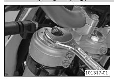
Turn the adjusting screws counterclockwise all the way.
