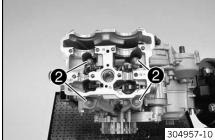
Mount nut ② with the washers and tighten in a crisscross pattern.
