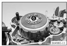
Install the screws 6 and tighten them diagonally.
