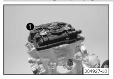
Remove the spark plug using special tool •.
