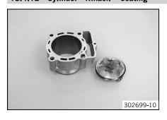
**Nikasil®** is a surface protection layer for a coating procedure developed by Mahle. The name is derived from the two materials used in this procedure - a layer of nickel into which is embedded the particularly hard silicone carbide.
