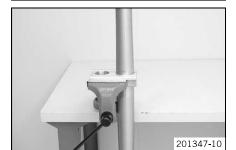
Clamp the fork leg in the area of lower triple clamp.
