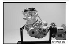
Mount the special tool on the engine mounting block.
