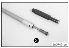
Remove piston rod 2 from the cartridge.
