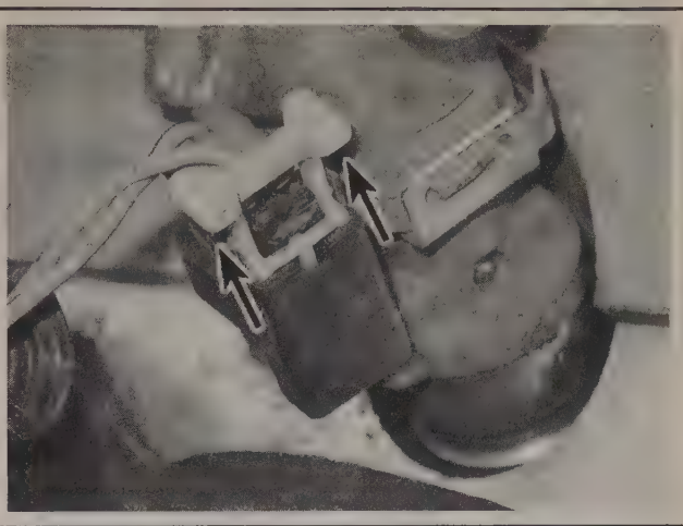
13.7 To disconnect the electrical connector from an injector on a four-cylinder model, pull up on this lock, then unplug the connector (this design is typical on these models; GM uses several variations of this design)
