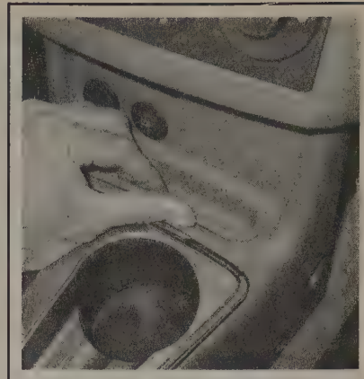
25.5 Pry out the console pen tray
