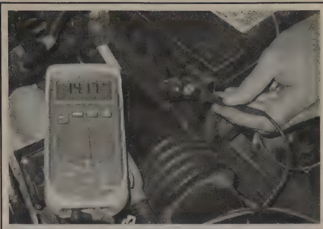
10.3 To measure charging voltage, turn on the engine and note the reading again, which should then be about 13.5 volts to 14.5 volts
