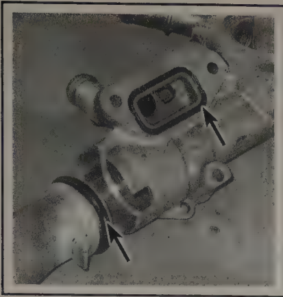
8.8 Remove the old seals and replace them with new ones
