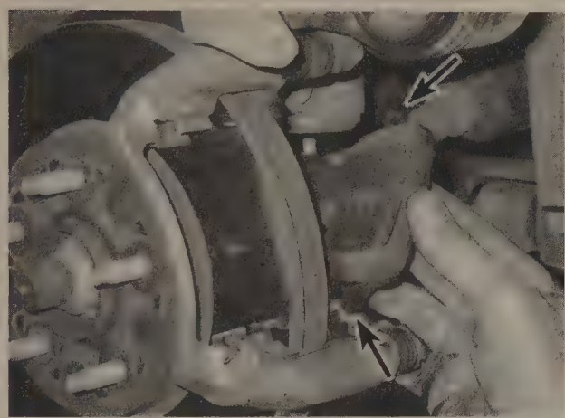
3.6j Make sure that the new pads are just like the old ones and complete with new shims (if equipped). Lubricate the ends of the new pads where they contact the anti-rattle clips with a small amount of high-temperature grease, then install the inner pad
