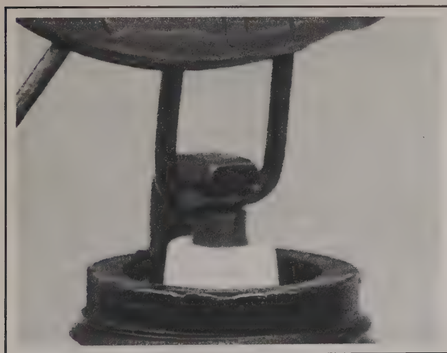
21.5a The manufacturer recommends using a wire-type thickness gauge when checking the gap - if the wire does not slide between the electrodes with a slight drag, adjustment is required
