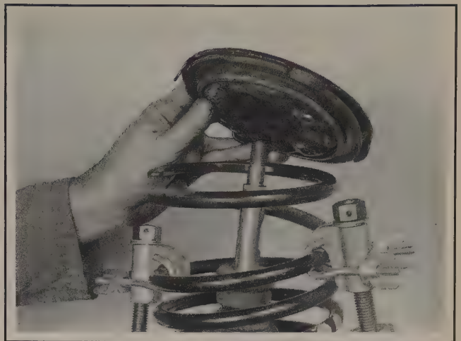
3.6 Remove the upper spring seat
