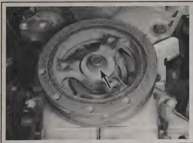
9.6 Remove the crankshaft bolt - it's very tight, so use a six-point socket and a breaker bar
