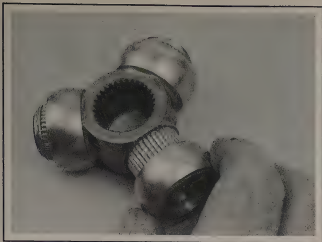
3.3i Clean all of the old grease out of the housing and spider assembly, then remove each bearing, one at time
