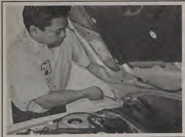
9.4 Support the hood with your shoulder while removing the hood bolts
