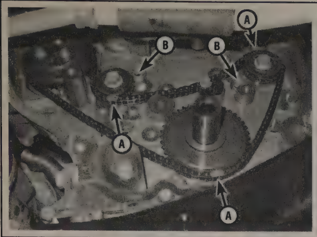
9.9 Balance shaft sprocket/chain alignment marks (A) and retainer bolts (B)
