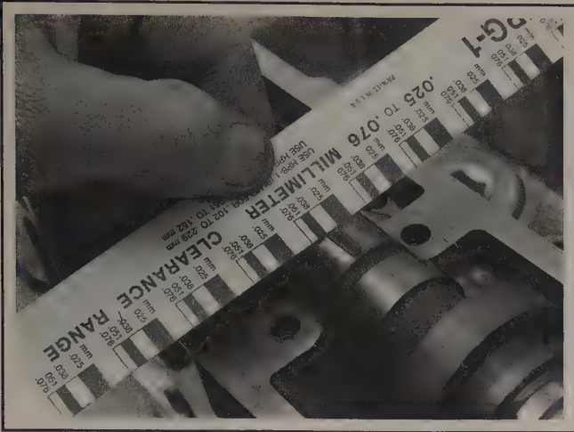
11.22 Compare the width of the crushed Plastigage to the scale on the package to determine the journal oil clearance
