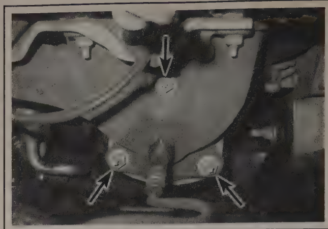
15.8 To disconnect the upper flange of the front catalyst/exhaust pipe assembly from the exhaust manifold flange on a V6 engine, remove these three nuts
