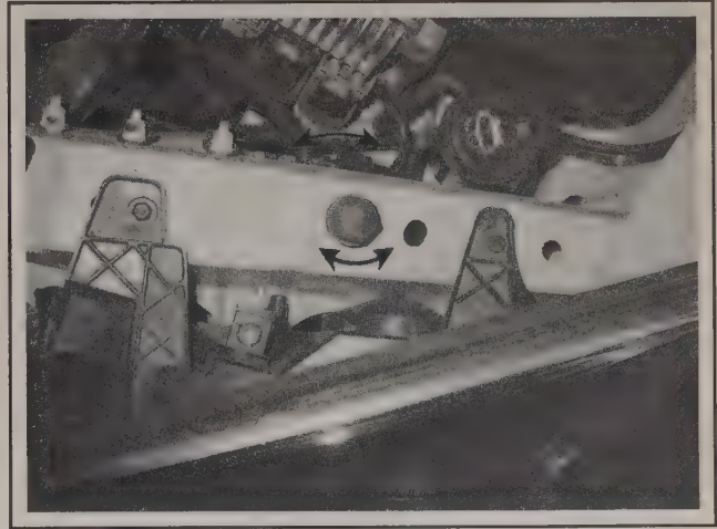
9.10 Adjust the hood closing height by turning the hood bumpers in or out
