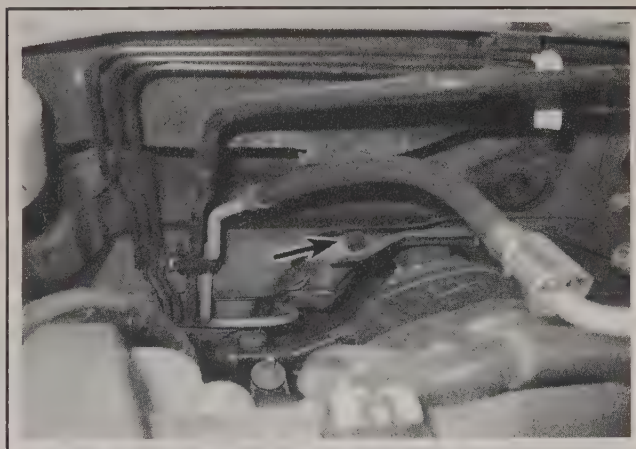
13.1 Look for the evaporator drain hose on the firewall towards the middle-right side (passenger's side)
