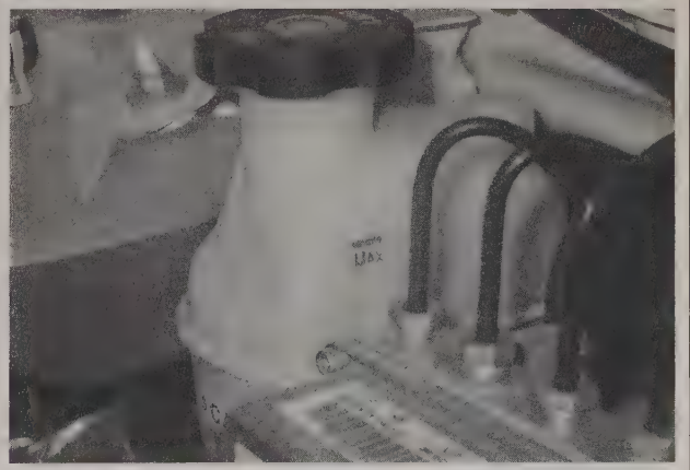
4.15 The brake fluid level should be kept between the MIN and MAX marks on the translucent plastic reservoir; the same reservoir contains the clutch fluid and is connected to the clutch master cylinder by a hose
