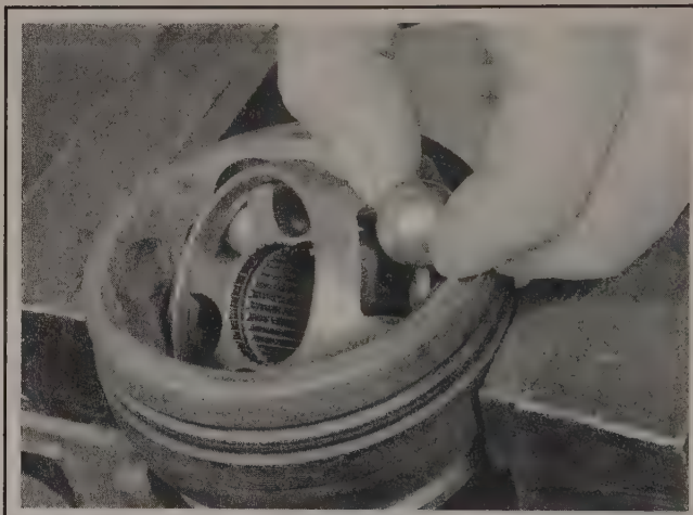
3.4j . . . press the balls into the cage windows, repeating until all of the balls are installed
