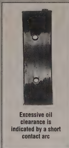
Result of a lower half assembled as an upper - blocking the oil flow
