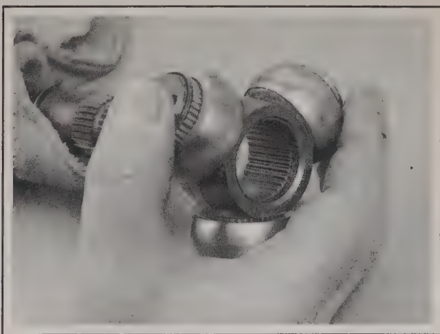
3.3n Install the spider bearing with the recess in the counterbore facing the end of the drive axle
