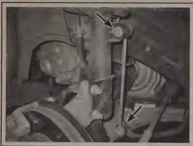
4.2 Remove the nuts on each end of the link to detach it. Hold the ballstud on the link with a tool to keep it from turning while removing the nut
