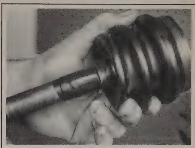
3.3l Wrap the axle shaft splines with tape to avoid damaging the boot, then slide the small clamp and boot onto the axle shaft
