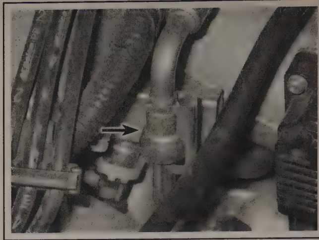
13.16 On V6 models, the fuel supply line is connected to the fuel rail with this metal collar type quick-connect fitting at the right end of the fuel rail. If you're unfamiliar with this type of fitting, refer to Section 4
