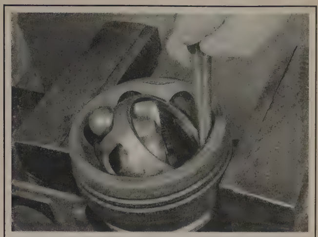
3.4b Press down on the inner race far enough to allow a ball bearing to be removed - if it's difficult to tilt, gently tap the cage and inner race with a brass punch and hammer
