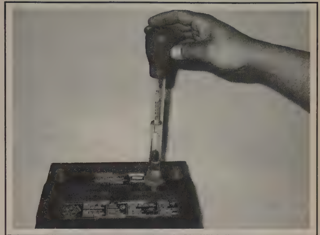
3.1a Use a battery hydrometer to draw electrolyte from the battery cell; this hydrometer is equipped with a thermometer to make temperature corrections
