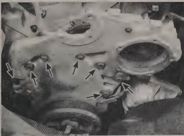
11.18a Timing chain cover bolt locations, upper . . .
