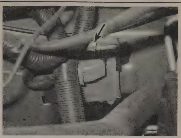
7.3 Push back the retaining tang and slide the TCM out of its bracket
