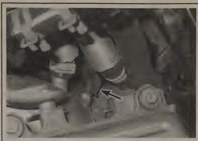
6.2 Disconnect the electrical connector from the ECT sensor (four-cylinder engines)
