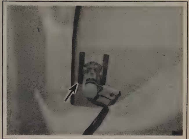
21.5 Remove the retaining clip from the lock cylinder
