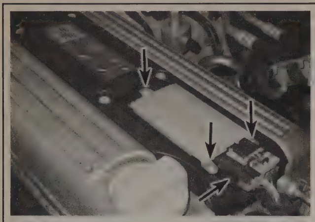
7.2 To remove the ignition control module, disconnect the electrical connector and remove the mounting screws
