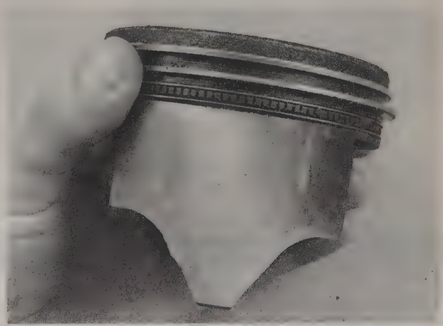
1.6 Uneven piston wear like this indicates a bent connecting rod
