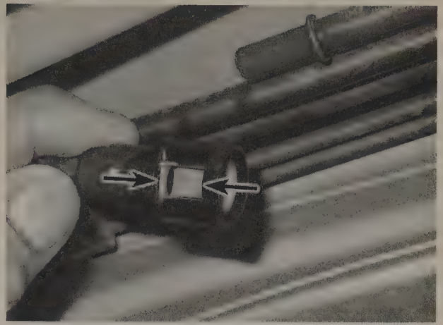
4.23 Install a new retainer in the female side of the fitting; make sure that the release tabs are aligned with the windows in the connector
