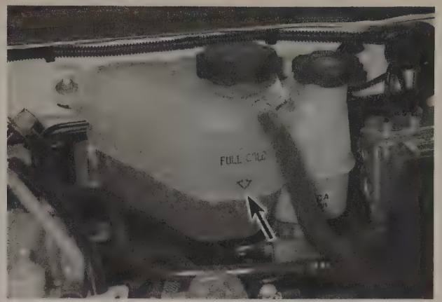
4.9 When the engine is cold, the engine coolant level should be at the COLD mark (expansion tank seam)
