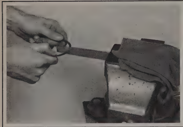
10.15 If the ring end gap is too small, clamp a file in a vise as shown and file the piston ring ends - be sure to remove all raised material
