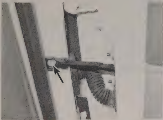
15.6 Remove the door check strap mounting bolt
