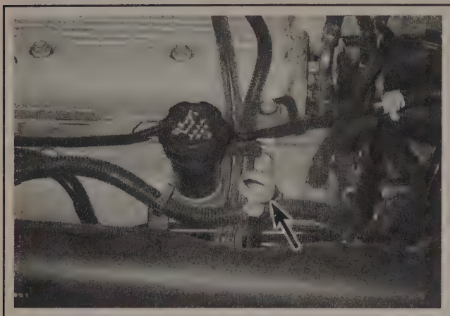
4.2a Engine oil dipstick location - V6 engines
