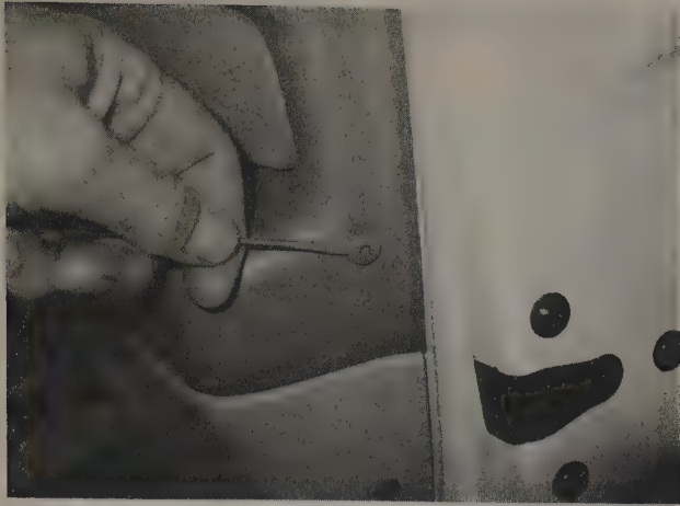
14.3 Remove the push-pin fasteners securing the door panel
