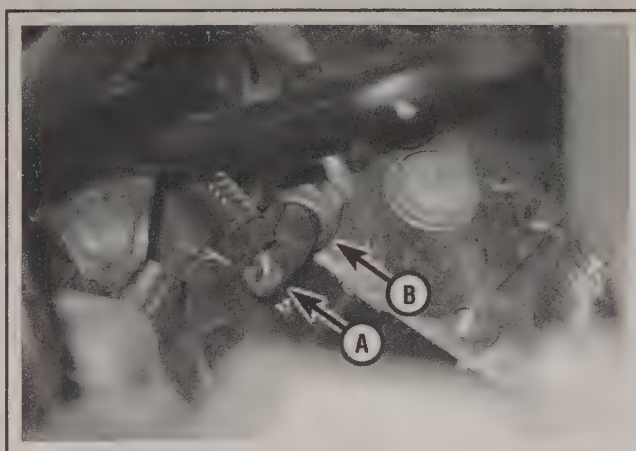
6.8 Disconnect the electrical connector (A) from the ECT sensor (B), then unscrew and remove the sensor (V6 engines)
