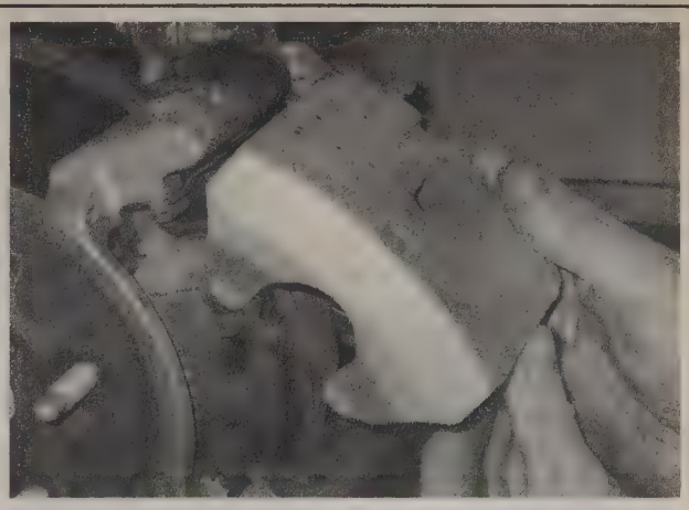
3.6m Place the caliper over the new pads and back onto the mounting bracket. On rear calipers, carefully align the notch in the piston with the pin on the back of the inner brake pad. Install the caliper mounting bolts and tighten them to the torque listed in this Chapter's Specifications
