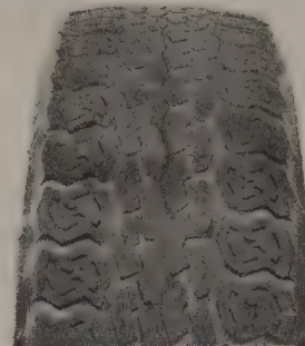
FEATHERING DUE TO MISALIGNMENT
