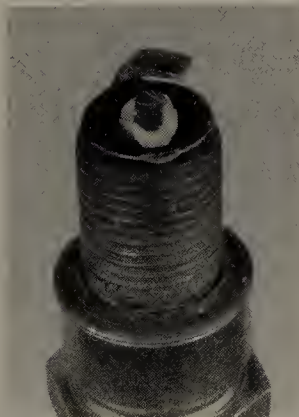
Fig. 105 Inspect the spark plug to determine engine running conditions
