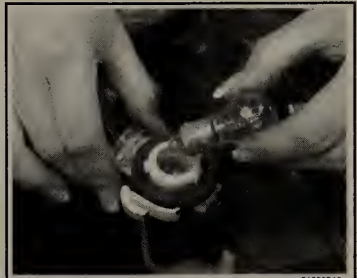
Fig. 61 Turn the bulb to align the nubs on the bulb with the channels in the socket, then carefully pull the bulb from the socket
