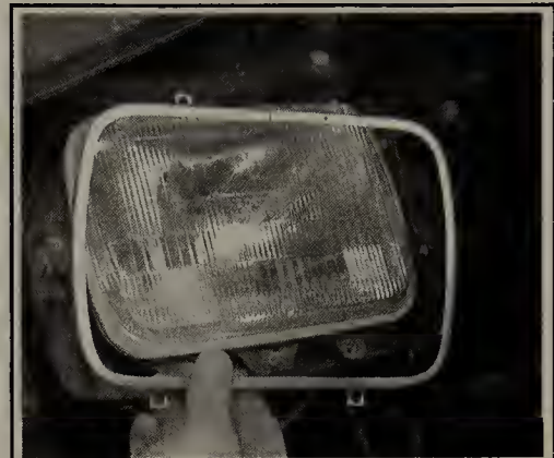
Fig. 54 Remove ONLY the 4 retaining ring screws, do NOT touch the aiming screws
