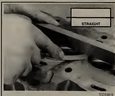
Fig. 144 Check the head for flatness across the center of the head surface using a straightedge and feeler gauge
