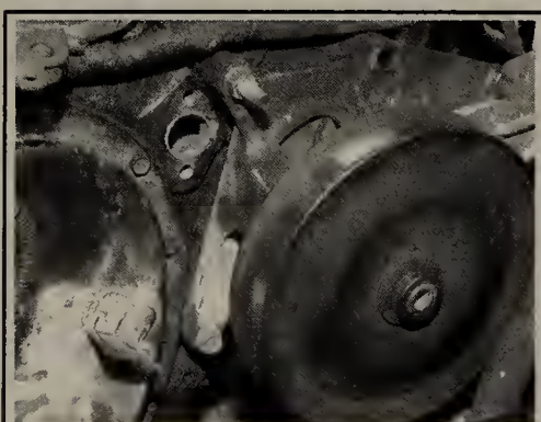
Fig. 57 Remove the power steering and alternator mounting bracket from the cylinder head
