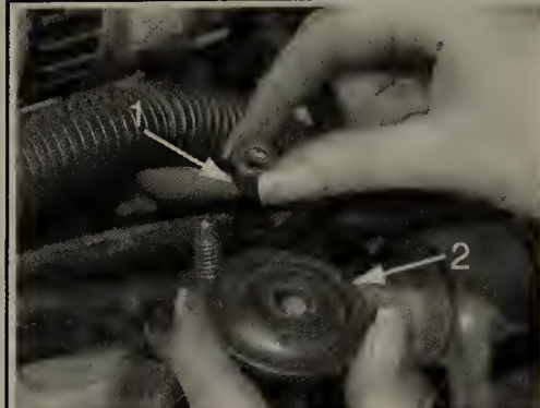
Fig. 15 Remove the upper shock mounting nut (1) and insulator retainer (2) . . .
