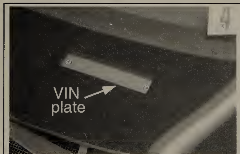
Fig. 32 The VIN is stamped into a plate which is visible through the windshield
