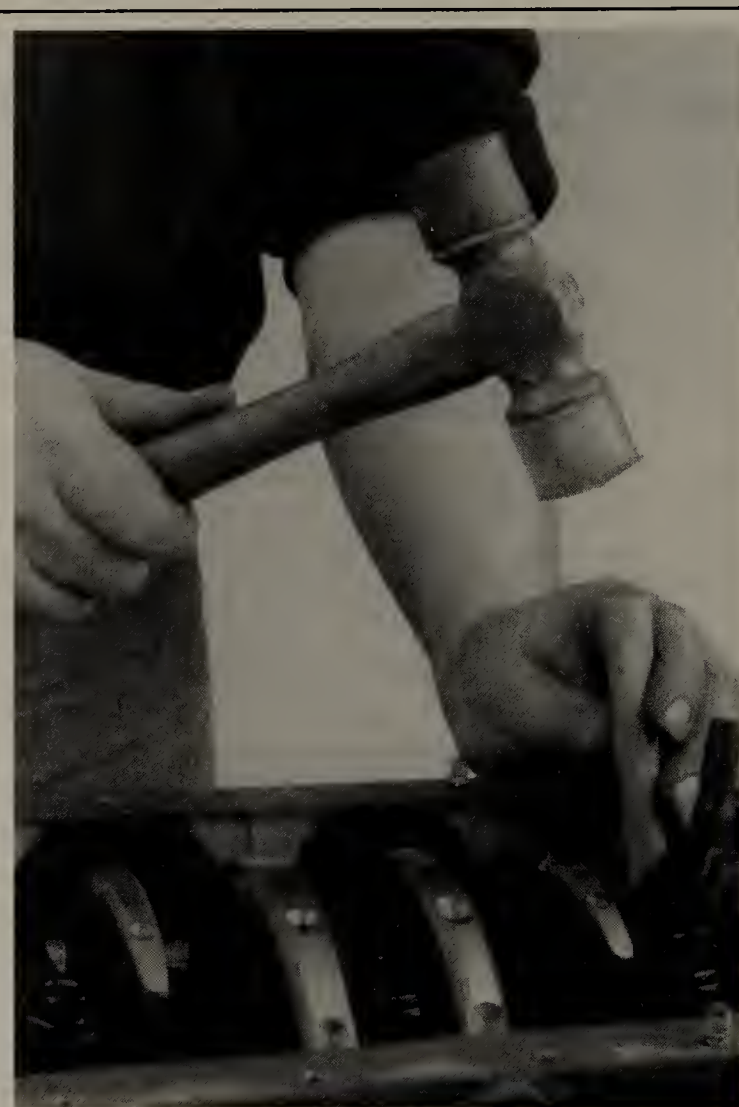
Fig. 147 Carefully tap the piston out of the bore using a wooden dowel
