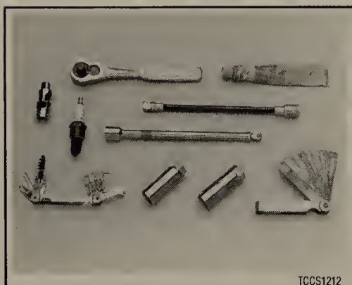
Fig. 10 A variety of tools and gauges should be used for spark plug gapping and installation
