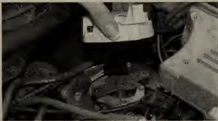
Fig. 124 . . . then pull the rotor straight up to remove it from the distributor
