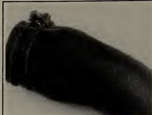
Fig. 95 A soft spongy hose (identifiable by the swollen section) will eventually burst and should be replaced
