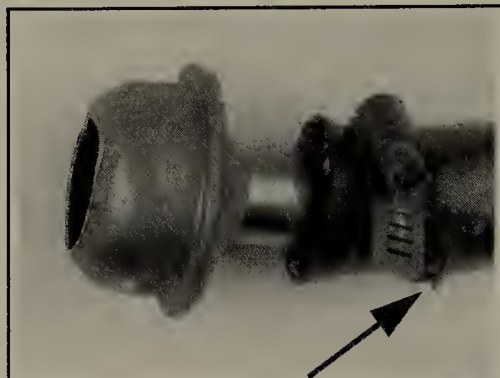
Fig. 94 A hose clamp that is too tight can cause older hoses to separate and tear on either side of the clamp
