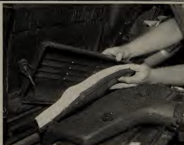
Fig. 42 Then, lift the cover off and pull the air cleaner element from the housing
