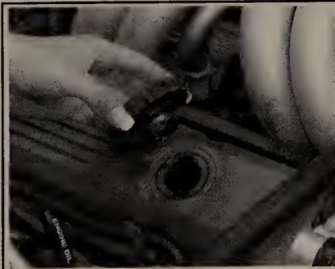
Fig. 158 If the level is low, remove the engine oil fill cap, located on the valve cover
