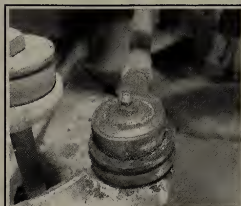
Fig. 222 Rear axle tie rod end grease fitting location
