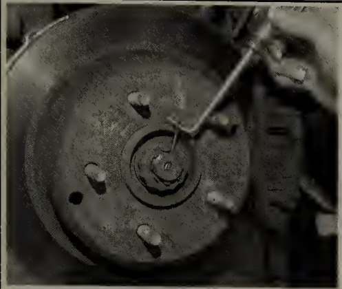
Fig. 63 Use a suitable tool to pull the cotter pin out of the wheel nut retainer
