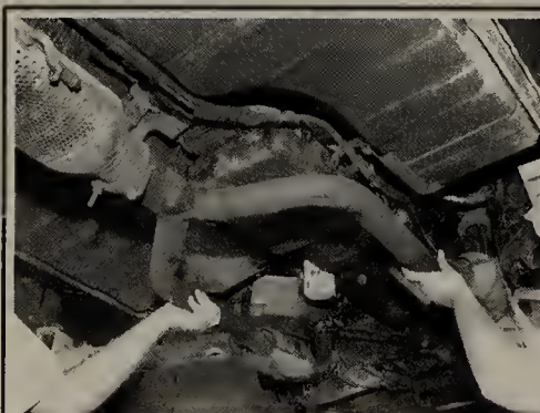
Fig. 84 With the help of at least one assistant, carefully lower the exhaust and place in a safe place
