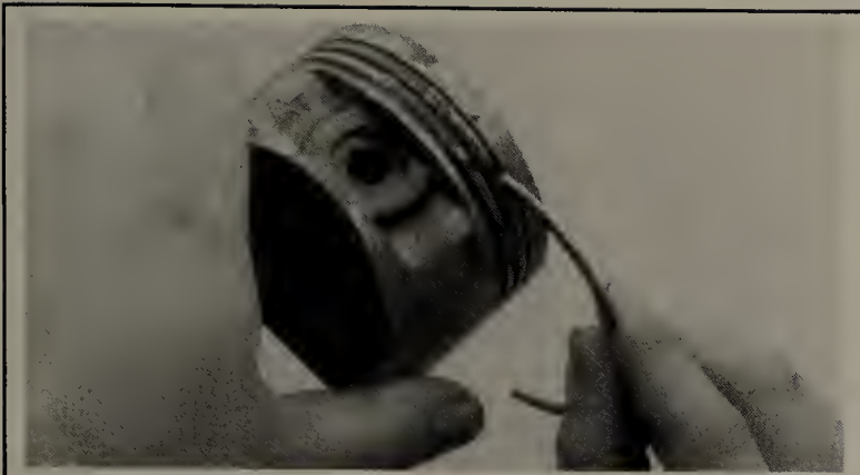
Fig. 127 . . . use a piece of an old ring to clean the grooves. Be careful, the ring can be quite sharp
