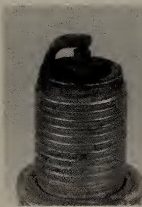
A carbon fouled plug, identified by soft, sooty, black deposits, may indicate an improperly tuned vehicle. Check the air cleaner, ignition components and engine control system.
