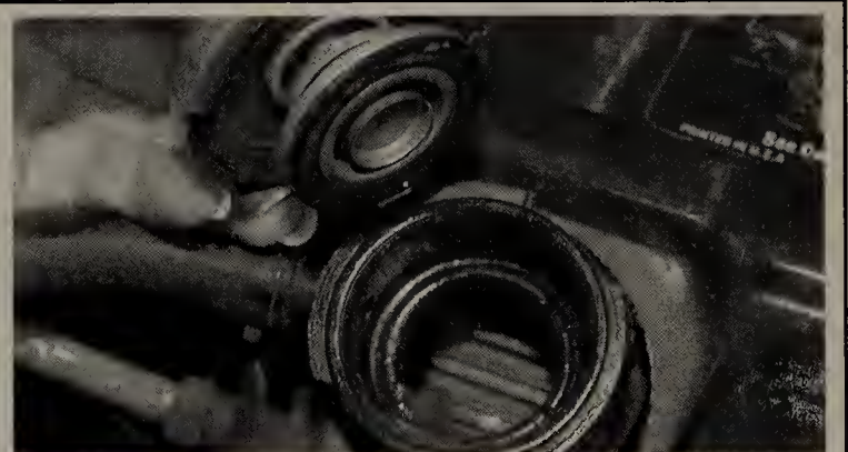
Fig. 202 When you remove the radiator cap, check the gaskets and make sure they are OK
