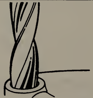
Fig. 130 Drill out the damaged threads with the specified size bit. Be sure to drill completely through the hole or to the bottom of a blind hole
