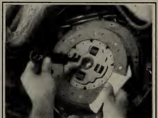
Fig. 21 Install a clutch alignment arbor, to align the clutch assembly during installation
