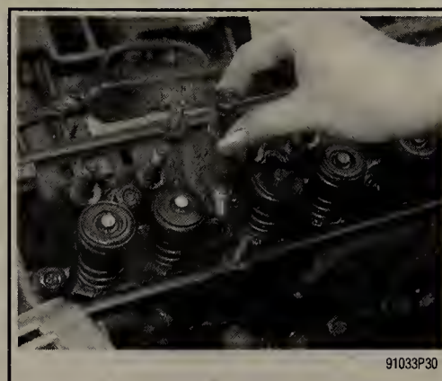
Fig. 62 When you remove the cylinder head bolts, keep them in order, because 2 different lengths of bolts are used
