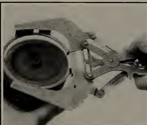
Fig. 125 Use a ring expander tool to remove the piston rings
