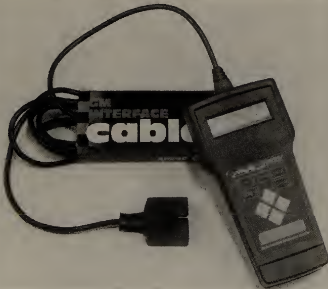
Fig. 102 Inexpensive scan tools, such as this Auto Xray®, are available to interface with your General Motors vehicle
