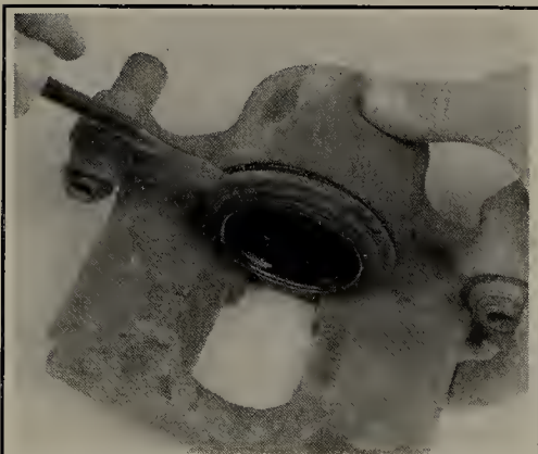
Fig. 68 Use a prytool to carefully pry around the edge of the boot . . .
