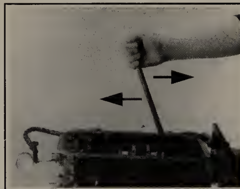
Fig. 155 Carefully pry the crankshaft back and forth while reading the dial gauge for end-play
