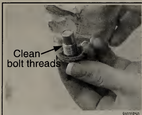
Fig. 163 Make sure you thoroughly clean the oil pan drain plug threads to avoid stripping the pan threads
