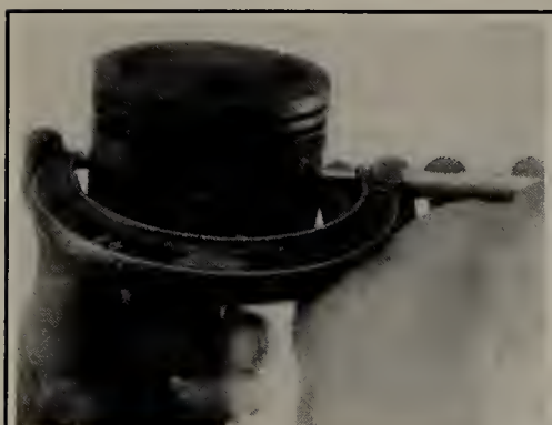
Fig. 149 Measure the piston's outer diameter, perpendicular to the wrist pin, with a micrometer
