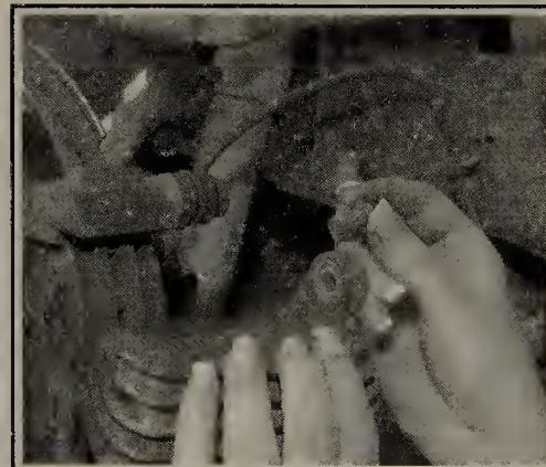
Fig. 31 Remove the bolt, then rotate the caliper down to access the brake pads
