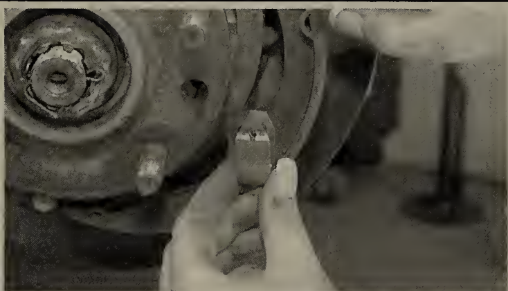
Fig. 83 Pull the shoe and lining out slightly, then remove the hold-down spring
