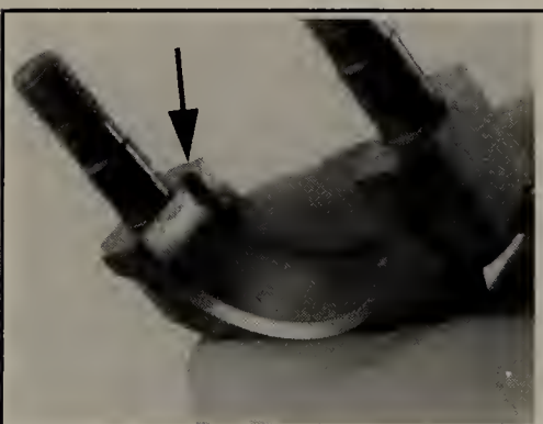
Fig. 157 The notch on the side of the bearing cap matches the tang on the bearing insert
