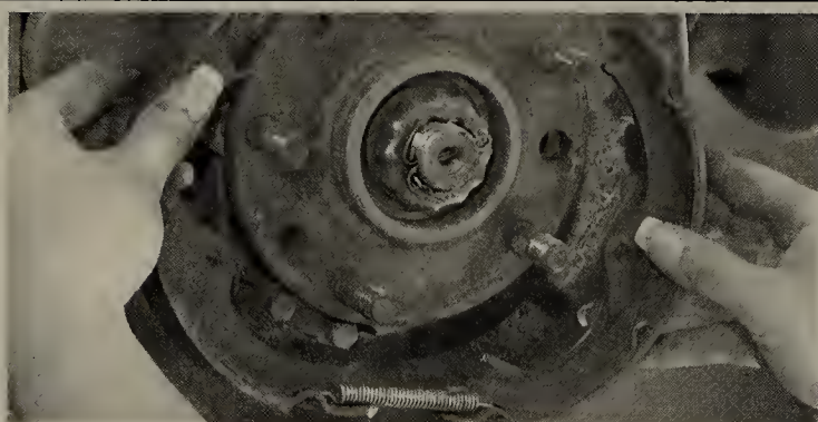
Fig. 84 Pull the shoe and linings apart enough to clear the hub and bearing, then remove the linings with the shoe return spring still engaged
