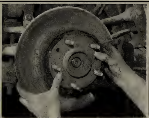
Fig. 69 Once the 3 bolts are removed, you can pull the hub and bearing, along with the backing plate off the driveshaft
