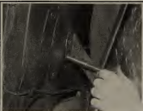
Fig. 9 It's very important to have the hood proper supported when removing the retaining bolts
