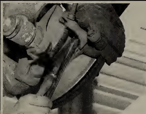
Fig. 54 If necessary, you can remove the entire assembly by loosening the lower caliper bracket bolt
