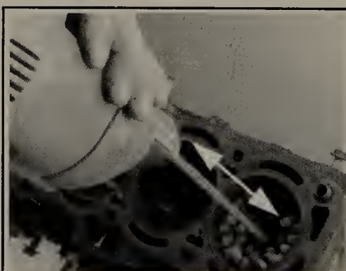
Fig. 150 Use a ball type cylinder hone to remove any glaze and provide a new surface for seating the piston rings
