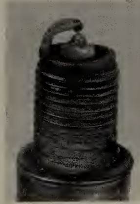
A physically damaged spark plug may be evidence of severe detonation in that cylinder. Watch that cylinder carefully between services, as a continued detonation will not only damage the plug, but could also damage the engine.
