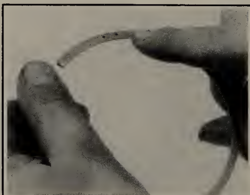
Fig. 158 Most rings are marked to show which side of the ring should face up when installed to the piston
