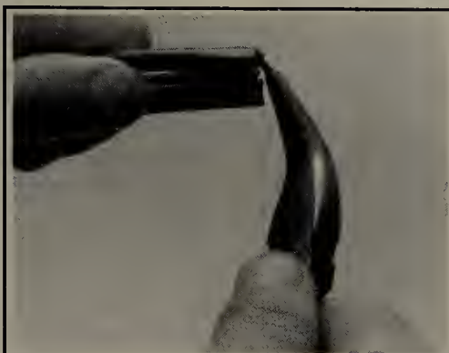
Fig. 139 On Trico® wiper blades, the tab at the end of the blade must be turned up . . .
