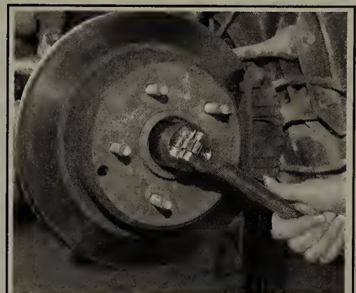
Fig. 65 With an assistant depressing the brakes, loosen the hub nut
