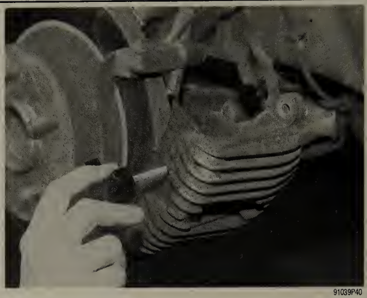
Fig. 35 Another way to push the piston in the caliper bore is to use this type of caliper piston compressor tool
