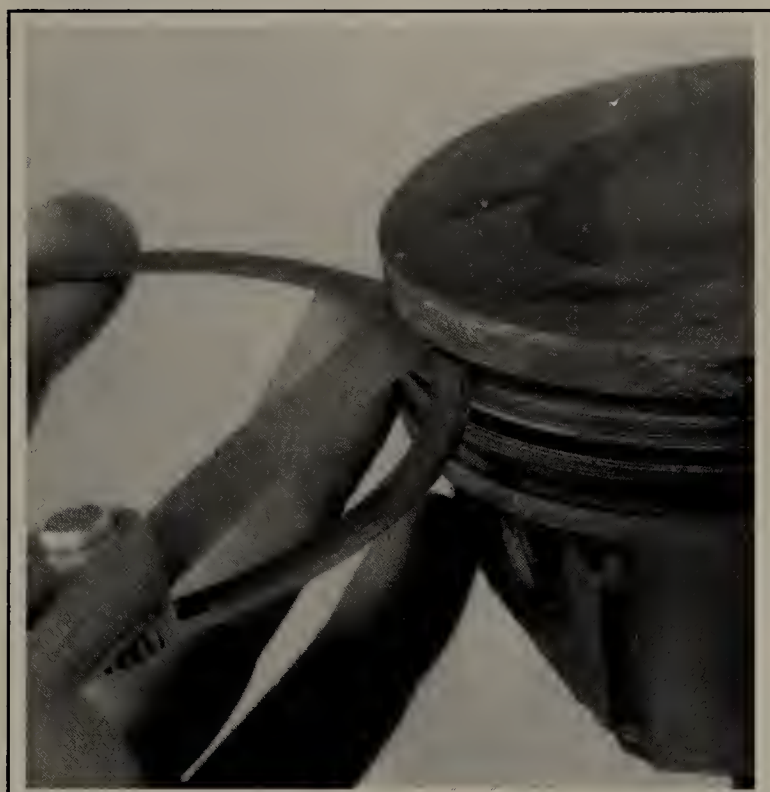
Fig. 156 Checking the piston ring-to-ring groove side clearance using the ring and a feeler gauge
