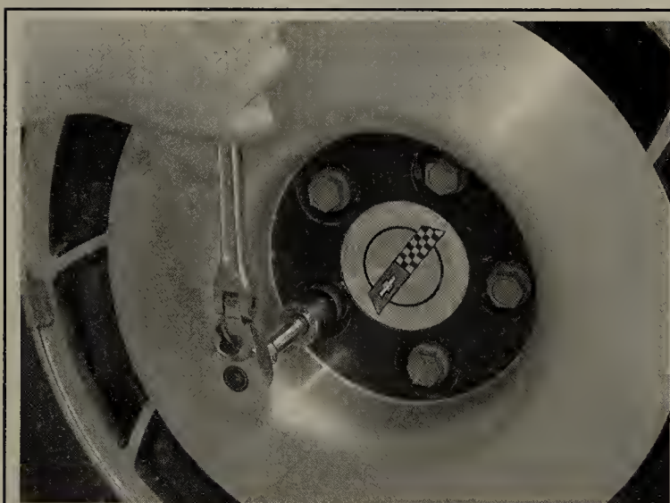
Fig. 1 Use a ratchet with an extension and a 19mm socket to loosen
