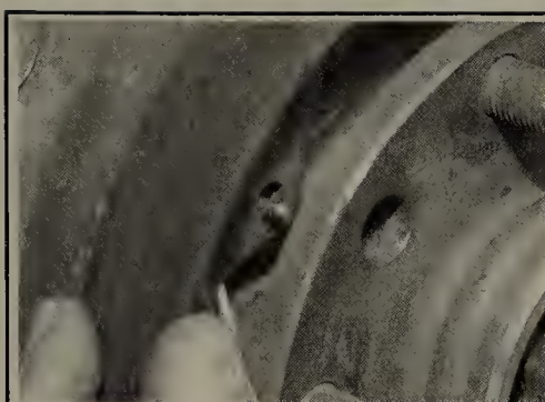
Fig. 91 Carefully place the shoe and lining assembly over the hold-down pins, being careful not to knock them out of the mounting holes
