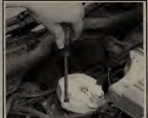
Fig. 123 Unfasten the 2 rotor retaining screws . . .
