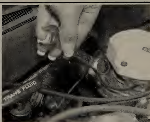
Fig. 18 The easiest way to loosen the distributor hold-down bolt is with a stubby wrench
