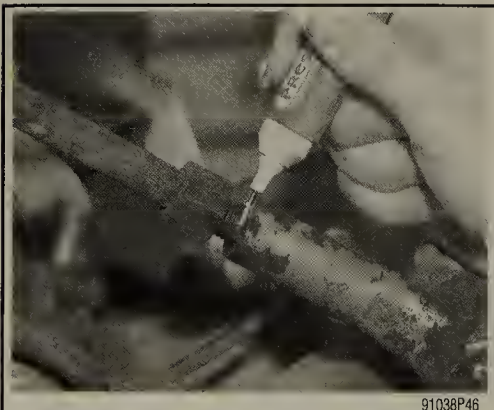
Fig. 88 Make sure you matchmark the installed position of the tie rod end for proper alignment during installation
