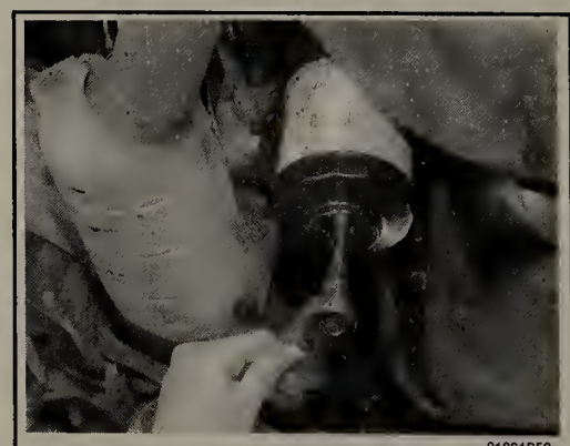
Fig. 165 You can use a cap-type oil filter wrench with a socket to loosen the oil filter
