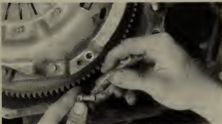
Fig. 22 You may want to use a threadlocking compound on the clutch assembly bolts
