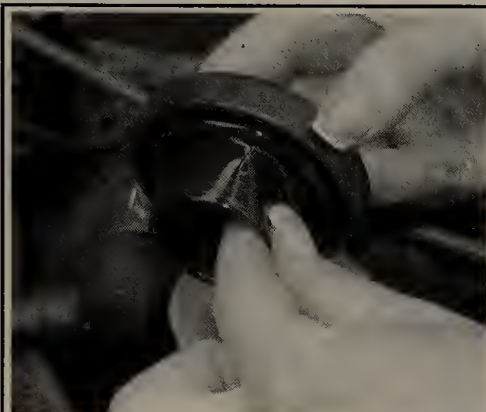
Fig. 211 If the cap diaphragm is extended due to low fluid levels . . .
