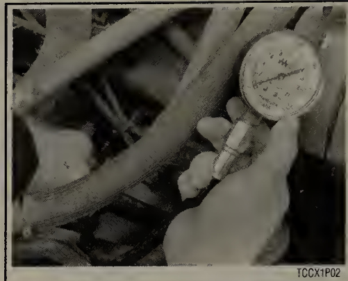
Fig. 12 A screw-in type compression gauge is recommended for compression testing
