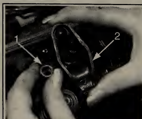
Fig. 59 Remove the rocker arm retaining nut (1) and rocker arm (2)
