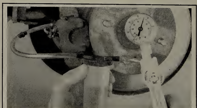
Fig. 72 There are tools, such as this Mighty-Vac, available to assist in proper brake system bleeding
