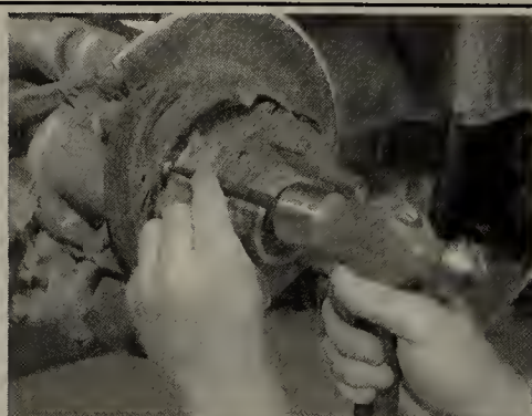
Fig. 88 If the wear shims become slightly distorted, they can usually be carefully tapped back into place
