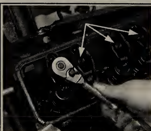
Fig. 58 Loosen the rocker arm nuts (see arrows)
