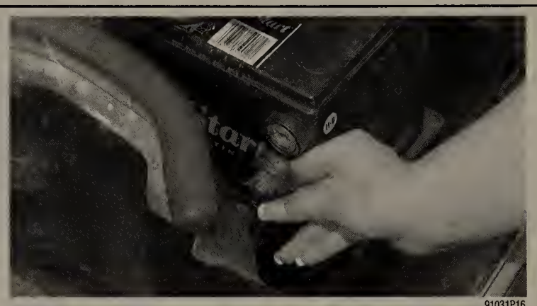
Fig. 77 Make sure to place the cable out of the way so it doesn't accidentally contact the terminal
