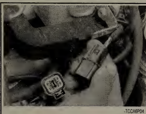
Fig. 6 Weatherproof connectors are most commonly used in the engine compartment or where the connector is exposed to the elements
