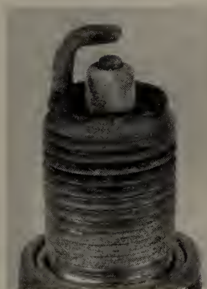
This spark plug has been left in the engine too long, as evidenced by the extreme gap. Plugs with such an extreme gap can cause misfiring and stumbling accompanied by a noticeable lack of power.
