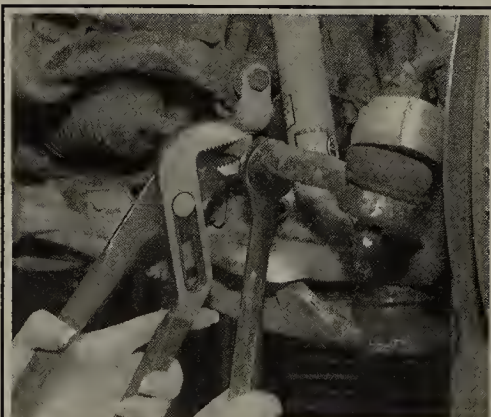
Fig. 89 Use pliers to hold the inner tie rod end, then loosen the jam nut
