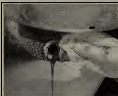
Fig. 164 Also, make sure to clean the oil pan drain plug mating surface
