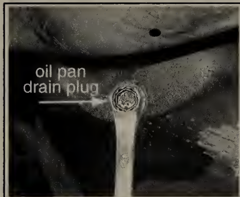
Fig. 160 Use a 13mm box-end wrench or ratchet to loosen the oil pan drain plug
