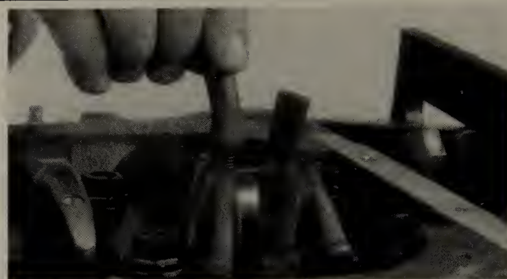
Fig. 146 Place rubber hose over the connecting rod studs to protect the crankshaft and cylinder bores from damage
