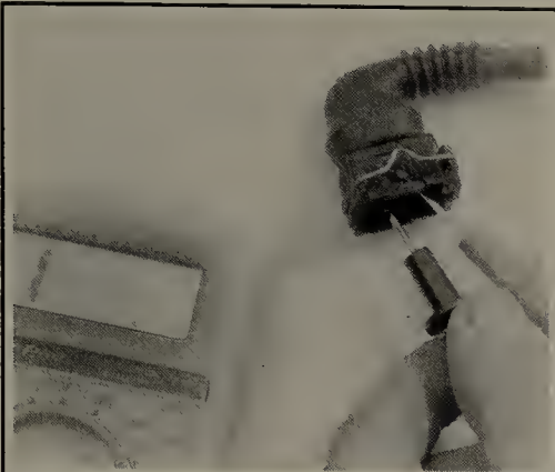
Fig. 8 The infinite reading on this multi-meter indicates that the circuit is open
